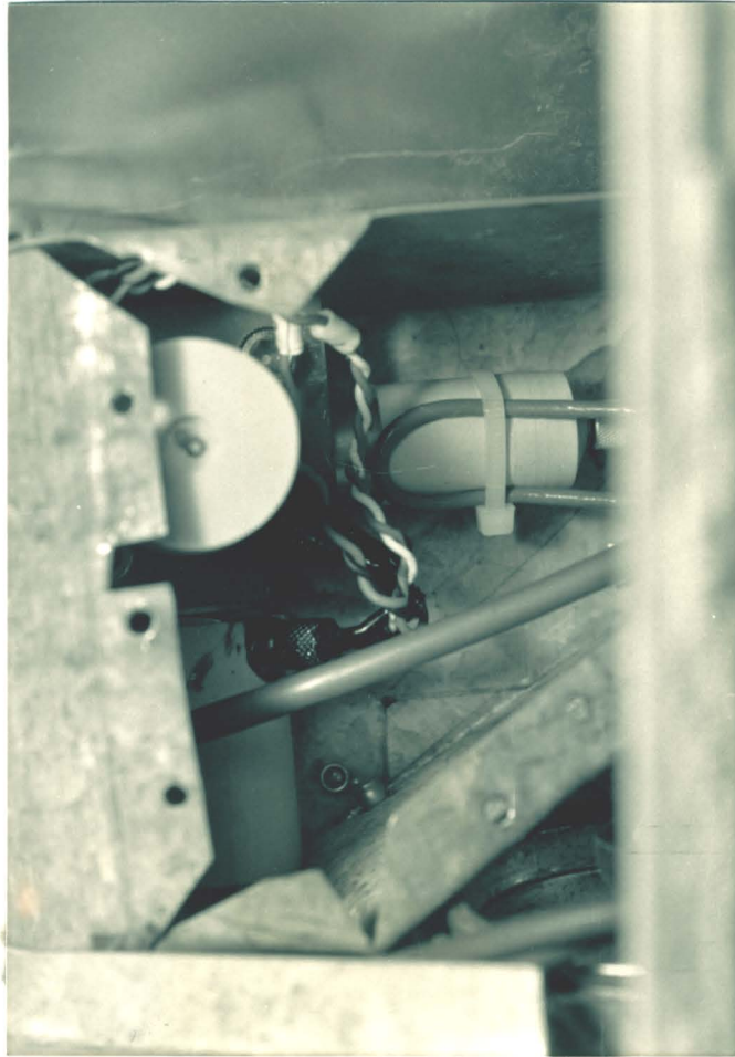
Figure 8 - PCB 312A Mounted on Lamp Frame
