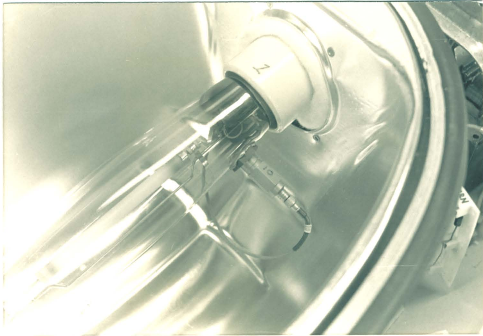
Figure 7 - PCB 312A Mounted on Lamp Surface
