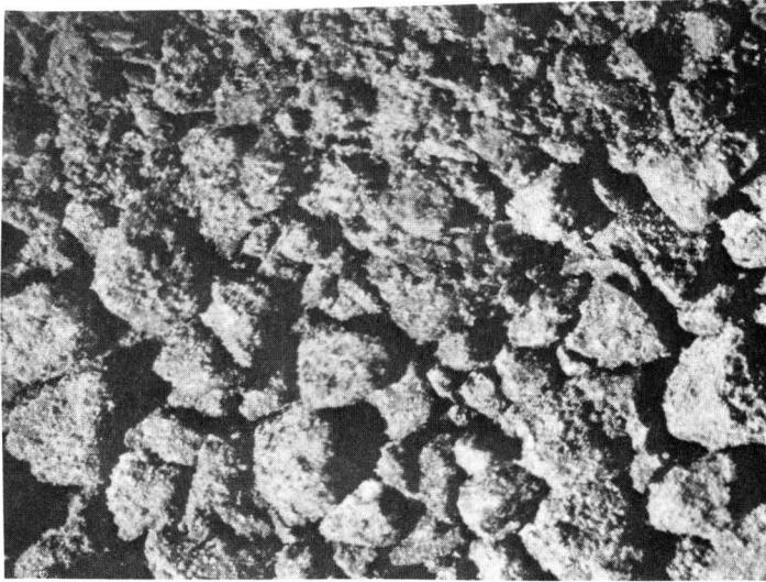
Fig. 25 Soil sample #71-411-R showing clay lumps and fine silt. (Mag. 7.5X)
