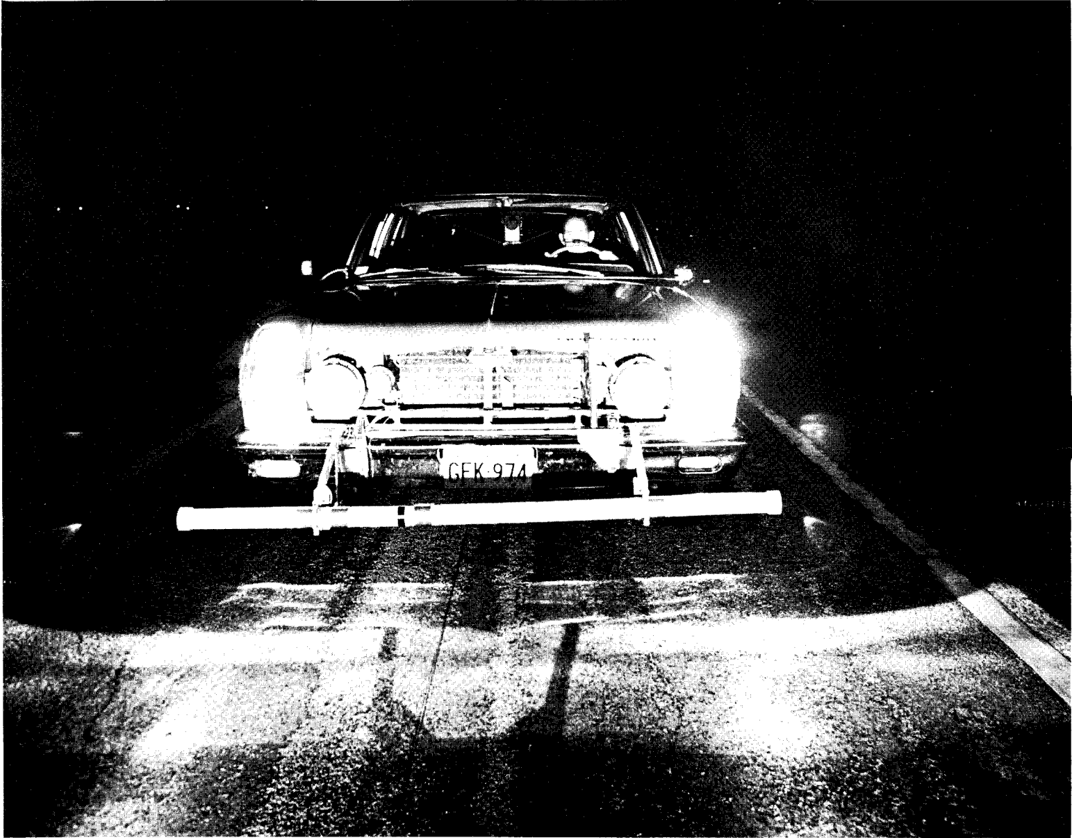
FIGURE 8. LATERAL DEVIATION SENSOR AND ANTENNA (ON ROAD SURFACE)
