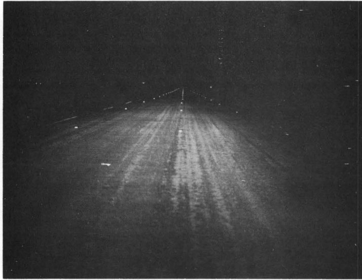
FIGURE 3. NIGHT VIEW OF REFLECTIVE LANE MARKERS VISIBLE ONLY TO GLARE CAR
