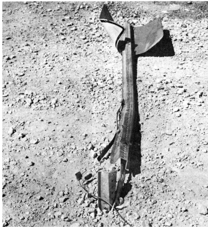
FIGURE 59. EZE-ERECT CONNECTION AFTER TEST 4.
