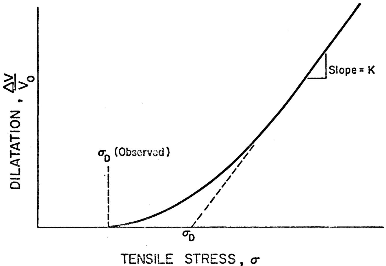
Fig. 14. Typical dilatation vs stress curve.
