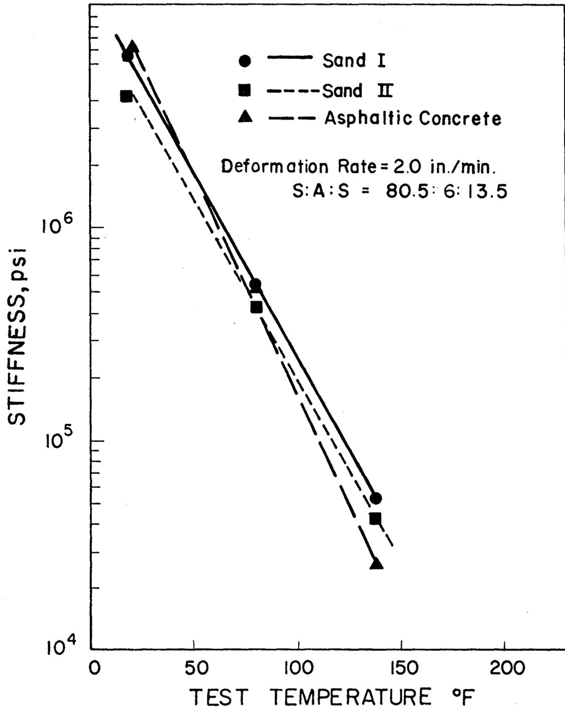
Fig. 19. Stiffness vs temperature for sulphur-asphalt and asphaltic concrete mixtures.
