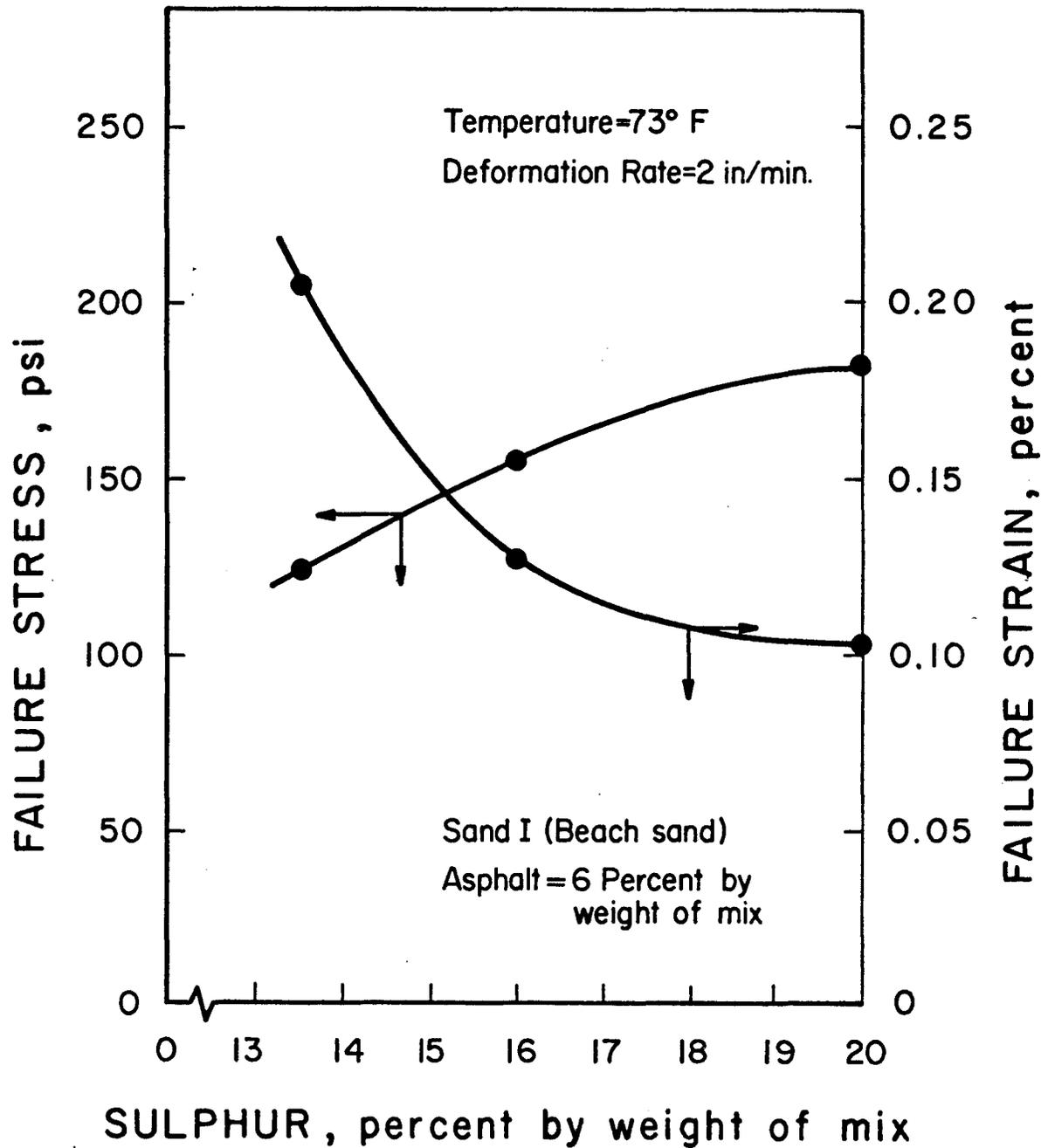
FIG. 17 - Effect of sulphur content on the stress and strain at failure of sand-asphalt-sulphur mixes.
