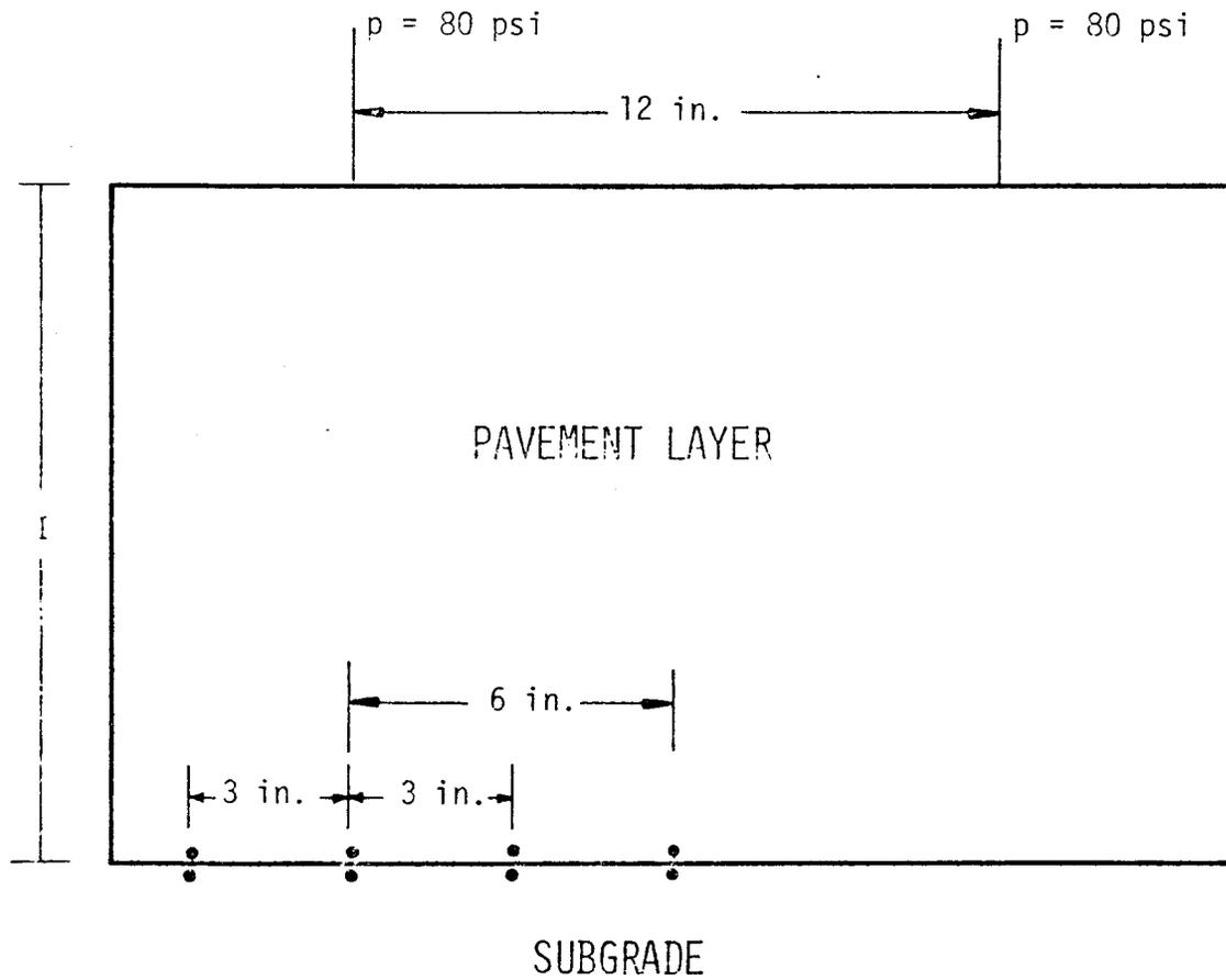
Fig. 21. Typical pavement section used in elastic layered analysis.
