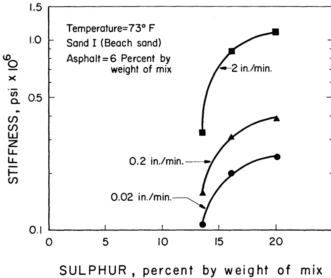
FIG. 16 - Effect of sulphur contents on the stiffness of sand-asphalt-sulphur mixes.
