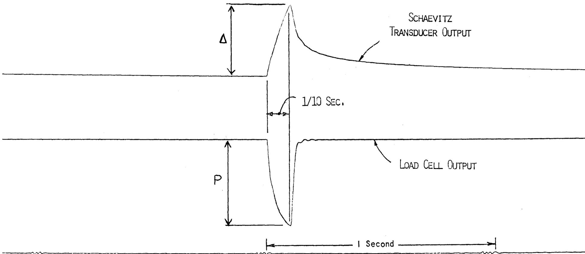
Fig. 8. Typical trace diametral measurement of resilient modulus.
