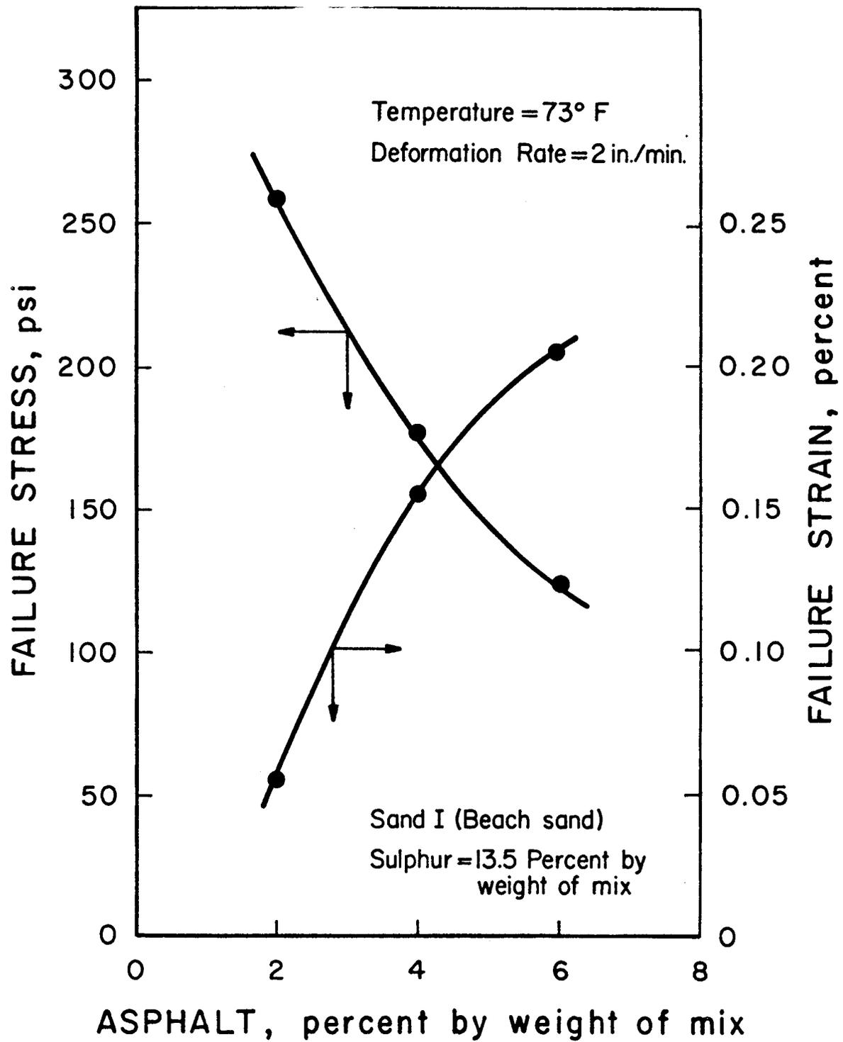
FIG. 18. - Effect of asphalt content on the stress and strain at failure of sand-asphalt-sulphur mixes.
