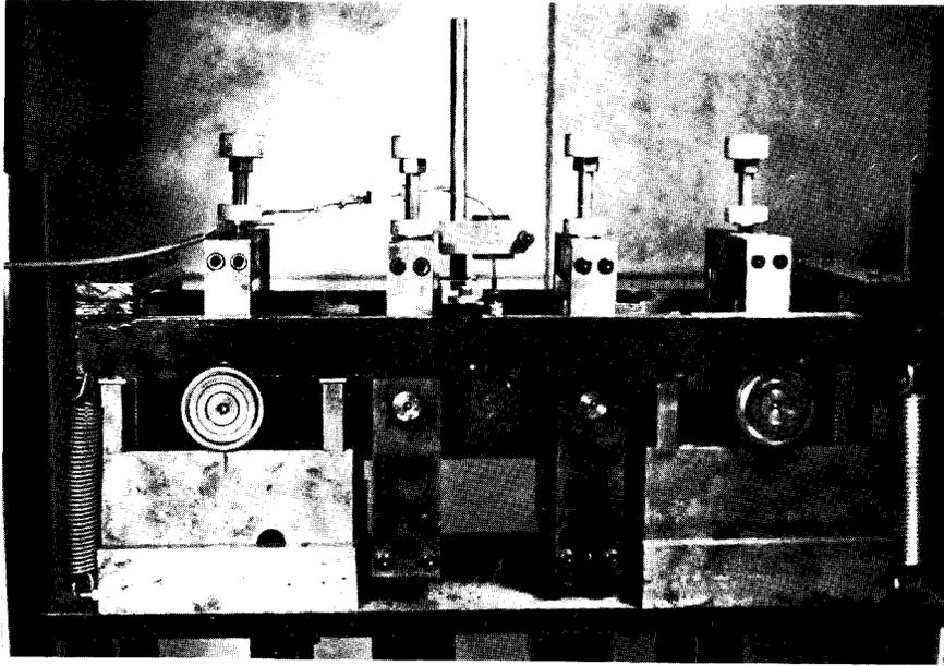
Fig. 3. Third-point flexure fatigue tester
