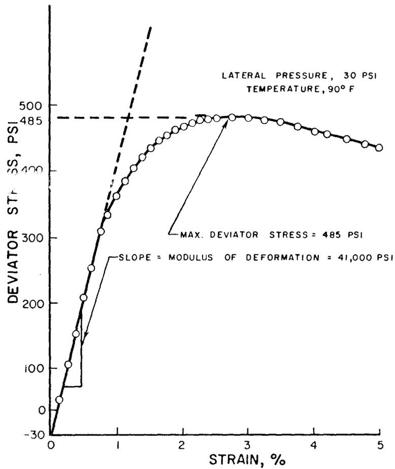
Fig. 10. Typical stress-strain curve (static triaxial test).
