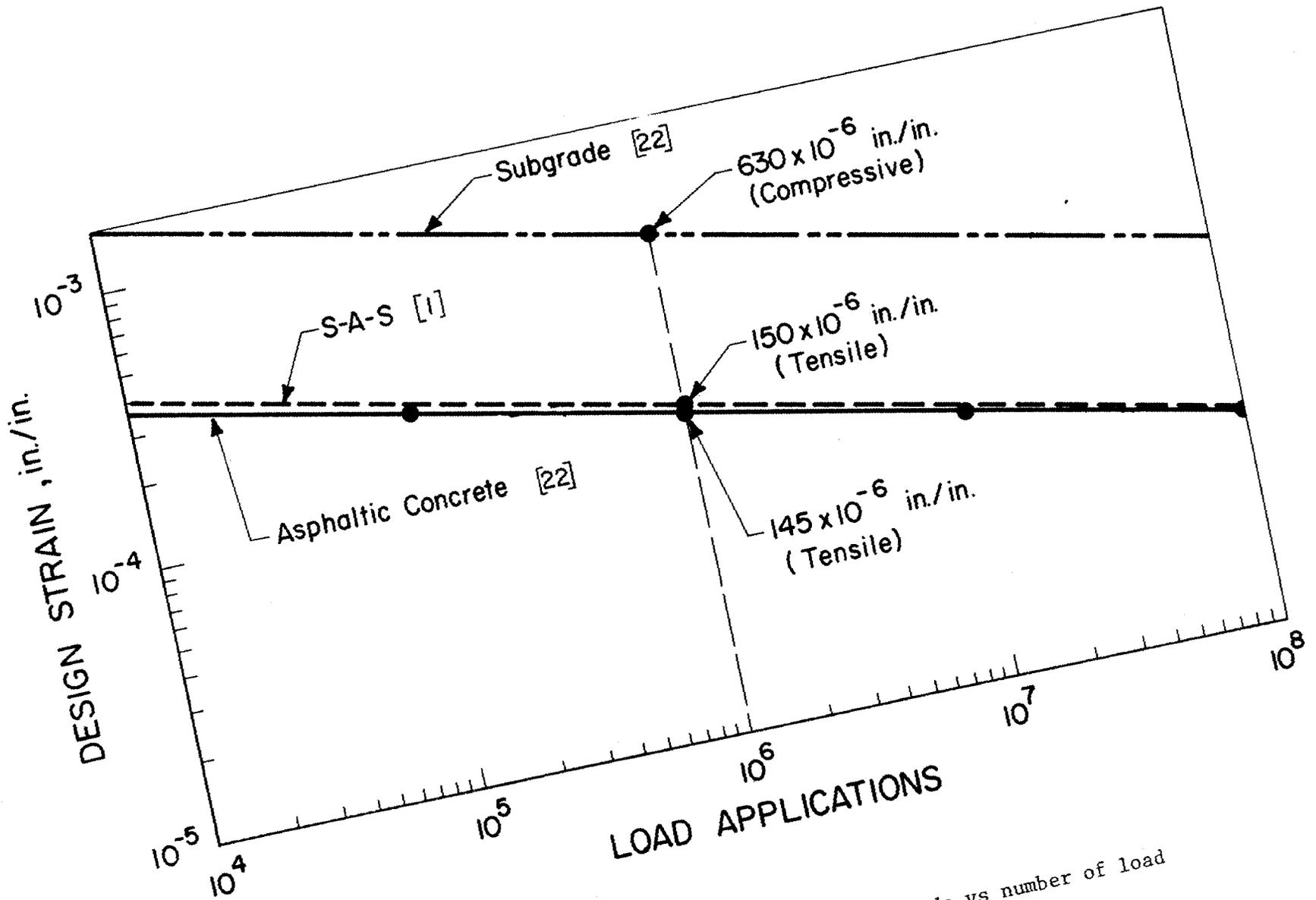
Fig. 22. Design strain of pavement and subgrade vs number of load applications.
