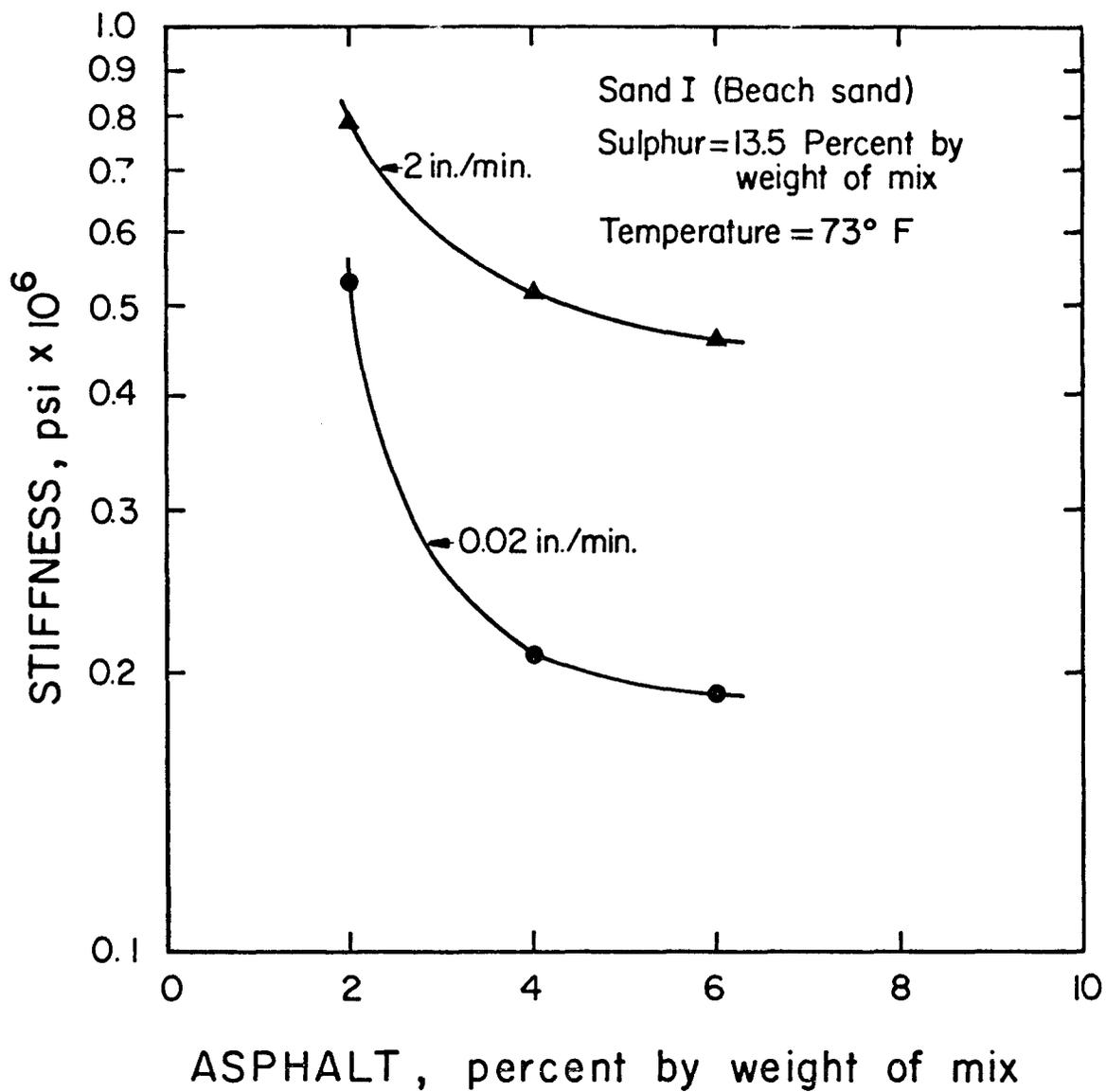
FIG. 15 - Effect of asphalt contents on the stiffness of sand-asphalt-sulphur mixes.
