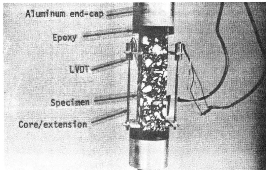
(b) A close-up view of the specimen under test
