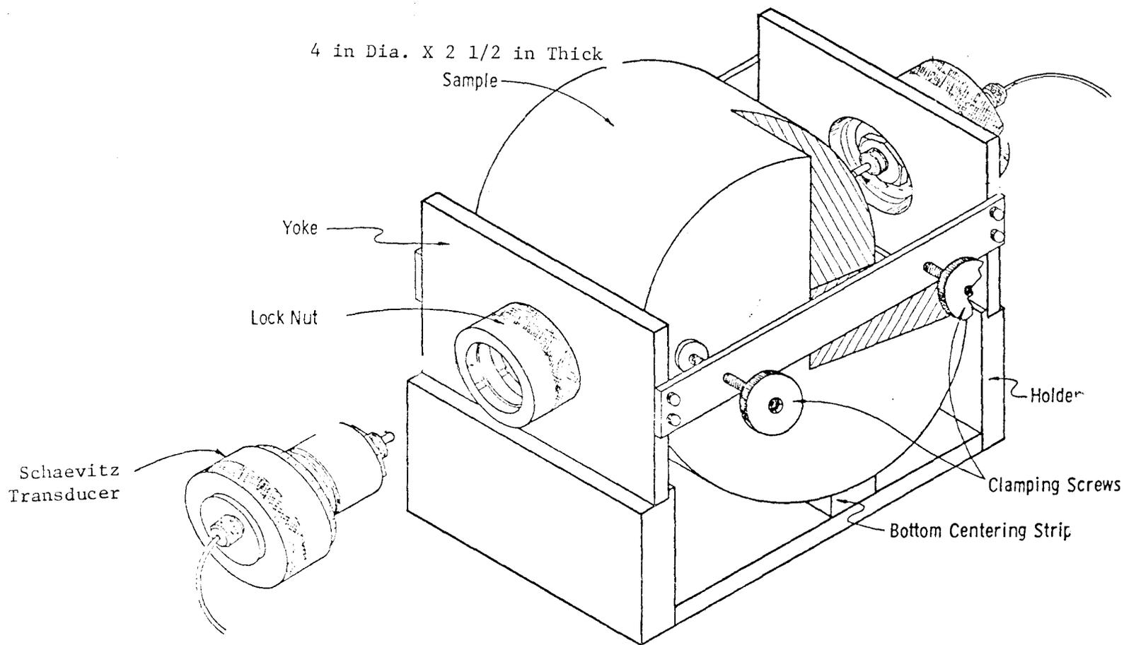
Fig. 7. Diametral resilient modulus device yoke and holder assembly.
