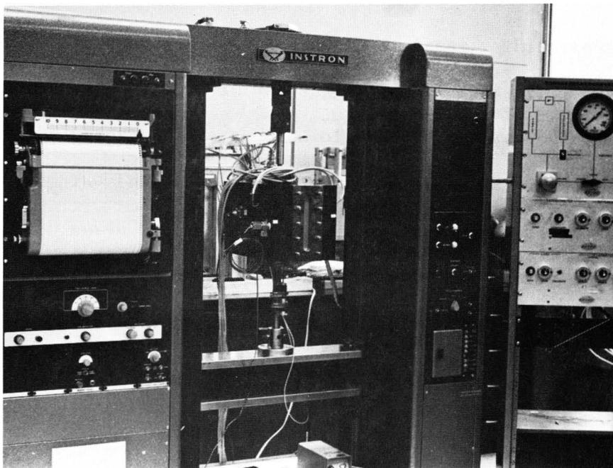
Fig. 13a. Test set-up for dilatation test.
