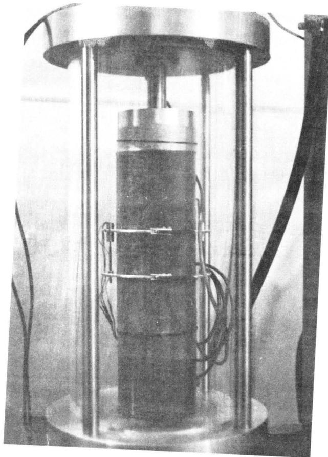
Fig. 9. Triaxial test setup.
