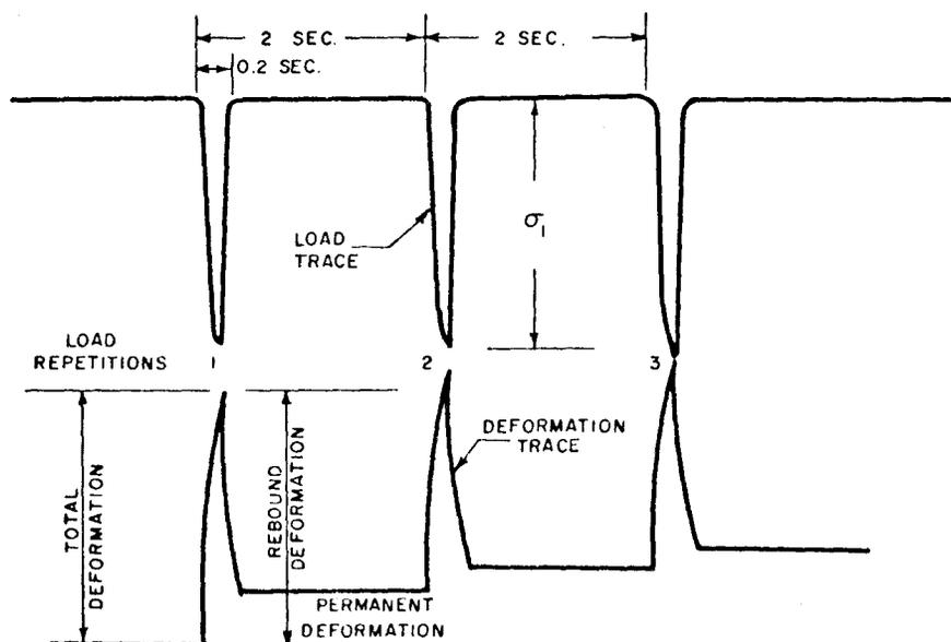
Fig. 11. Typical load-deformation record (repeated load triaxial test).
