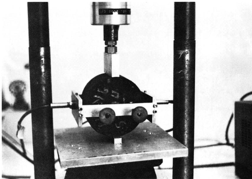
Fig. 6. Diametral resilient modulus ( $M_R$ ) device.
