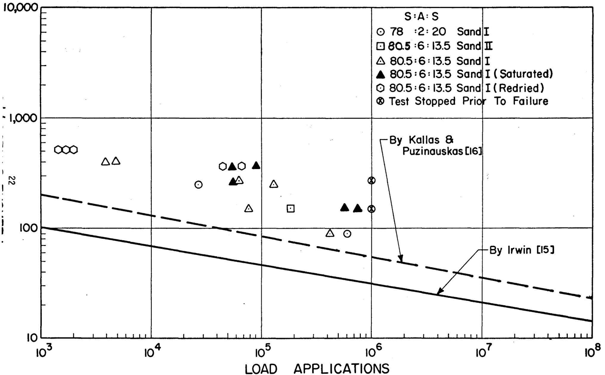
Fig. 20. Comparison of fatigue life of sulphur-asphalt and asphaltic concrete - three-point flexure at constant stress-amplitude.
