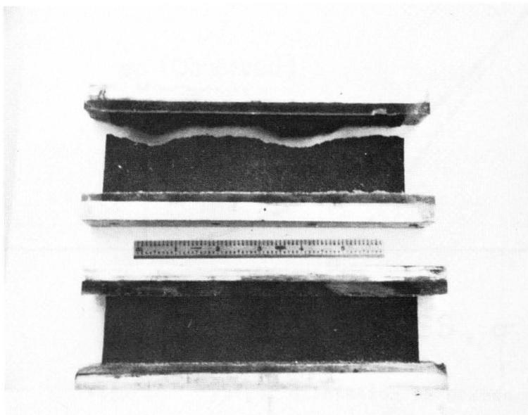
Fig. 13b. Dilatation samples before and after test.
