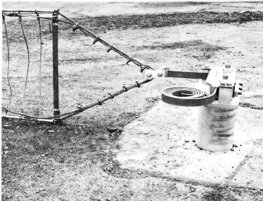
FIGURE IV.1.B.3. METAL BENDER WITH 25,000 LB. TAPE ATTACHED TO NET.
