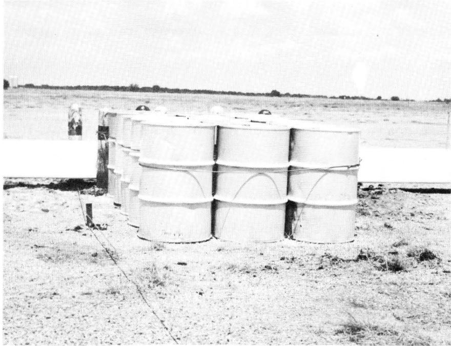
FIGURE IV.2.A.5. FIFTEEN 55-GALLON STEEL DRUMS FILLED WITH EMPTY BEVERAGE CANS BEFORE TEST 505-1C.
