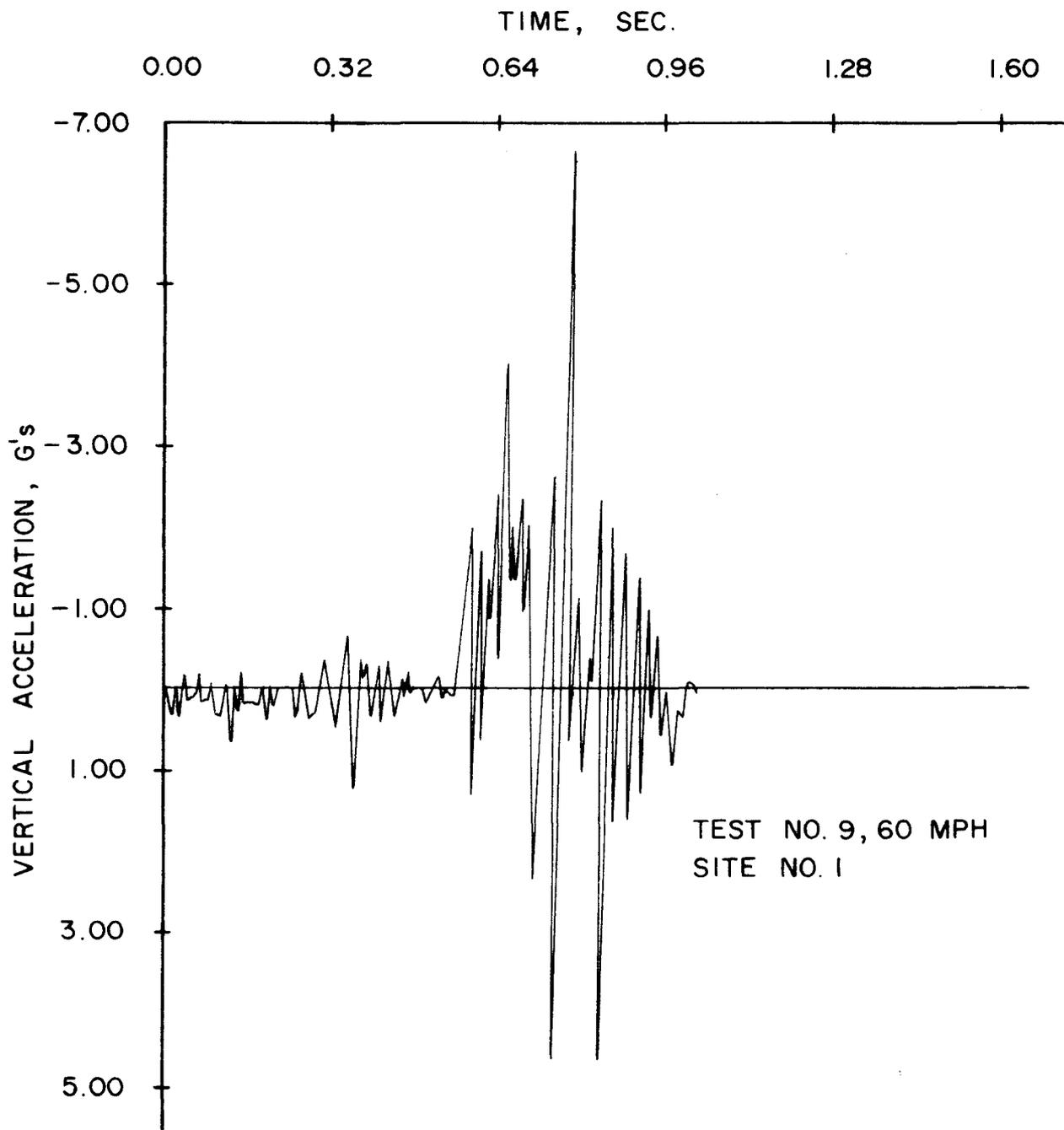
Vertical Acceleration Data from Visicorder (V-Ditch)
