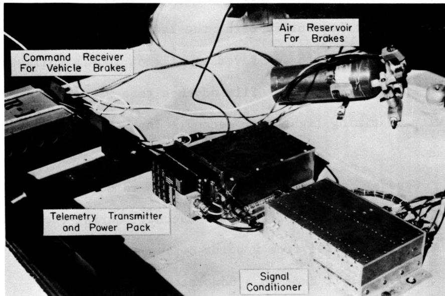
Telemetry Equipment in Trunk of Test Vehicle
