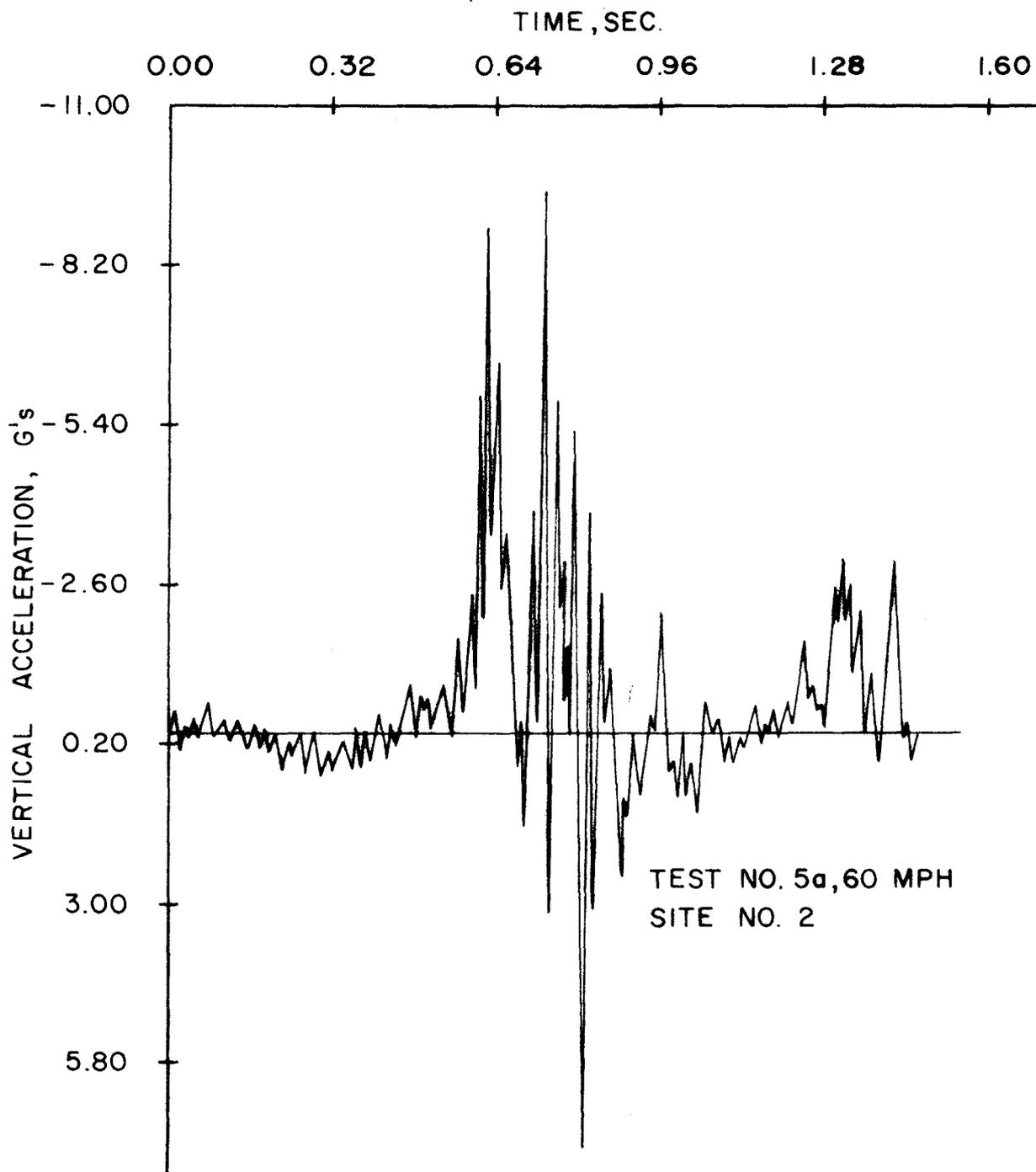
Vertical Acceleration Data from Visicorder (Round Ditch)
