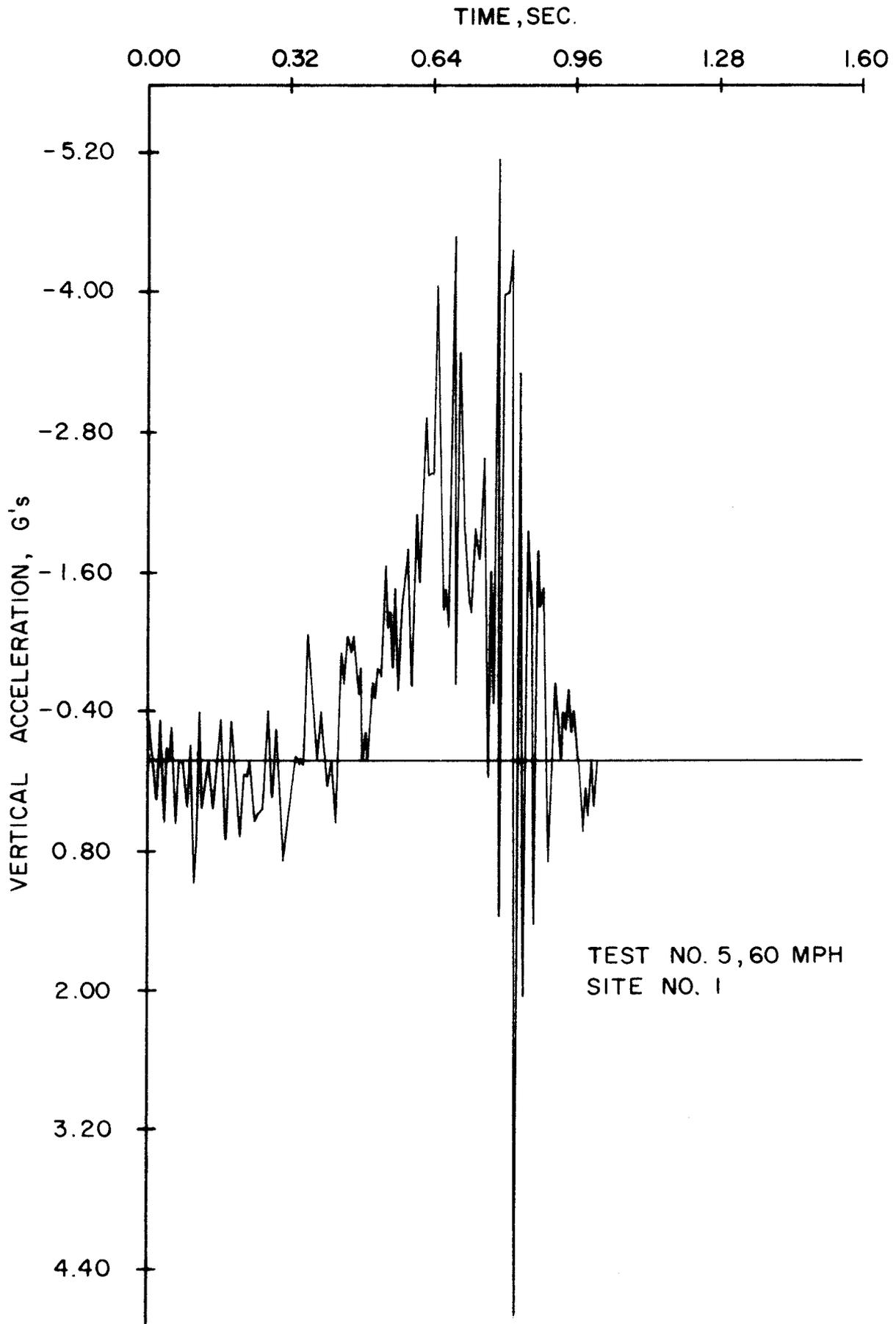
Vertical Acceleration Data from Visicorder (Round Ditch)
