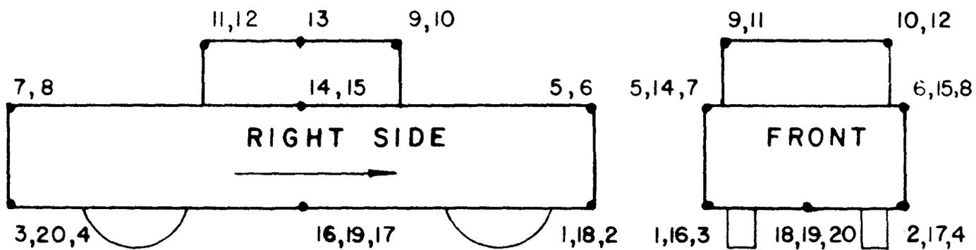
Location of Vehicle Ground-Contact Monitoring Points (1)
