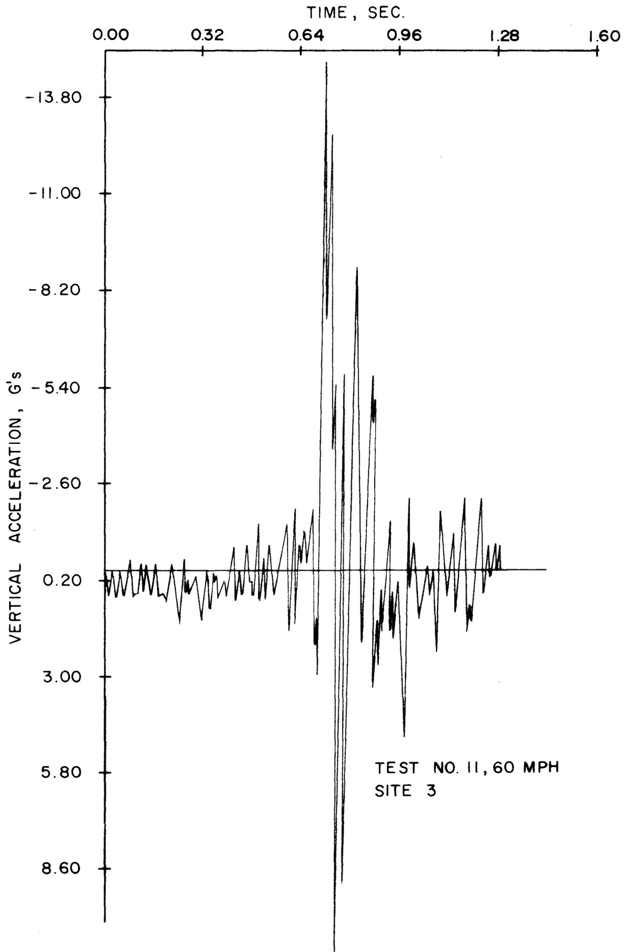
Vertical Acceleration Data from Visicorder (V-Ditch)
