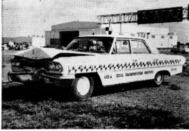
Test 605-A Impact Speed 25.7 mph Penetration 12 inches
