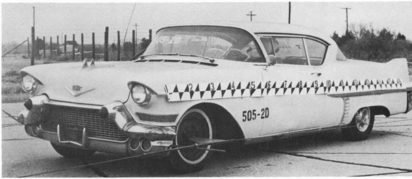
FIGURE 17. VEHICLE BEFORE COLLISION. TEST 2D. 1957 CAD., WEIGHT 5000 LB.
