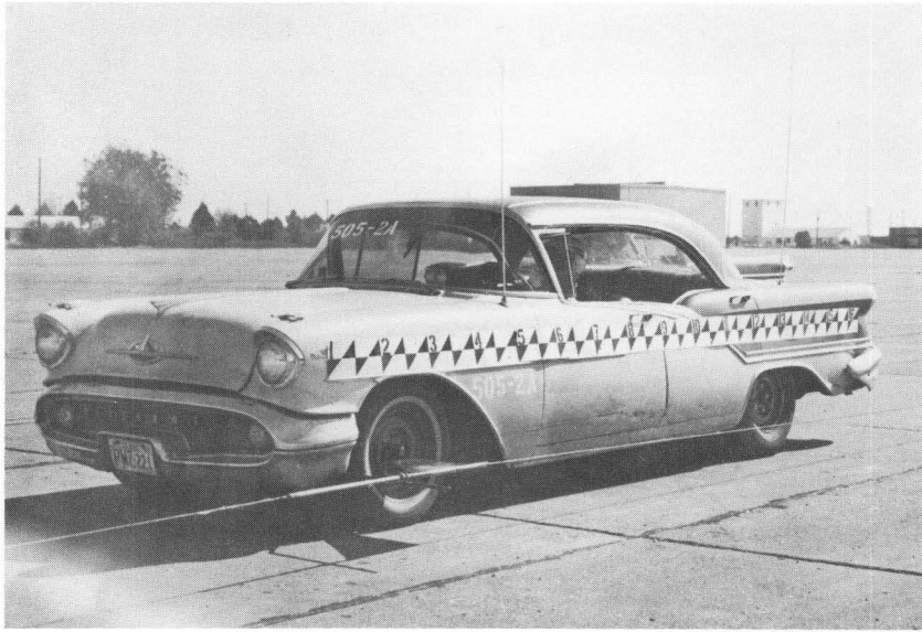
FIGURE 3. VEHICLE BEFORE COLLISION. TEST 2A. 1957 OLDS, WEIGHT 4600 LB.
