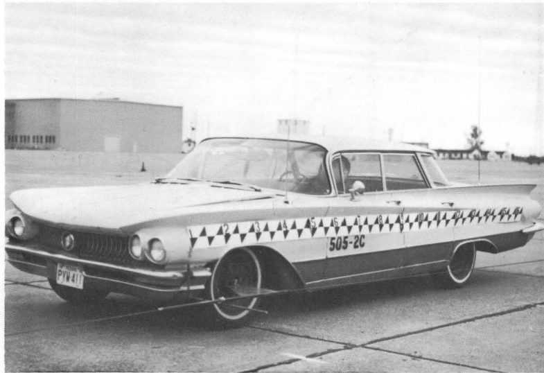
FIGURE 12. VEHICLE BEFORE COLLISION. TEST 2C, 1960 BUICK, WEIGHT 4940 LB.
