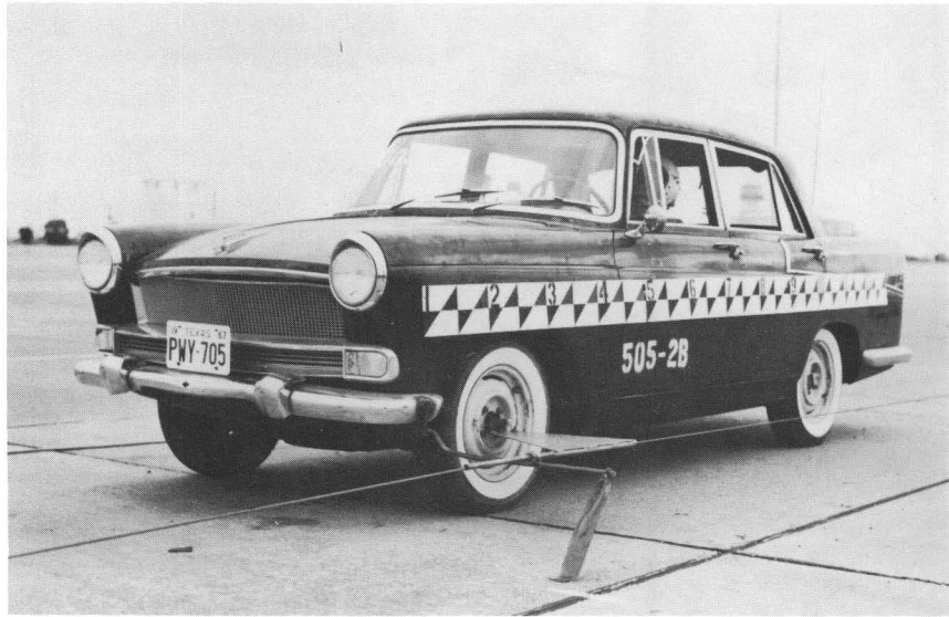
FIGURE 8 . VEHICLE BEFORE COLLISION. TEST 2B, 1957 AUSTIN, WEIGHT 2520 LB.
