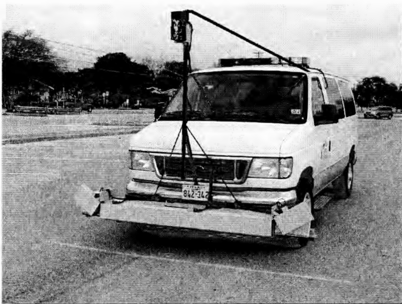
Light bar installed on front bumpers
