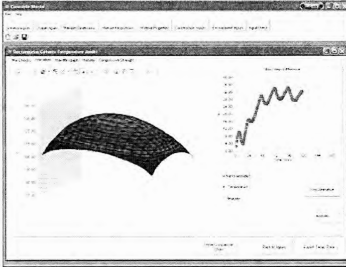
An output screen from ConcreteWorks, graphically representing the temperature distribution within a rectangular column.
