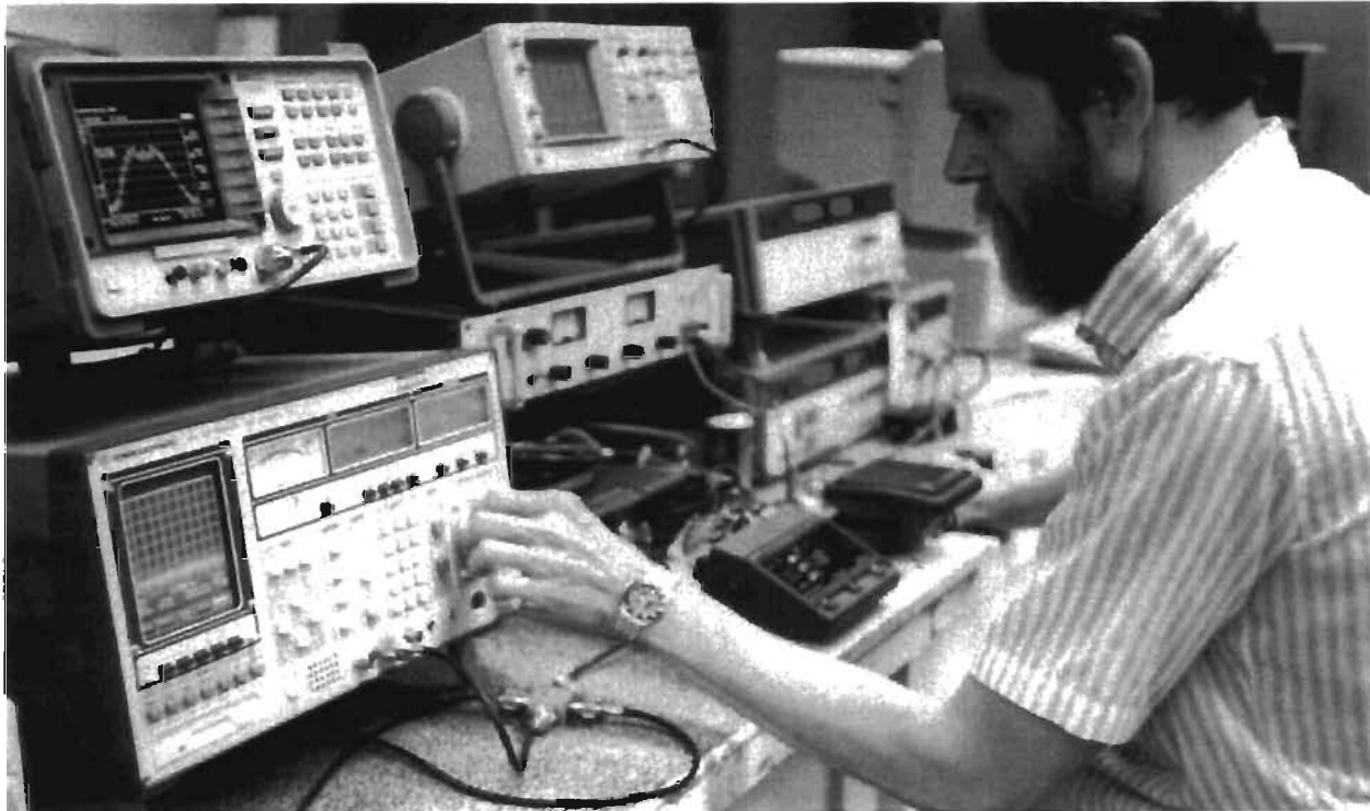
Figure 3. Laboratory evaluation of RF noise with EMI receiver and FM radio
