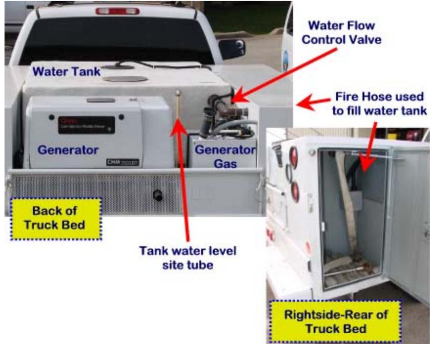
Figure 5 – Equipment locations in bed of truck.
