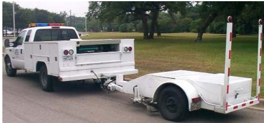
**Figure 1 - Two-wheeled trailer with left wheel path locking tire.**
