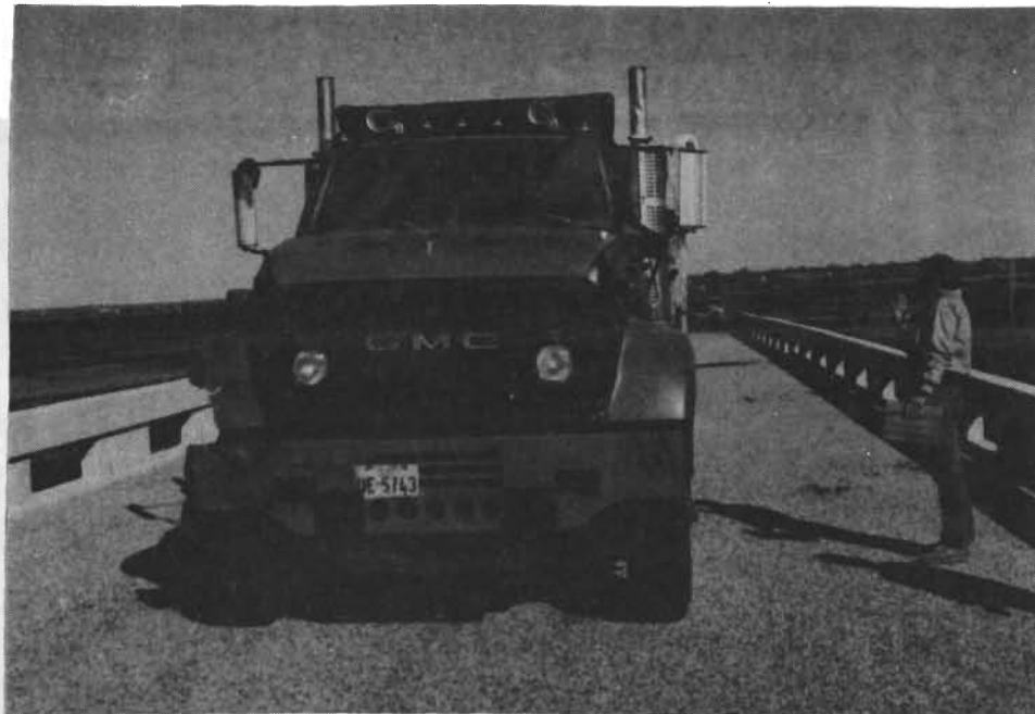
Fig. 3. Positioning of dump truck for simulation of HS20-44 loading
