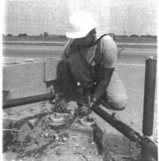
Fig 2.10. Joint width measurement using dial-caliper.
