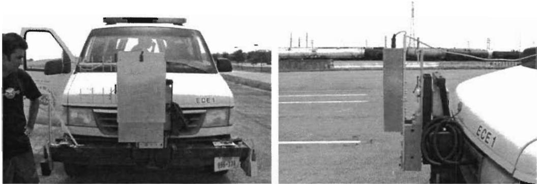
Figure 3, mount the scanning laser device on the vehicle.
