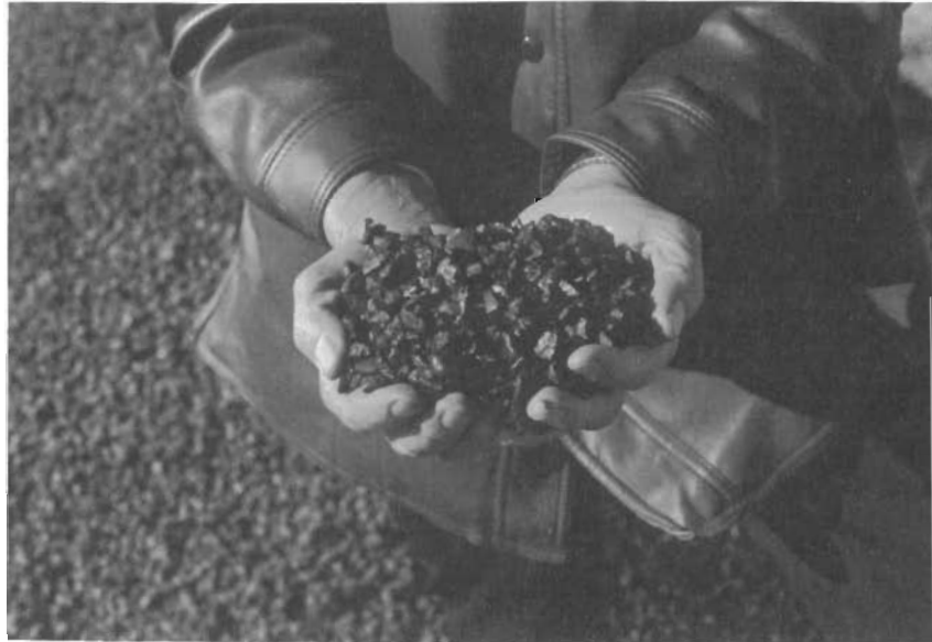
Figure 2 Precoated Sprinkle Treatment Aggregate
