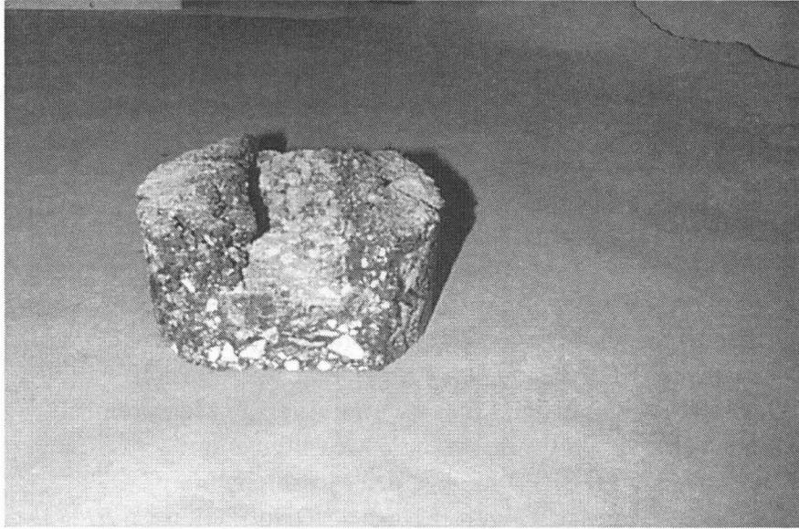
*Figure 3.4 Specimen After HWTD Test (Rough Surface – Low Degradation)*
