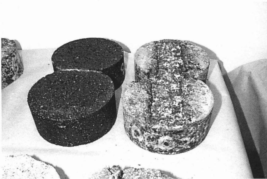
*Figure 3.1 Specimens before and after HWTD Test*
