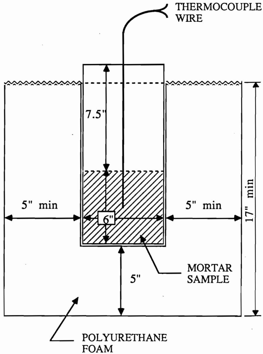
Figure 4.4 Mortar sample insulated by polyurethane foam. Plastic cylinder containing mortar is sealed with a 7.5" deep cylindrical foam plug.
