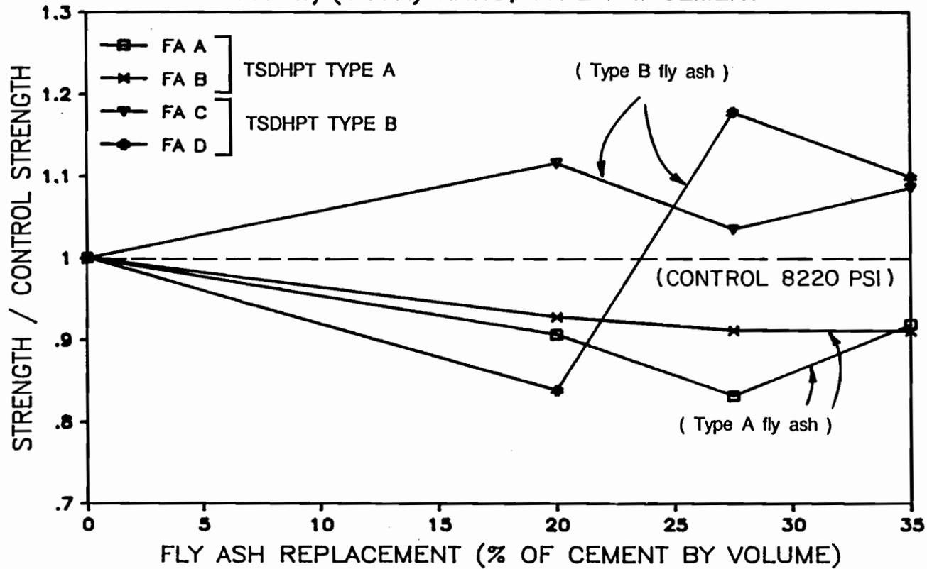
Figure 5.45 Relative compressive strength of Type I-II cement mortars containing fly ash at 28 days.
