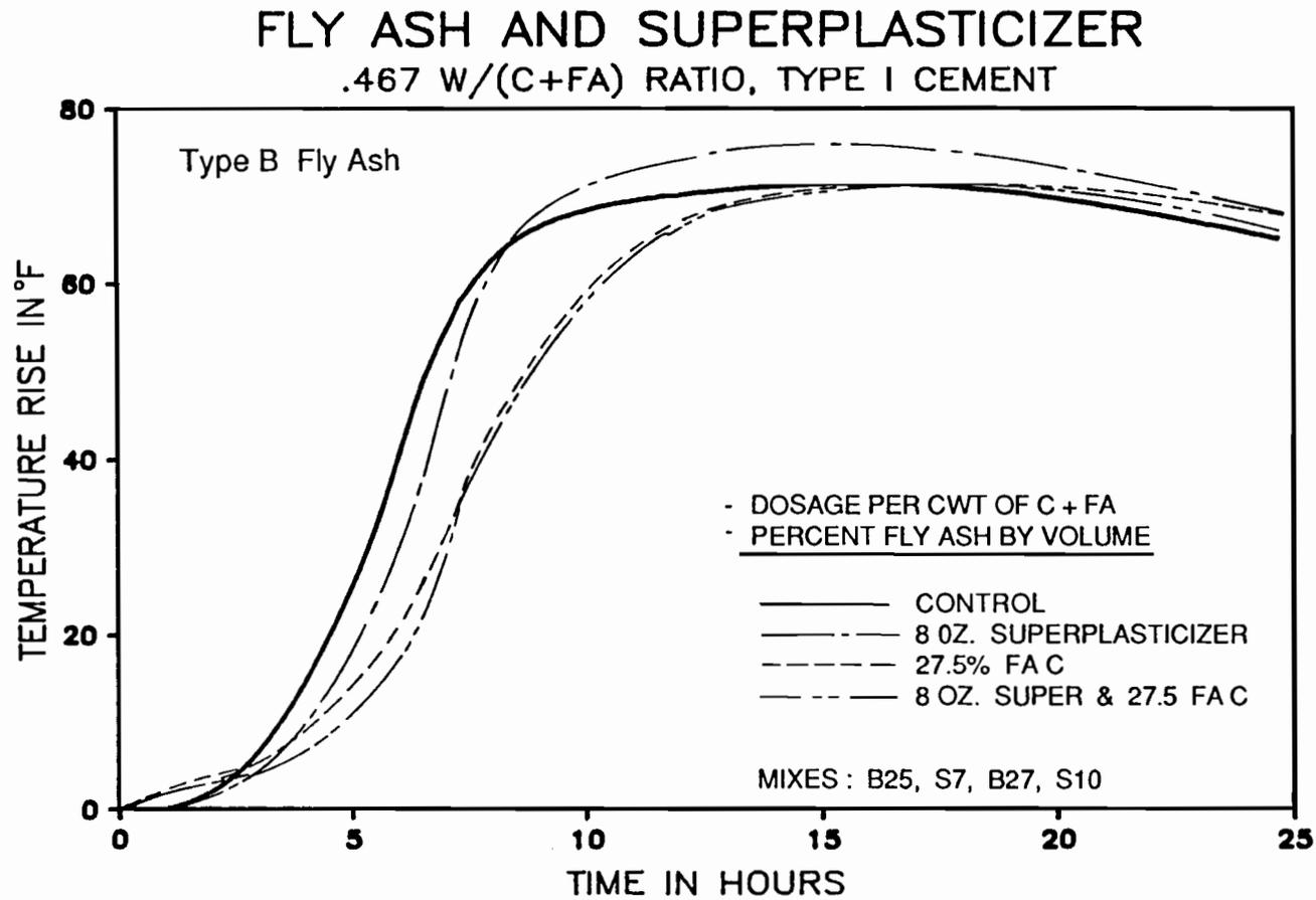
Figure 7.4 Effect of a superplasticizer on the temperature rise in Type I cement mortar with or without Type B fly ash.
