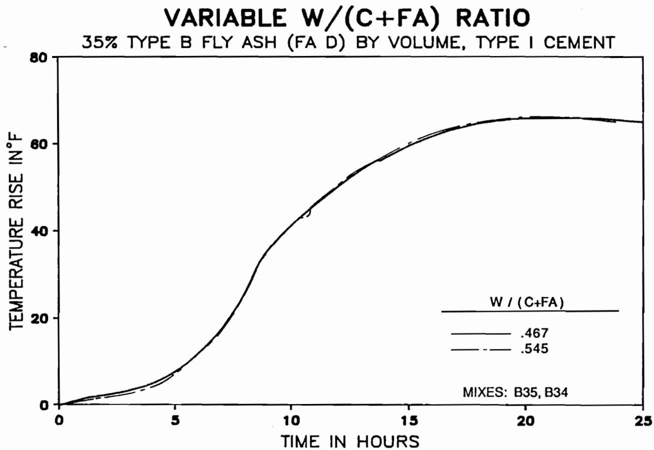
Figure 5.19 Effect of the water to cementitious materials ratio on the temperature rise in mortar containing fly ash.
