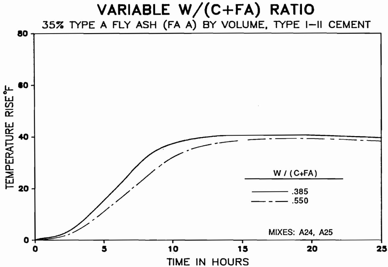
Figure 5.21 Effect of the water to cementitious materials ratio on the temperature rise in mortar containing fly ash.
