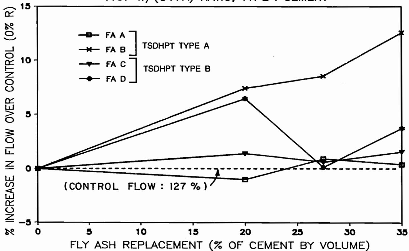
Figure 5.50 Relative flow of Type I cement mortars containing fly ash.
