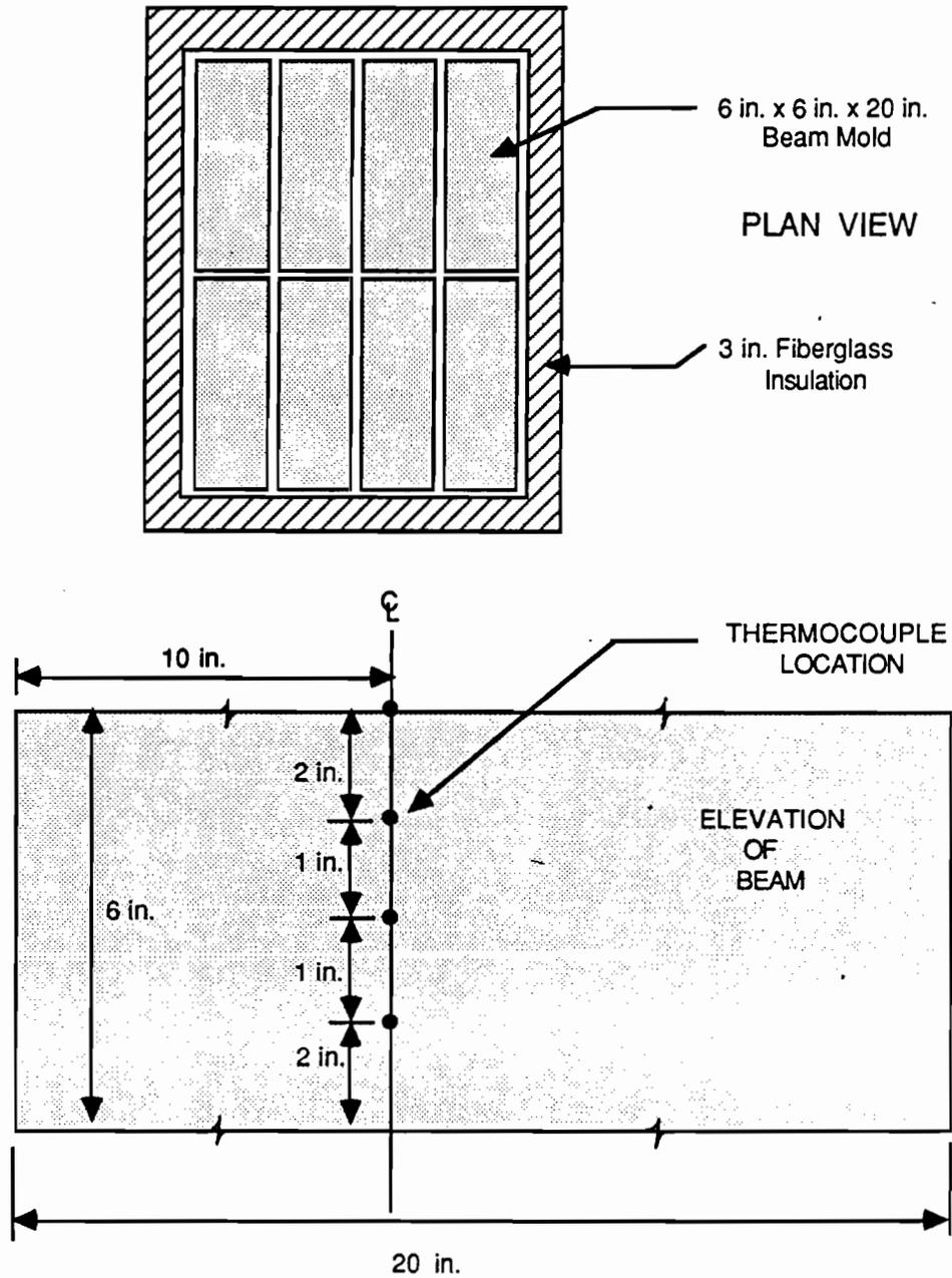
Figure 4.2 Dimensions and thermocouple locations for the samples used in Test 3.
