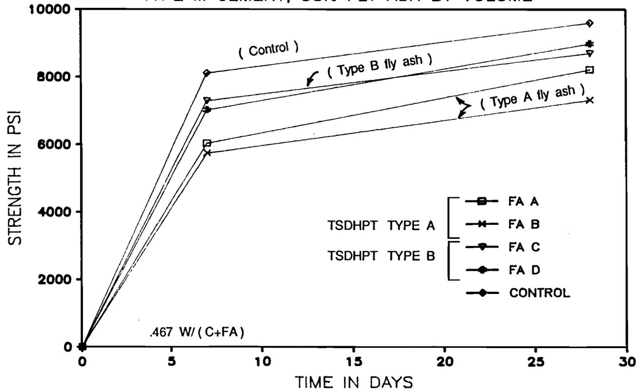
Figure 6.7 Strength development of Type III cement mortars containing fly ash.
