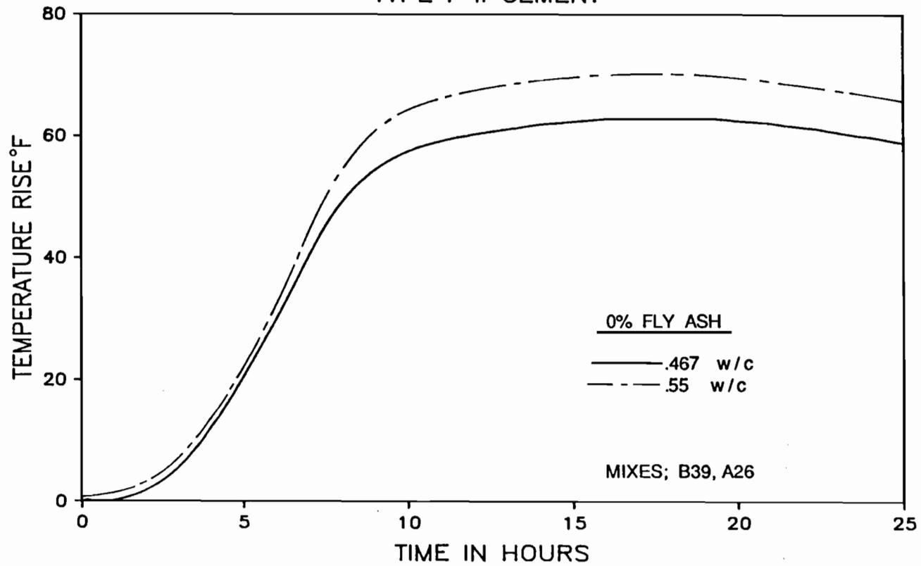
Figure 5.20 Effect of the water to cement ratio on the temperature rise in mortar.
