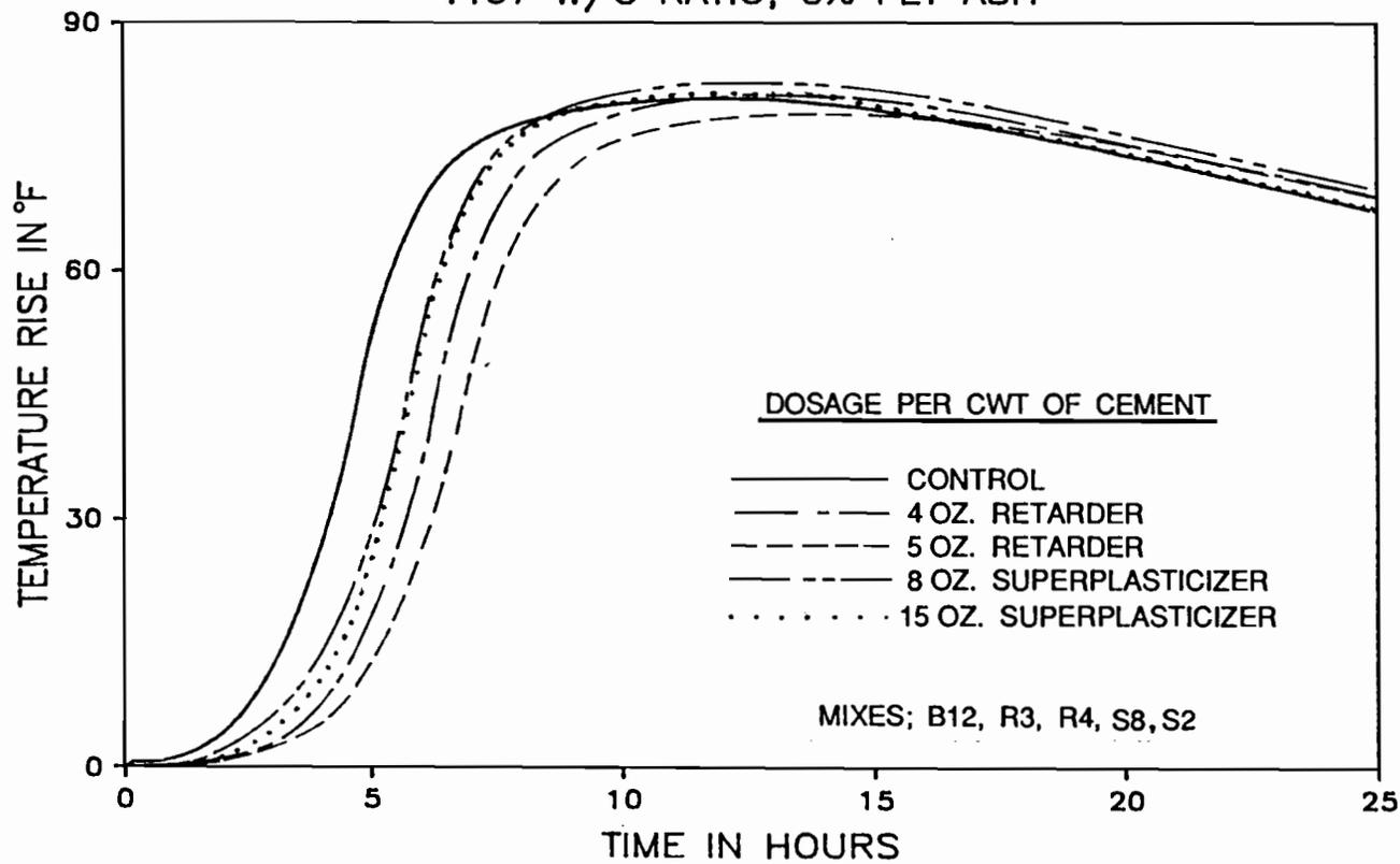
Figure 5.41 Effect of admixture addition on the temperature rise in Type III cement mortar during the initial 25 hours.
