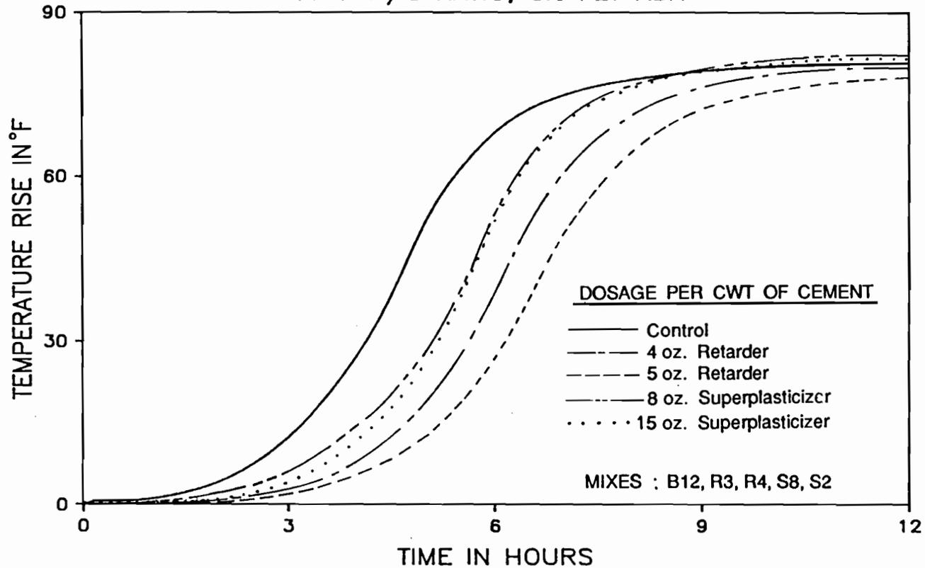
Figure 5.40 Effect of admixture addition on the temperature rise in Type III cement mortar during the initial 12 hours.
