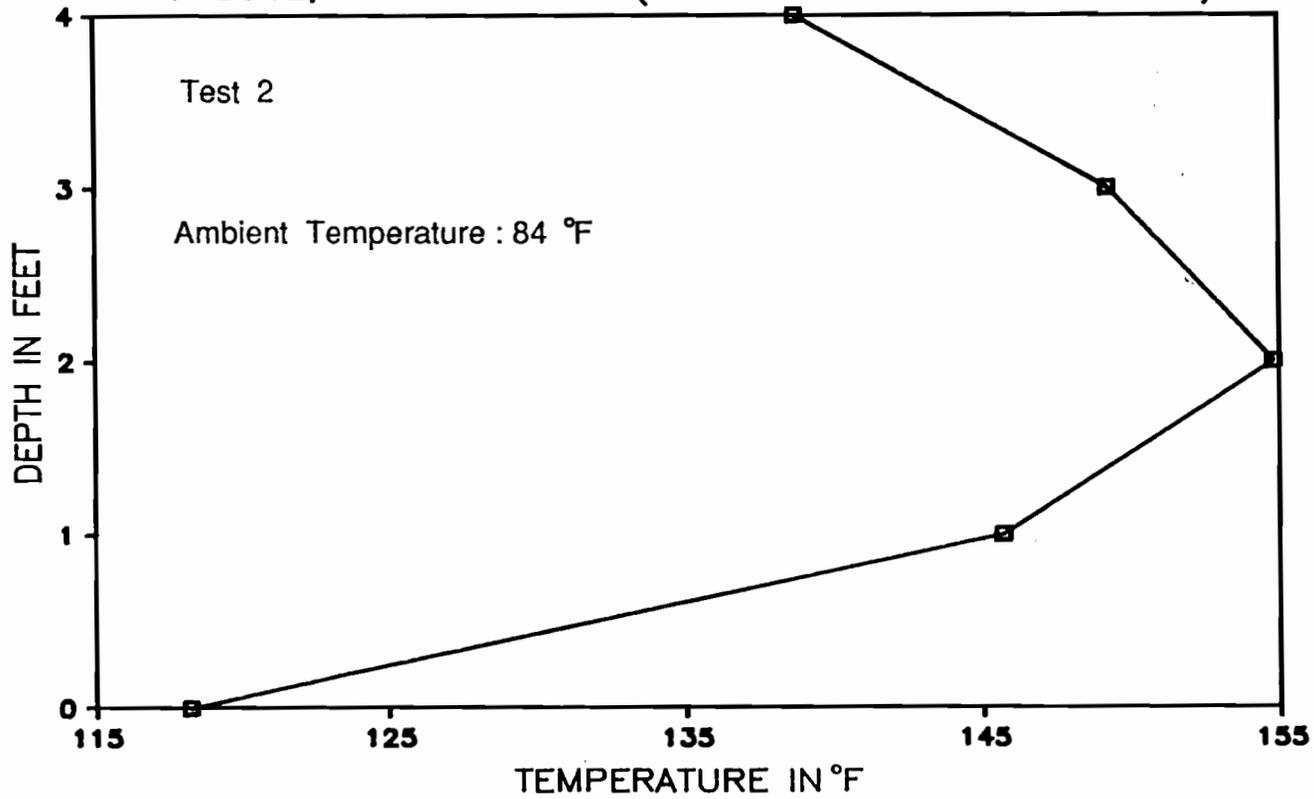
Figure 5.4 Maximum vertical temperature gradient for Test 2.
