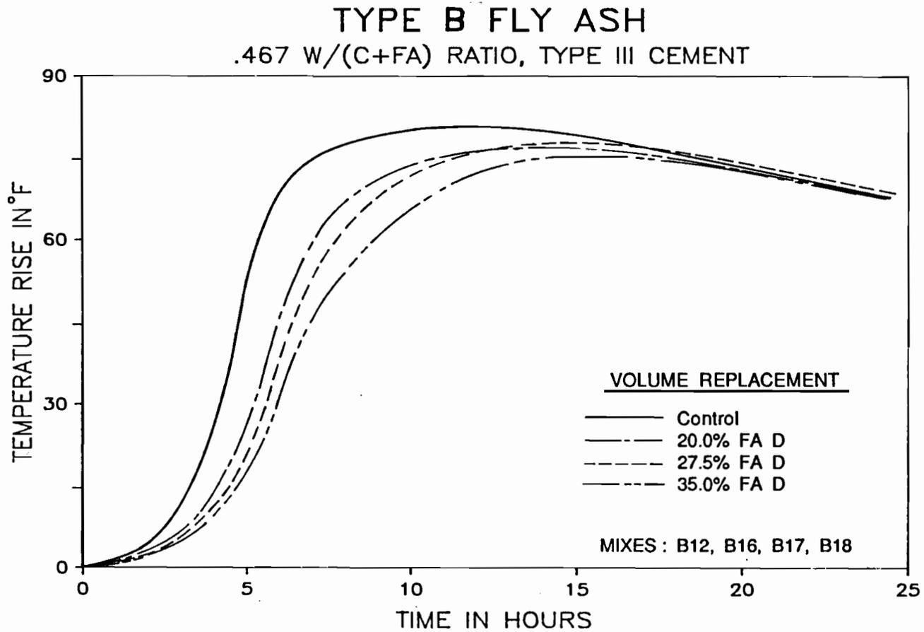
Figure 5.35 Effect of varying content of Type B fly ash on the temperature rise in Type III cement mortar.
