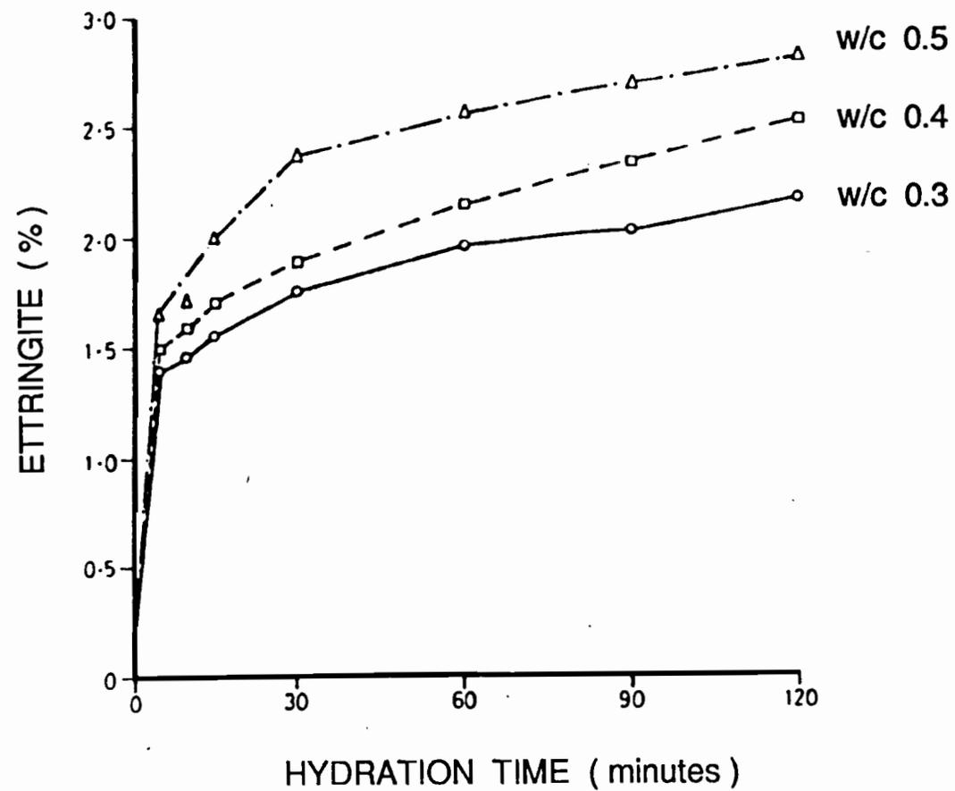
Figure 2.4 Ettringite Production vs. Hydration Time for ordinary Portland cement. [11]
