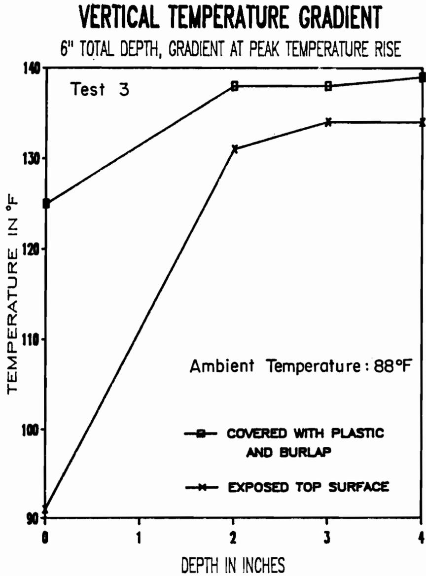
Figure 5.7 Maximum vertical temperature gradients for Test 3 samples.
