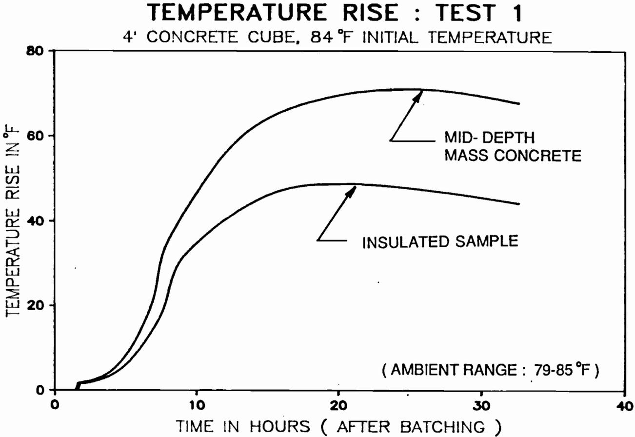
Figure 5.11 Comparison of temperature rise in Test 1 sample to insulated sample.
