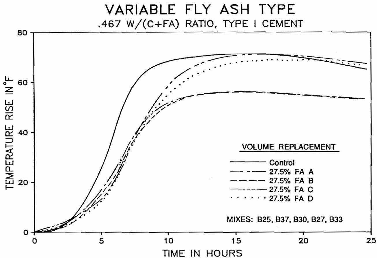
Figure 5.31 Effect of fly ash type on the temperature rise in mortar with 27.5% replacement of Type I cement.
