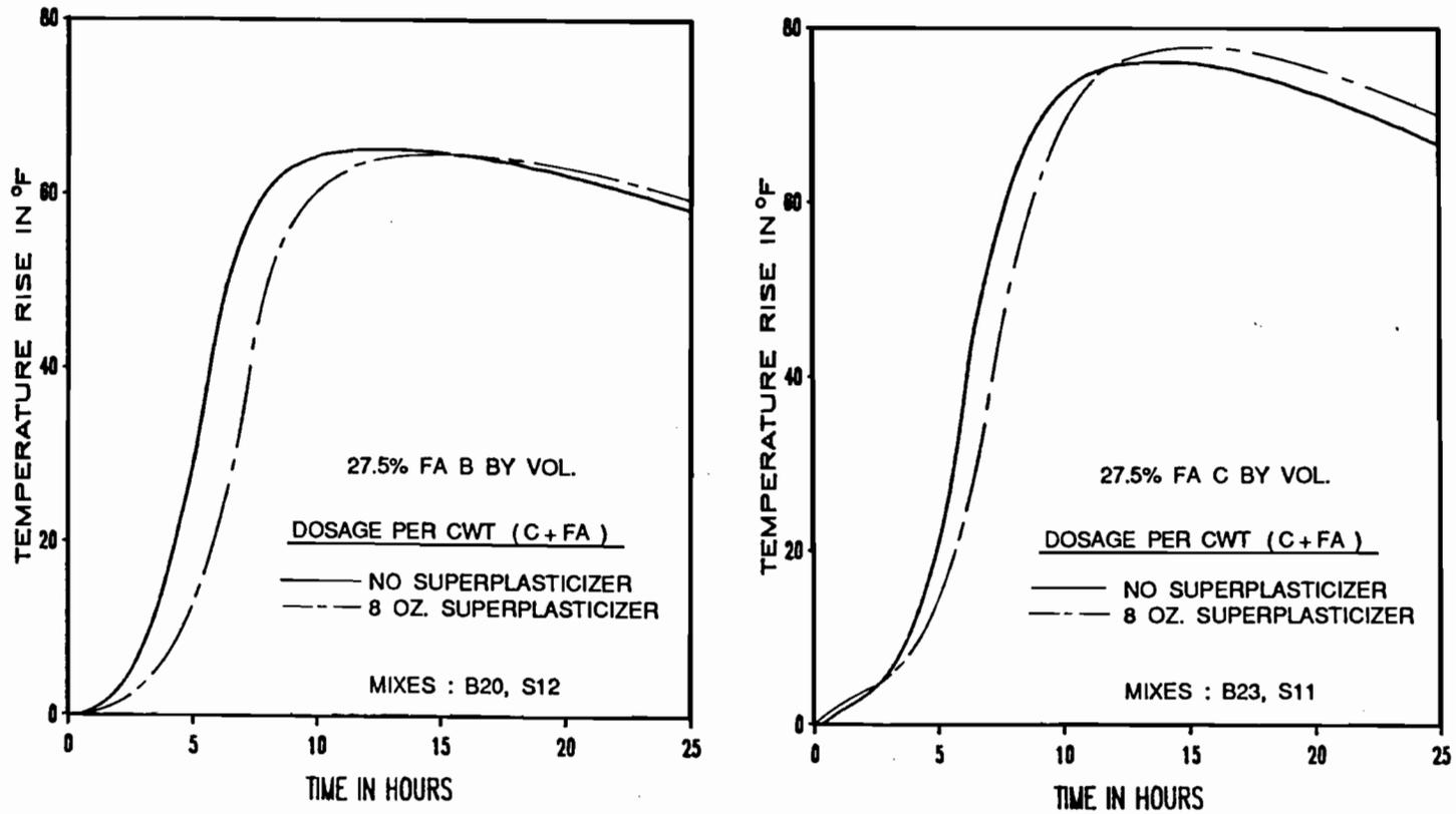
Figure 5.43 Effect of the addition of a superplasticizer on the temperature rise in Type III cement mortar containing fly ash.
