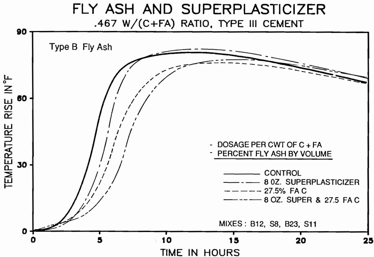
Figure 7.6 Effect of a superplasticizer on the temperature rise in Type III cement mortar with or without Type B fly ash.
