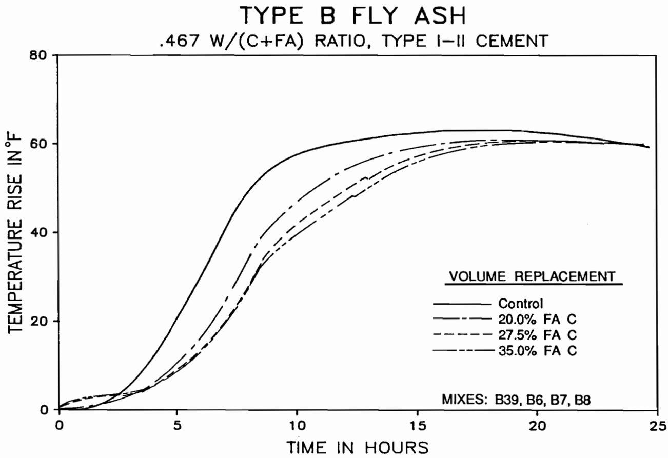
Figure 5.24 Effect of varying content of Type B fly ash on the temperature rise in Type I-II cement mortar.
