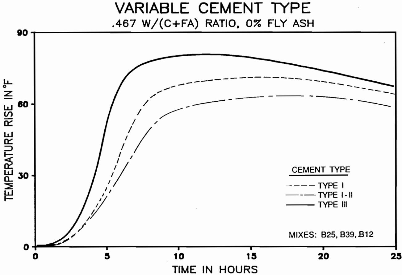
Figure 5.16 Effect of cement type on the temperature rise in mortar.
