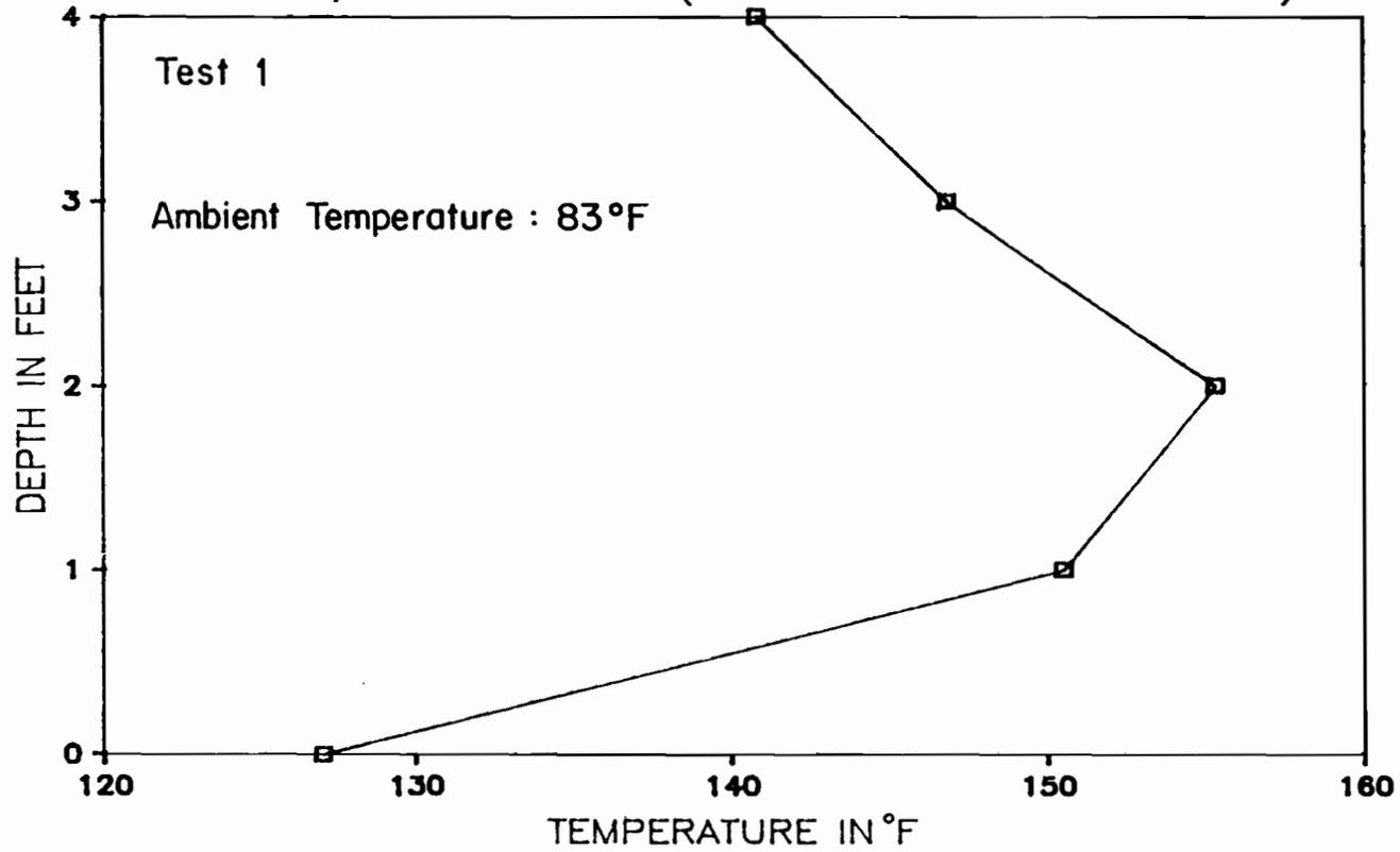
Figure 5.2 Maximum vertical temperature gradient for Test 1.
