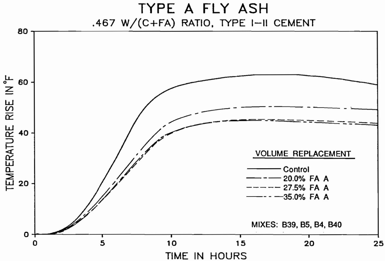
Figure 5.22 Effect of varying content of Type A fly ash on the temperature rise in Type I-II cement mortar.
