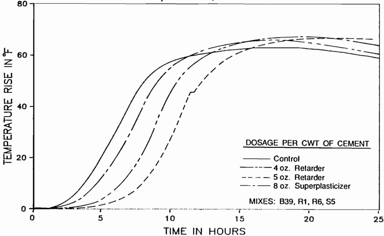
Figure 5.37 Effect of admixture addition on the temperature rise in Type I-II cement mortar.
