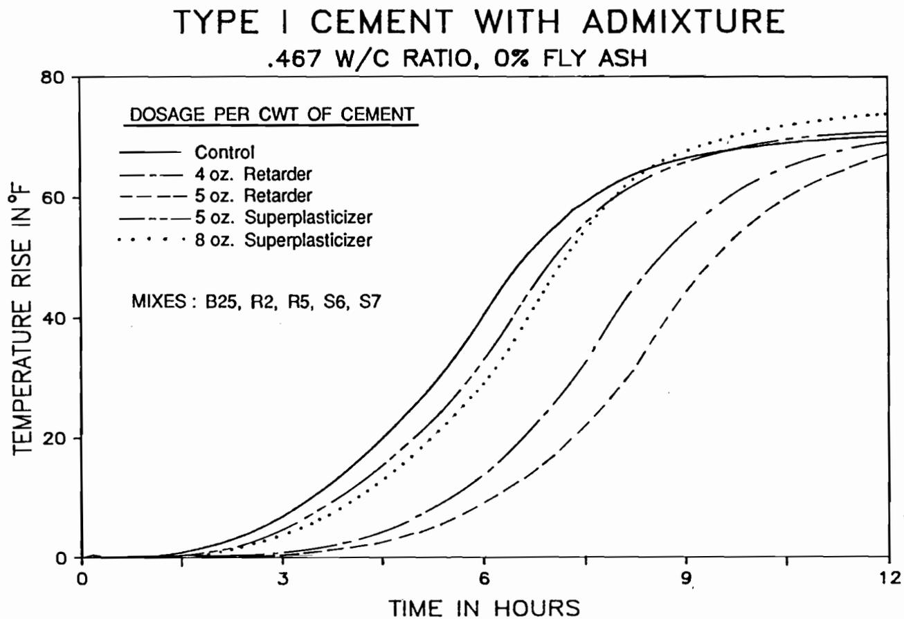
Figure 5.38 Effect of admixture addition on the temperature rise in Type I cement mortar during the initial 12 hours.
