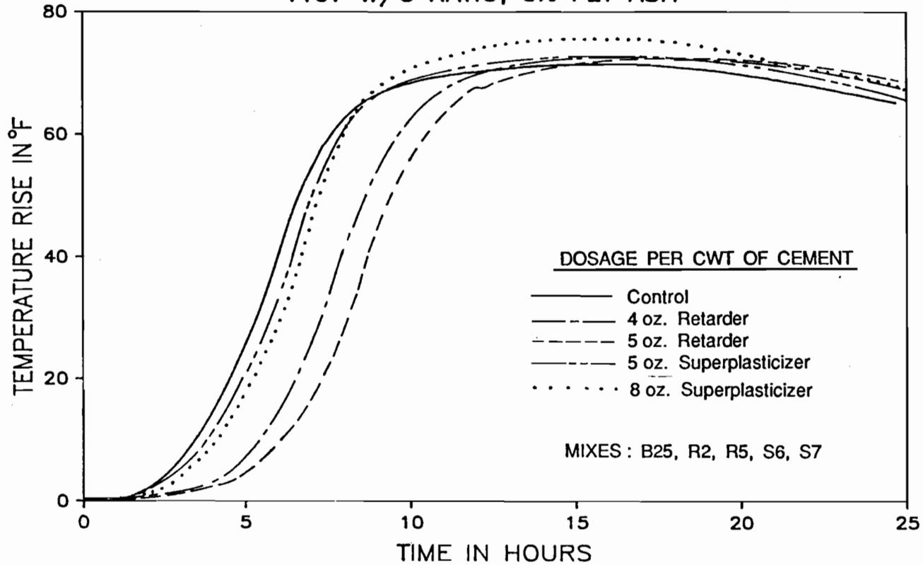
Figure 5.39 Effect of admixture addition on the temperature rise in Type I cement mortar during the initial 25 hours.
