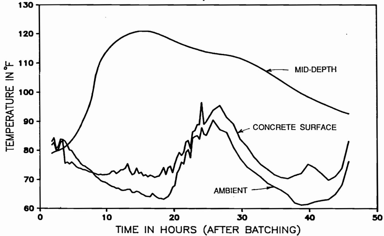
Figure 5.8 Temperature profile for Test 4 sample with top surface exposed.
