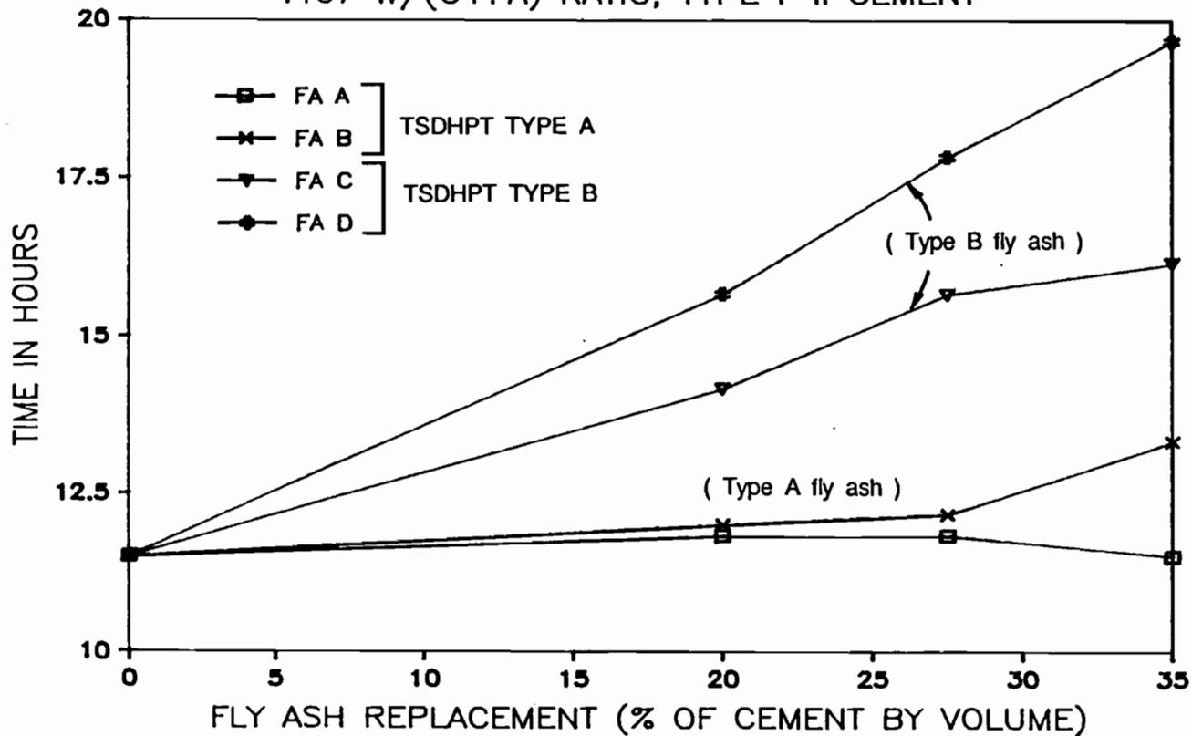
Figure 6.4 Time to 95% of the peak temperature rise in mortar vs. percent replacement of Type I-II cement.
