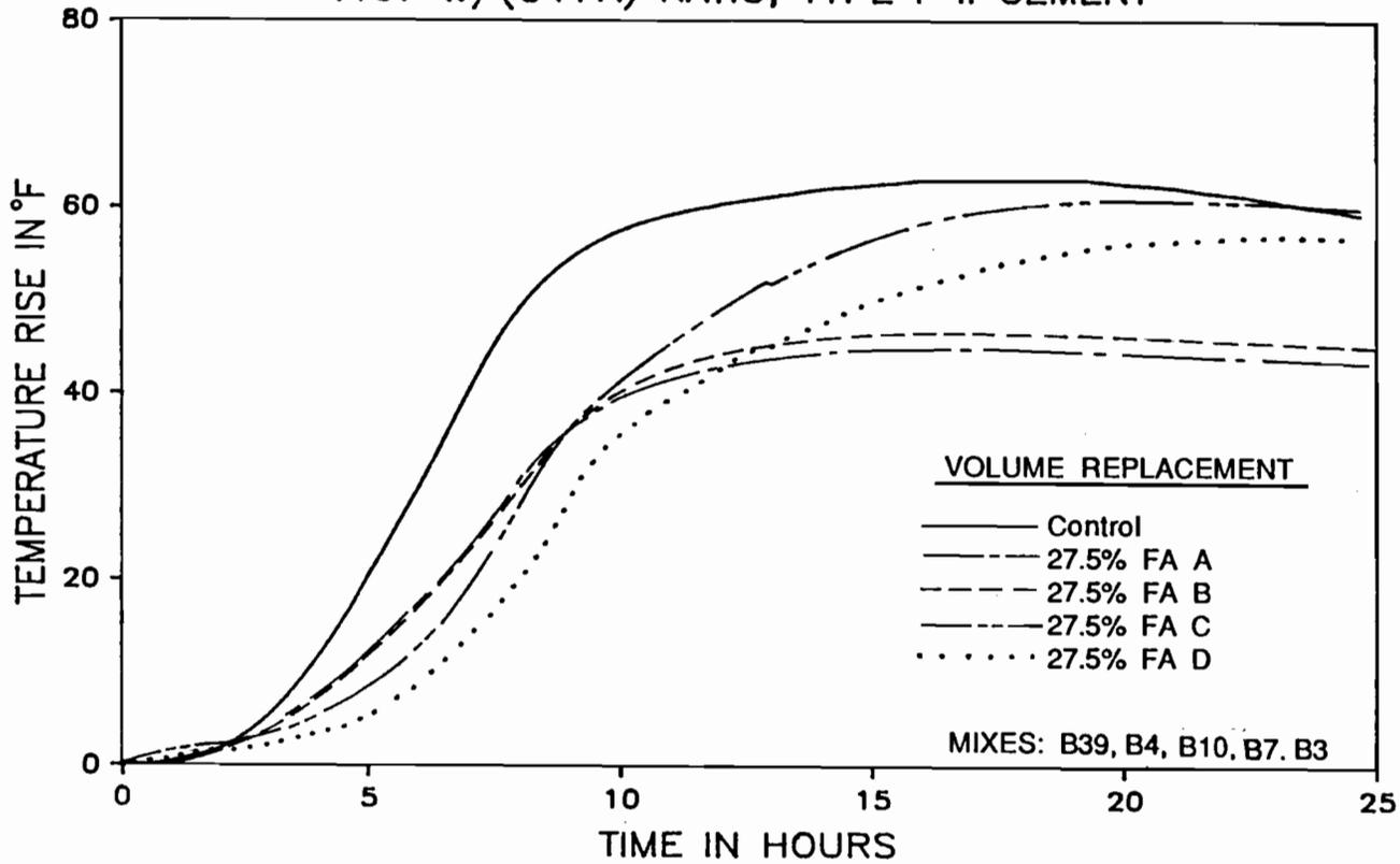
Figure 5.26 Effect of fly ash type on the temperature rise in mortar with 27.5% replacement of Type I-II cement.
