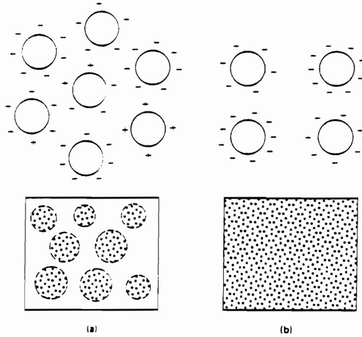
Figure 3.12 Dispersing action of superplasticizer (schematic representation) : a) flocculated paste ; b) dispersed paste. [8]
