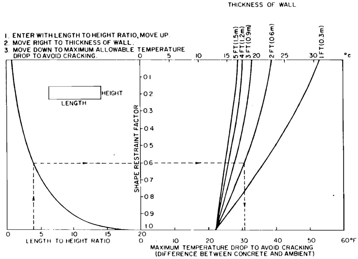
Figure 3.5 Graphical determination of safe concrete form stripping temperature. [21]
