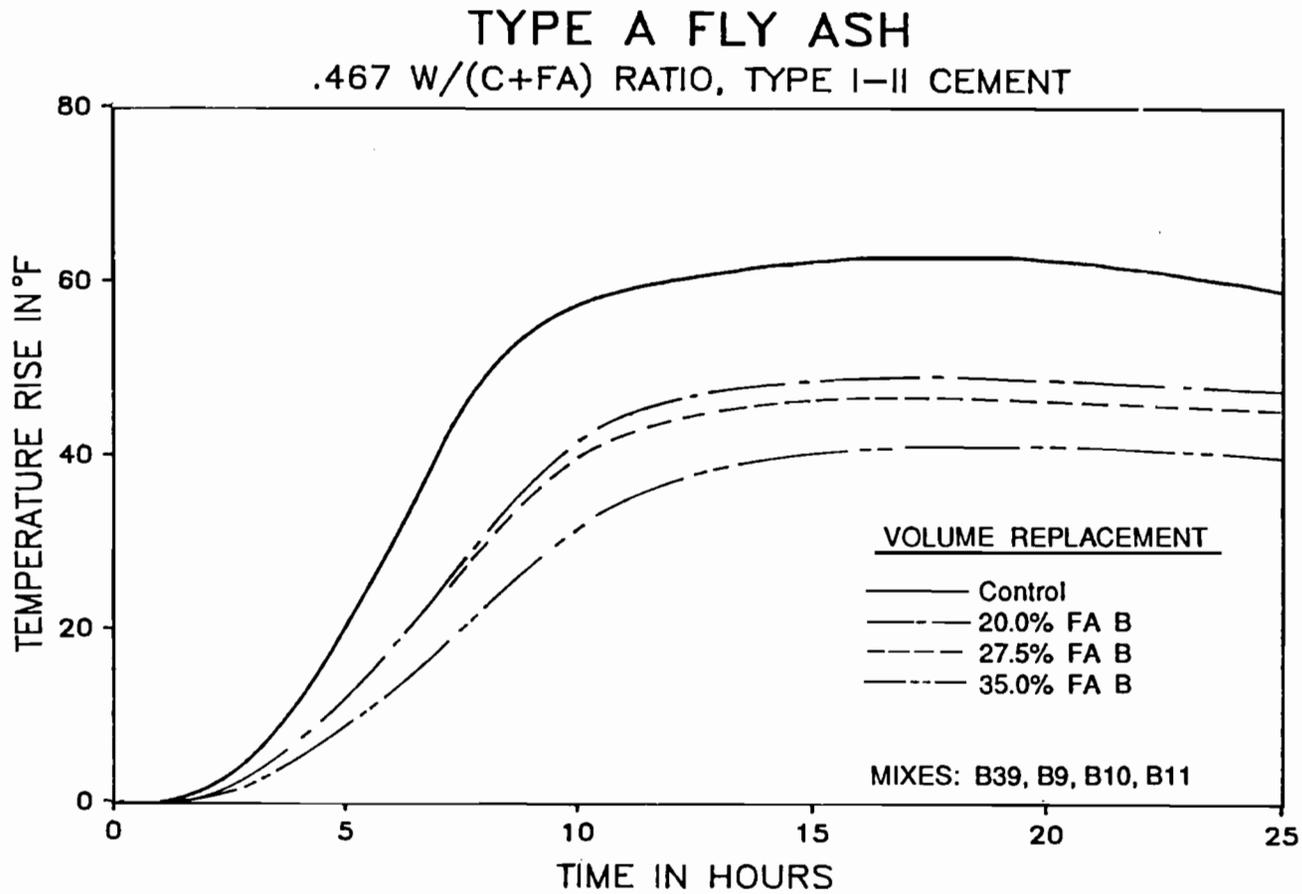
Figure 5.23 Effect of varying content of Type A fly ash on the temperature rise in Type I-II cement mortar.
