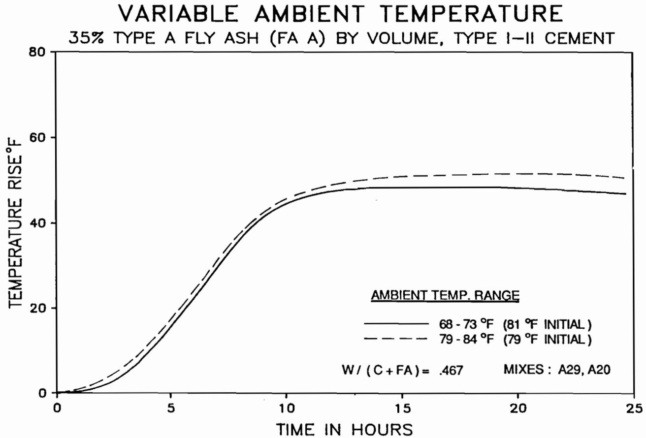
Figure 5.13 Effect of ambient temperature on the temperature rise in mortar containing Type A fly ash.
