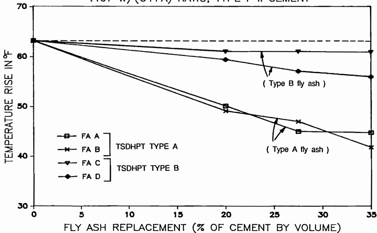
Figure 6.1 Maximum temperature rise in mortar vs. percent replacement of Type I-II cement with fly ash.
