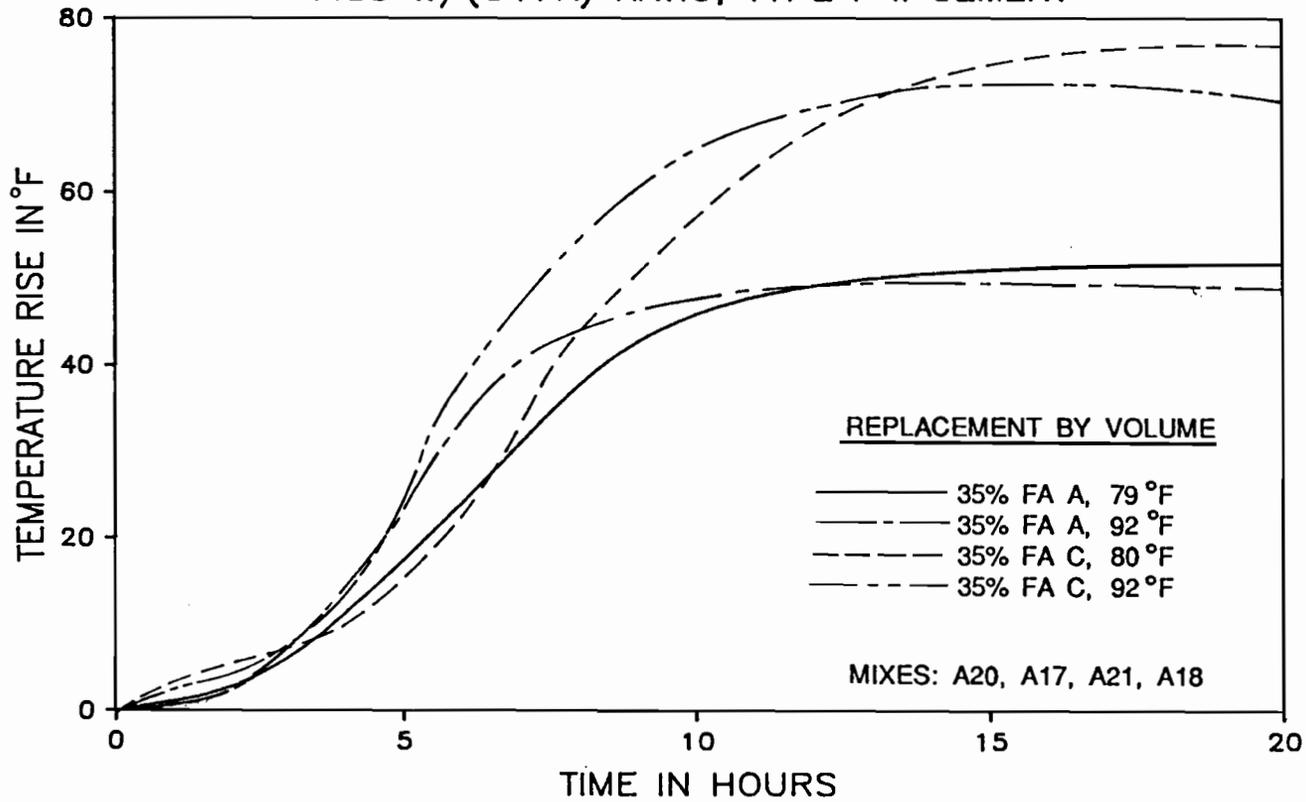
Figure 5.15 Effect of initial mix temperature on the temperature rise in mortar containing fly ash.
