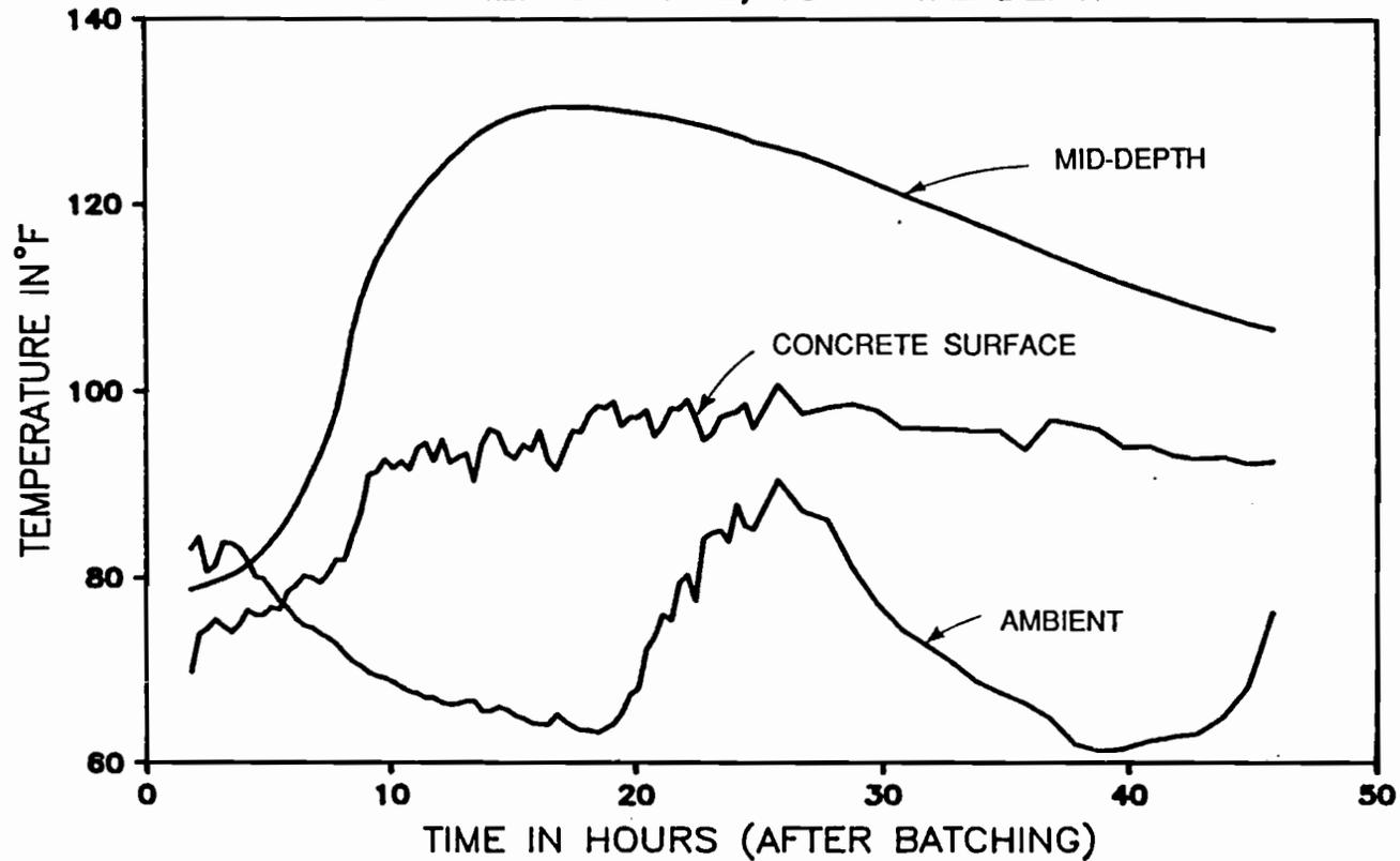
Figure 5.9 Temperature profile for Test 4 sample with top surface covered with damp burlap and plastic.
