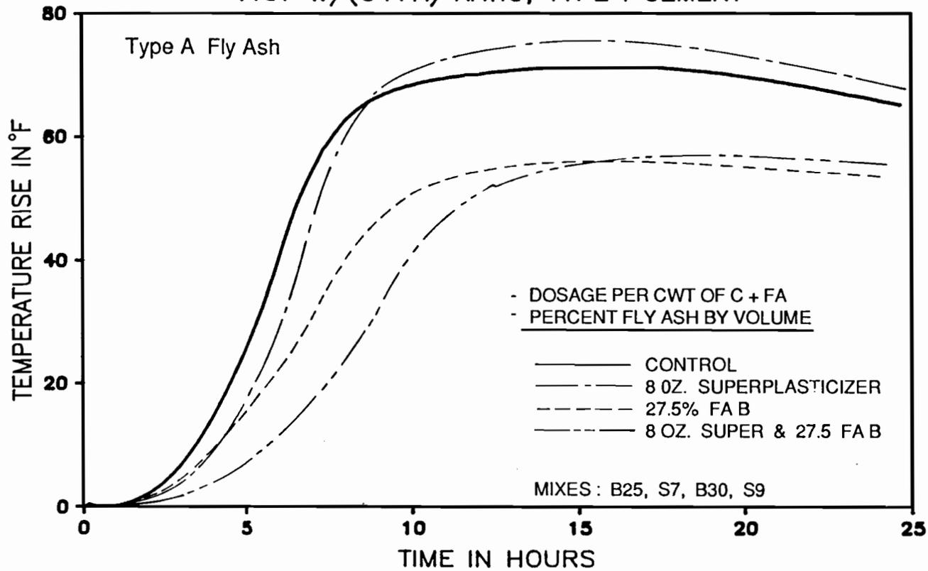
Figure 7.3 Effect of a superplasticizer on the temperature rise in Type I cement mortar with or without Type A fly ash.
