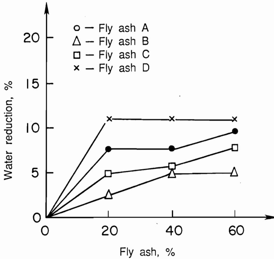
Figure 3.9 Water reduction in mortar vs. fly ash replacement of Portland cement. [30] Selected properties of the fly ashes are in Table 3.2.
