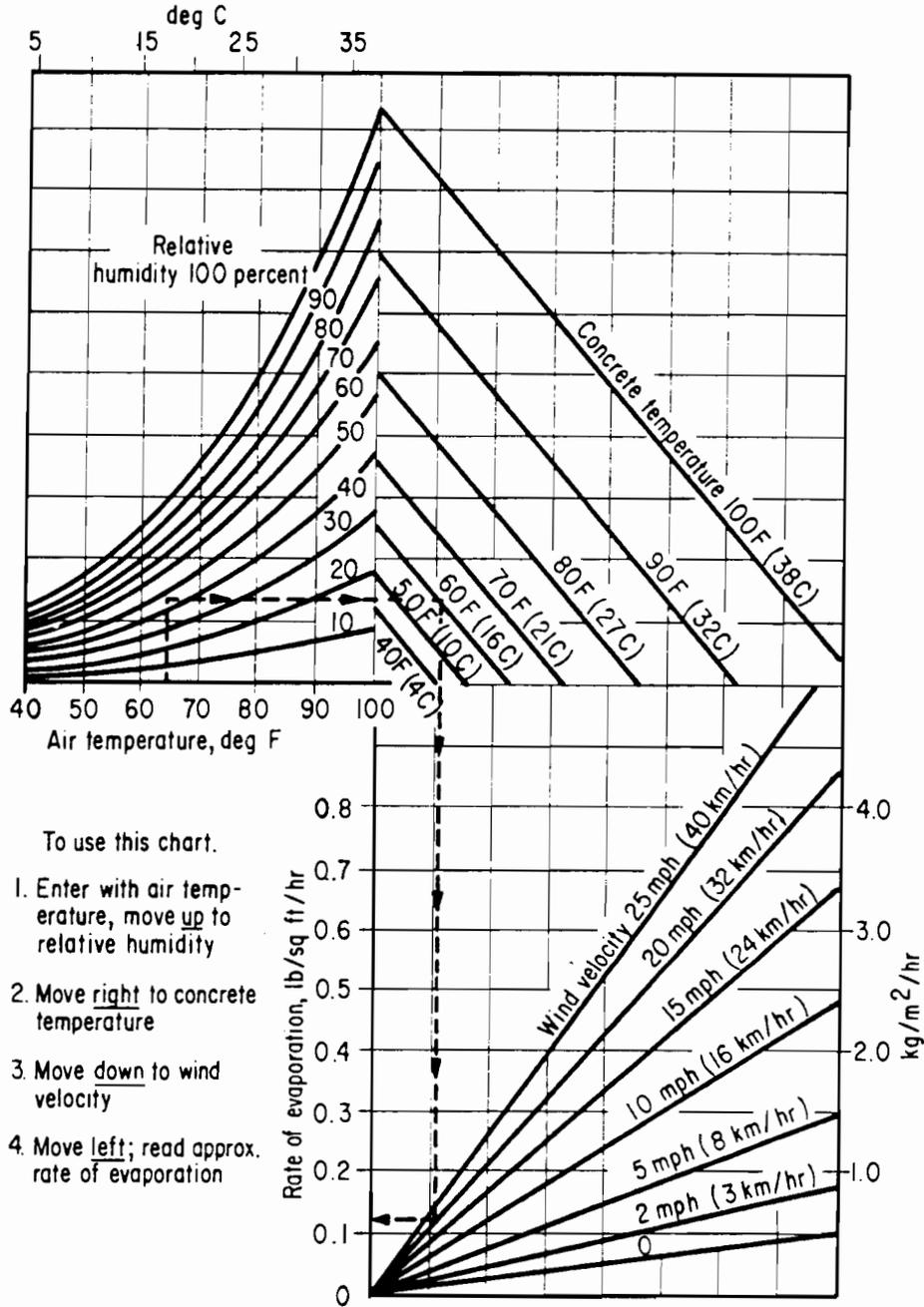
Figure 1.1 Effect of concrete temperature, air temperature, relative humidity, and wind velocity on the rate of evaporation of surface moisture from concrete. [4]
