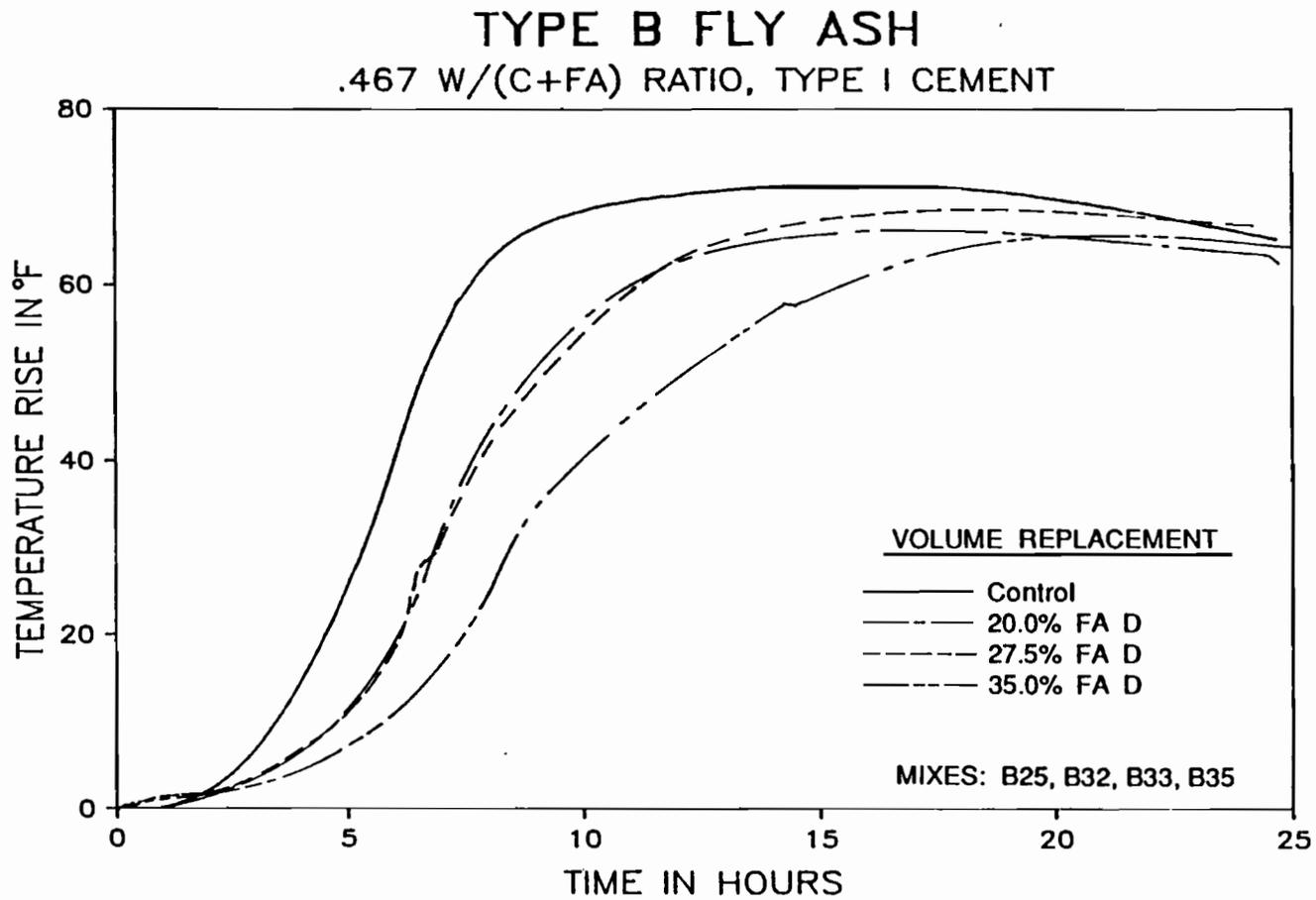
Figure 5.30 Effect of varying content of Type B fly ash on the temperature rise in Type I cement mortar.
