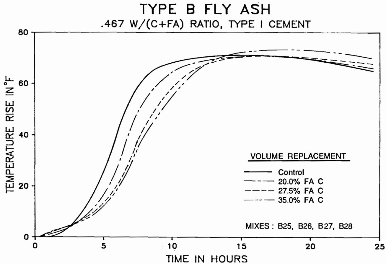
Figure 5.29 Effect of varying content of Type B fly ash on the temperature rise in Type I cement mortar.
