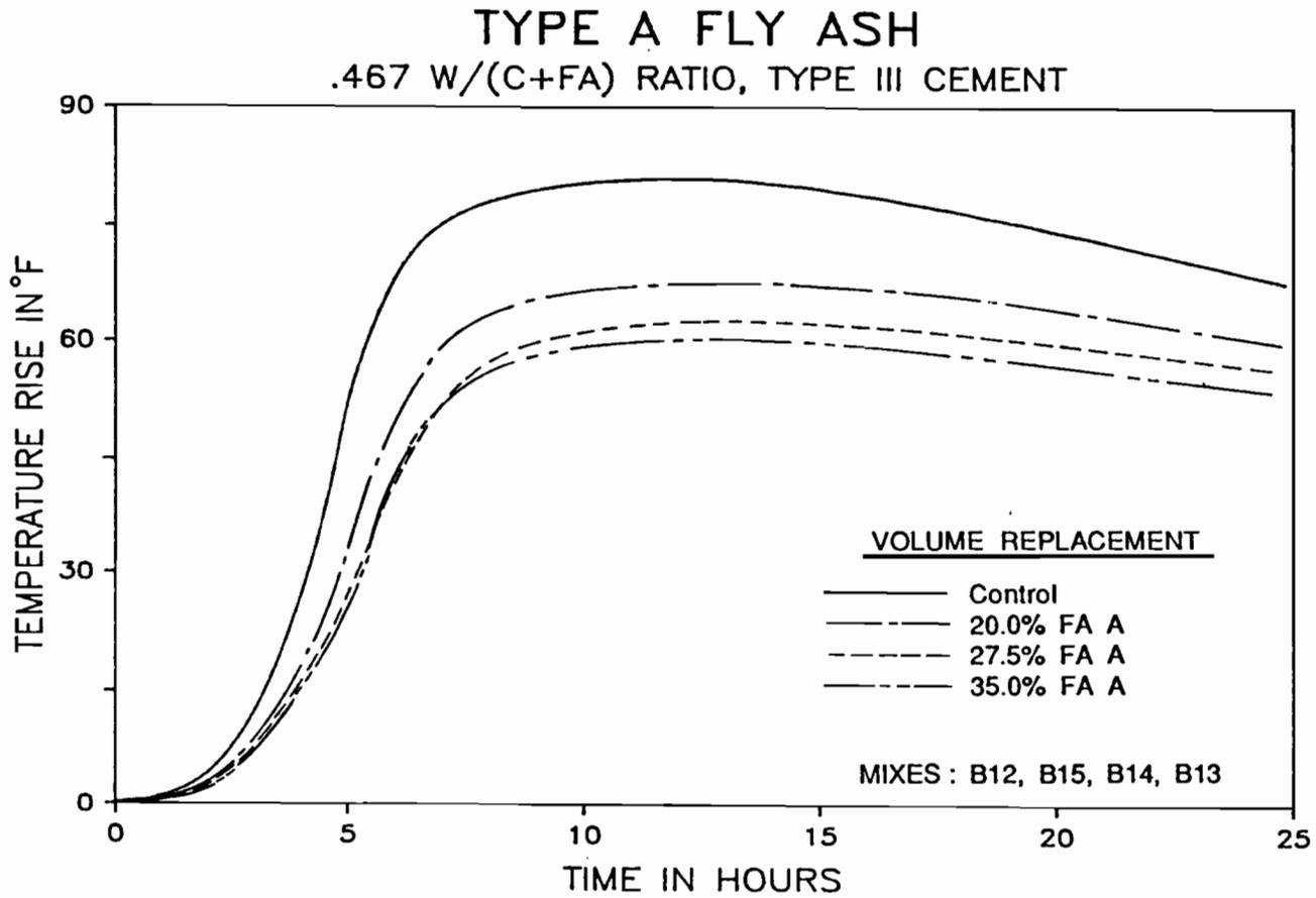
Figure 5.32 Effect of varying content of Type A fly ash on the temperature rise in Type III cement mortar.
