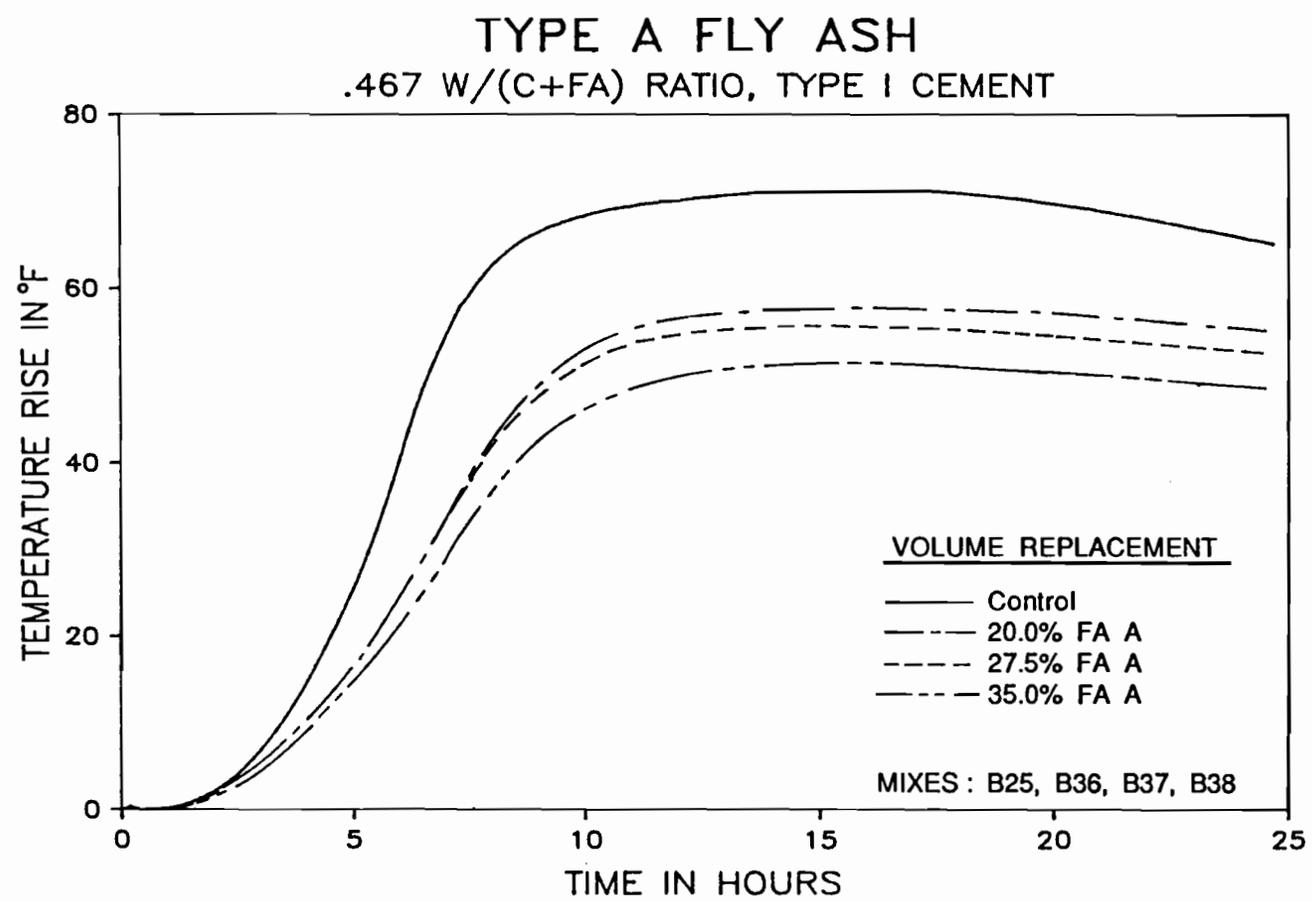
Figure 5.27 Effect of varying content of Type A fly ash on the temperature rise in Type I cement mortar.
