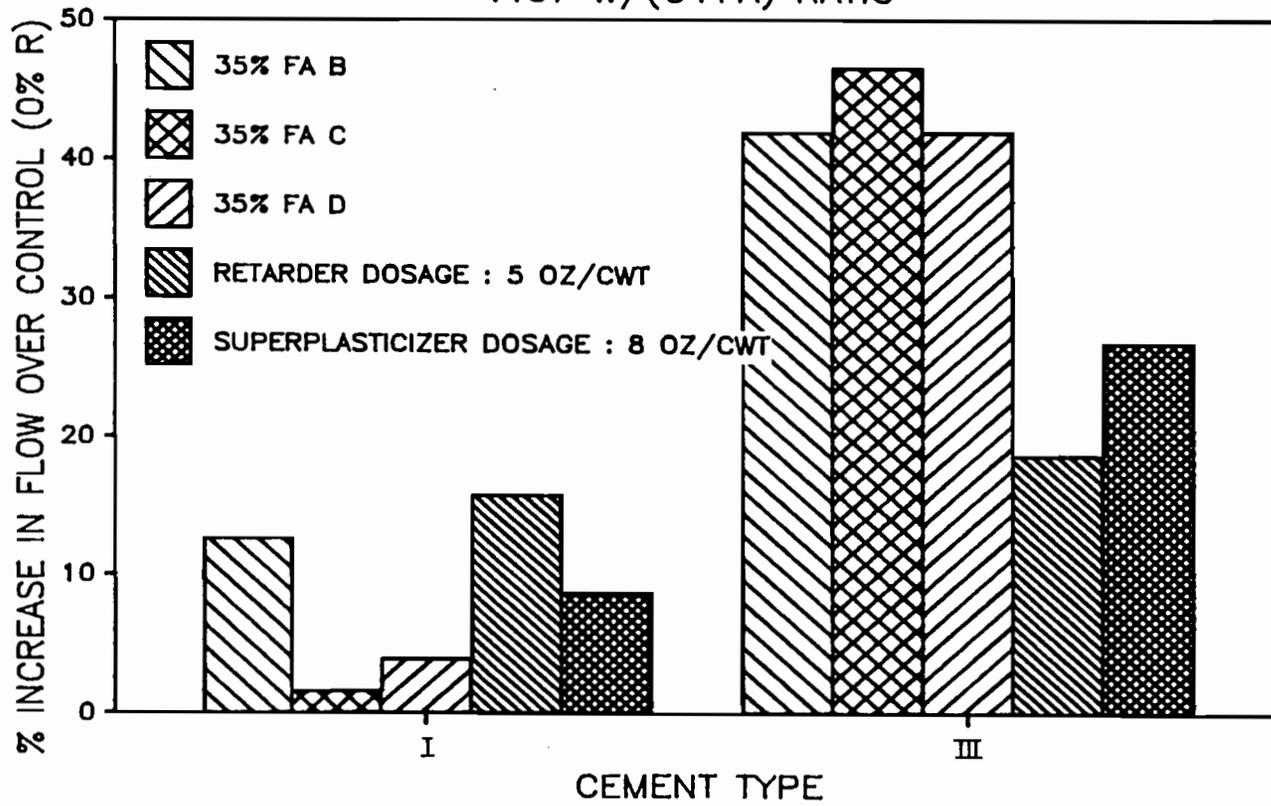
Figure 7.8 Effect of fly ash and chemical admixture on the flow of mortar.
