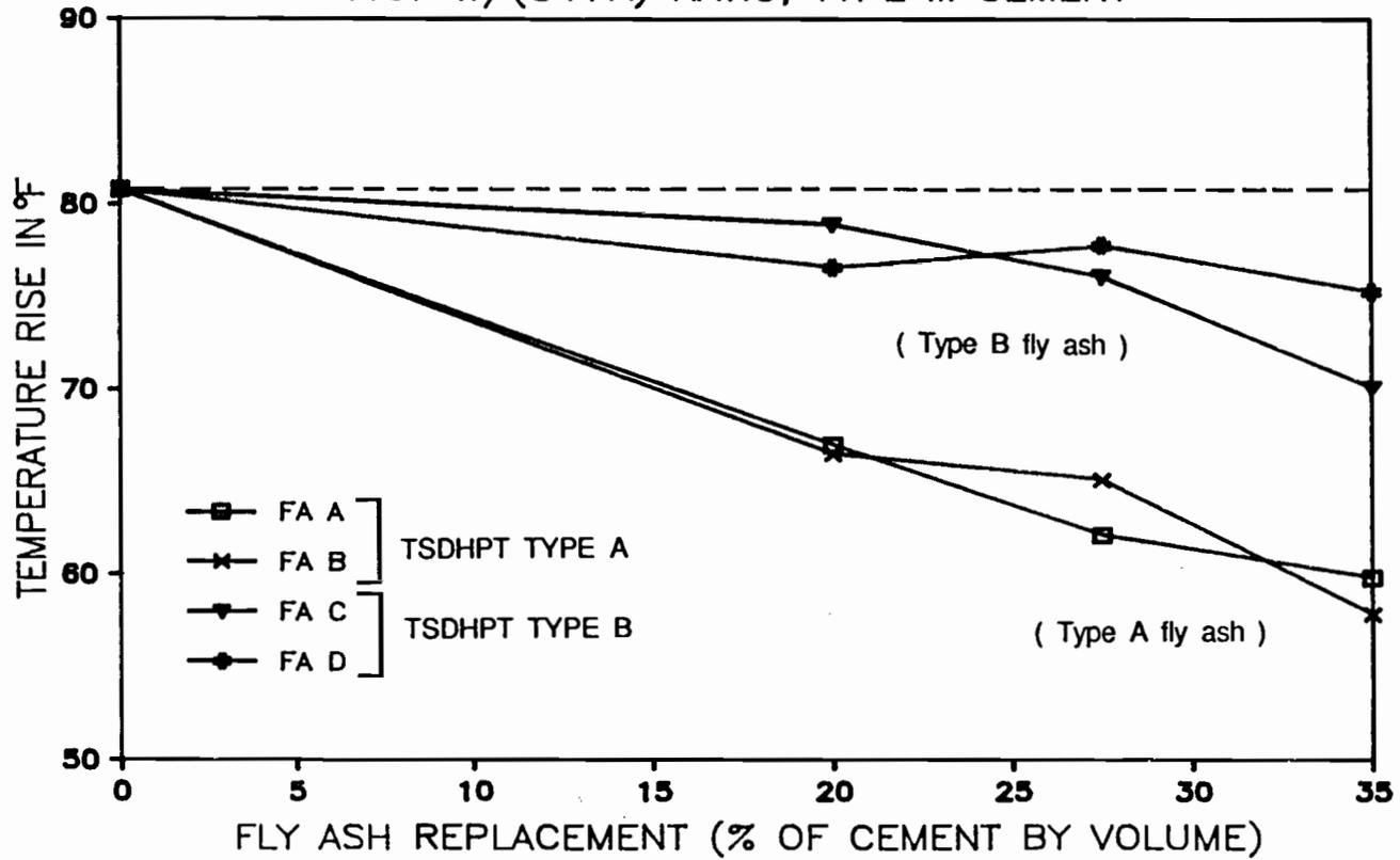
Figure 6.3 Maximum temperature rise in mortar vs. percent replacement of Type III cement with fly ash.
