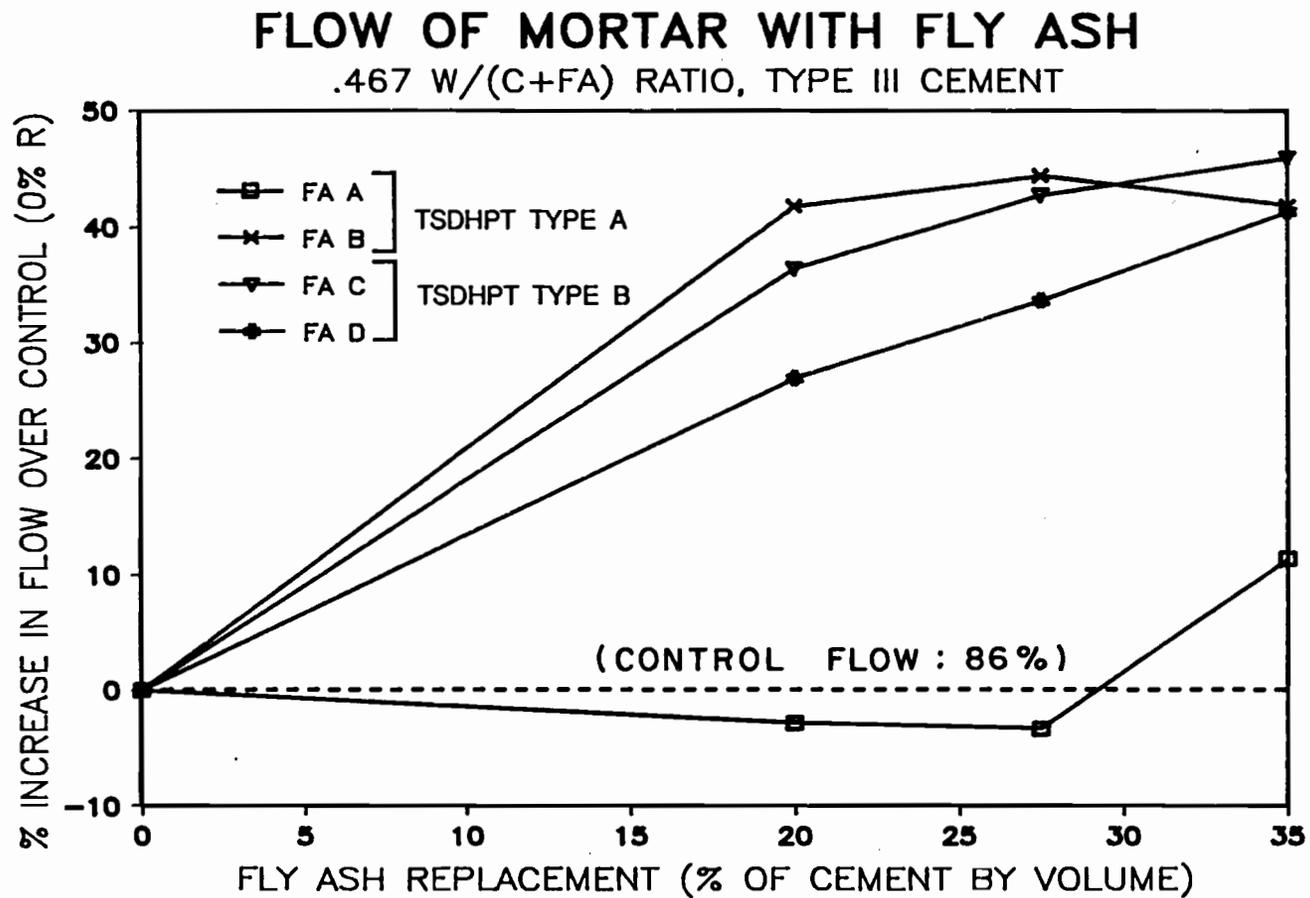
Figure 5.51 Relative flow of Type III cement mortars containing fly ash.
