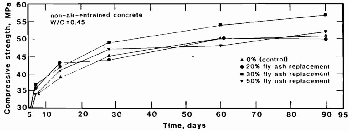
Figure 3.8 Compressive strength development of concretes containing high calcium fly ash. [3]
