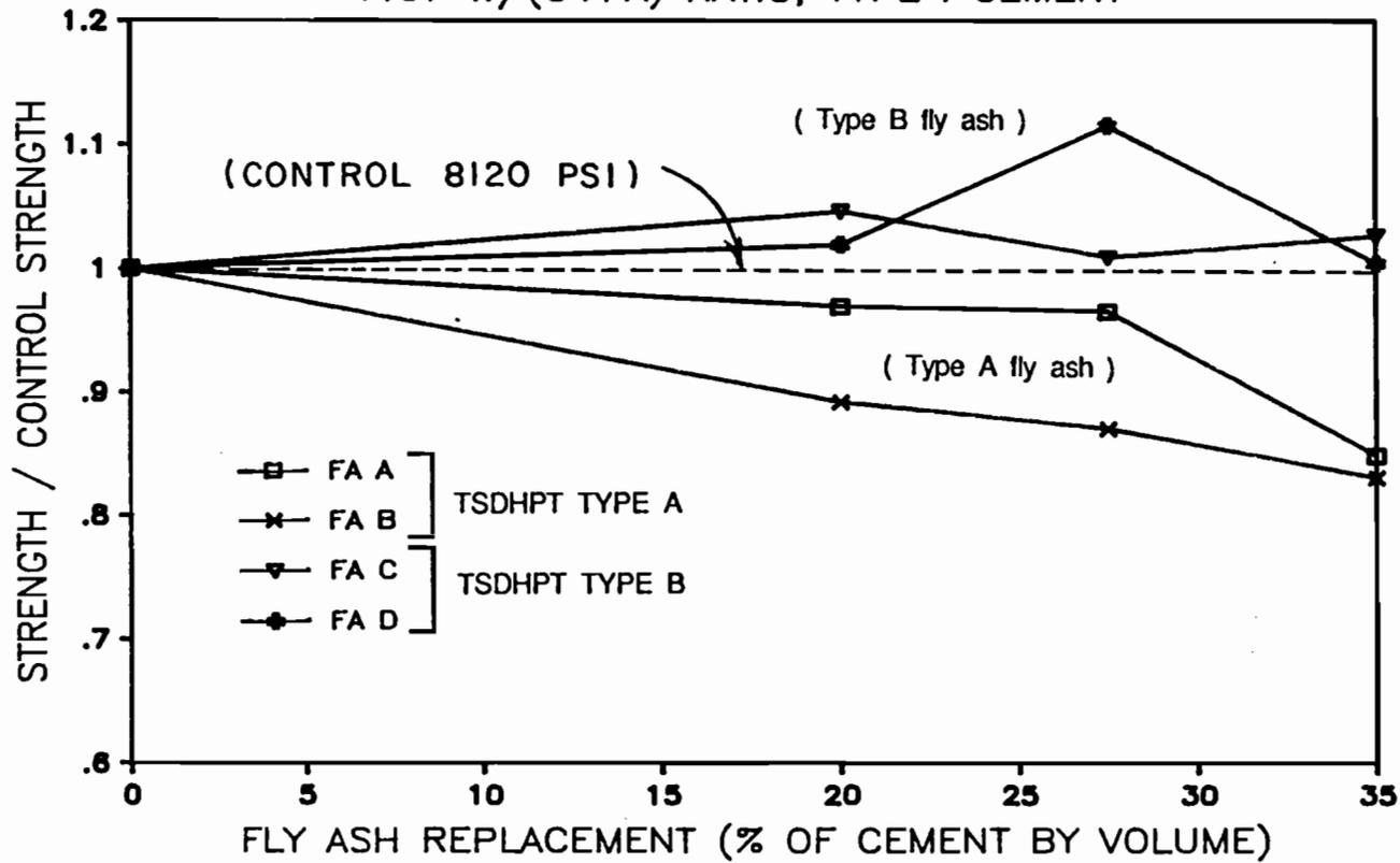
Figure 5.47 Relative compressive strength of Type I cement mortars containing fly ash at 28 days.
