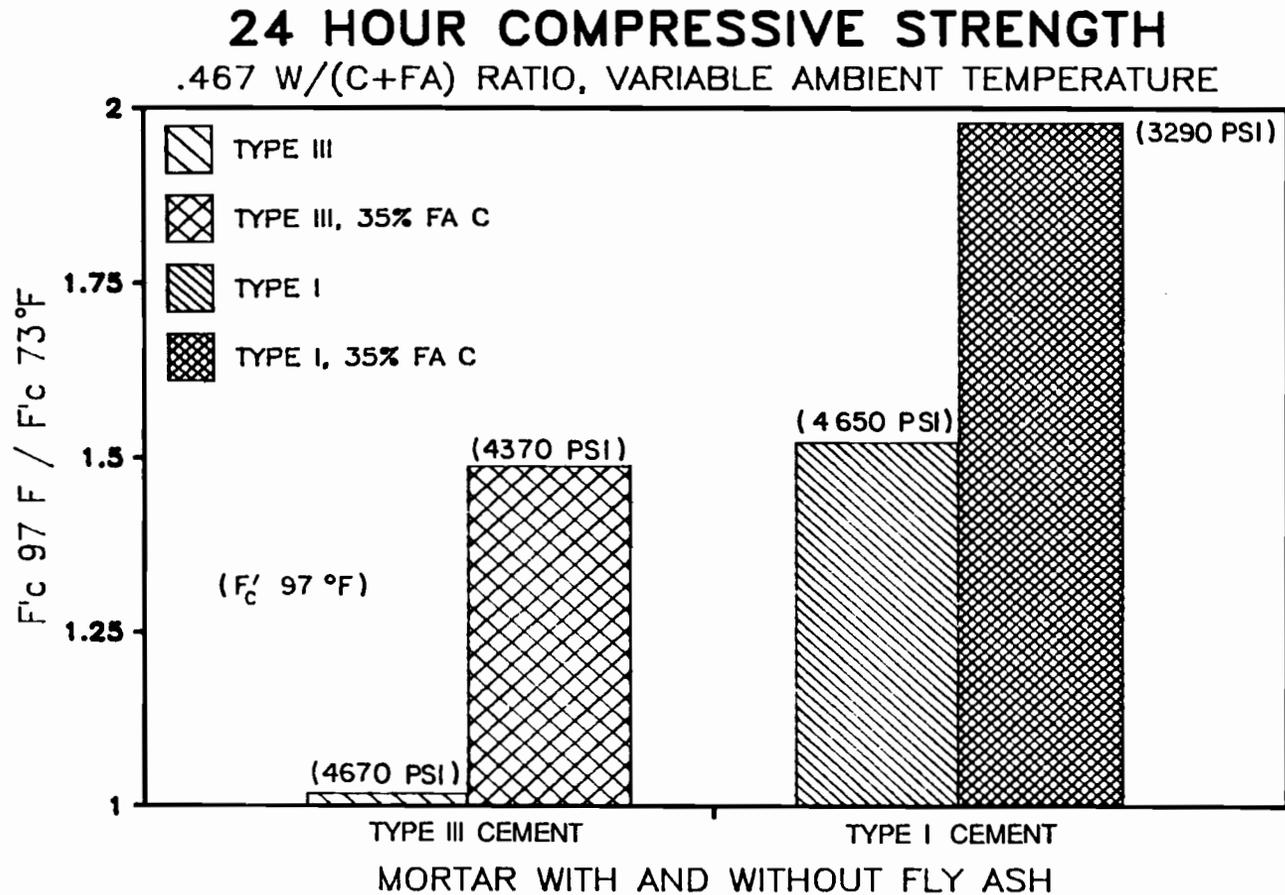
Figure 6.10 Effect of curing temperature on the relative strength of mortar with or without Type B fly ash.
