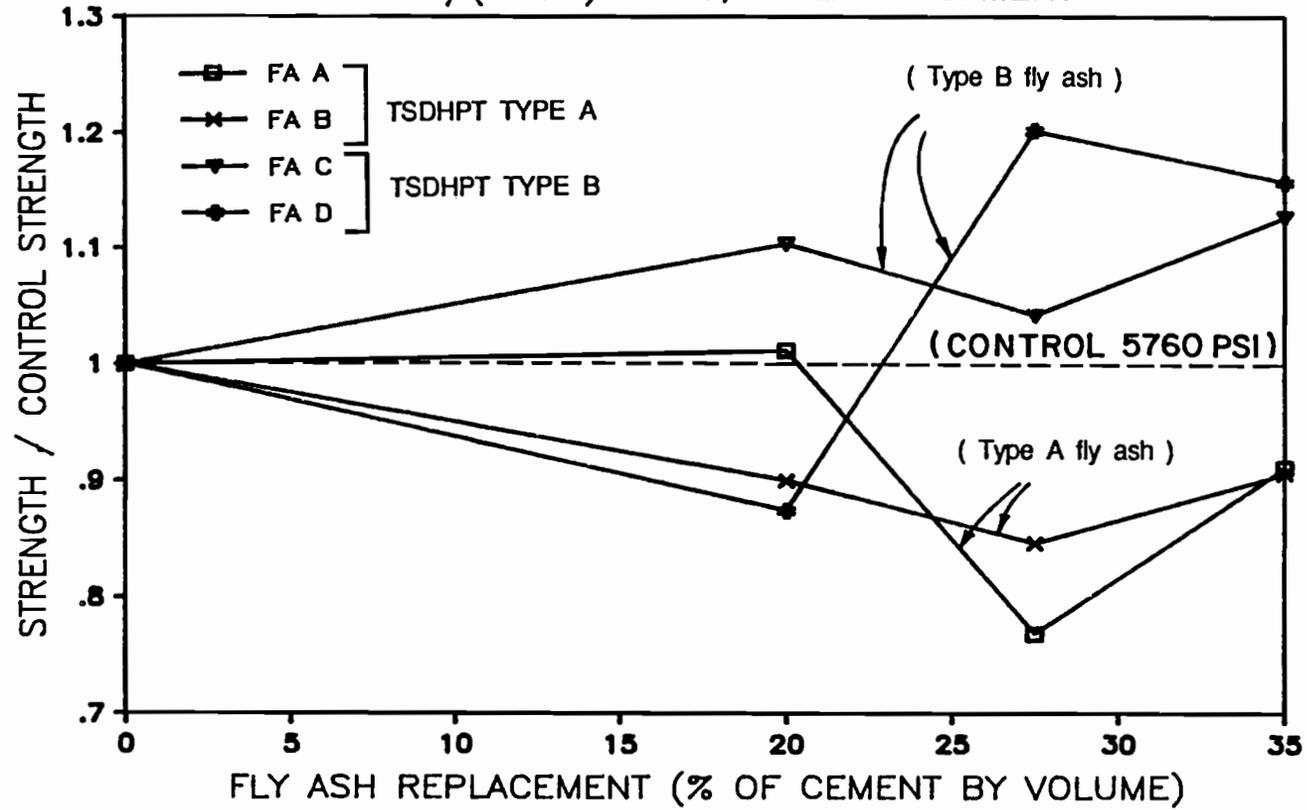
Figure 5.44 Relative compressive strength of Type I-II cement mortars containing fly ash at 7 days.
