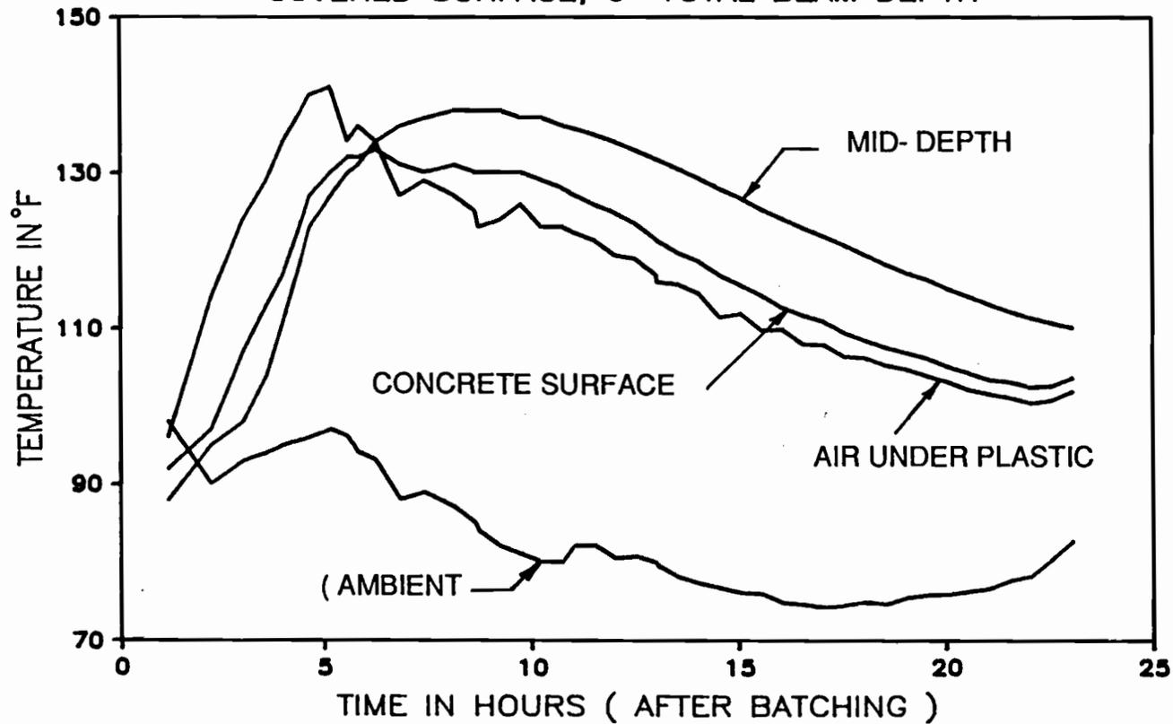
Figure 5.6 Temperature profile for Test 3 sample with top surface covered with damp burlap and plastic.
