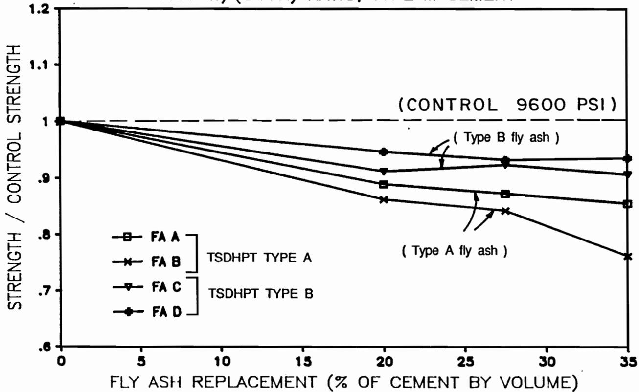
Figure 5.49 Relative compressive strength of Type III cement mortars containing fly ash at 28 days.
