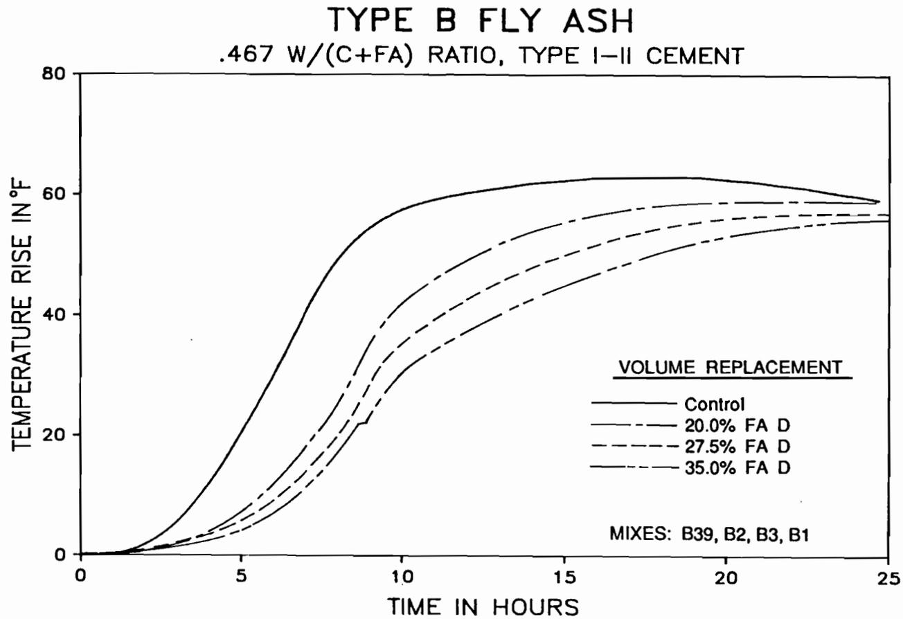
Figure 5.25 Effect of varying content of Type B fly ash on the temperature rise in Type I-II cement mortar.
