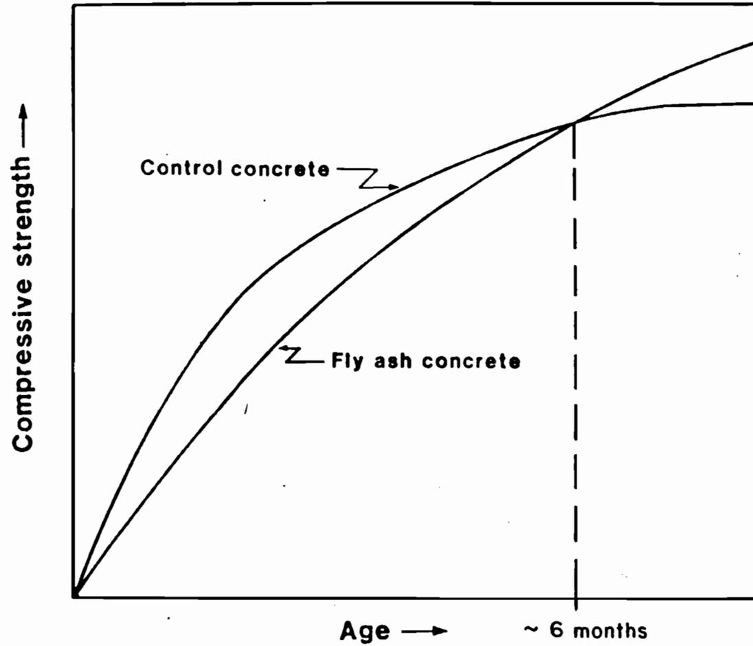
Figure 2.5 Typical rates of strength increase for plain concrete and fly ash concrete proportioned by simple replacement. [3]
