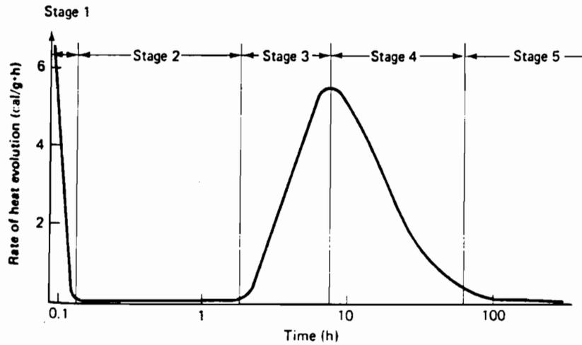
Figure 2.1 Rate of heat evolution during the hydration of tricalcium silicate. [8]
