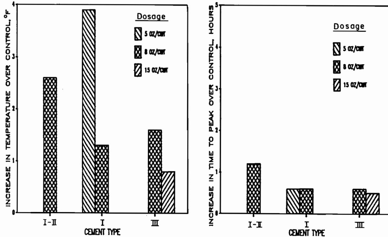
Figure 7.2 Effect of a naphthalene based superplasticizer on the temperature rise and the time to the peak temperature in mortar containing no fly ash.
