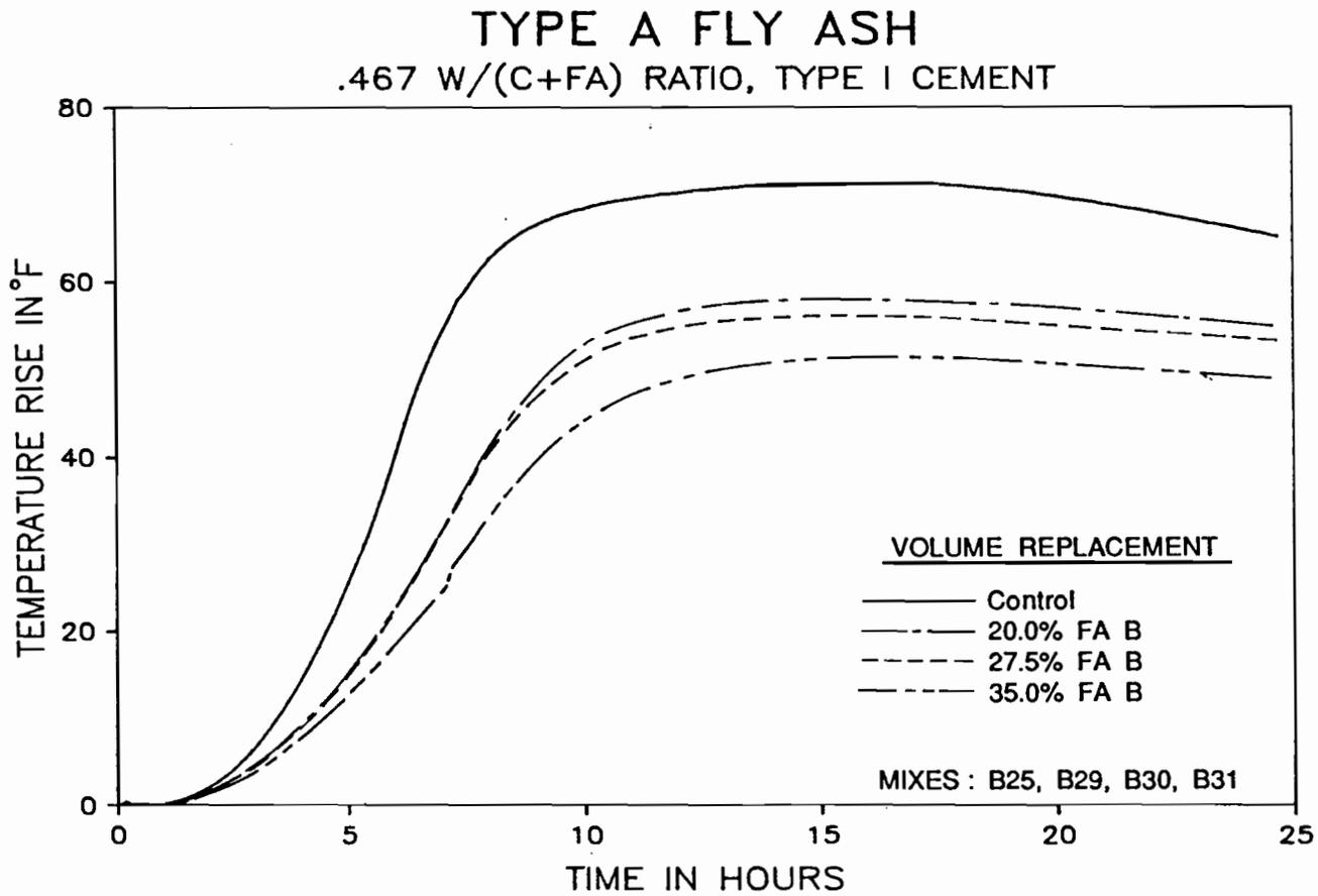
Figure 5.28 Effect of varying content of Type A fly ash on the temperature rise in Type I cement mortar.
