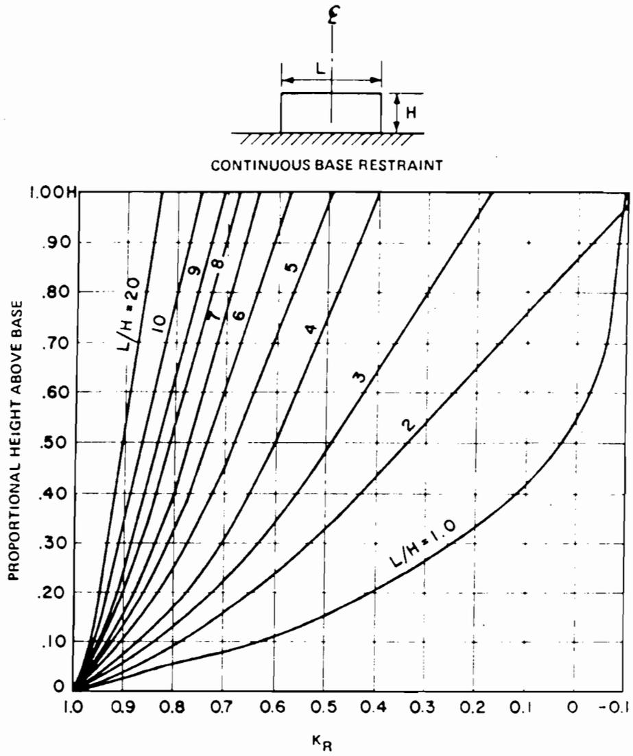
Figure 3.3 Degree of tensile restraint at center section. [18]
