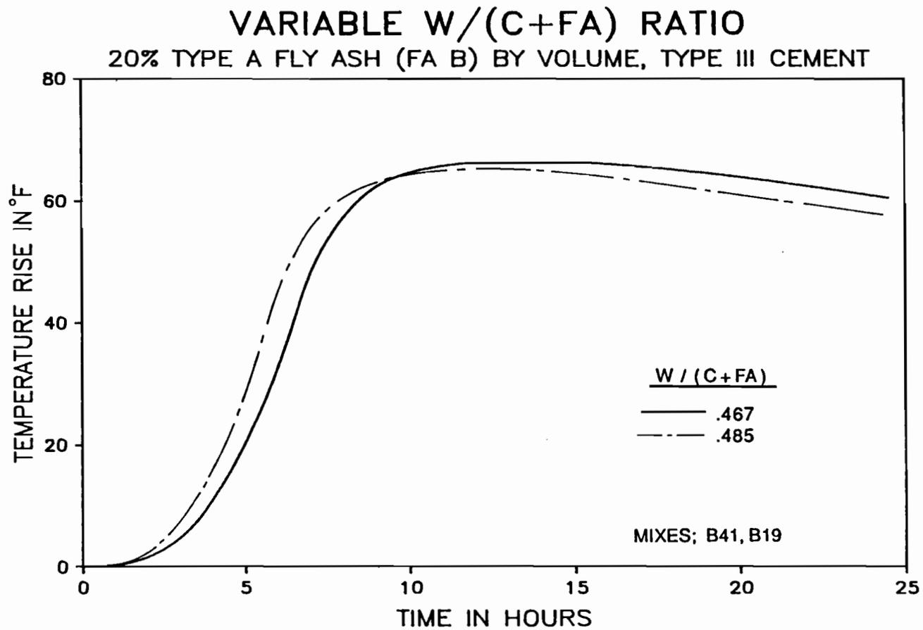
Figure 5.18 Effect of the water to cementitious materials ratio on the temperature rise in mortar containing fly ash.
