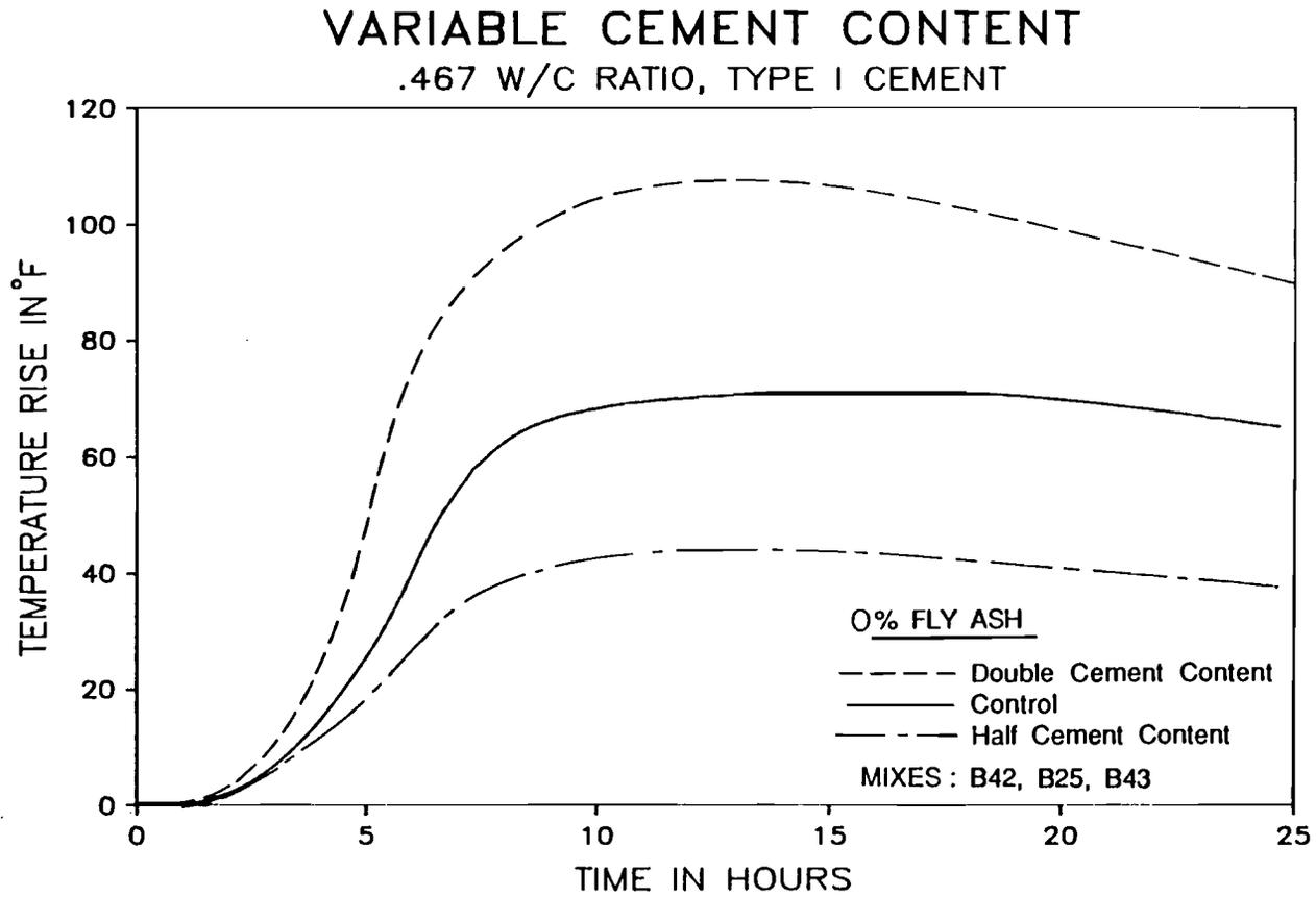
Figure 5.17 Effect of cement content on the temperature in mortar.
