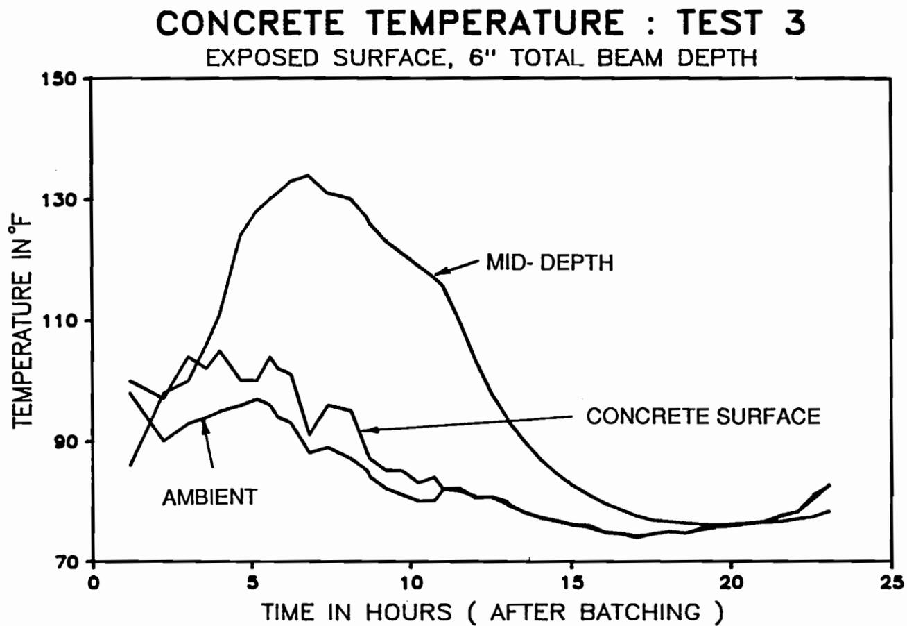
Figure 5.5 Temperature profile for Test 3 sample with top surface exposed.
