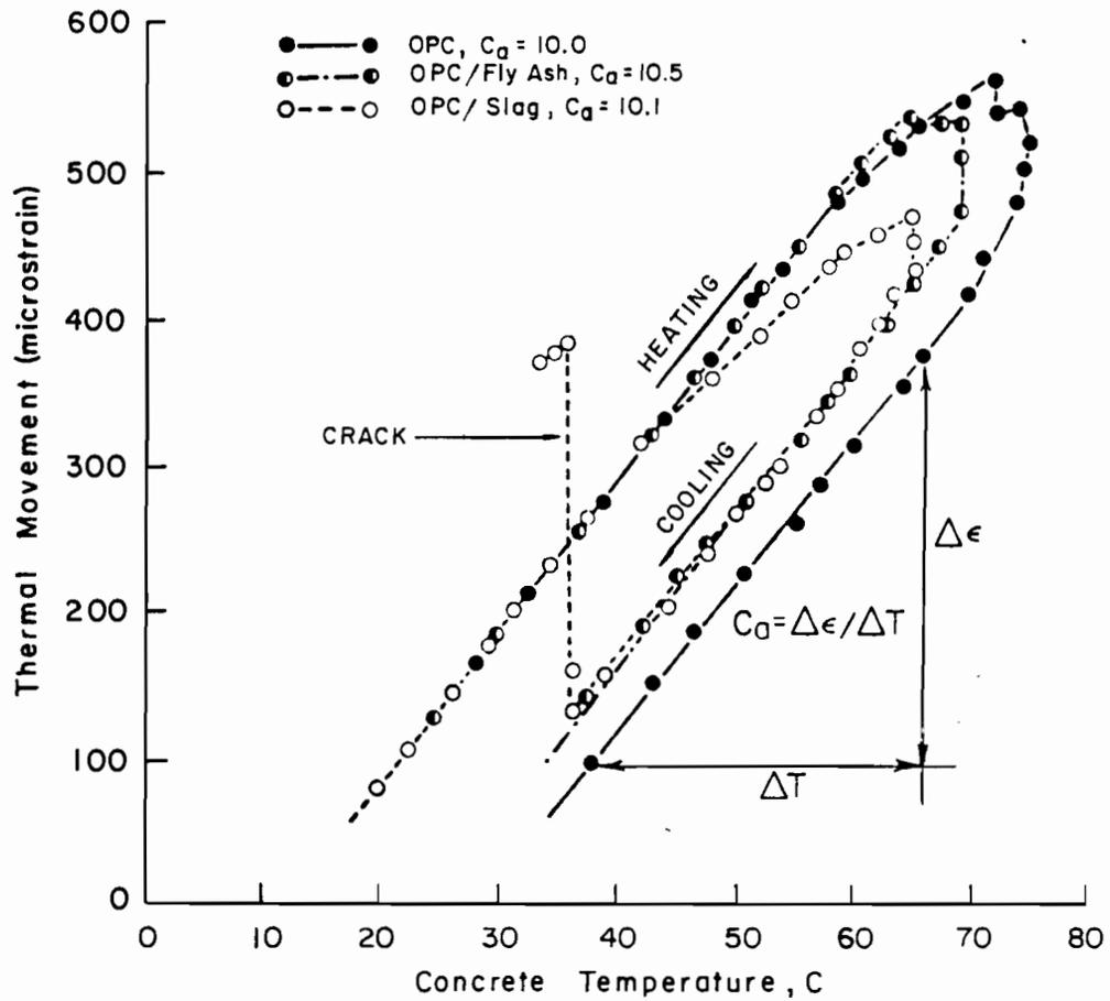
Figure 3.2 Relationship between strain and temperature recorded at mid-height of concrete foundations. [17] OPC = Ordinary Portland cement
