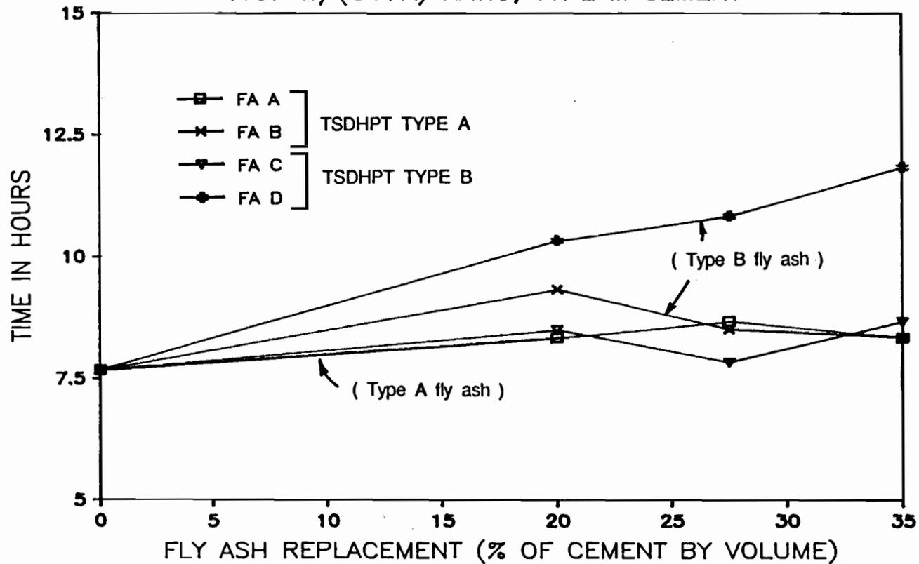
Figure 6.6 Time to 95% of the peak temperature rise in mortar vs. percent replacement of Type III cement.
