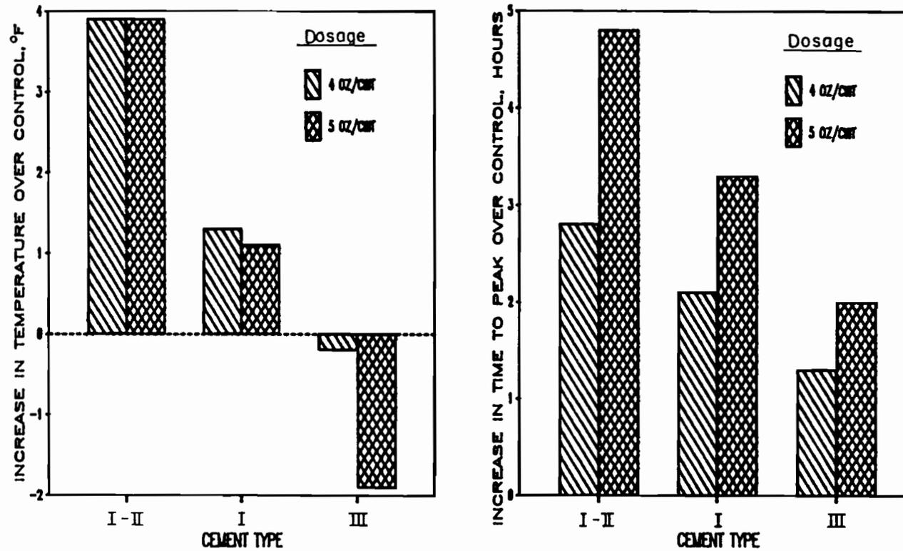
Figure 7.1 Effect of a lignosulfate based retarder on the temperature rise and the time to the peak temperature in mortar containing no fly ash.
