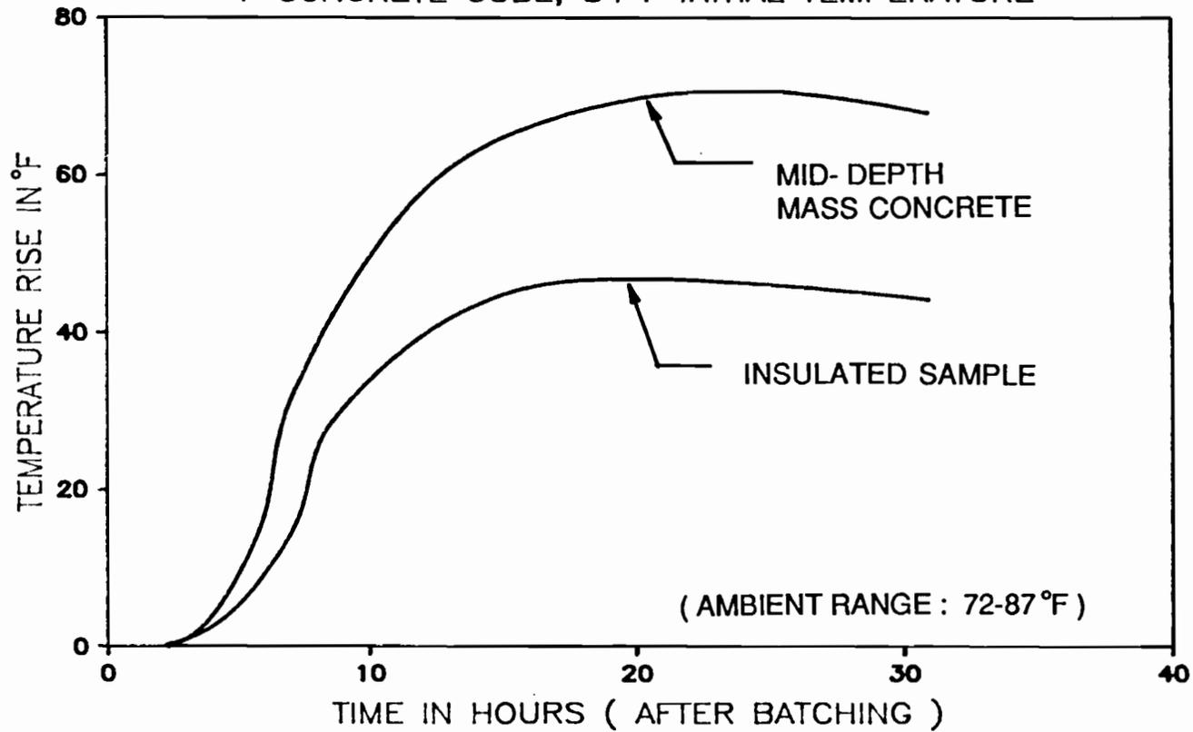
Figure 5.12 Comparison of temperature rise in Test 2 sample to insulated sample.
