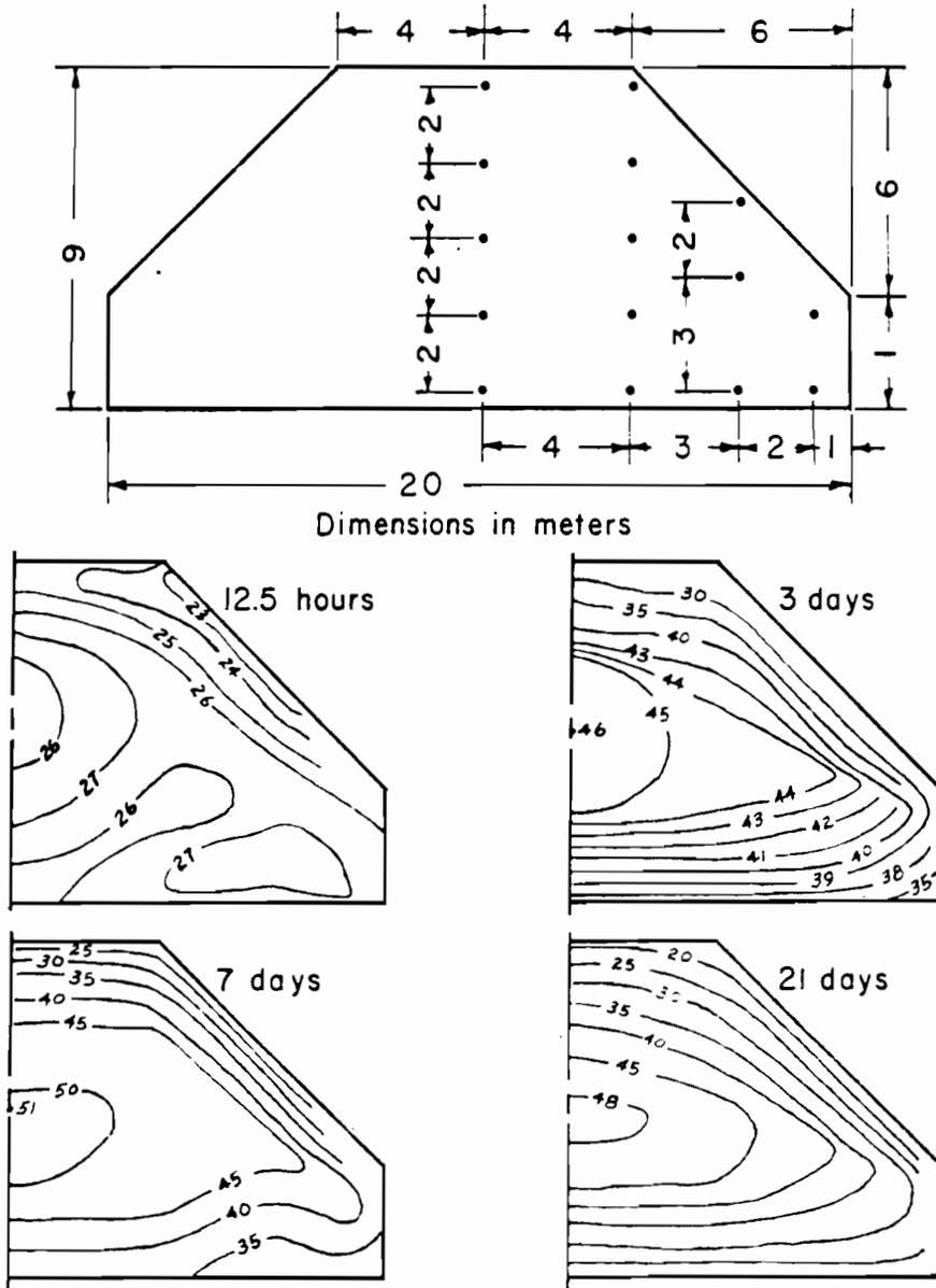
Figure 3.4 Isothermic curves in deg. C for horizontal section of a concrete buttress head for various ages. [20]
