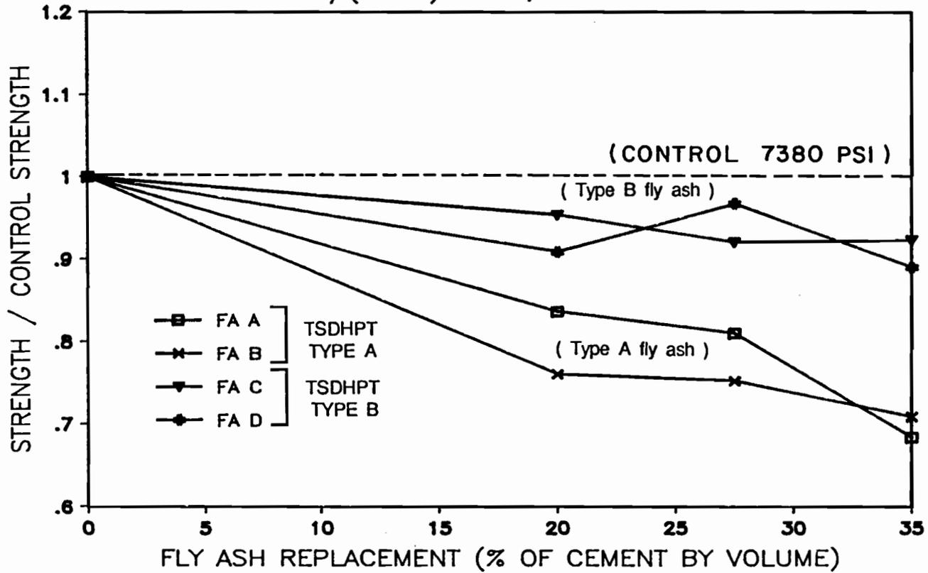
Figure 5.46 Relative compressive strength of Type I cement mortars containing fly ash at 7 days.
