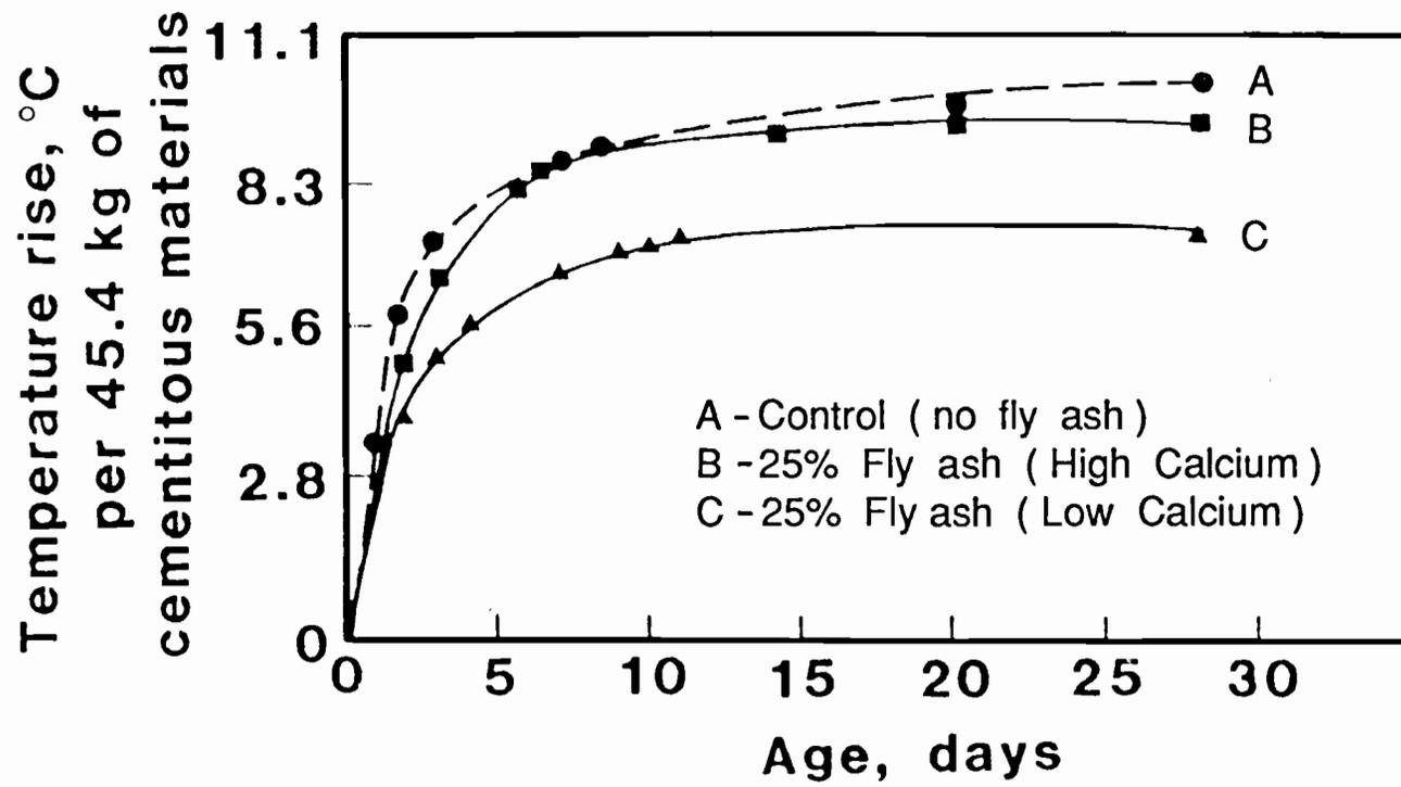
Figure 3.6 Adiabatic temperature rise in concrete containing high calcium fly ash. [3]
