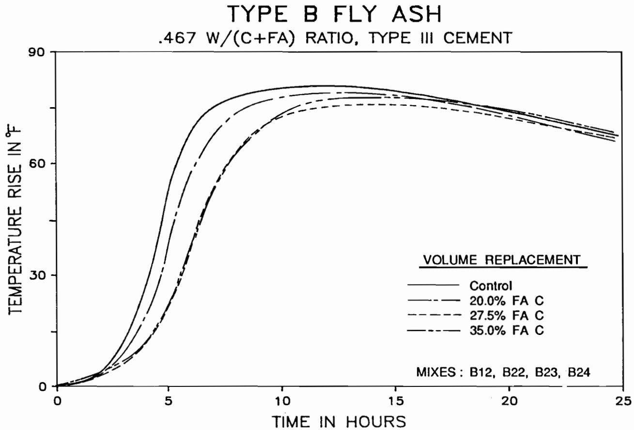
Figure 5.34 Effect of varying content of Type B fly ash on the temperature rise in Type III cement mortar.
