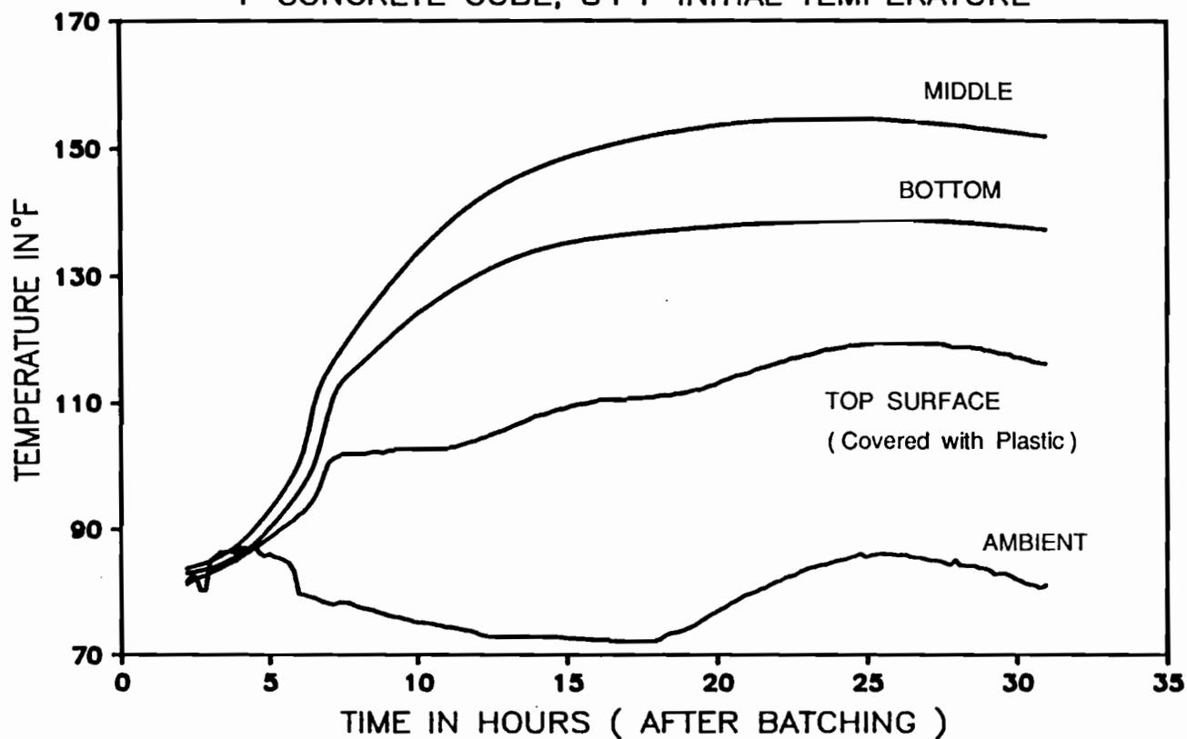
Figure 5.3 Temperature profile for Test 2.
