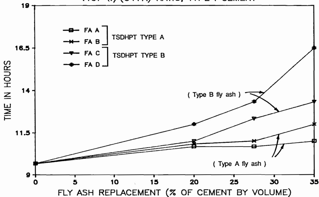
Figure 6.5 Time to 95% of the peak temperature rise in mortar vs. percent replacement of Type I cement.
