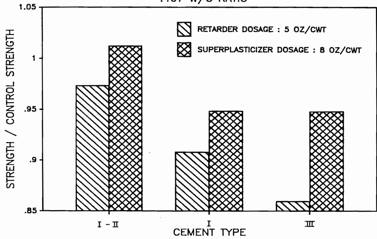
Figure 7.7 Effect of chemical admixture on the 28 day strength of mortar containing no fly ash.
