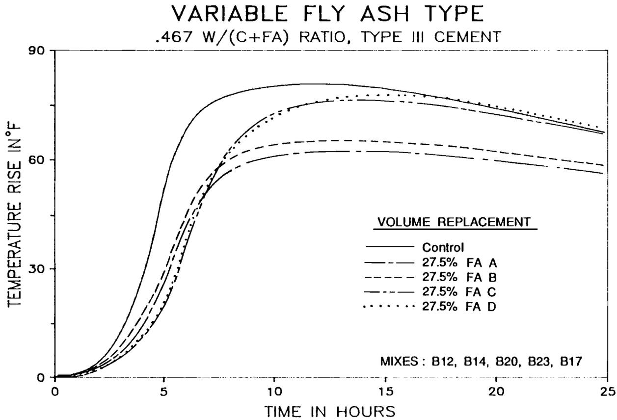
Figure 5.36 Effect of fly ash type on the temperature rise in mortar with 27.5% replacement of Type III cement.
