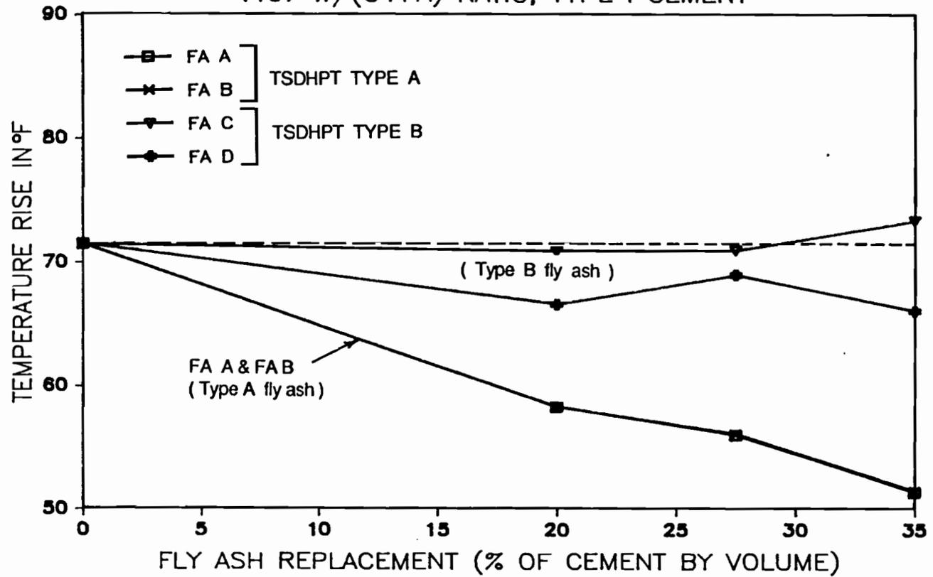
Figure 6.2 Maximum temperature rise in mortar vs. percent replacement of Type I cement with fly ash.
