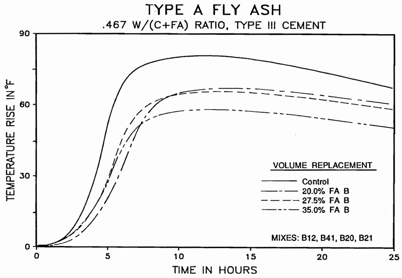
Figure 5.33 Effect of varying content of Type A fly ash on the temperature rise in Type III cement mortar.
