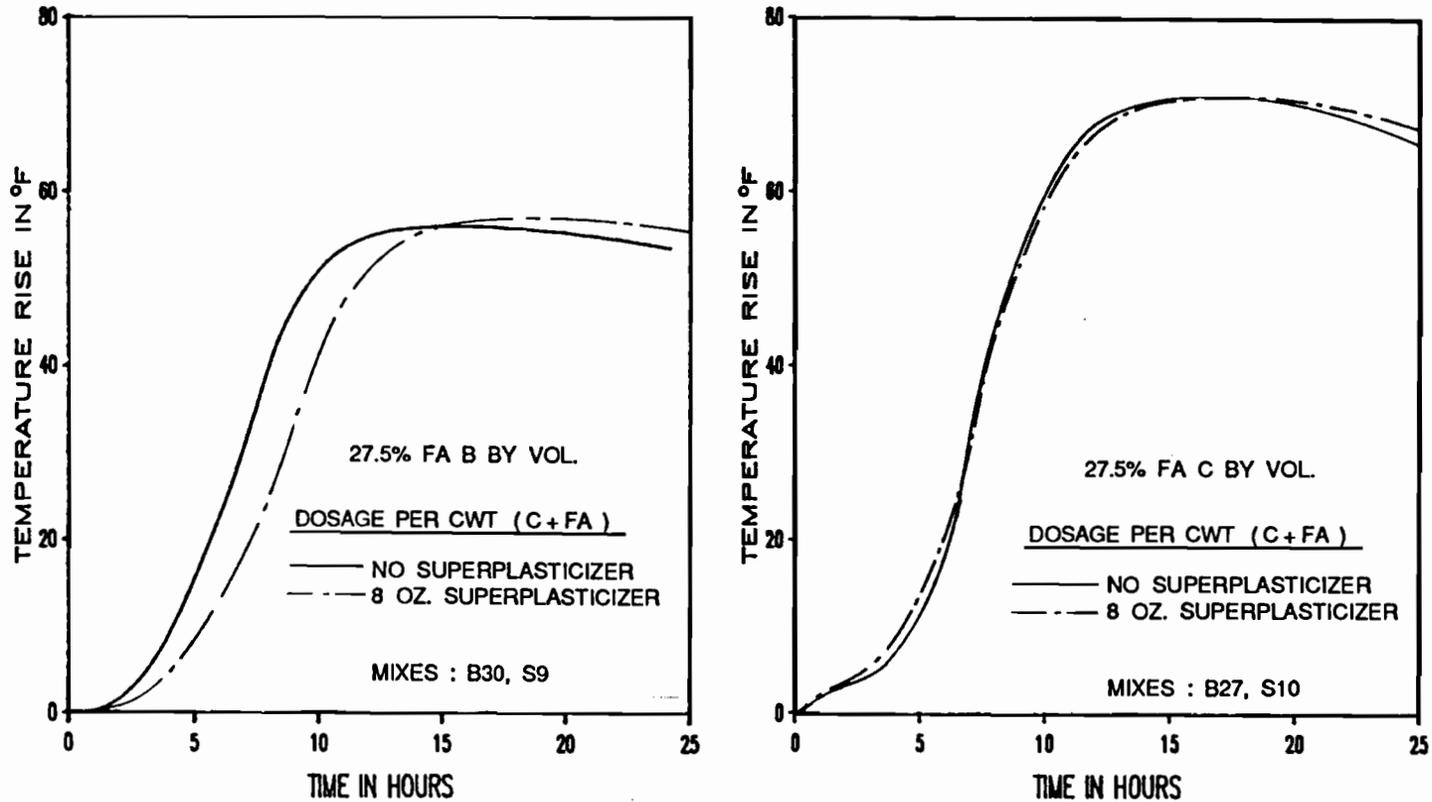
Figure 5.42 Effect of the addition of a superplasticizer on the temperature rise in Type I cement mortar containing fly ash.
