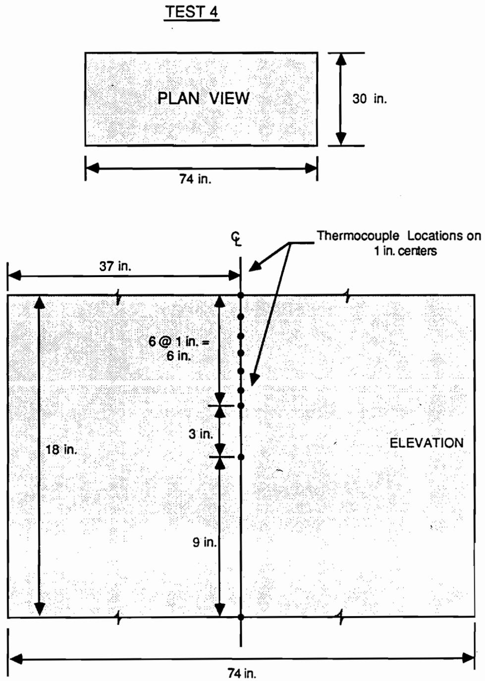
Figure 4.3 Dimensions and thermocouple locations for the samples used in Test 4.
