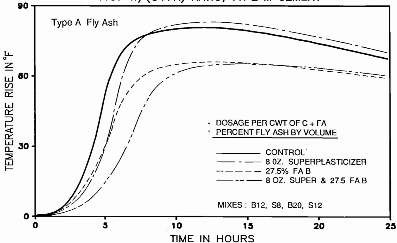
Figure 7.5 Effect of a superplasticizer on the temperature rise in Type III cement mortar with or without Type A fly ash.
