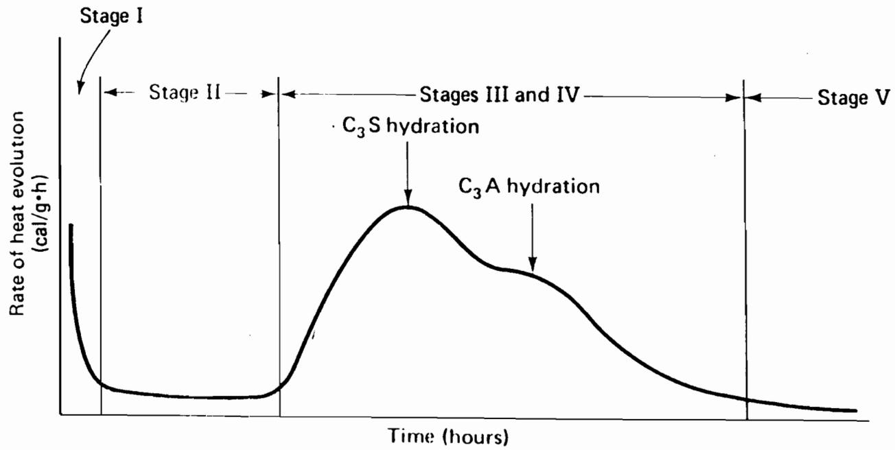
Figure 2.3 Rate of heat evolution during the hydration of Portland cement. [8]
