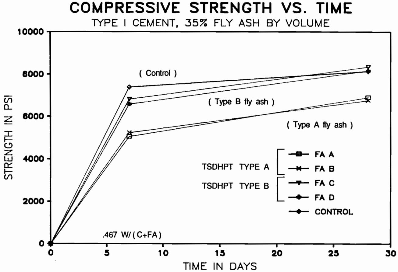
Figure 6.8 Strength development of Type I cement mortars containing fly ash.
