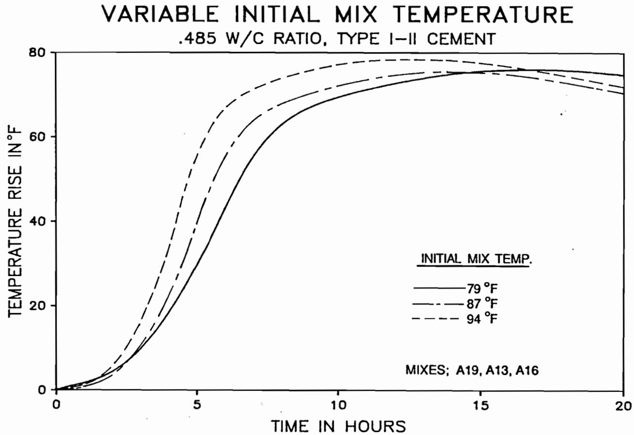
Figure 5.14 Effect of initial mix temperature on the temperature rise in mortar.
