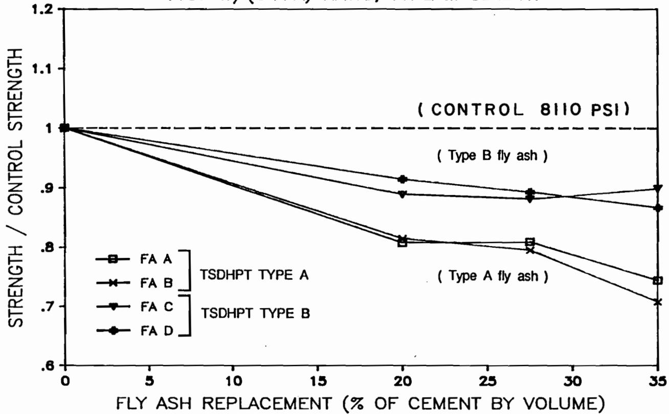
Figure 5.48 Relative compressive strength of Type III cement mortars containing fly ash at 7 days.
