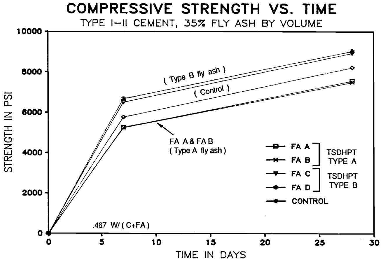
Figure 6.9 Strength development of Type I-II cement mortars containing fly ash.
