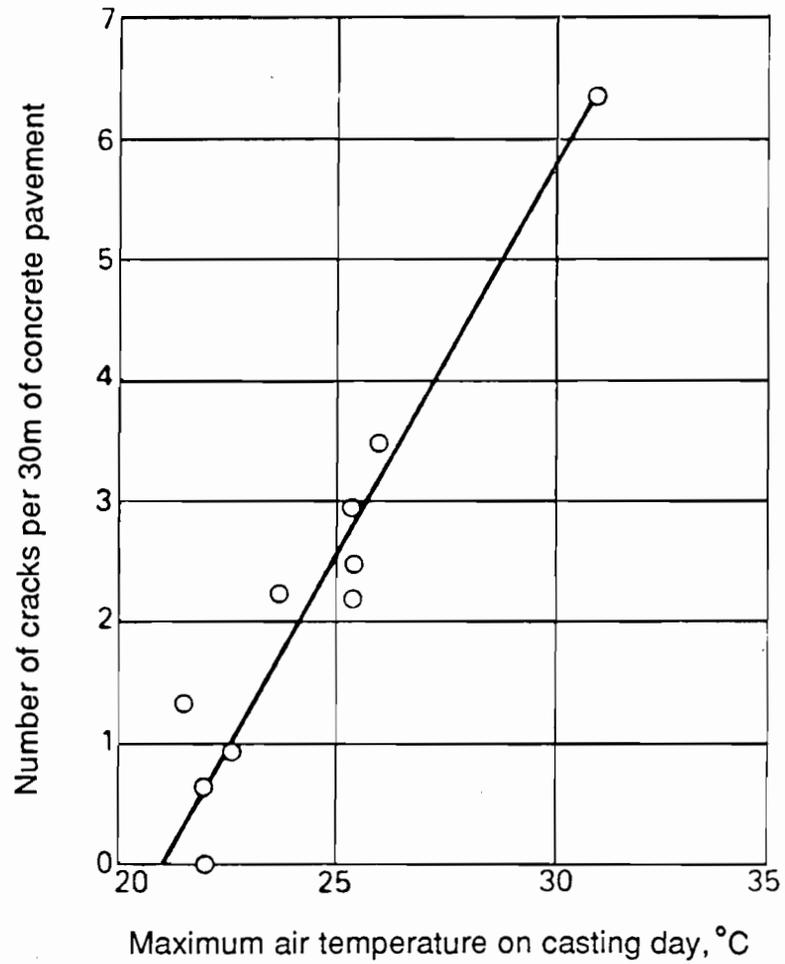
Figure 3.7 Number of Cracks per 30m of Day's Work vs. Maximum Air Temperature on Casting Day during construction of a concrete road in Great Britain. [23]
