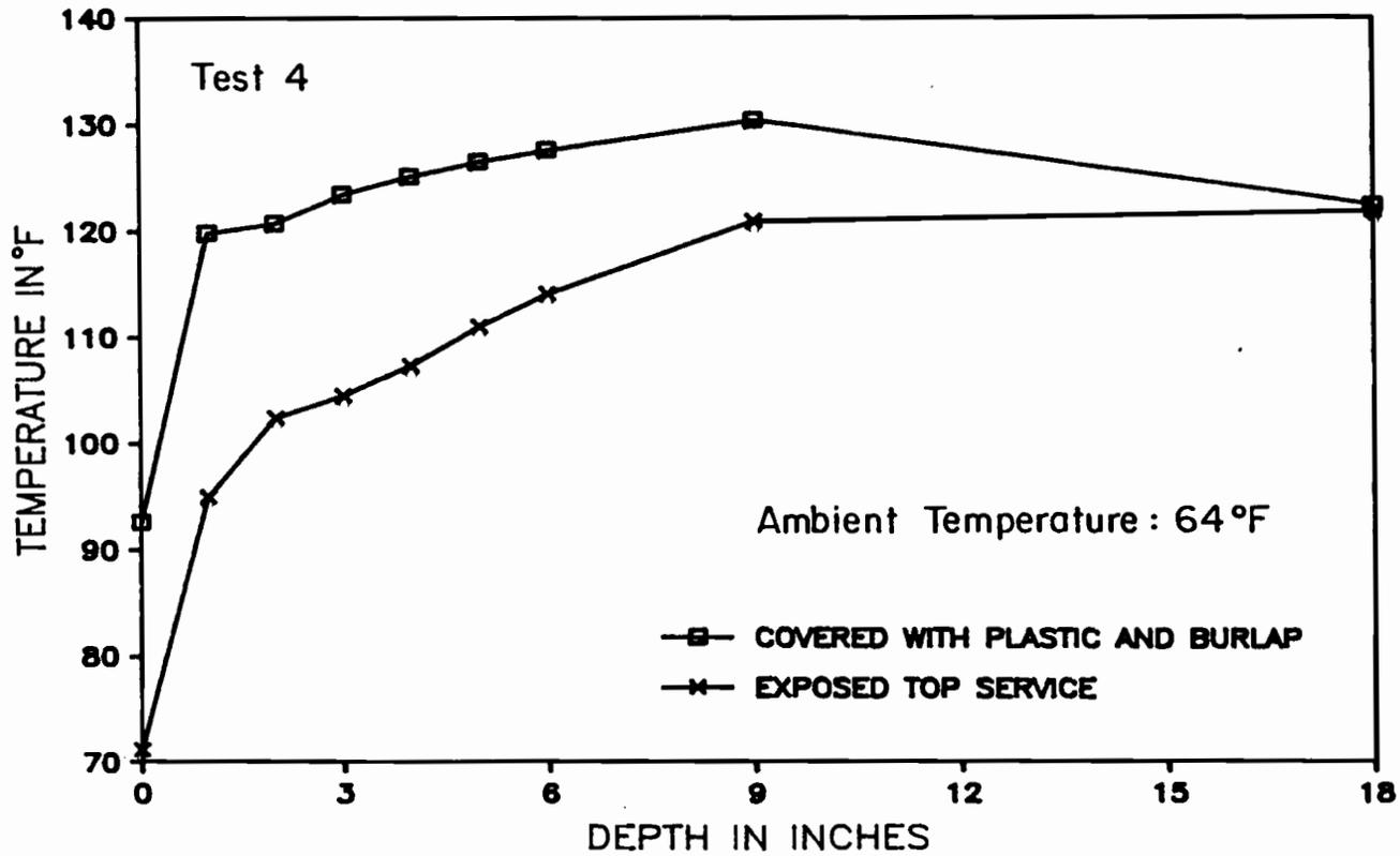
Figure 5.10 Maximum vertical temperature gradients for Test 4 samples.
