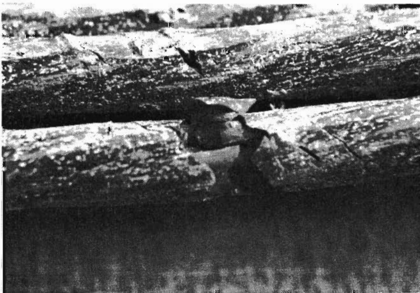
Figure 4.24 Fractures in epoxy coated strand
