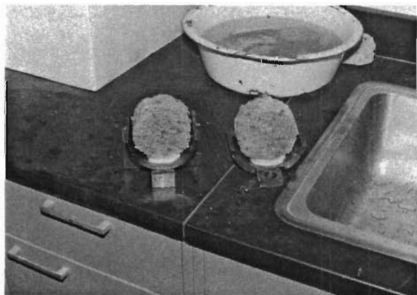
Fig 6.1. Cores being prepared for testing.
