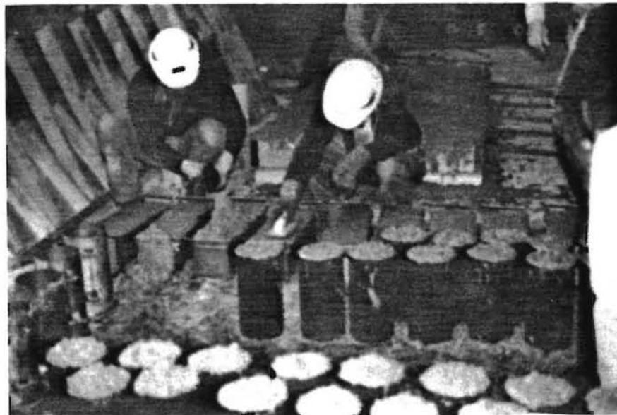
Fig 4.4. Preparing specimens for concrete strength tests.
