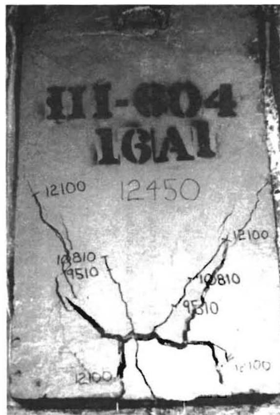
(b) Ultimate failure at 12.45 kips.
