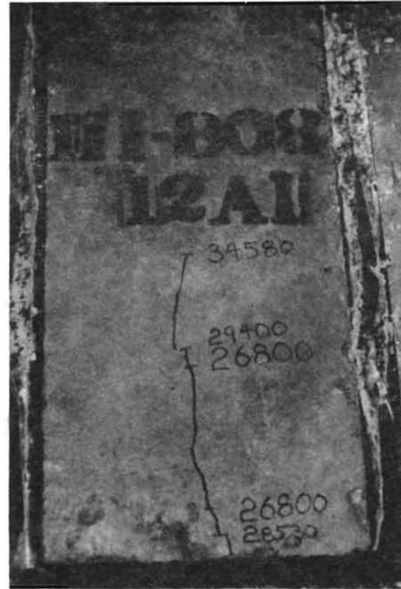
(b) Extended crack at 34.58 kips.
