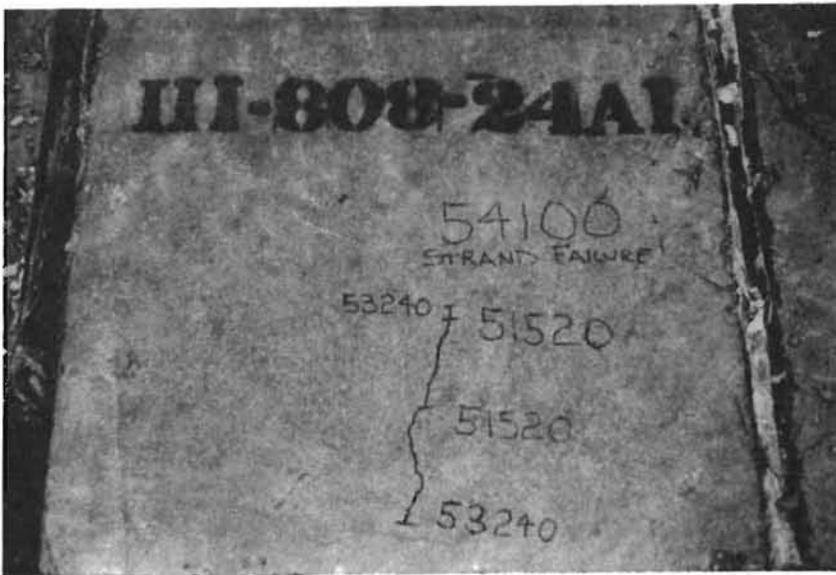
(b) Strand failure at 54.10 kips .
