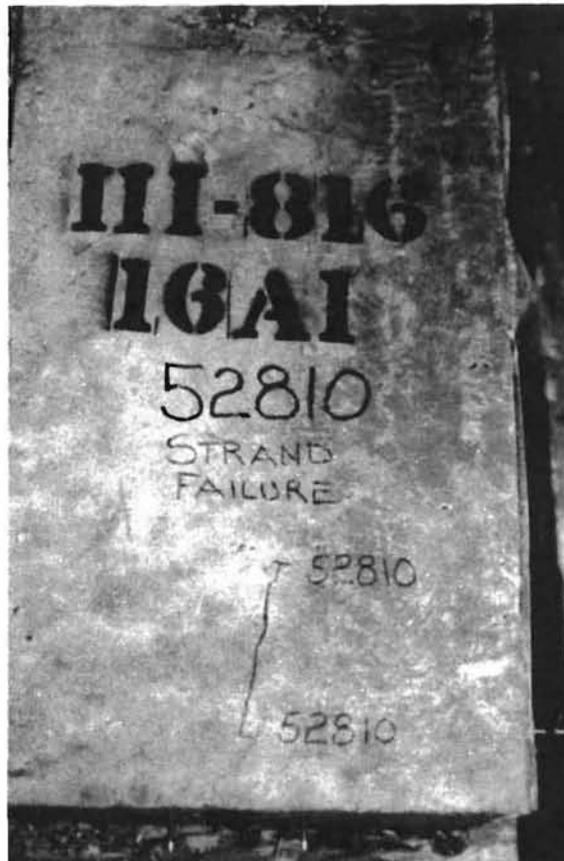
Fig B.29. First crack detected after strand failure at 52.81 kips for Specimen III 816-16A1.
