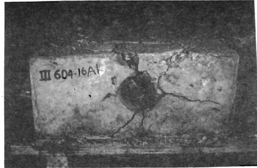
(f) Back edge of slab after ultimate failure.
