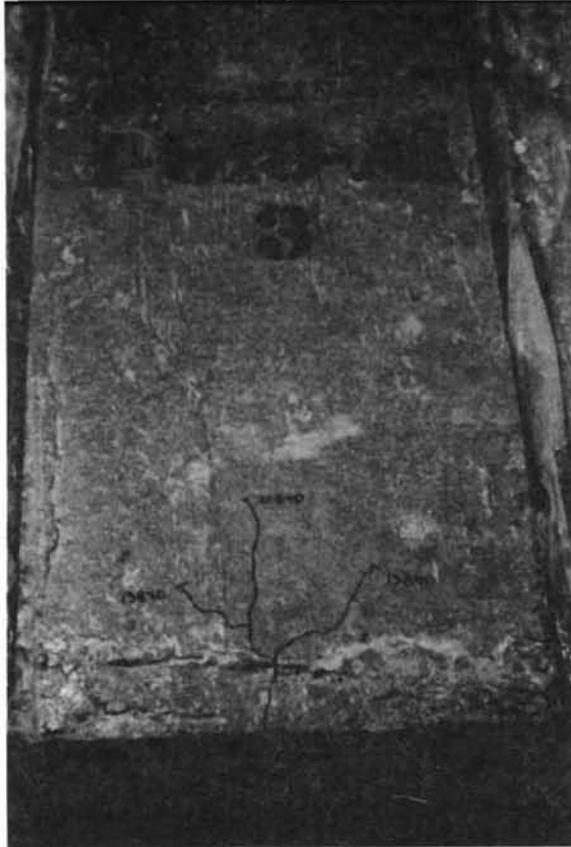
(a) First cracking at 13.84 kips.
