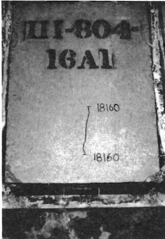
(a) First crack at 18.16 kips.
