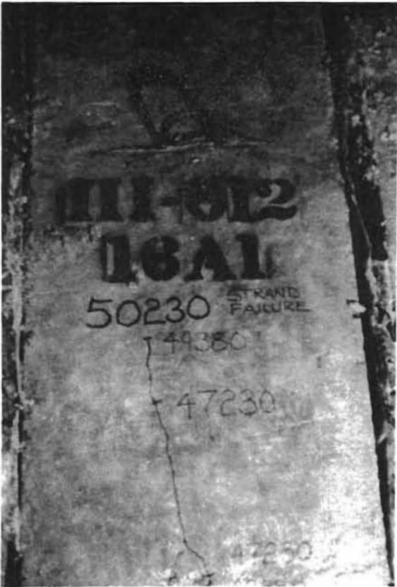
Fig B.24. First crack at 47.23 kips followed by strand failure at 50.23 kips for Specimen III 612-16A1.
