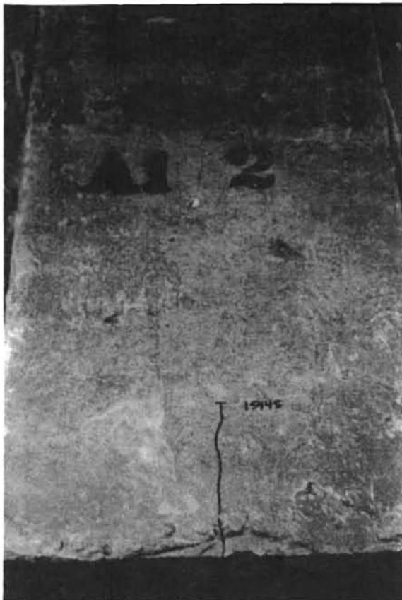
(a) First crack at 29.53 kips .
