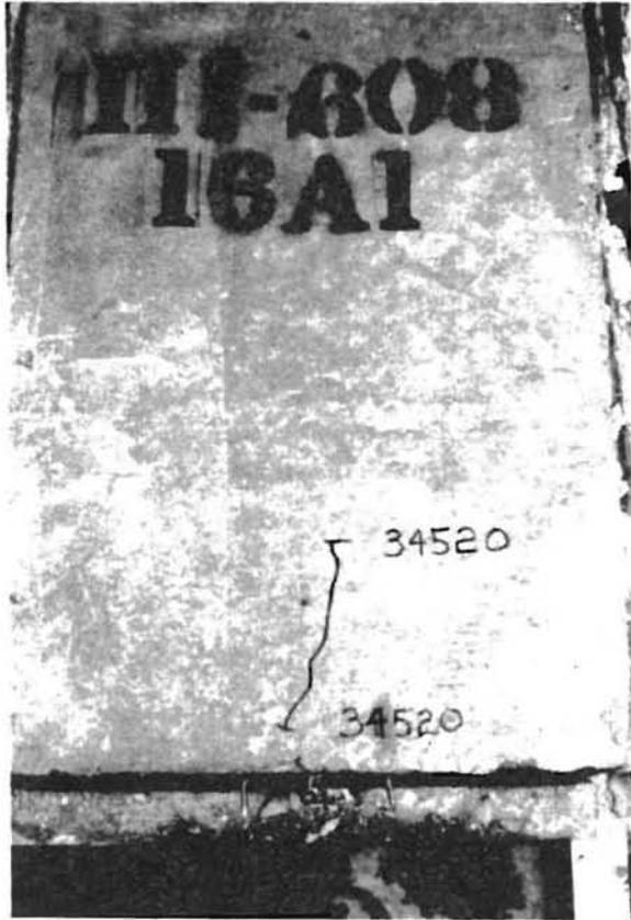
(a) First crack at 34.52 kips.
