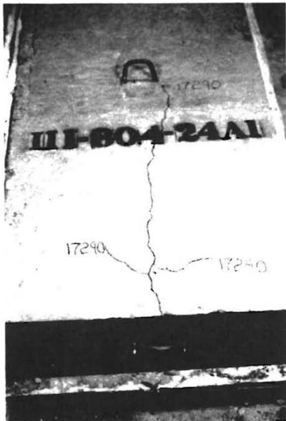
(a) First crack at 17.29 kips .
