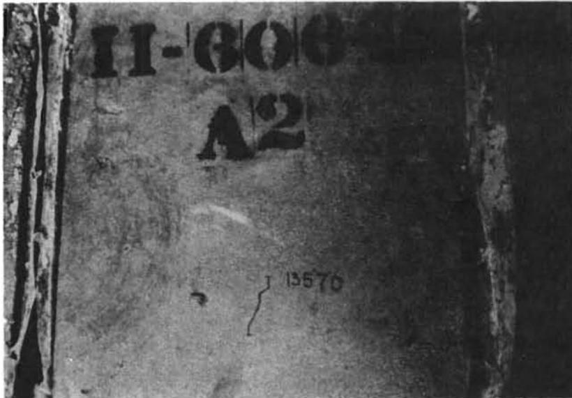
(a) First crack at 13.57 kips.
