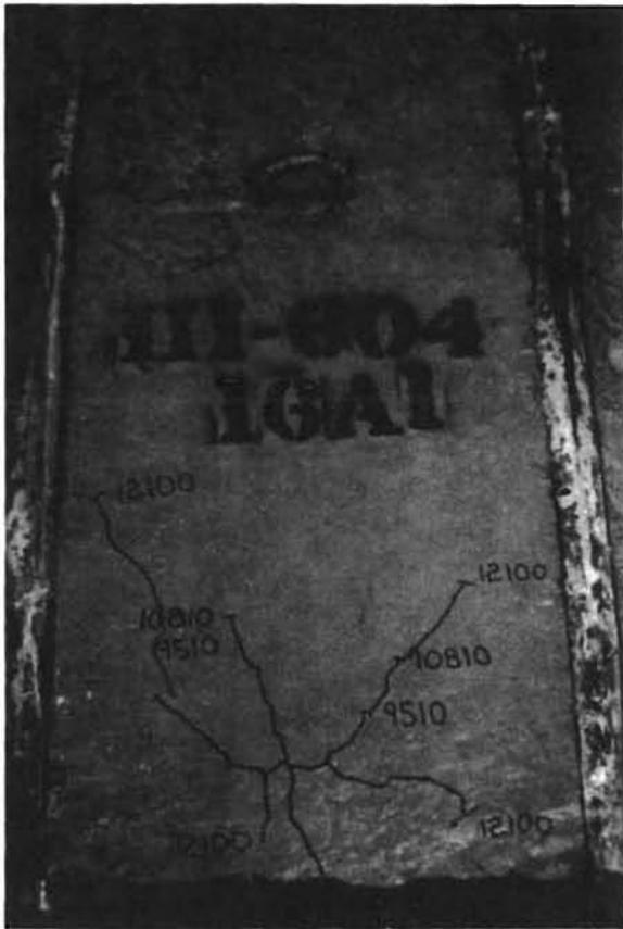
(c) Increased cracking at 12.10 kips.
