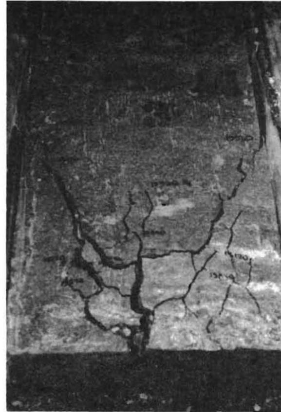
(b) Ultimate failure at 15.56 kips.
