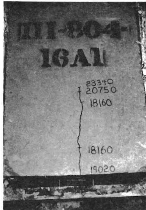
(b) Extended crack at 23.34 kips.
