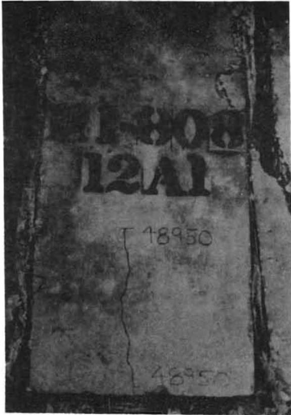
(a) First crack at 48.95 kips .
