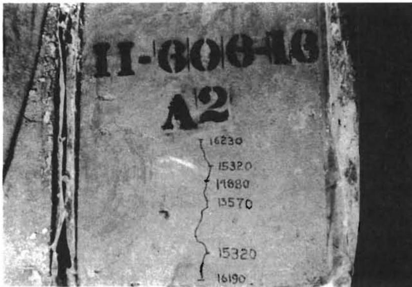
(b) Extended crack before ultimate failure at 19.00 kips.
