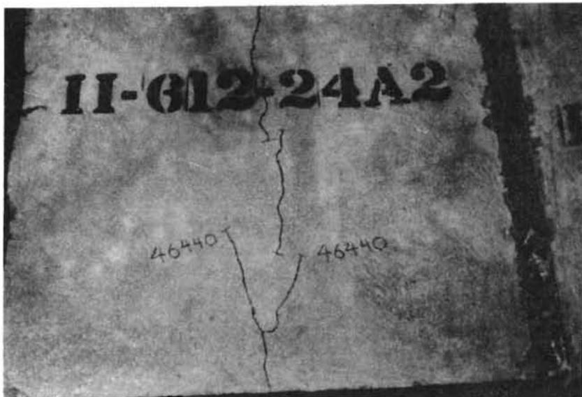
Fig B.10. First crack at 46.44 kips for Specimen II 612-24A2.
