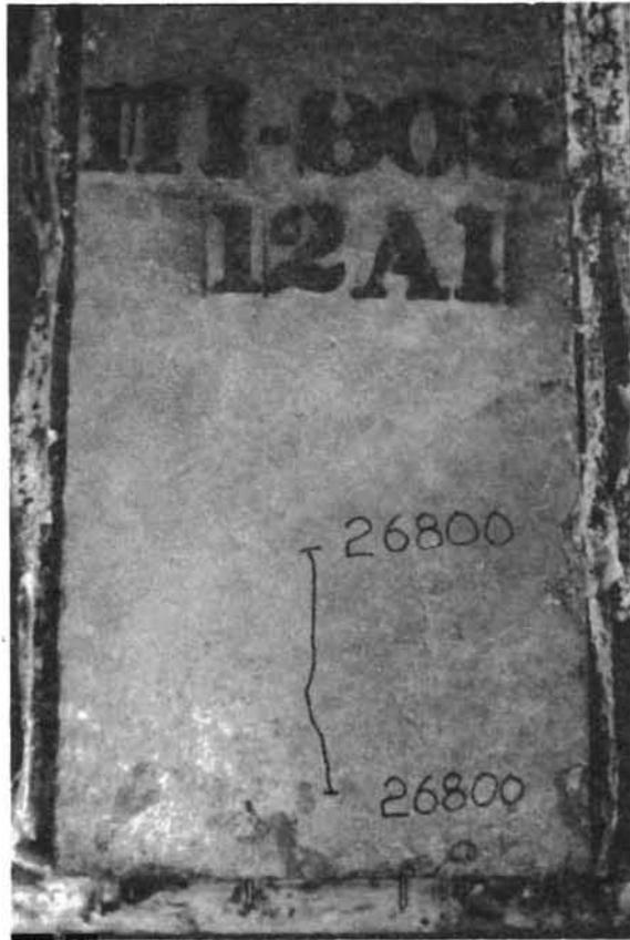
(a) First crack at 26.88 kips.
