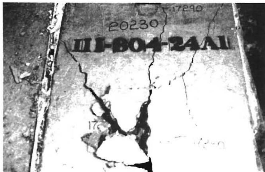
(b) Ultimate failure at 20.23 kips,
