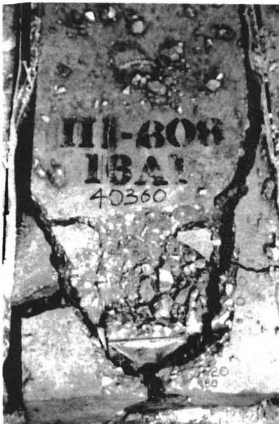
(c) Ultimate failure at 40.36 kips.
