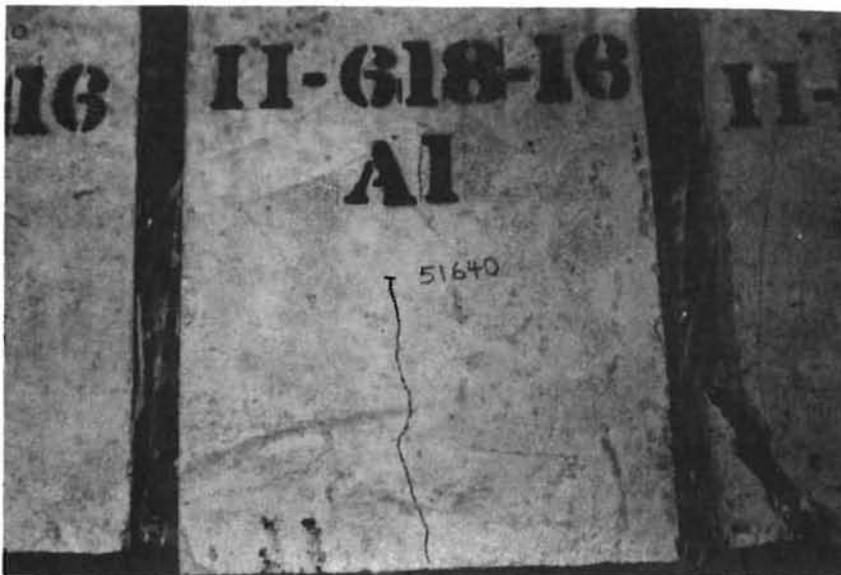
Fig B.12. First crack at 51.64 kips for Specimen II 618-16A1.
