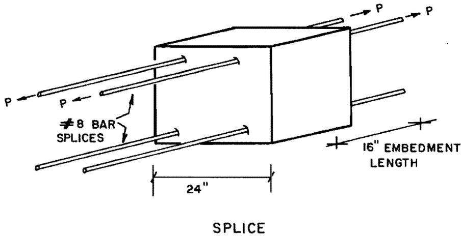
Fig. 2.3 Bond test specimens.
