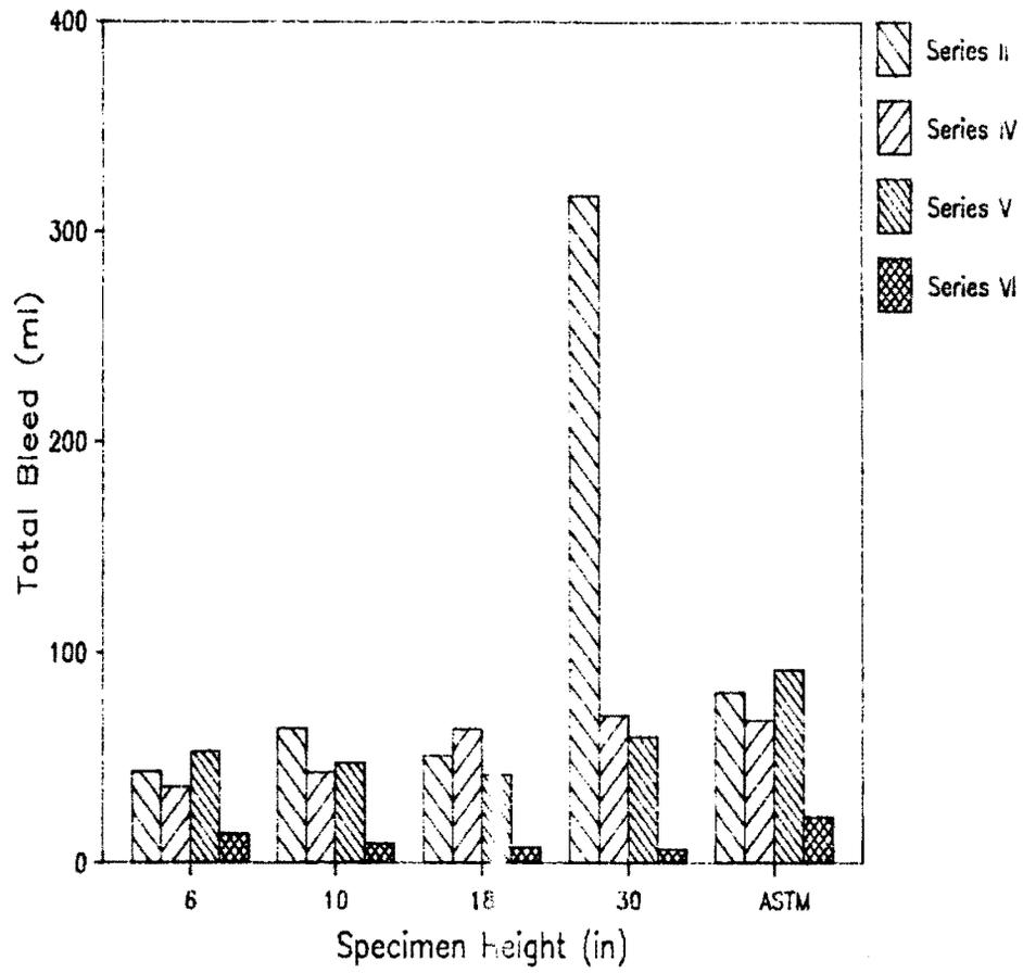
Fig. 4.7 Bleed vs. height--high slump
