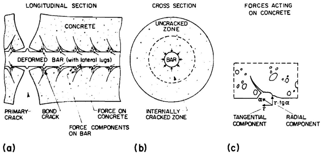
Fig. 1.2 Internal bond cracks and forces acting on concrete [20].
