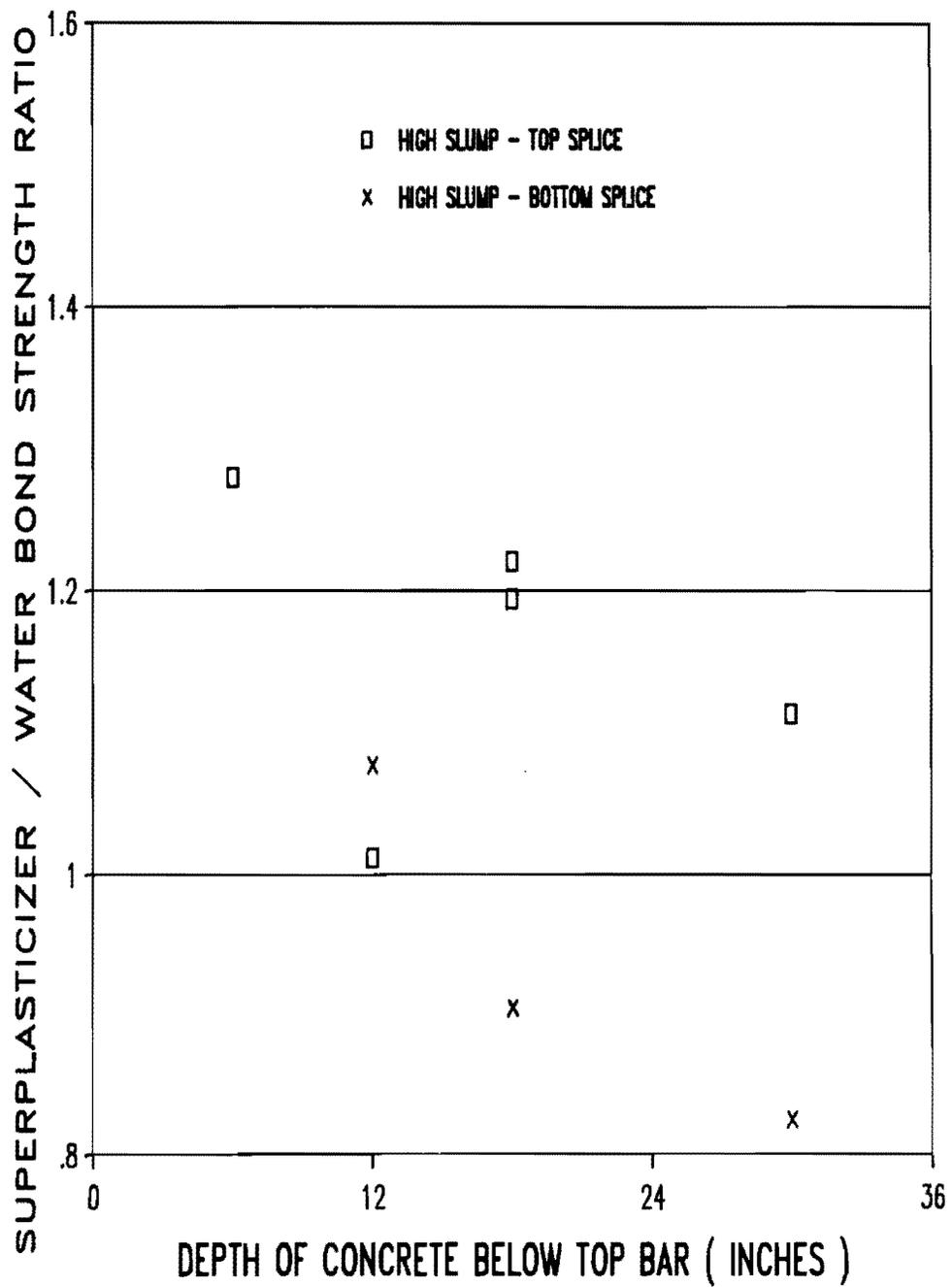
Fig. 3.18 High (6.5 in.) slump superplasticized concrete vs. high (7.5 in.) slump ordinary concrete - splice tests.
