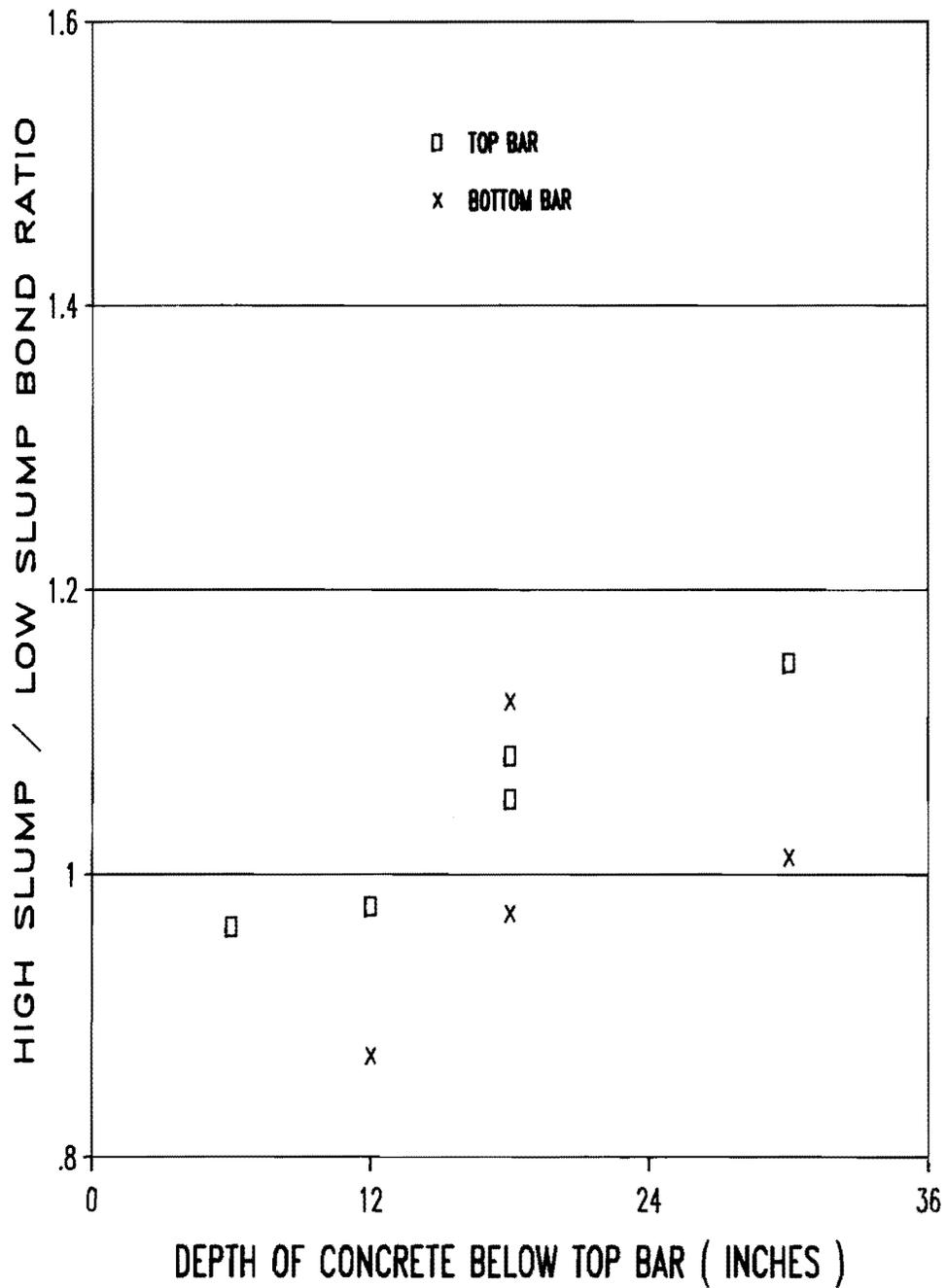
Fig. 3.14 Ratio of bond strength in high (7 in.) slump superplasticized concrete and low (2.5 in.) slump ordinary concrete. development test - low temperature (Series II).
