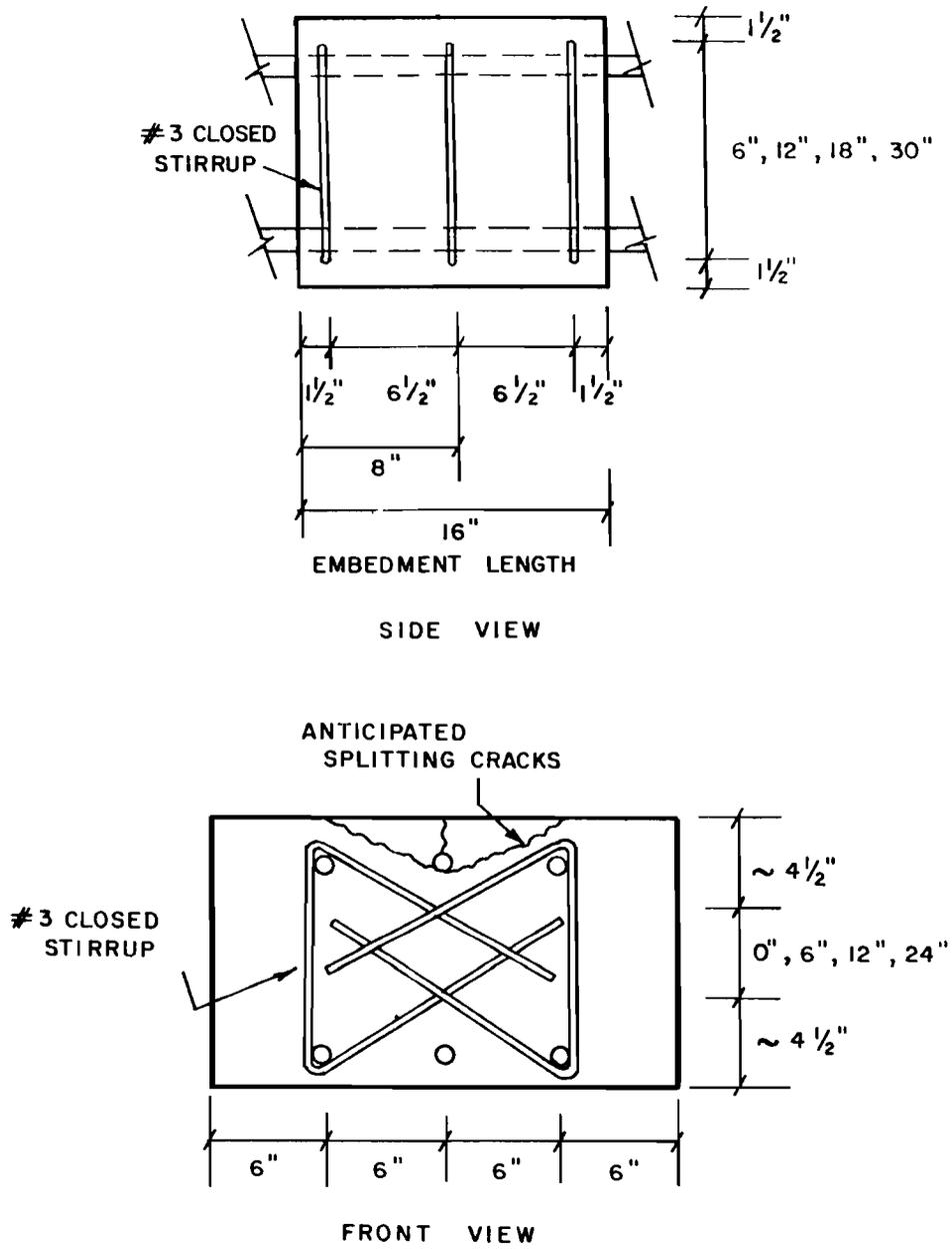
Fig. 2.5 Transverse reinforcement - development length test specimen.
