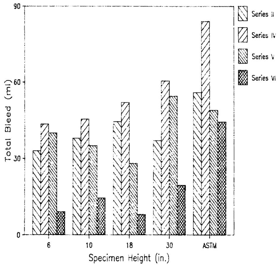
Fig. 4.6 Bleed vs. height--low slump
