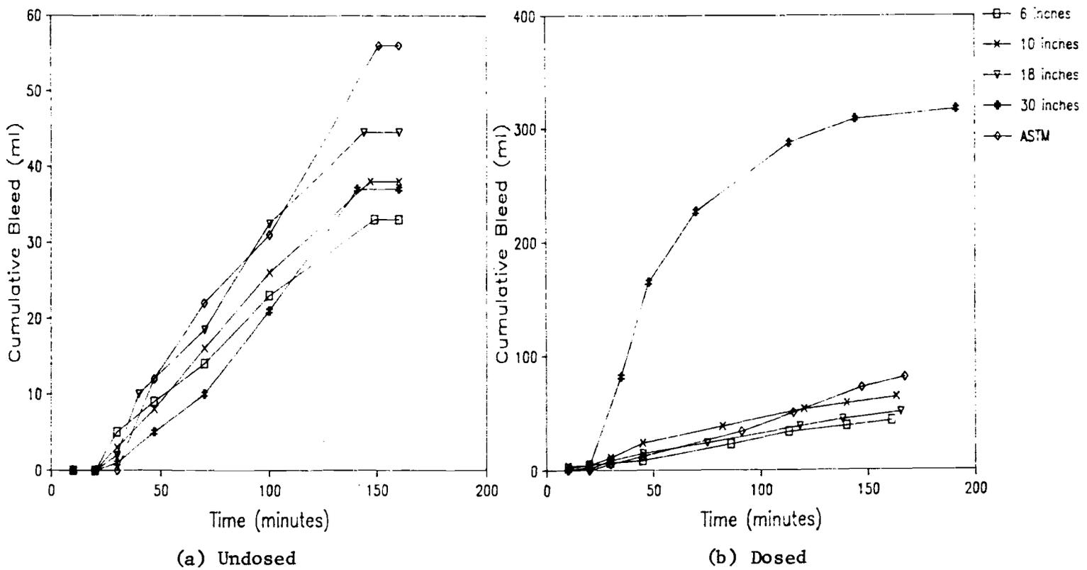
Fig. 4.1 Cumulative bleed vs. time, Series II
