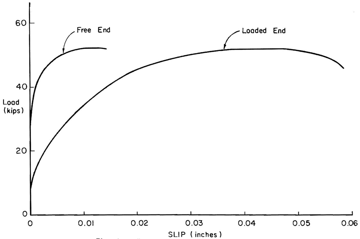
Fig. 3.3 Typical load vs. slip curves - #8 bar development length test.
