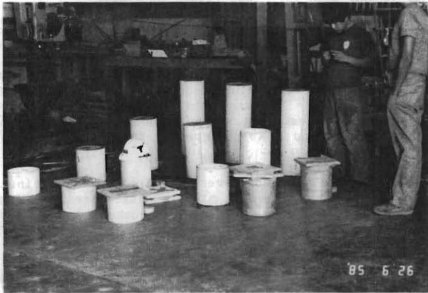
Fig. 2.14 Bleed containers arranged for testing.
