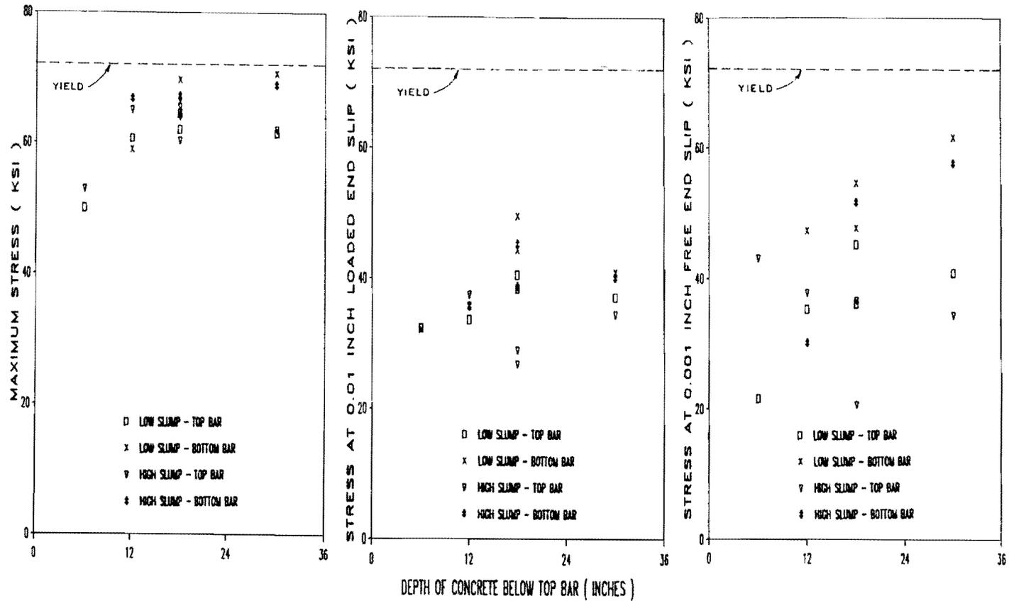
Fig. 3.6 Stress vs. specimen height. #8 development test - high temperature (Series VI).
