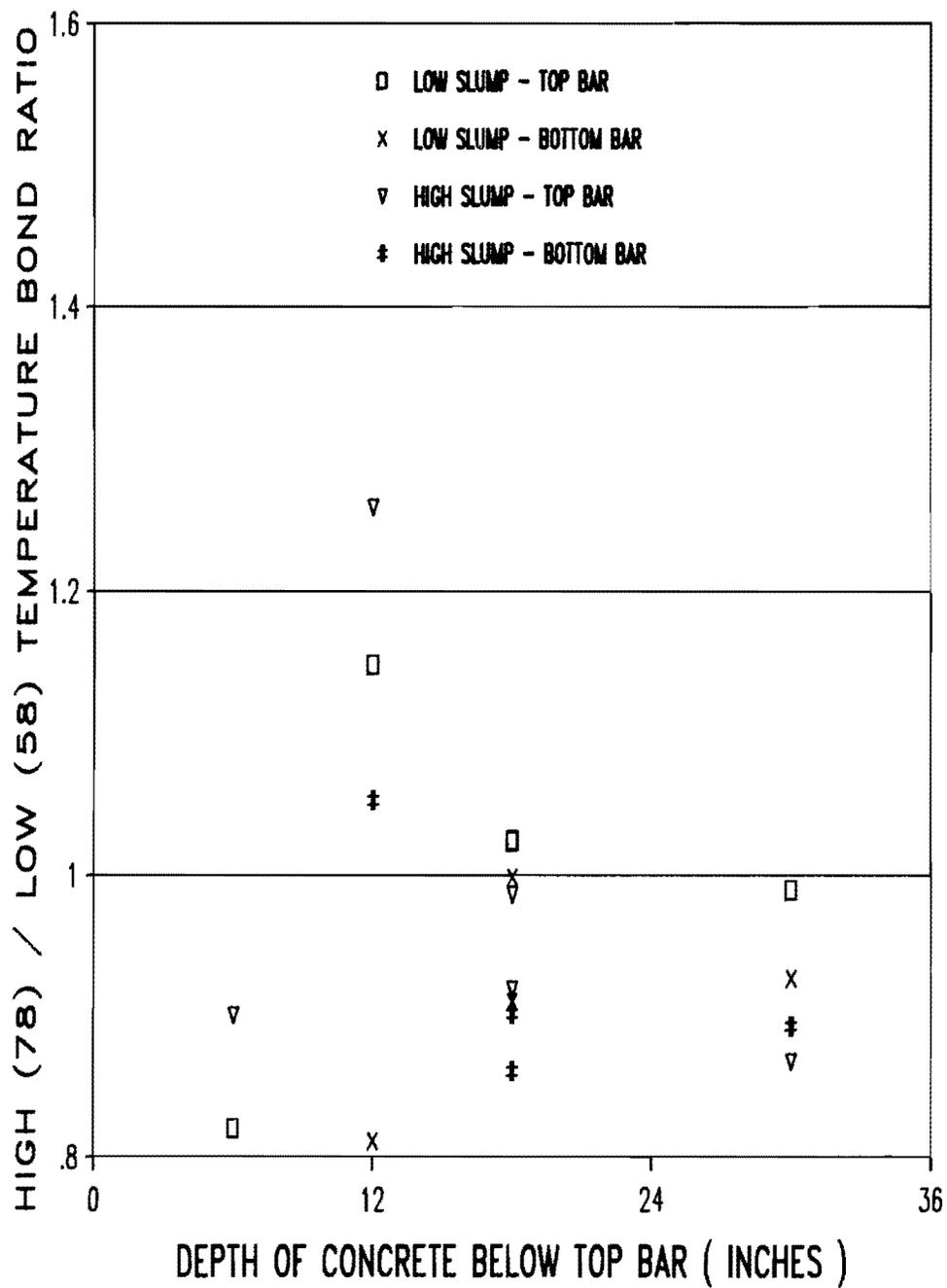
Fig. 3.19 Effect of casting temperature on bond capacity - development tests.
