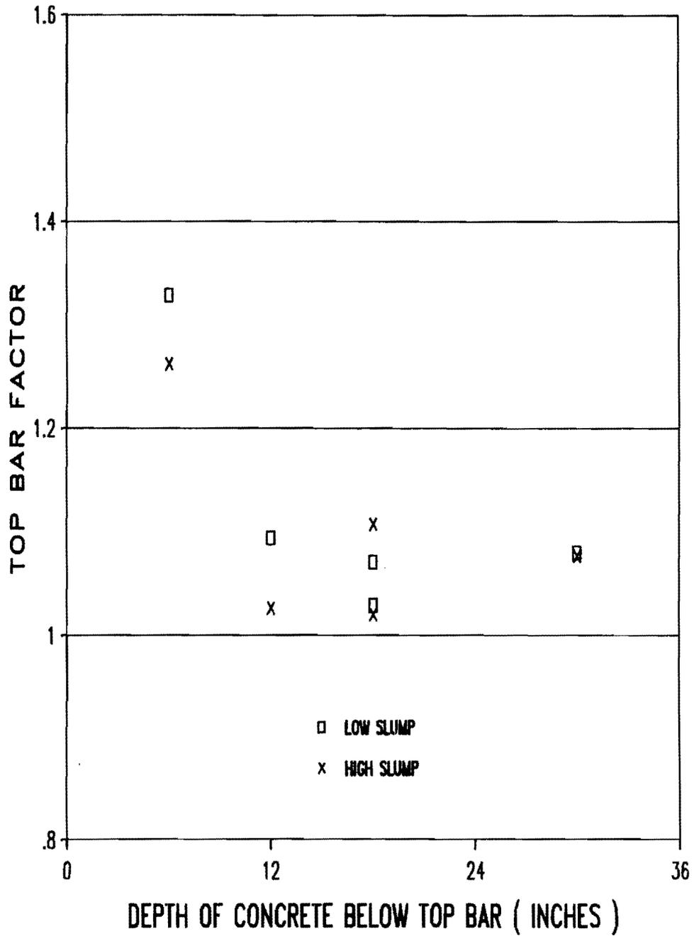
Fig. 3.23 Top bar development length factor. Series VI (high temperature).
