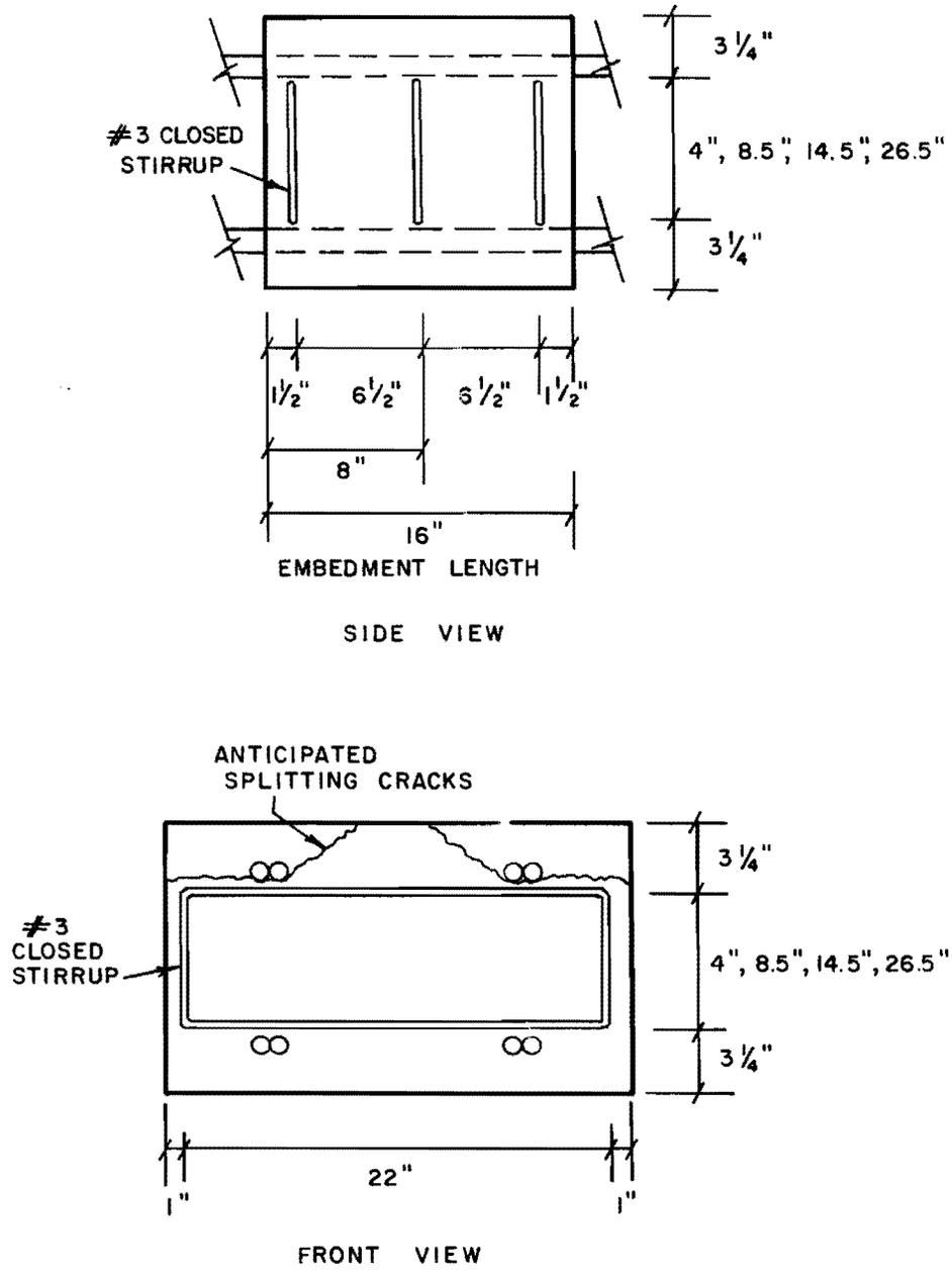
Fig. 2.6 Transverse reinforcement - splice test specimen.
