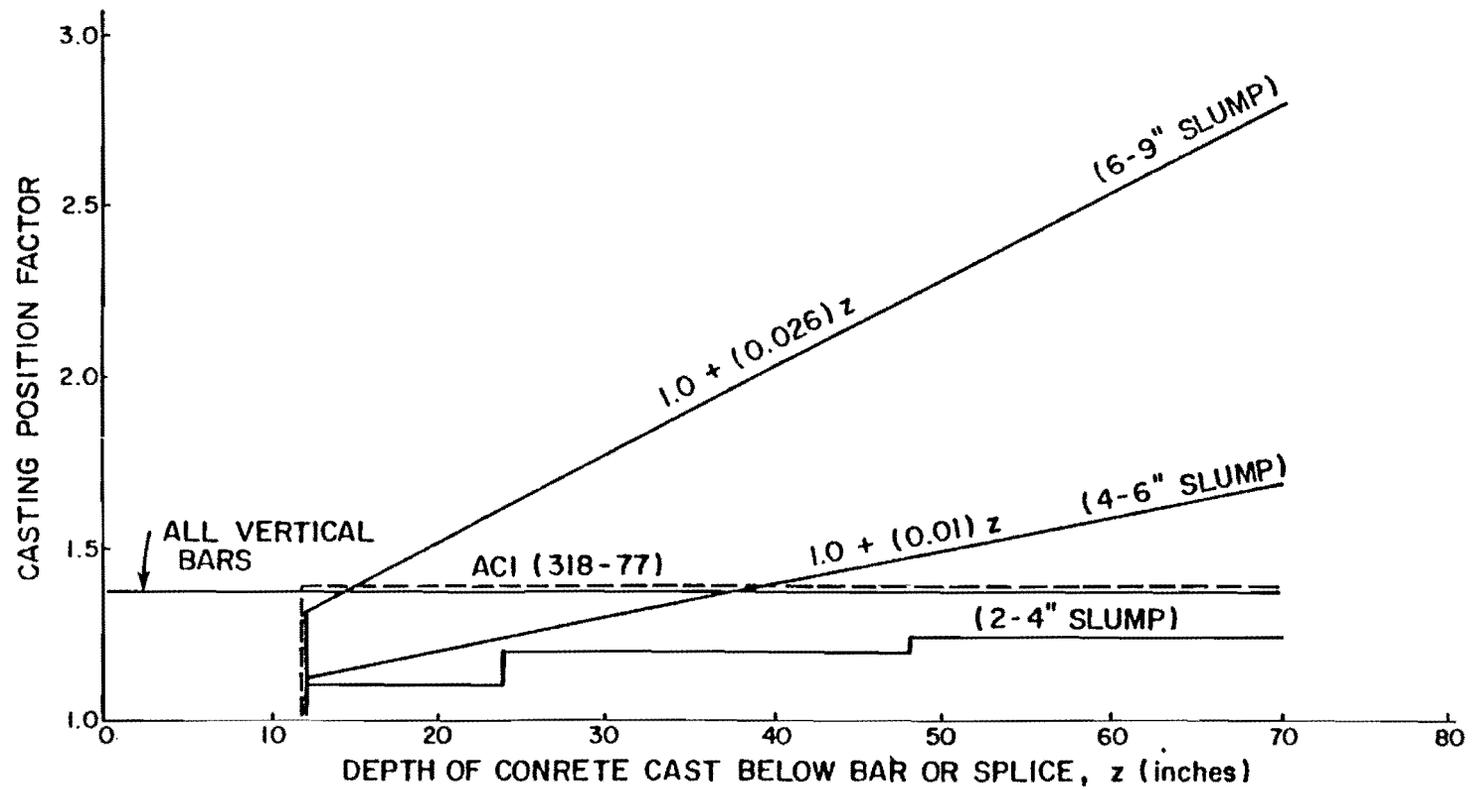
Fig. 1.6 Recommended casting position factors for all ranges of slump investigated [30].
