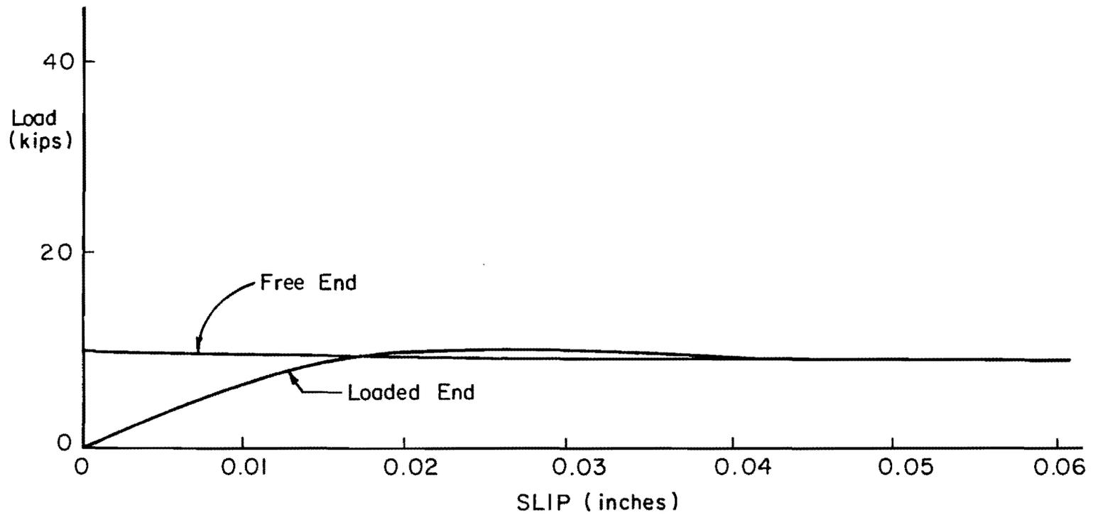
Fig. 3.12 Typical load vs. slip curves - 1/2 in. strand development length test.
