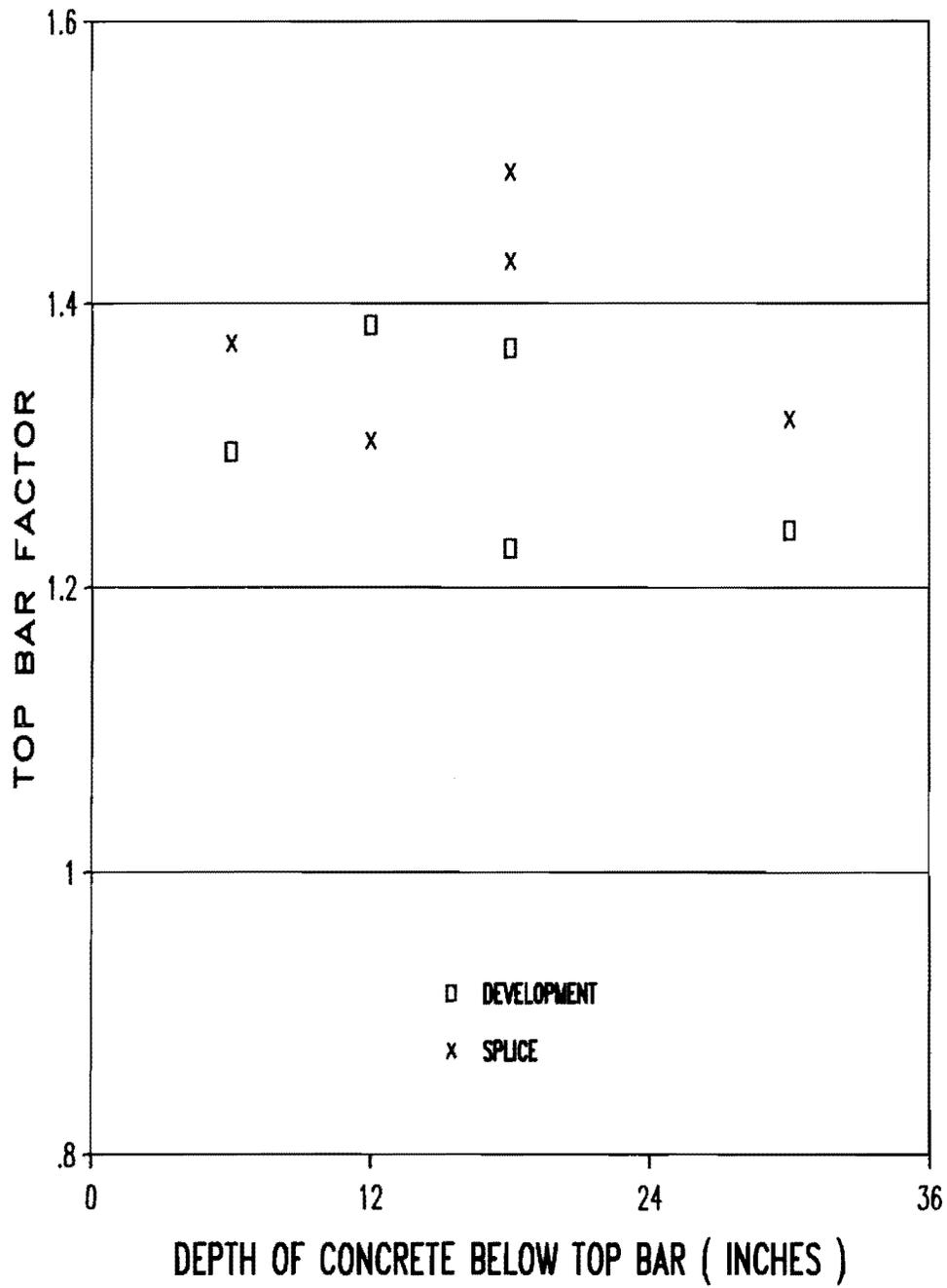
Fig. 3.22 Top bar and splice development length factor.
