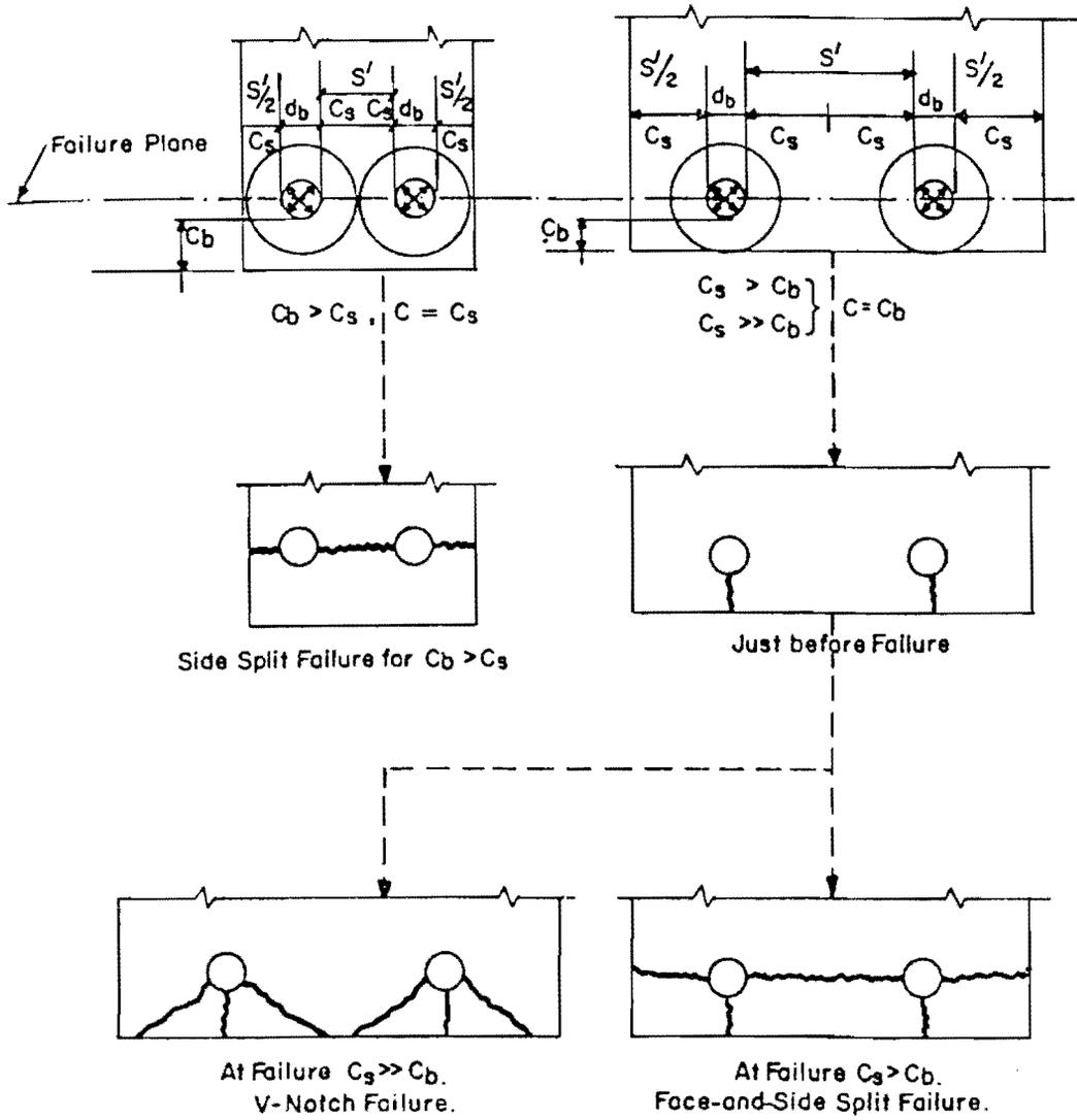
Fig. 1.3 Failure patterns of deformed bars [38].
