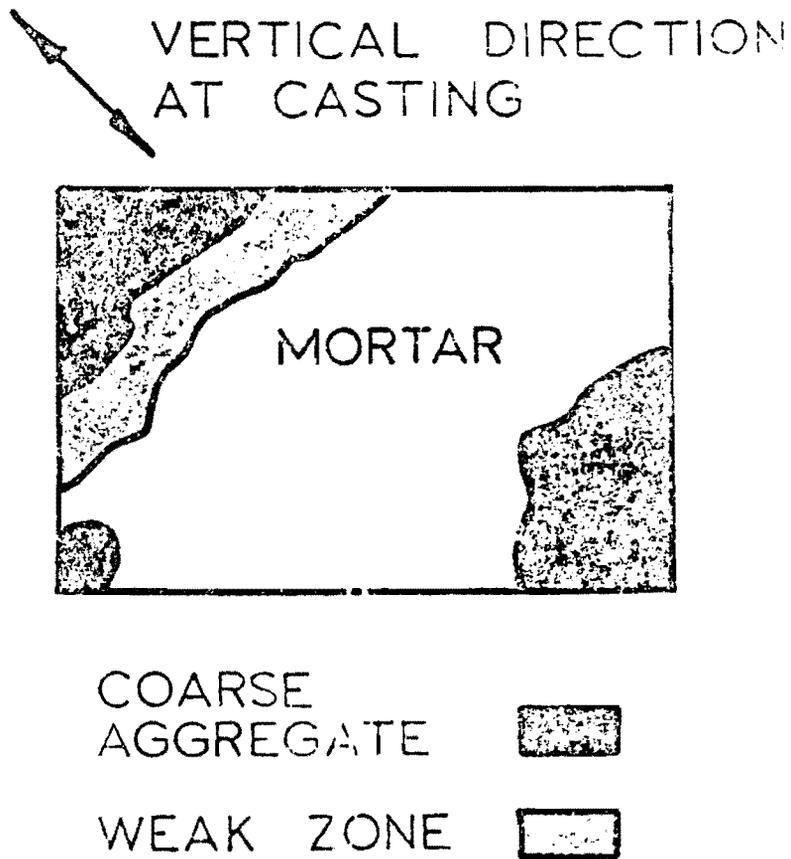
Fig. 1.9 Ground section showing weak pocket of mortar beneath a coarse aggregate particle (approx. magnification = X100) [7]
