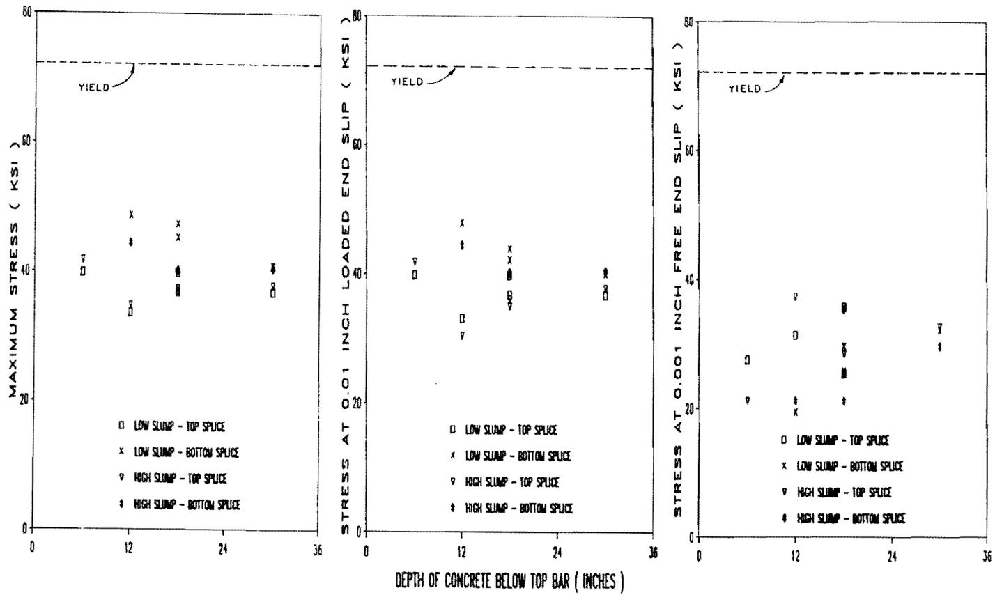
Fig. 3.10 Stress vs. specimen height. #8 splice test (Series IV).
