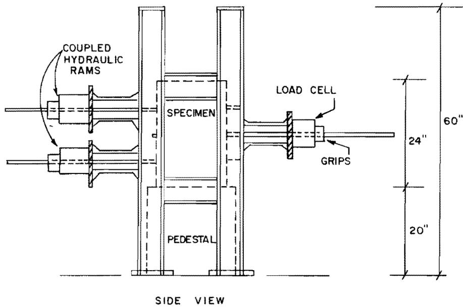
Fig. 2.15 Test frame (schematic)
