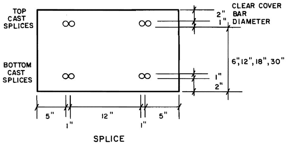
Fig. 2.4 Front view of test specimens.
