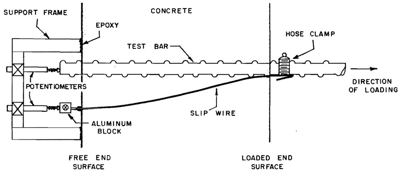
Fig. 2.19 Top view of slip wire arrangement.
