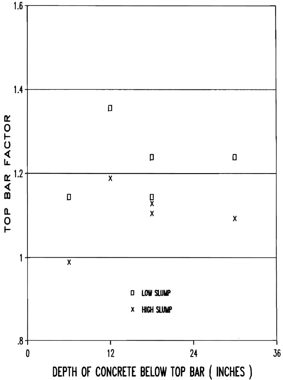
Fig. 3.21 Top splice development length factor. Series IV (low temperature).
