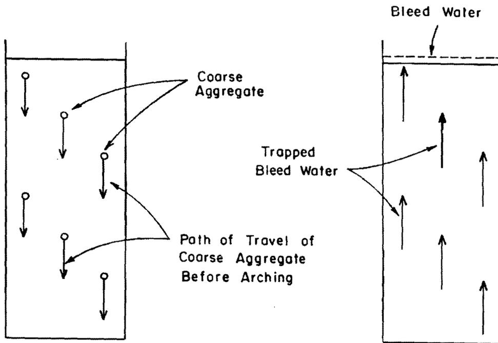
Fig. 4.8 Schematic model for bleed-settlement of coarse aggregate phenomena
