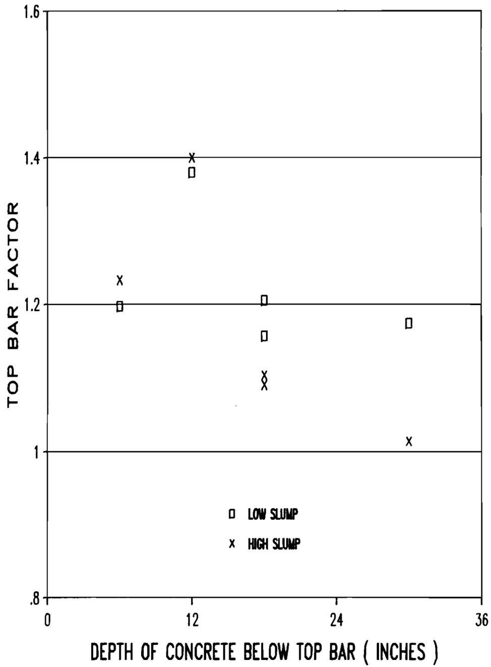
Fig. 3.20 Top bar development length factor. Series II (low temperature).
