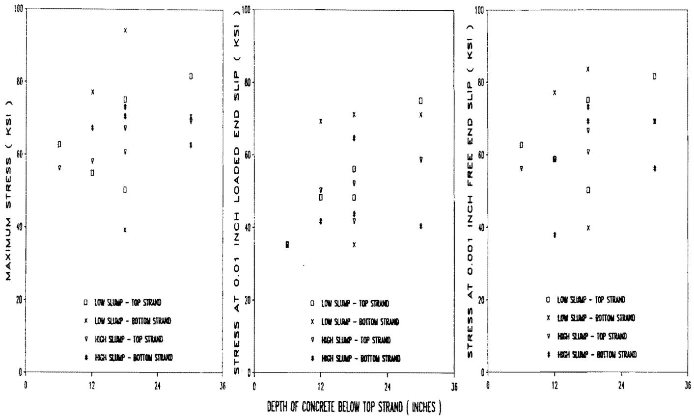
Fig. 3.13 Stress vs. specimen height. 1/2 in. strand development length test.
