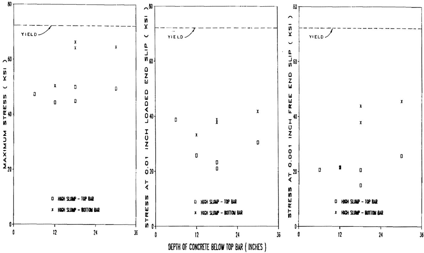
Fig. 3.5 Stress vs. specimen height. #8 development test - high slump concrete, no superplasticizer (Series V).
