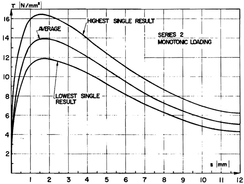
Fig. 1.1 Typical local bond stress-slip relationship measured in a slip-controlled test [16].
