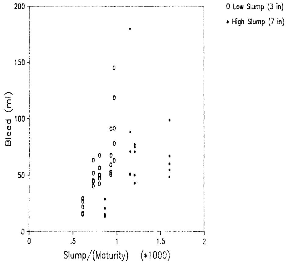
Fig. 4.10 Bleed vs. slump--maturity ratio
