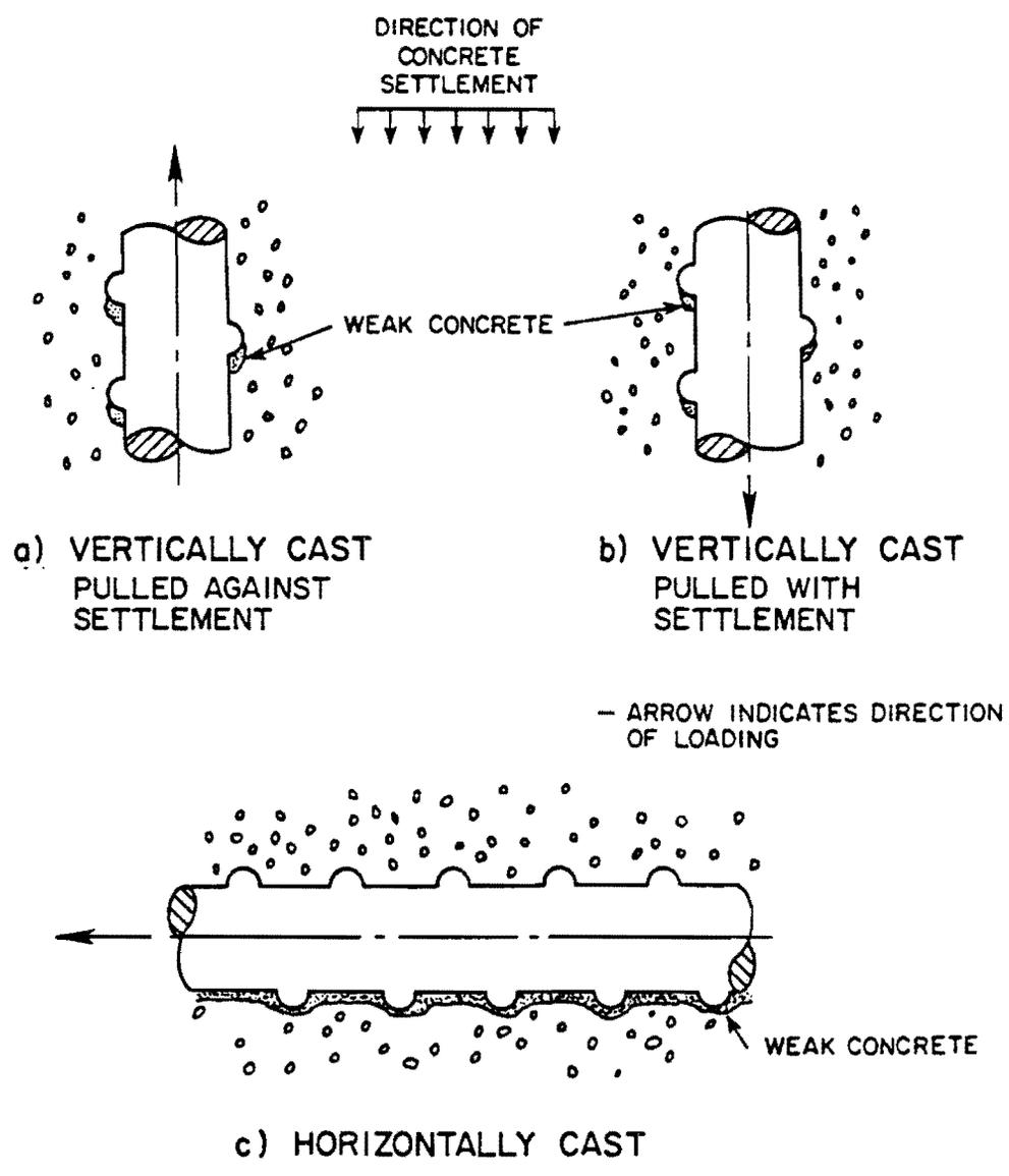
Fig. 1.5 Definition of casting position [30].
