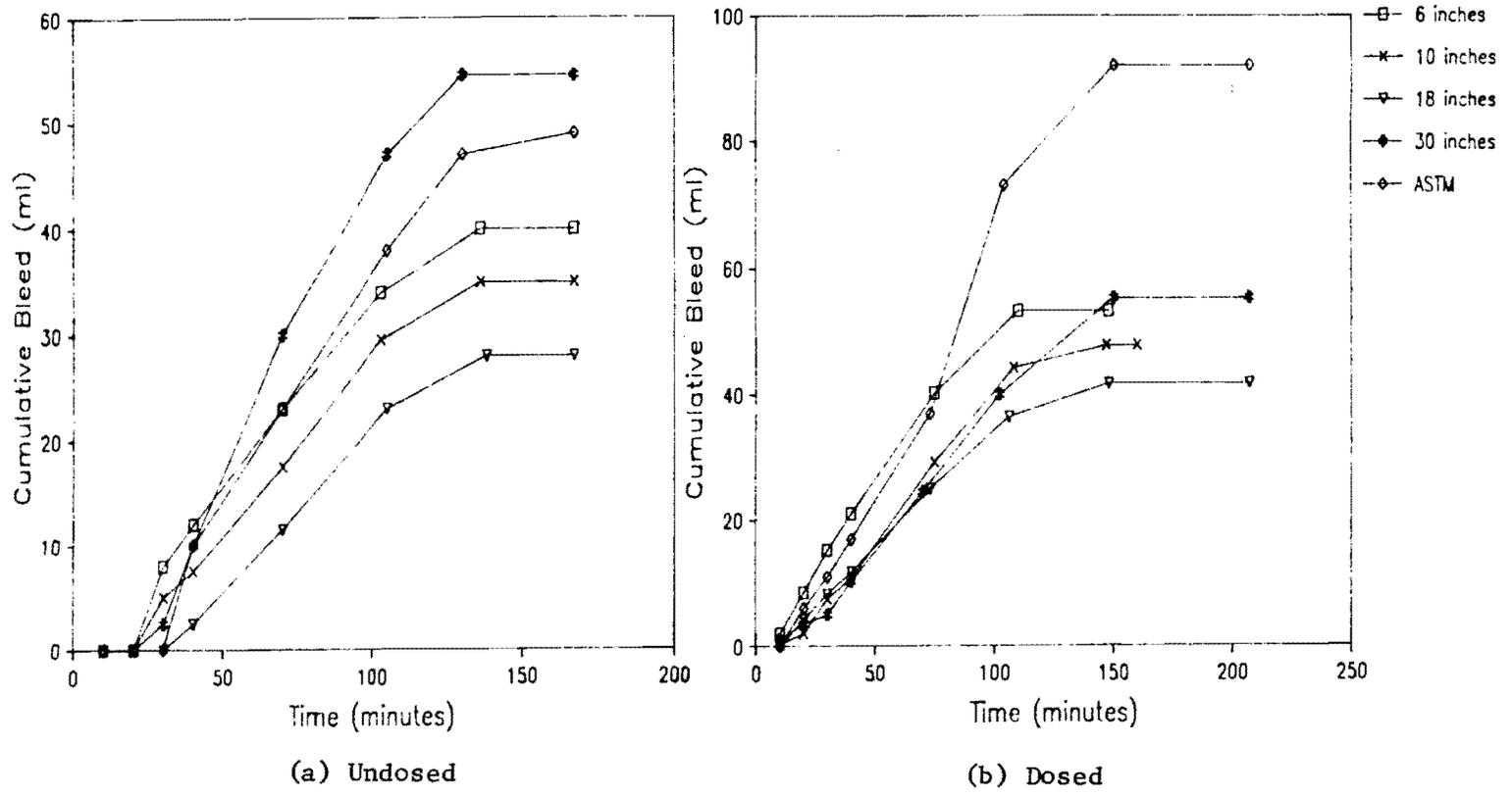
Fig. 4.4 Cumulative bleed vs. time, Series V
