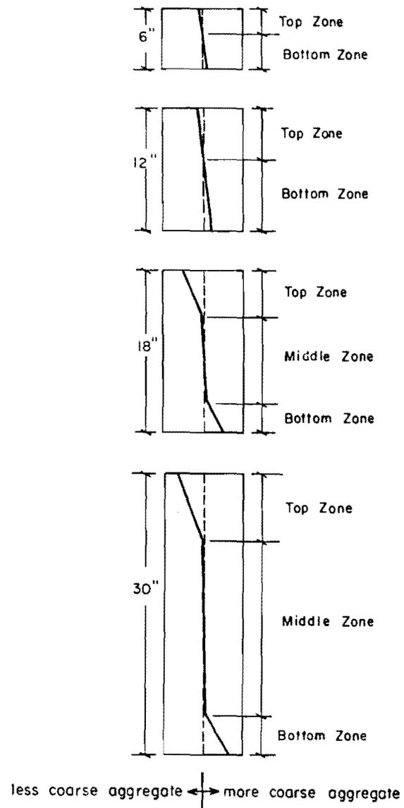
Fig. 4.9 Segregation of coarse aggregate [42]
