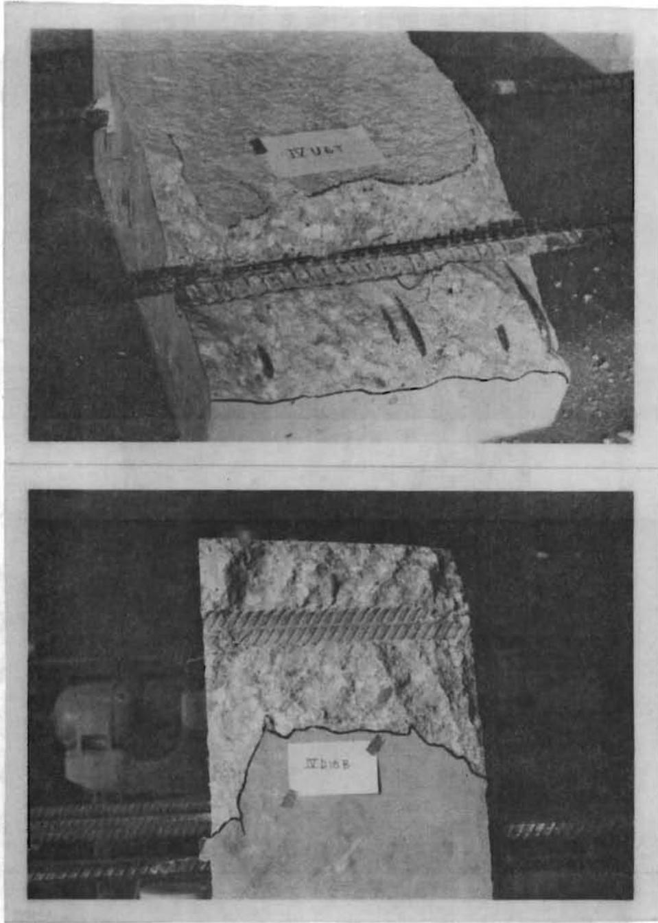
Fig. 3.8 Failure surface - #8 splice specimens.
