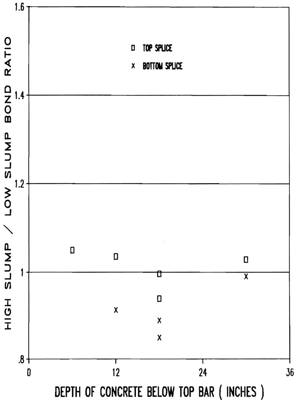
Fig. 3.15 Ratio of bond strength in high (6.5 in.) slump superplasticized concrete and low (3 in.) slump ordinary concrete. Splice test (Series IV).
