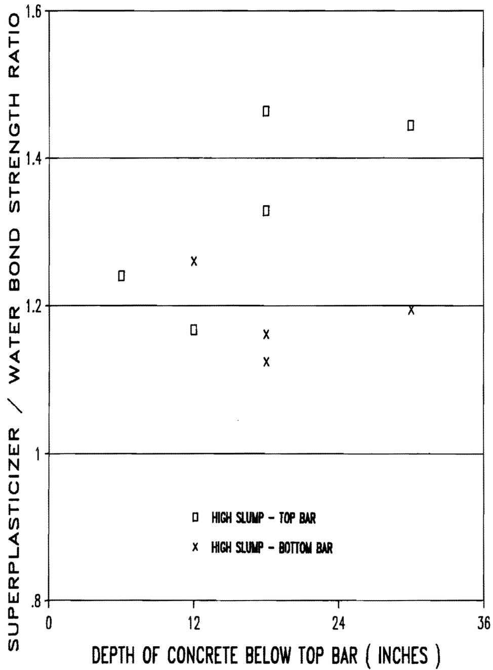
Fig. 3.17 High (7 in.) slump superplasticized concrete vs. high (7.5 in.) slump ordinary concrete - development tests.
