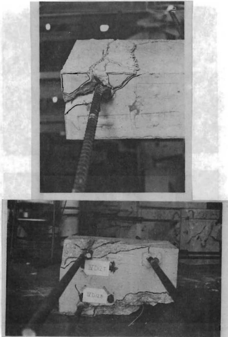
Fig. 3.7 Crack Pattern - #8 splice specimens.
