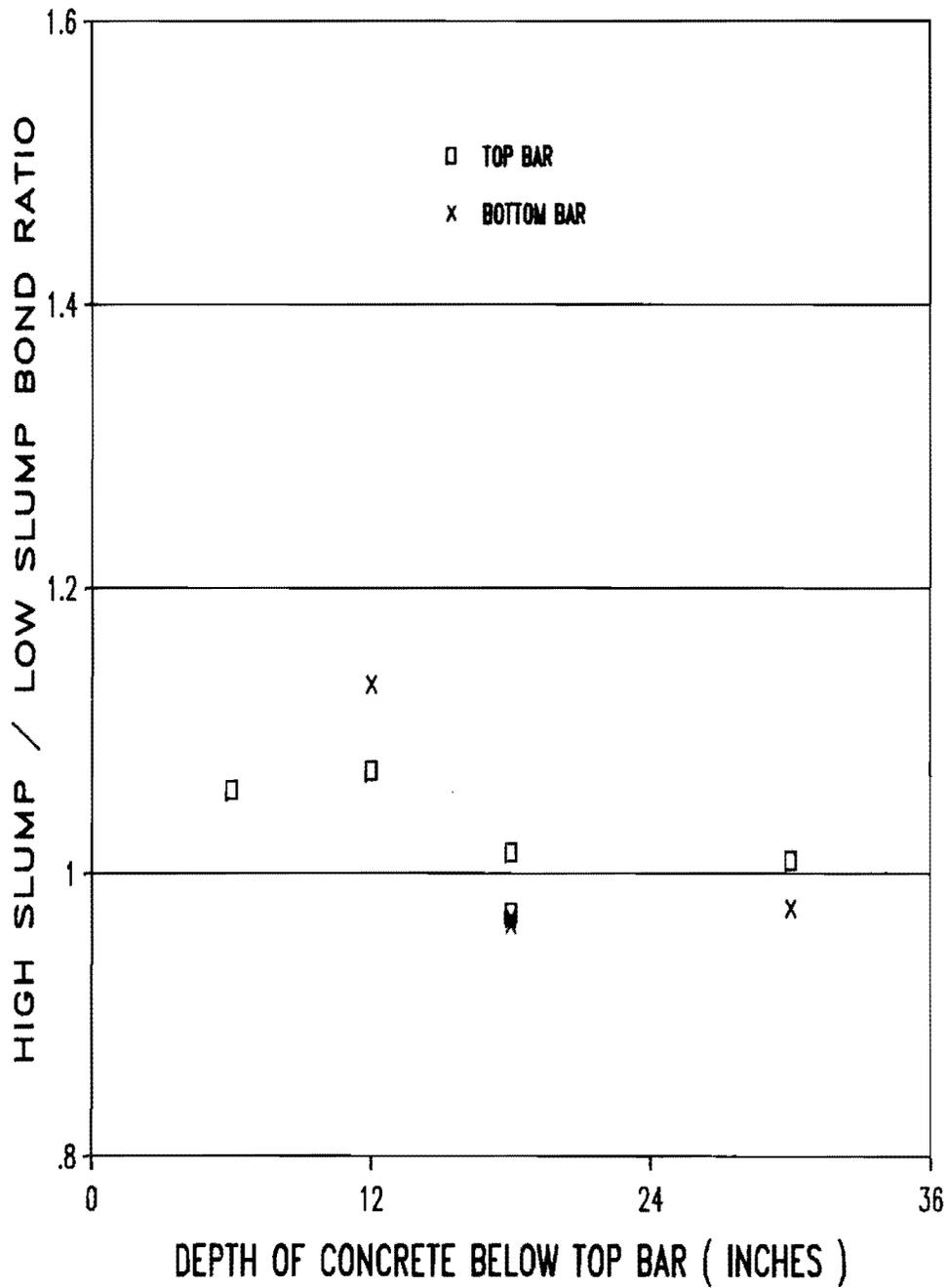
Fig. 3.16 Ratio of bond strength in high (7.5 in.) slump superplasticized concrete and low (3 in.) slump ordinary concrete. Development test - high temperature (Series VI).
