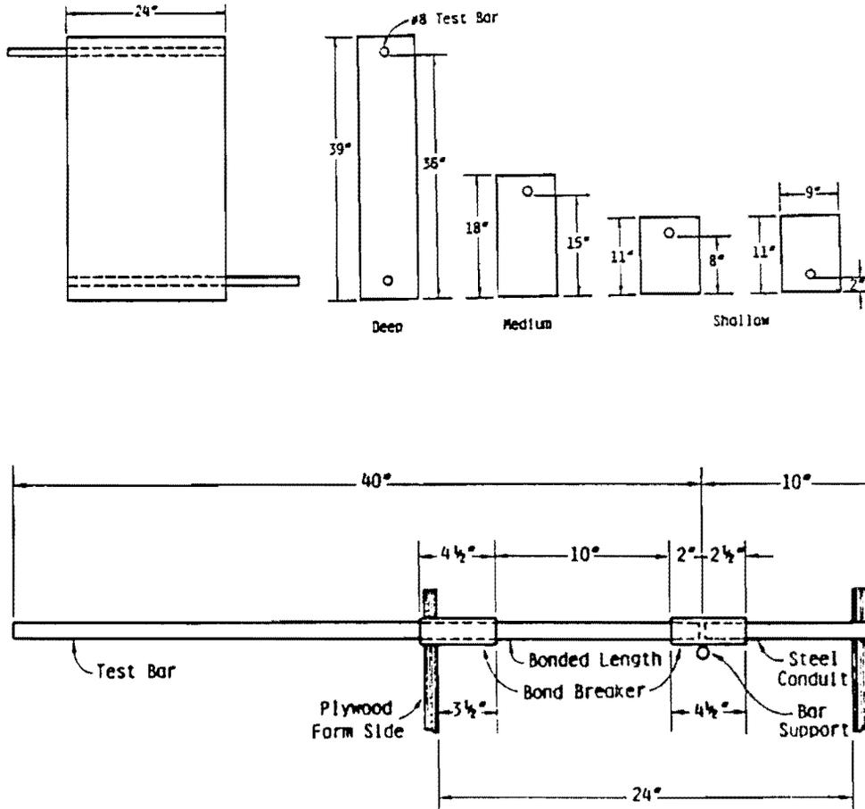
Fig. 1.12 Test specimens and test bar installation [9].
