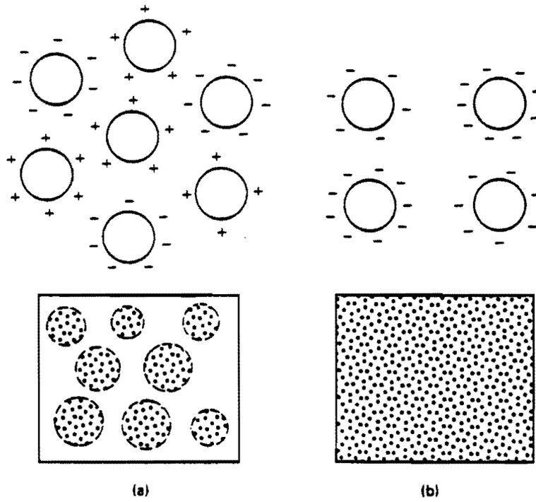
Fig. 1.7 Dispersing action of superplasticizer (schematic representation): (a) flocculated paste; (b) dispersed paste [35].
