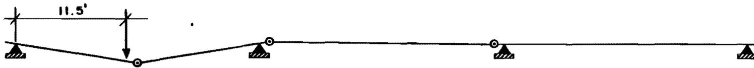
**g) Shear Test of North Span - Mechanism #2**
