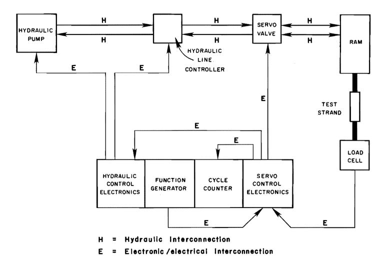
Figure 3-3: Block Diagram: Strand Test Servo Control System
