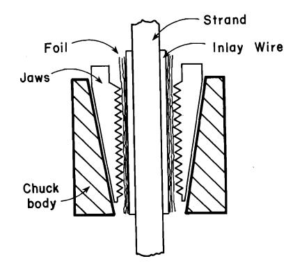
Figure 3-4: Section Through Foil-Protected Chuck
