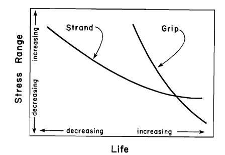
Figure 4-4: Generalized Strand and Grip Fatigue Models
