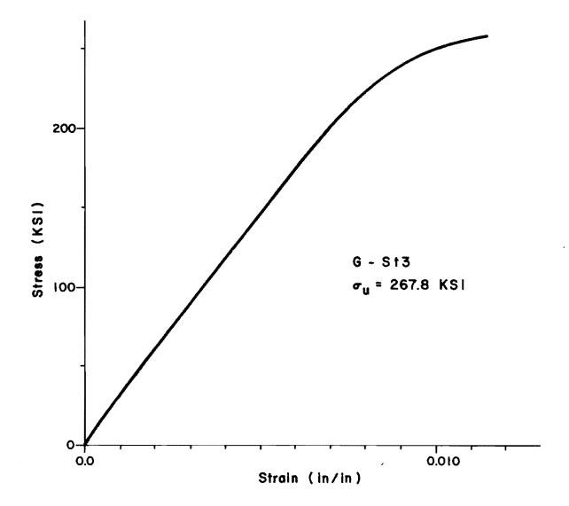
Figure C-1: Stress-Strain Curve for Specimen G-St3
