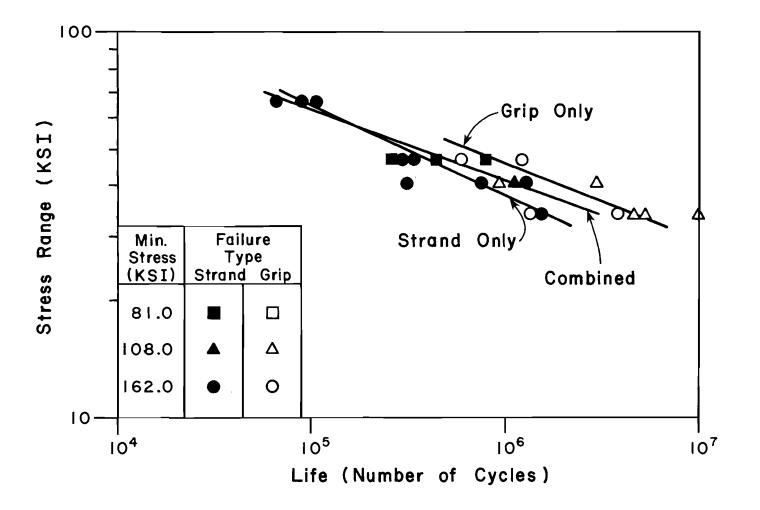
Figure 4-3: Girder Strand Failure Data
