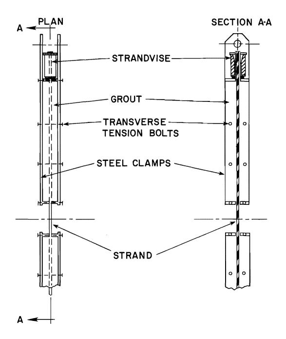
Figure 2-2: Lane and Ekberg's Grip Method (After Figure 6, Reference [21])
