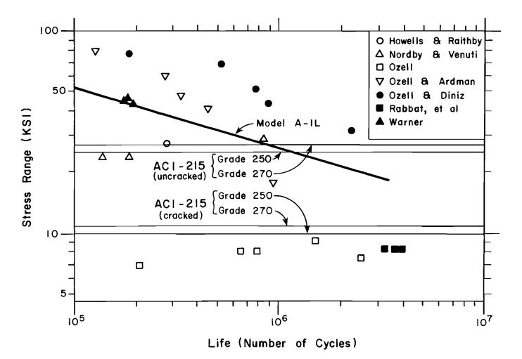
Figure 5-5: Comparison with Cracked Beam and Cracked Girder Tests
