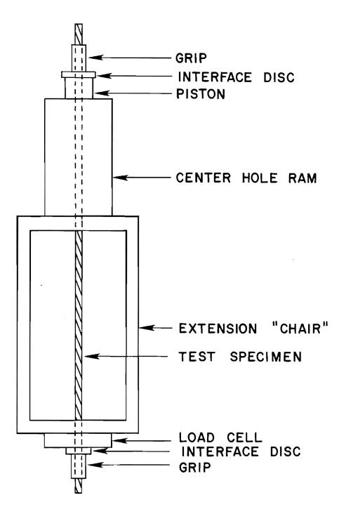
Figure 3-1: Strand Fatigue Set-Up
