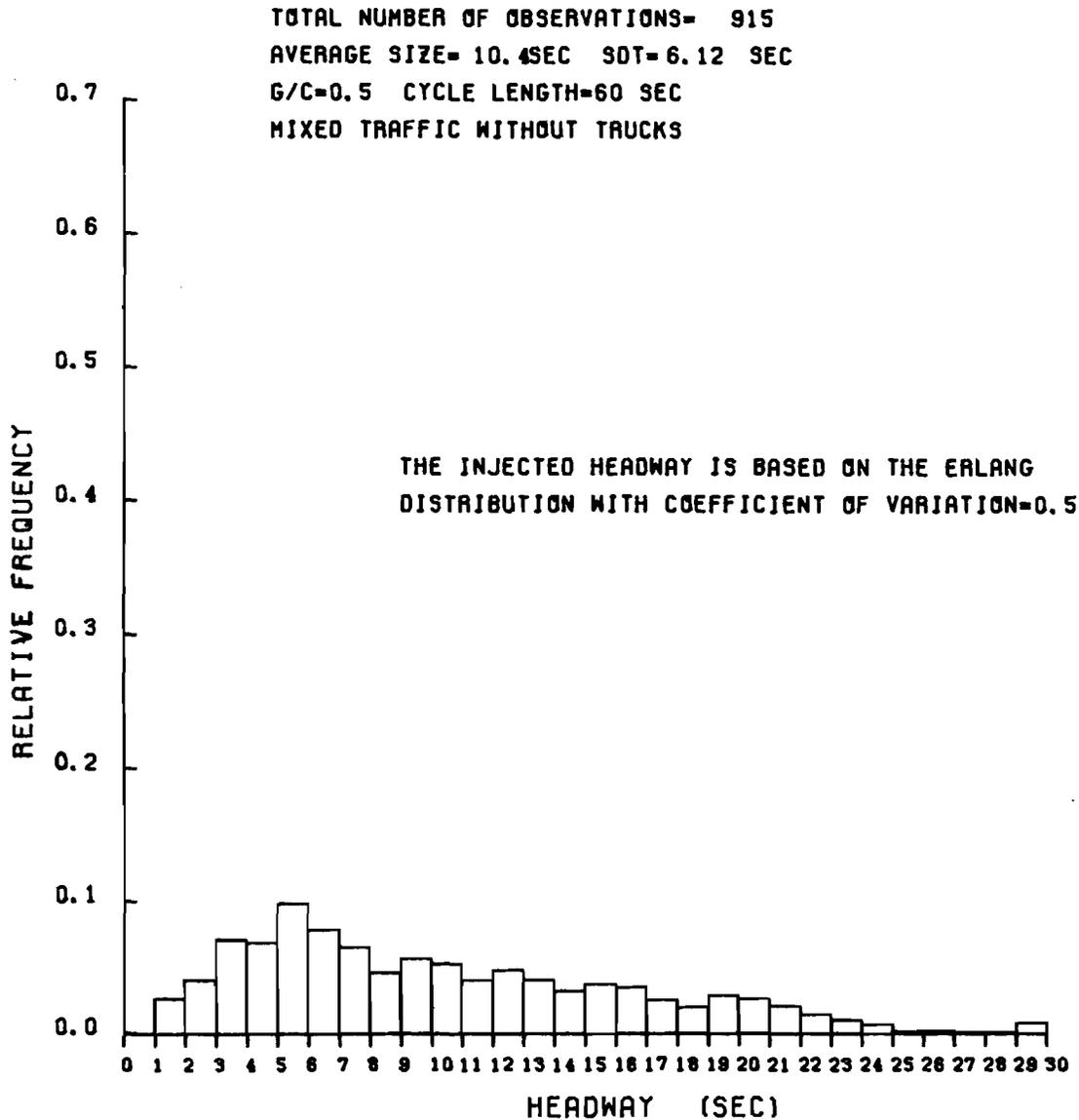
Fig 3-10. Histogram of opposing headways at the stop line after queue dissipation when the vehicles are injected at 1000 feet upstream according to an Erlang distribution with c.v. = 0.5, and mean = 18 sec.
