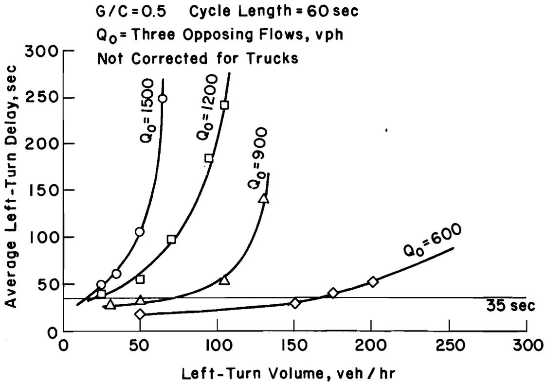
Fig 5-6. The average left-turn delay under various traffic conditions at six-by-six signalized intersections with adequate bay length.
