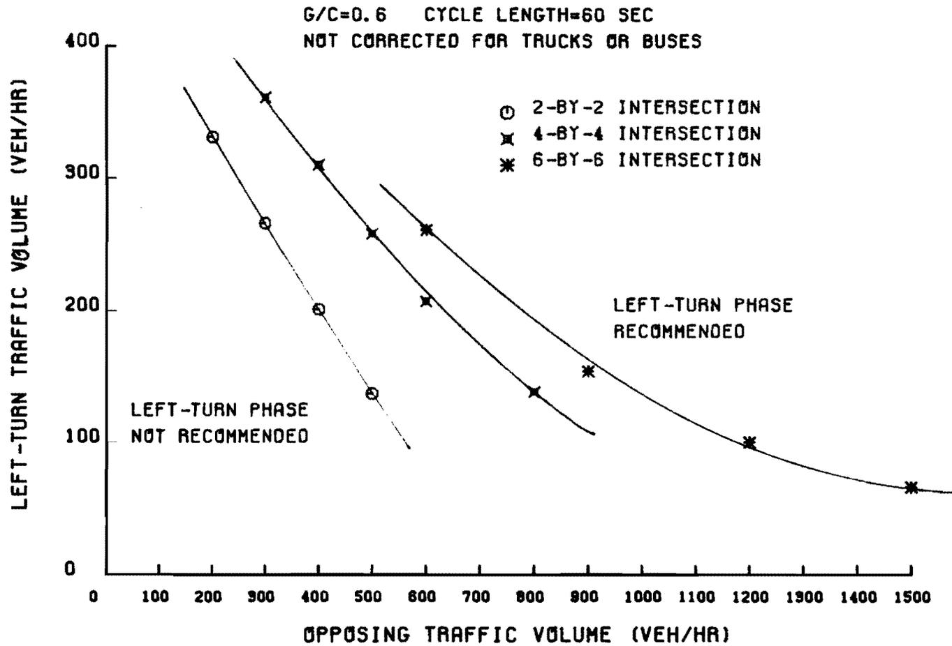
Fig 6-4. Decision chart for implementing a separate left-turn phase at signalized intersections with  $G/C = 0.6$  and  $C = 60$  sec.
