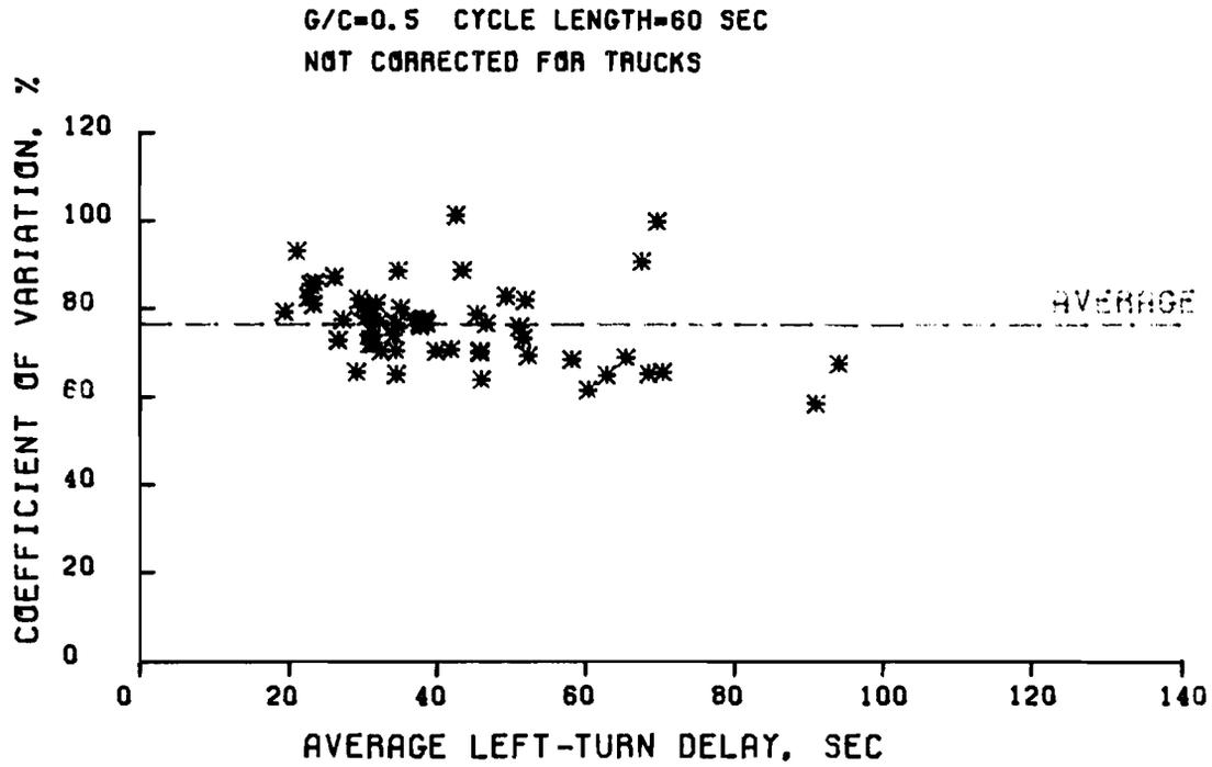
Fig 5-3. Relation between the average left-turn delay and the coefficient of variation.
