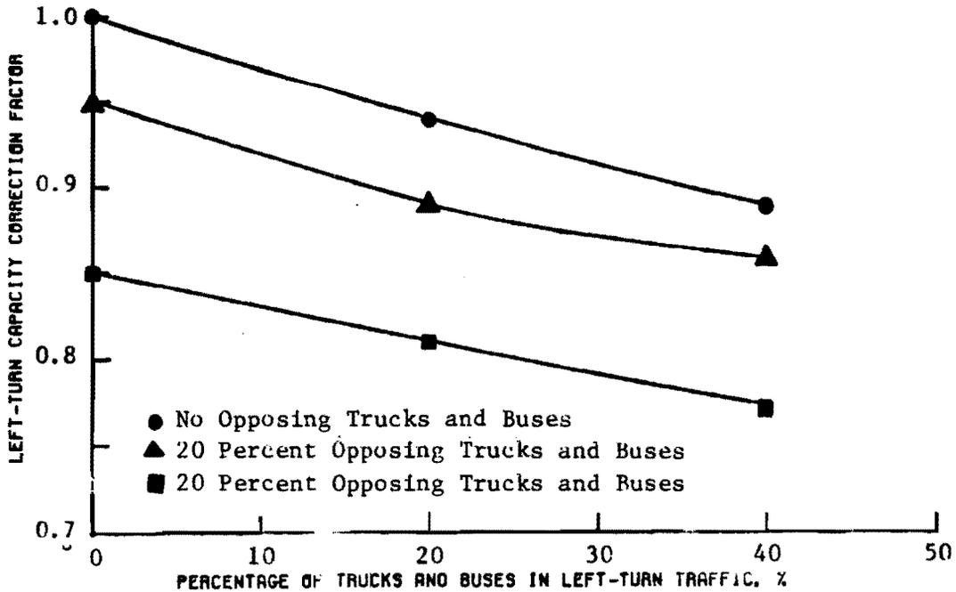
Fig 4-15. Factors for adjusting left-turn capacity for different combinations of opposing and left-turn truck percentages.
