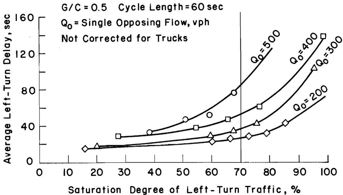
Fig 5-17. The relation between the average left-turn delay and degree of left-turn saturation at two-by-two signalized intersections.
