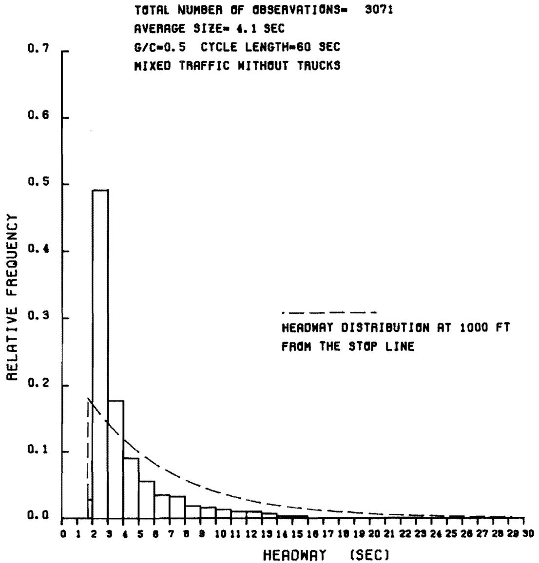
Fig 3-8. Histogram of opposing headways at the stop line after queue dissipation when the opposing volume is 500 vph.
