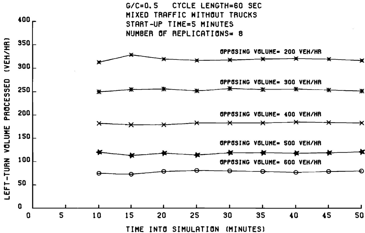
Fig 2-2. Stable behavior of left-turn flow under oversaturated conditions.
