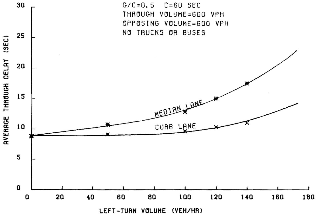
Fig 5-22. Comparison between the through delay in the median lane and that in the curb lane.
