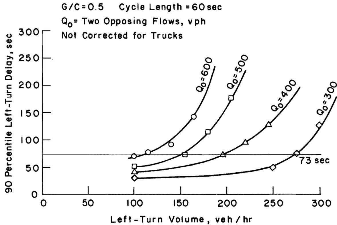
Fig 5-10. The ninety percentile left-turn delay under various traffic conditions at four-by-four signalized intersections with adequate length of bay.
