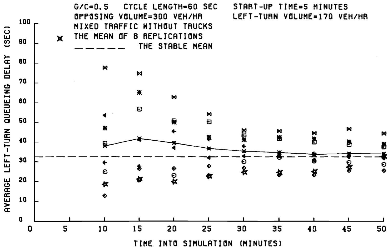
Fig 2-4. Stable behavior of the mean of the average left-turn delay over eight independent replications for opposing volume 300 vph.
