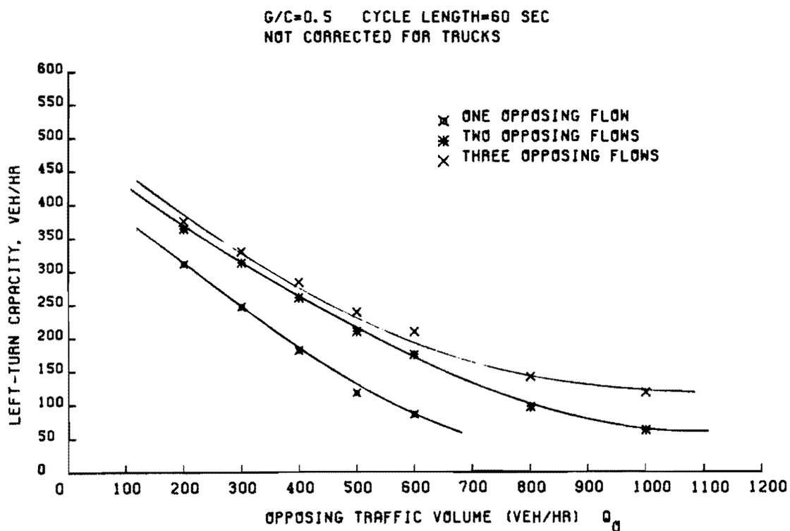
Fig 4-18. Left-turn capacity at signalized intersections having adequate length of bay for  $G/C = 0.5$  and  $C = 60$  sec.
