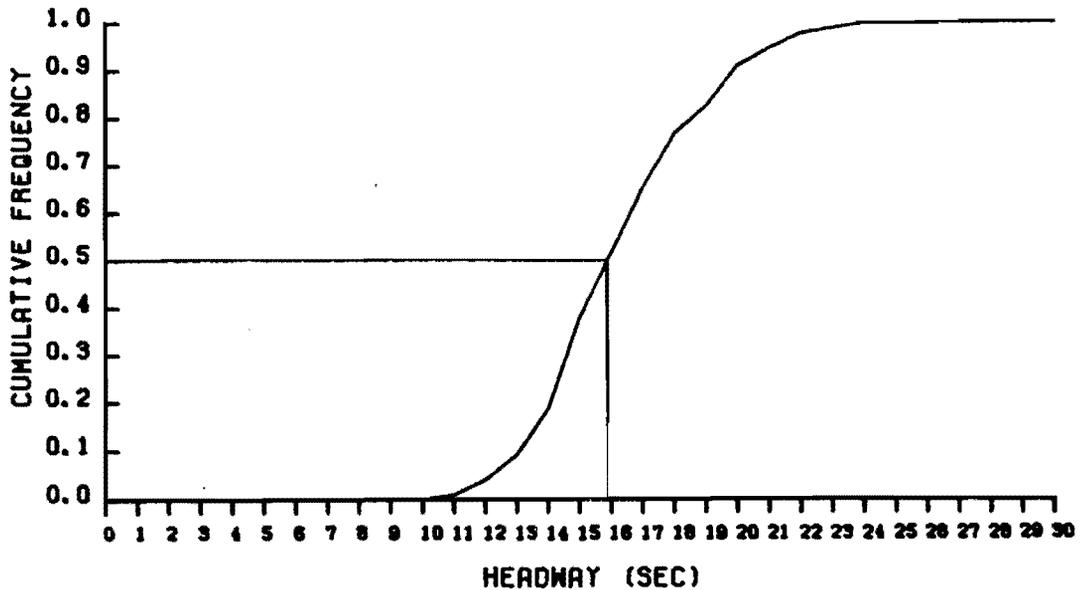
Fig 3-22. Histogram and cumulative frequency of headways in opposing traffic for accommodating four left-turns.
