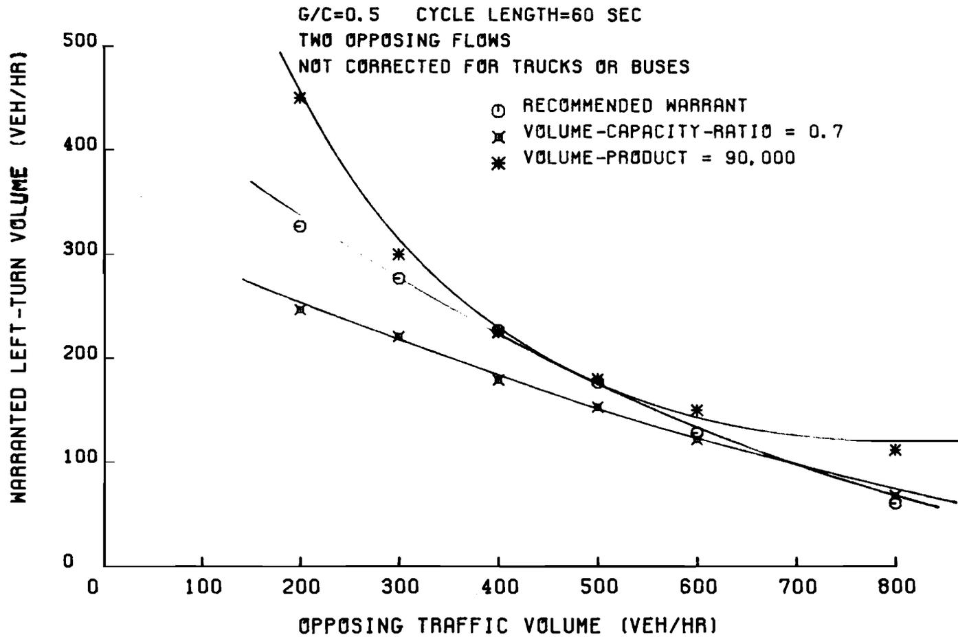
Fig 6-6. Comparisons among different warrants for a separate left-turn phase at four-by-four signalized intersections.
