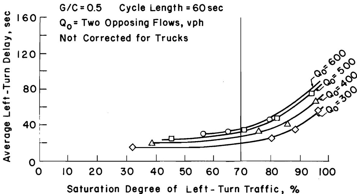
Fig 5-18. The relation between the average left-turn delay and degree of left-turn saturation at four-by-four signalized intersections.
