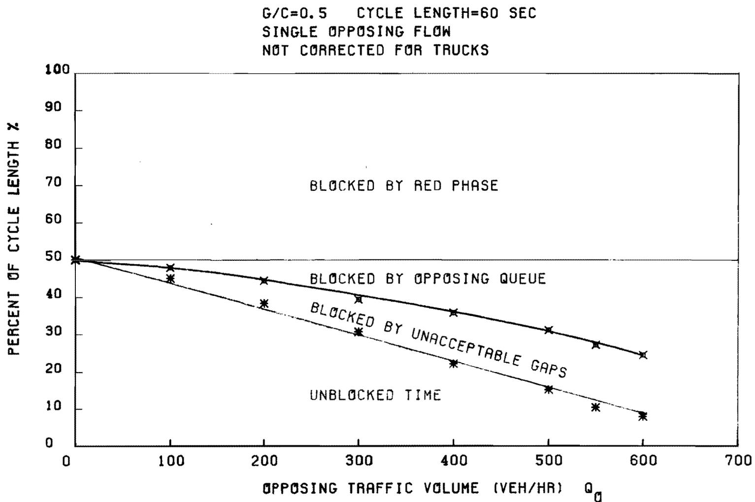
Fig 4-4. The blocked and unblocked durations for left-turning movements under different levels of opposing volume.
