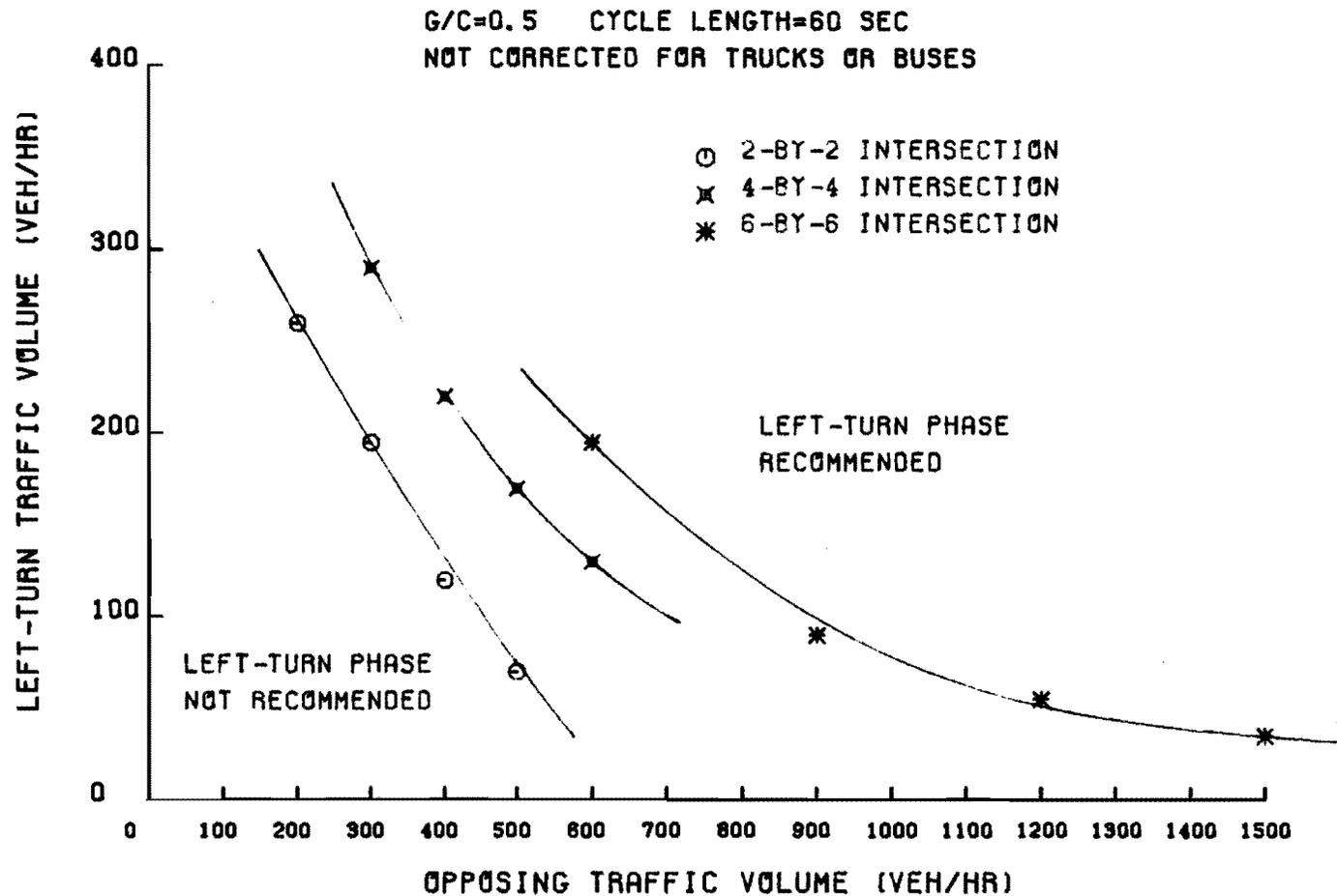
Fig 6-3. Decision chart for implementing a separate left-turn phase at signalized intersections with  $G/C = 0.5$  and  $C = 60$  sec.
