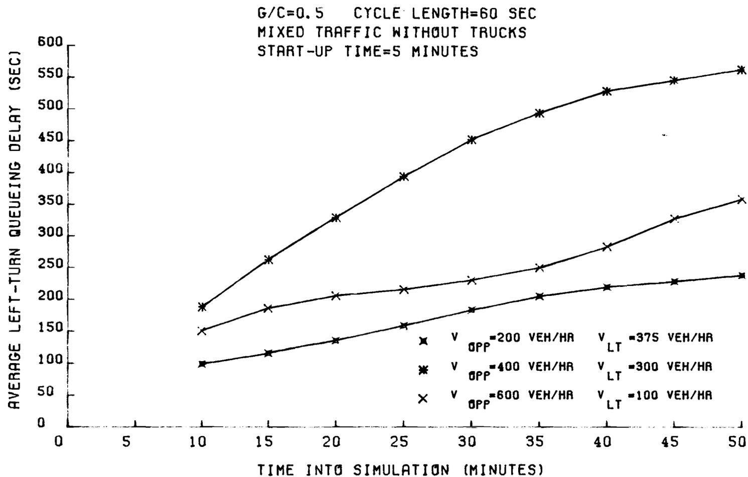
Fig 2-1. Unstable behavior of average left-turn delay statistics under oversaturated conditions.
