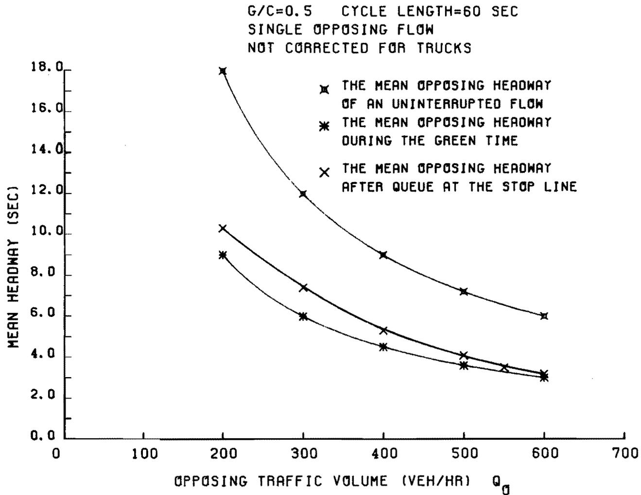
Fig 4-3. The comparison between the average headway of an uninterrupted flow and that of an interrupted flow at signalized intersections with  $G/C = 0.5$ , and  $C = 60$  sec.
