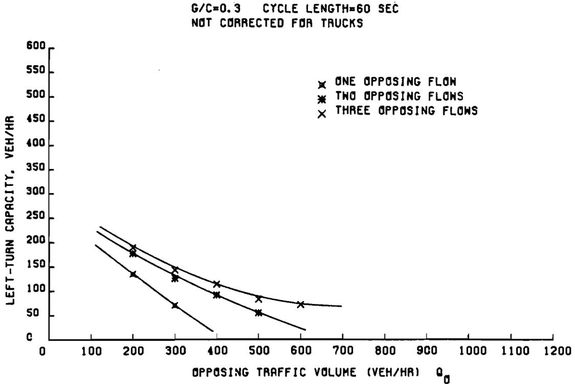
Fig 4-16. Left-turn capacity at signalized intersections having adequate length of bay for  $G/C = 0.3$  and  $C = 60$  sec.
