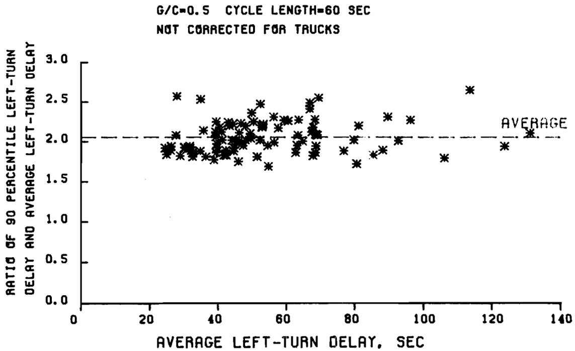
Fig 5-8. The relation between the average and 90 percentile values of left-turn delay.
