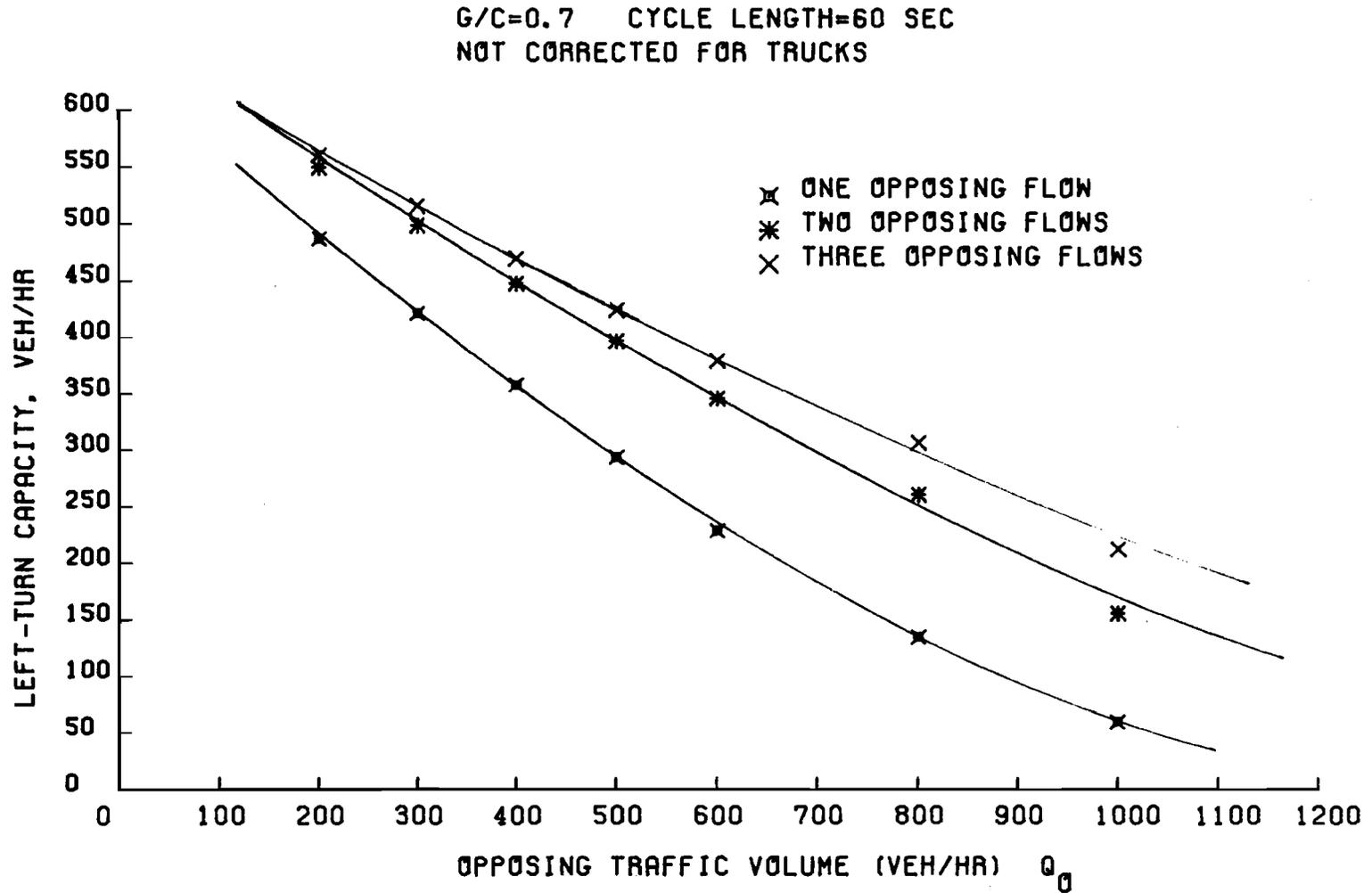
Fig 4-20. Left-turn capacity at signalized intersections having adequate length of bay for  $G/C = 0.7$  and  $C = 60$  sec.
