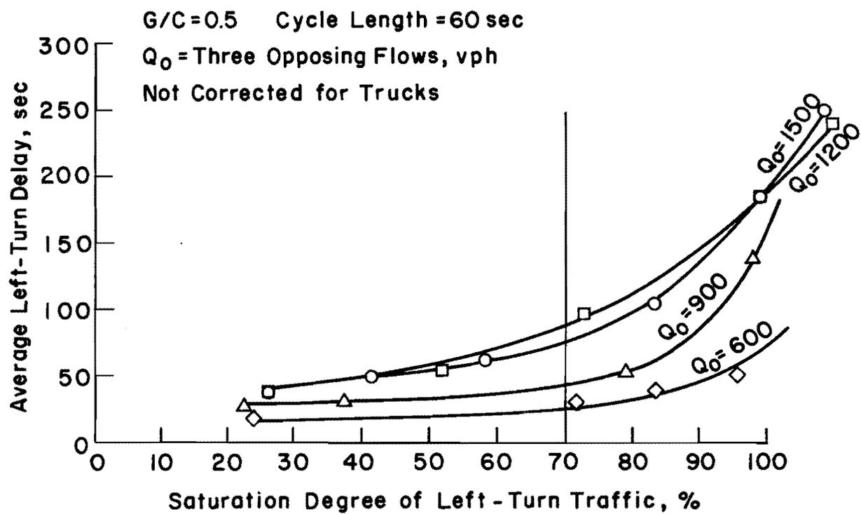
Fig 5-19. The relation between the average left-turn delay and degree of left-turn saturation at six-by-six signalized intersections.
