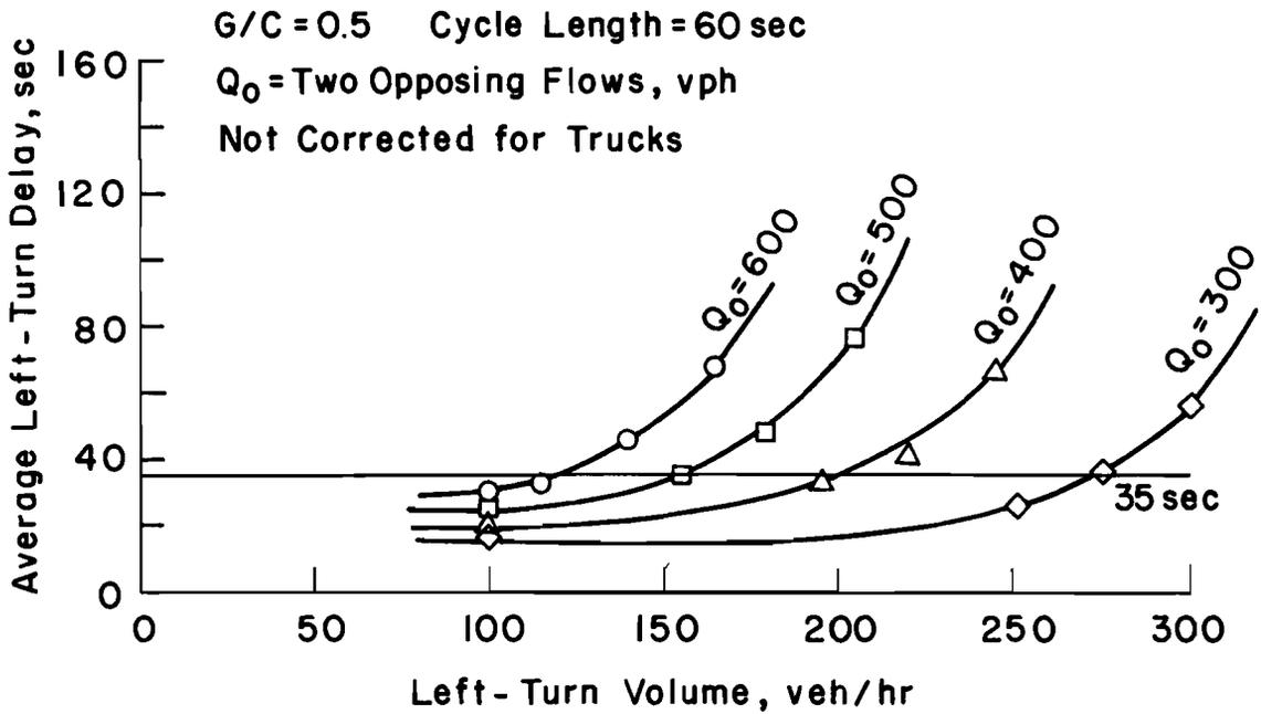
Fig 5-5. The average left-turn delay under various traffic conditions at four-by-four signalized intersections with adequate bay length.
