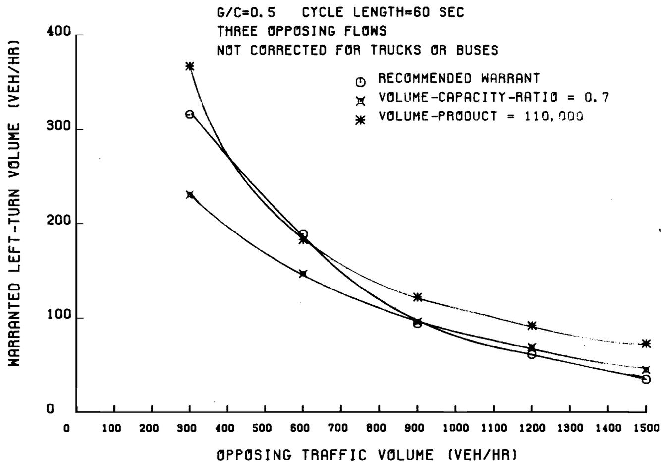
Fig 6-7. Comparisons among different warrants for a separate left-turn phase at six-by-six signalized intersections.
