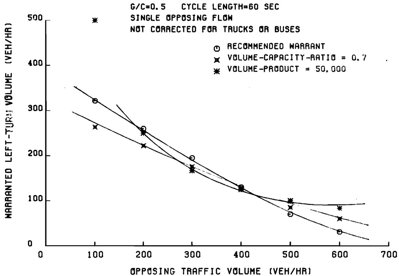
Fig 6-5. Comparisons among different warrants for a separate left-turn phase at two-by-two signalized intersections.
