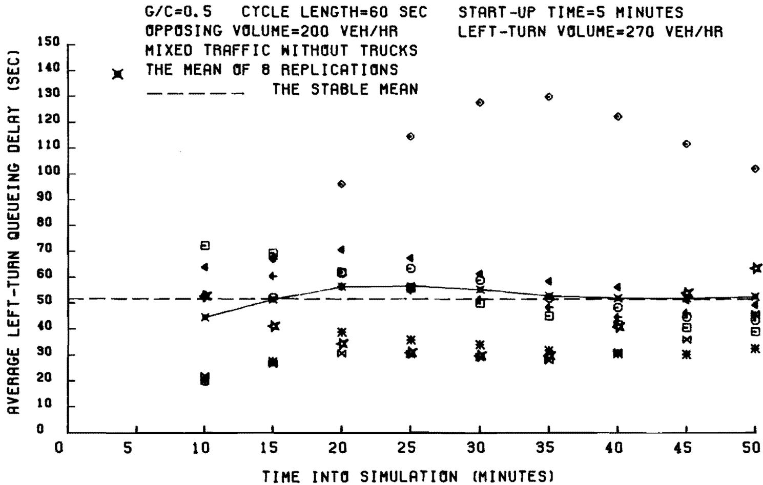
Fig 2-3. Stable behavior of the mean of the average left-turn delay over eight independent replications for opposing volume 200 vph.
