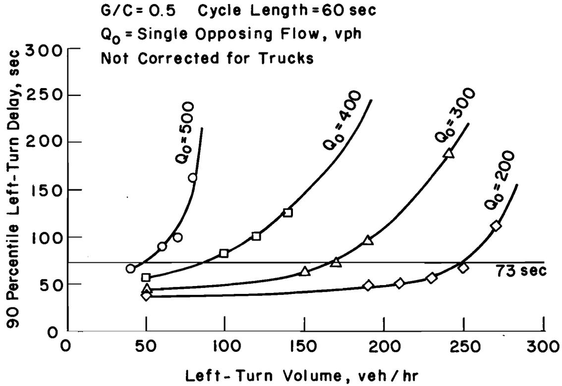
Fig 5-9. The ninety percentile left-turn delay under various traffic conditions at two-by-two signalized intersections with adequate length of bay.
