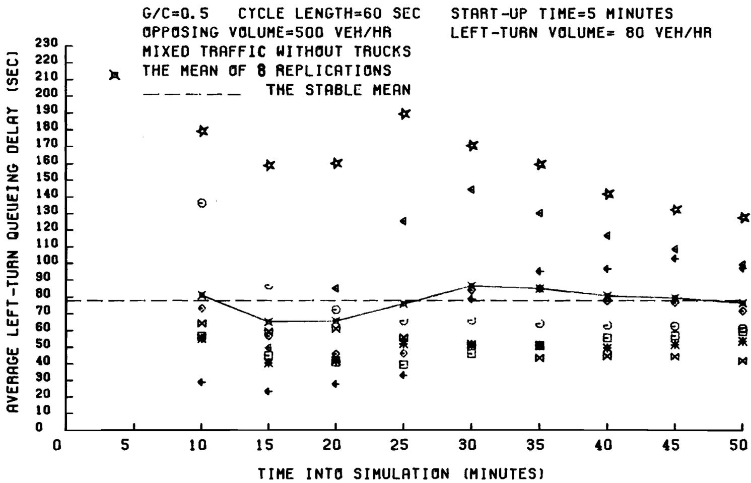
Fig 2-6. Stable behavior of the mean of the average left-turn delay over eight independent replications for opposing volume 500 vph.
