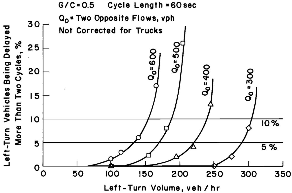
Fig 5-13. The percentage of left turners being delayed more than two cycles under various traffic conditions at four-by-four signalized intersections with adequate length of bay.
