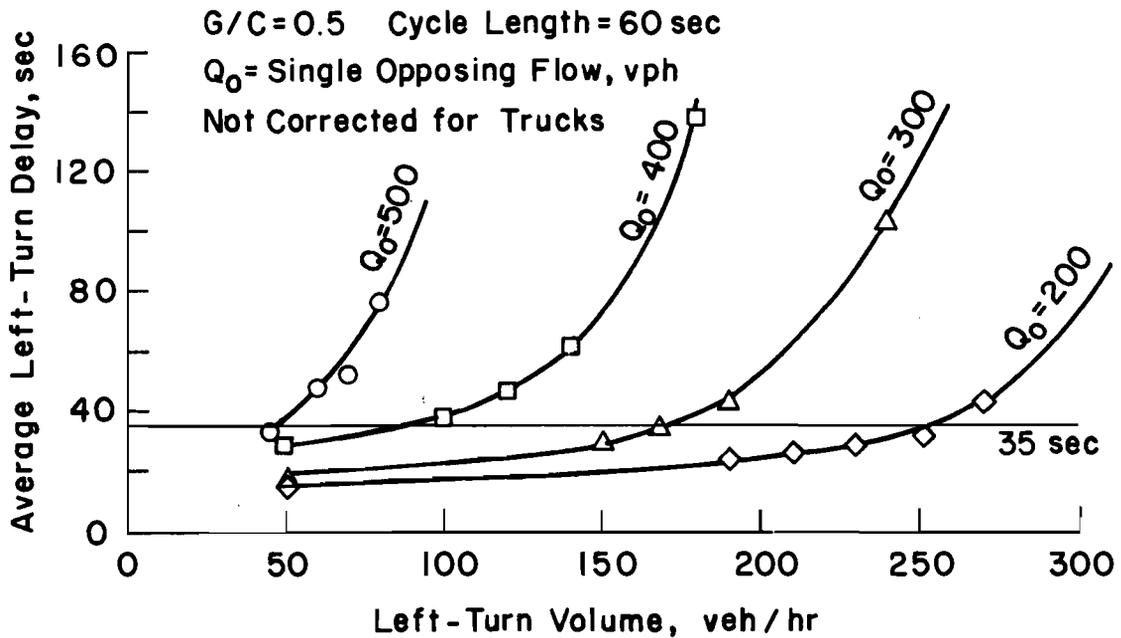
Fig 5-4. The average left-turn delay under various traffic conditions at two-by-two signalized intersections with adequate bay length.
