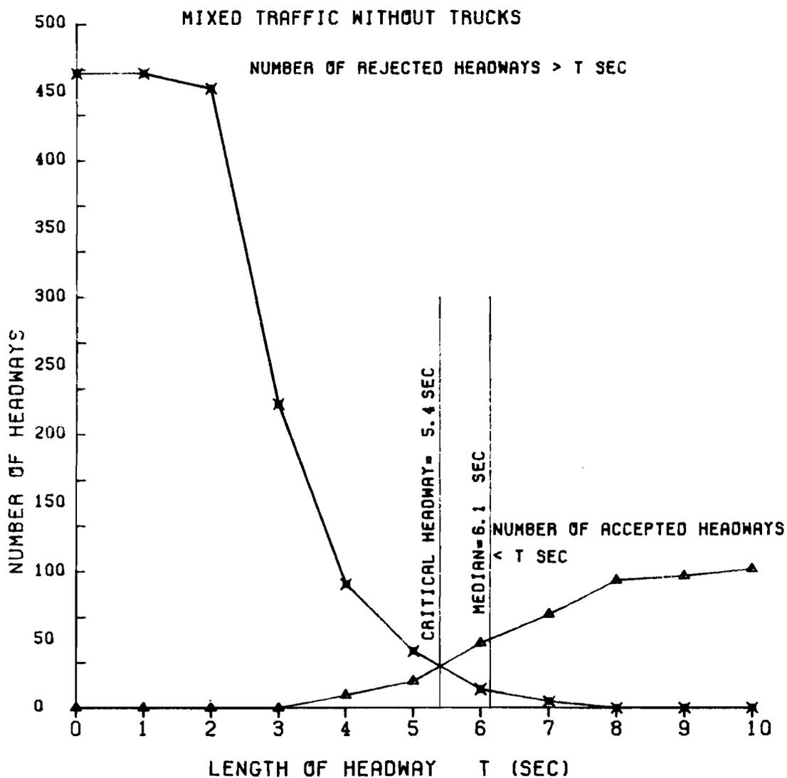
Fig 3-17. The critical headway and the median headway in opposing traffic obtained from the TEXAS Model.
