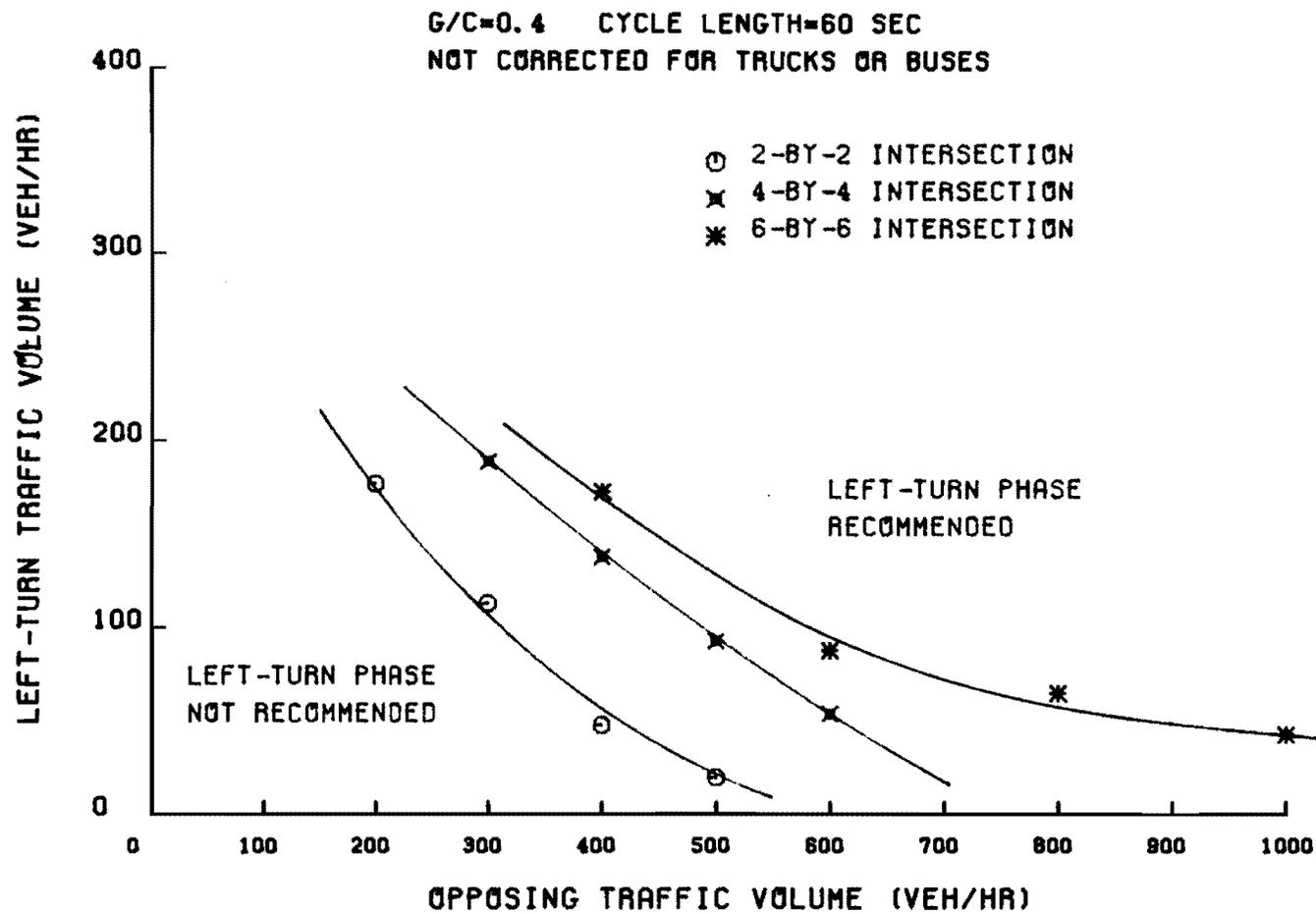
Fig 6-2. Decision chart for implementing a separate left-turn phase at signalized intersections with  $G/C = 0.4$  and  $C = 60$  sec.
