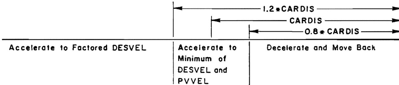
(a) Leading driver-vehicle unit is going faster than the following driver-vehicle unit.
