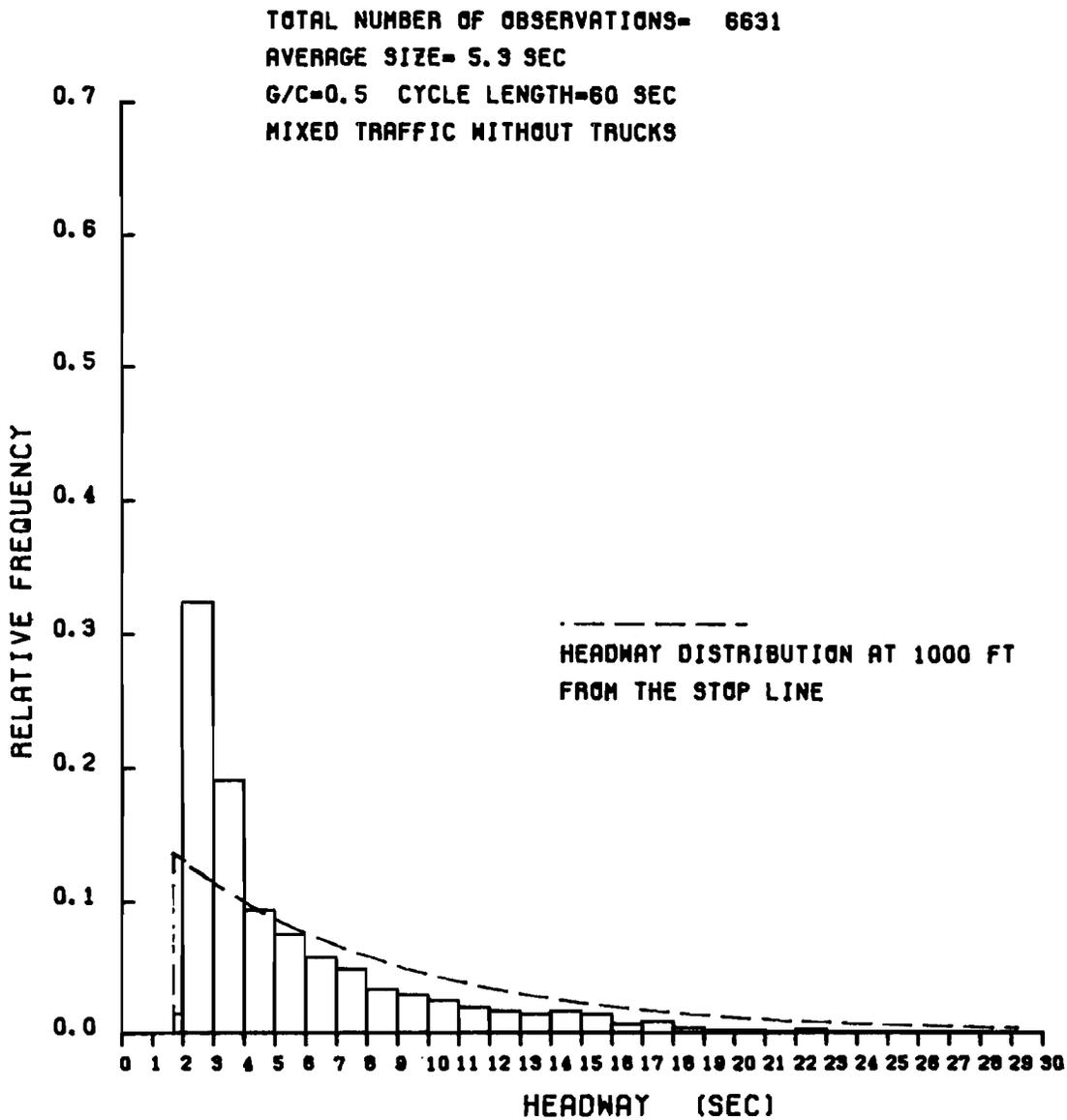
Fig 3-7. Histogram of the opposing headways at the stop line after queue dissipation when the opposing volume is 400 vph.
