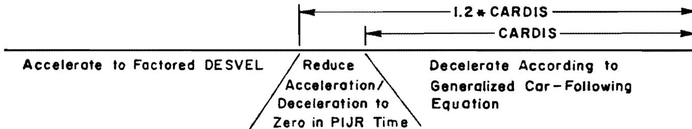
(b) Following driver-vehicle unit is going faster than the leading driver-vehicle unit.
