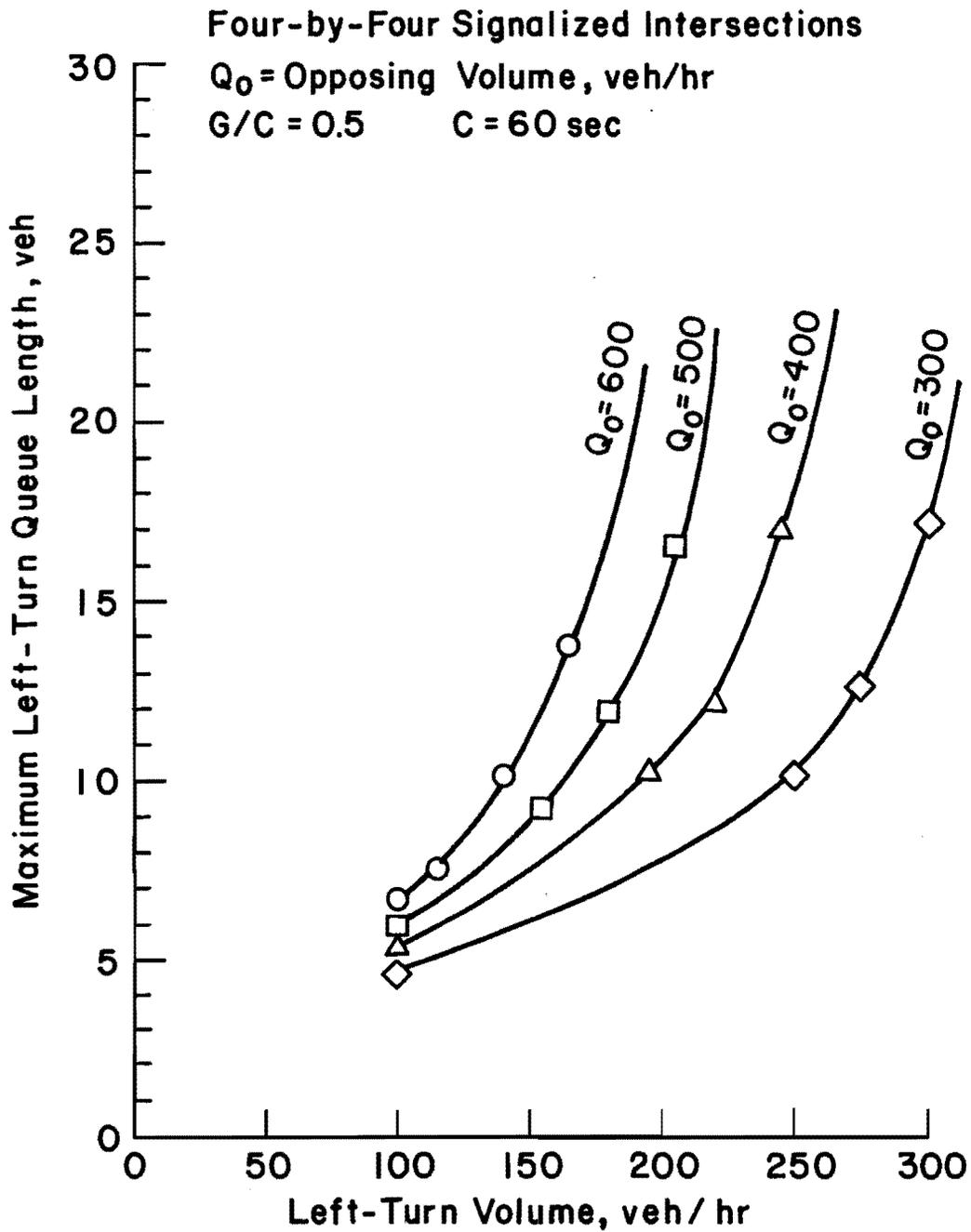
Fig 6-9. The maximum number of left-turn vehicles stored in the bay under various traffic conditions at four-by-four signalized intersections.
