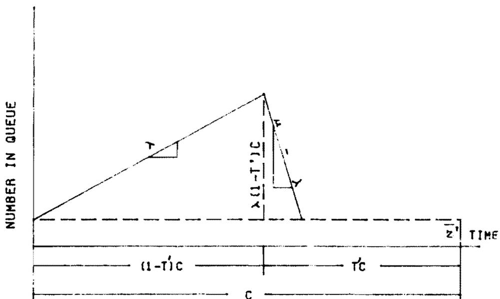
Fig 5-21. The change in queue diagram when the cycle split is increased.
