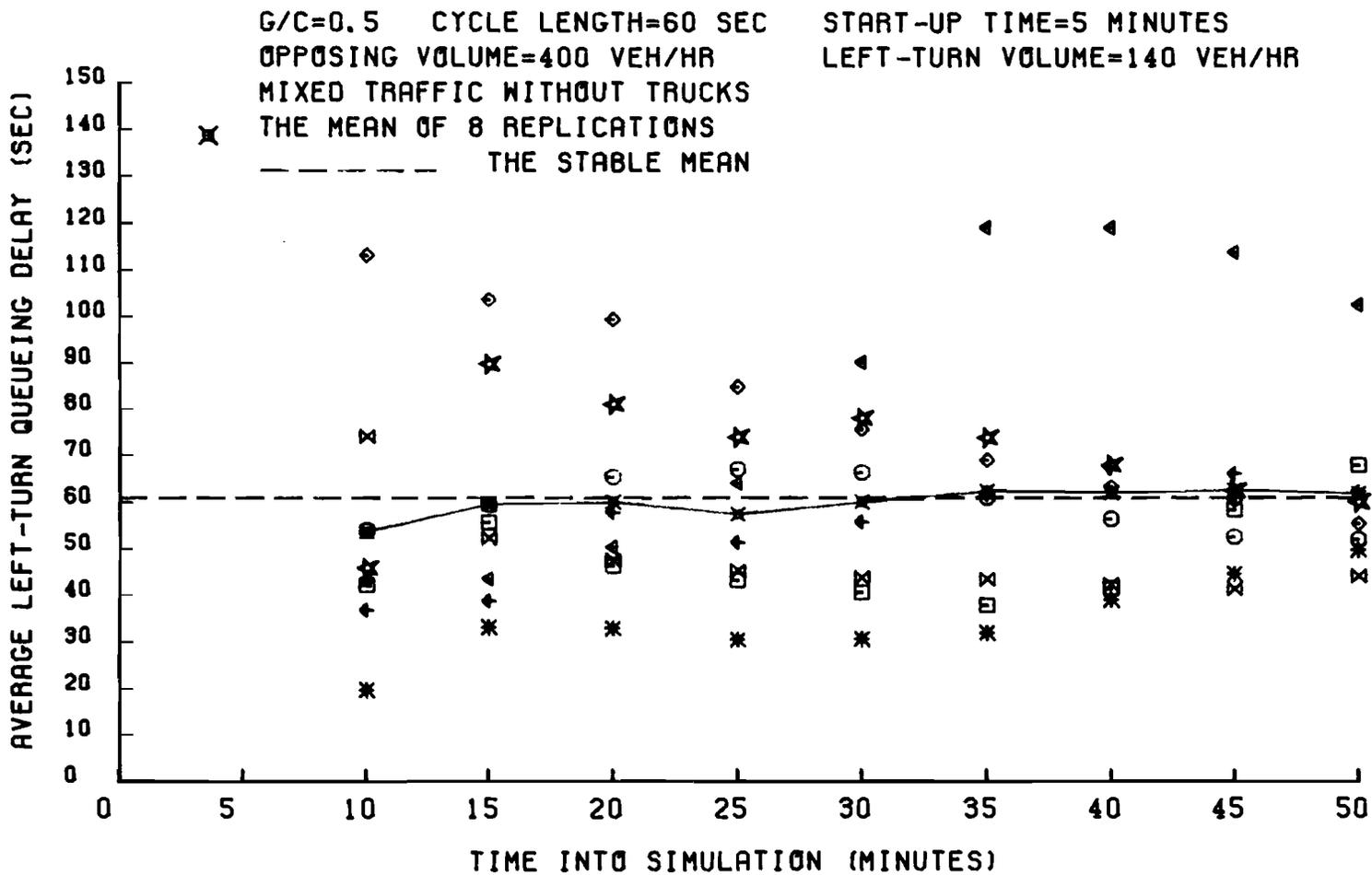
Fig 2-5. Stable behavior of the mean of the average left-turn delay over eight independent replications for opposing volume 400 vph.
