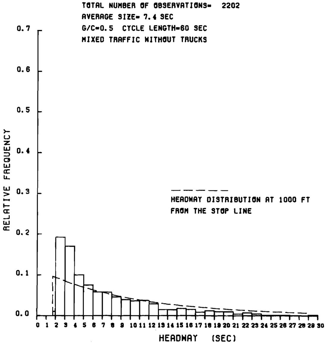
Fig 3-6. Histogram of the opposing headways at the stop line after queue dissipation when the opposing volume is 300 vph.
