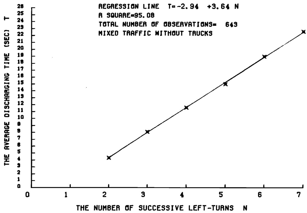
Fig 3-16. The average time required for completing N successive left turns.
