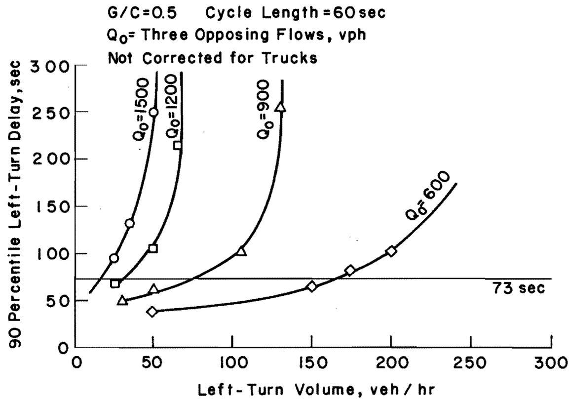
Fig 5-11. The ninety percentile left-turn delay under various traffic conditions at six-by-six signalized intersections with adequate length of bay.
