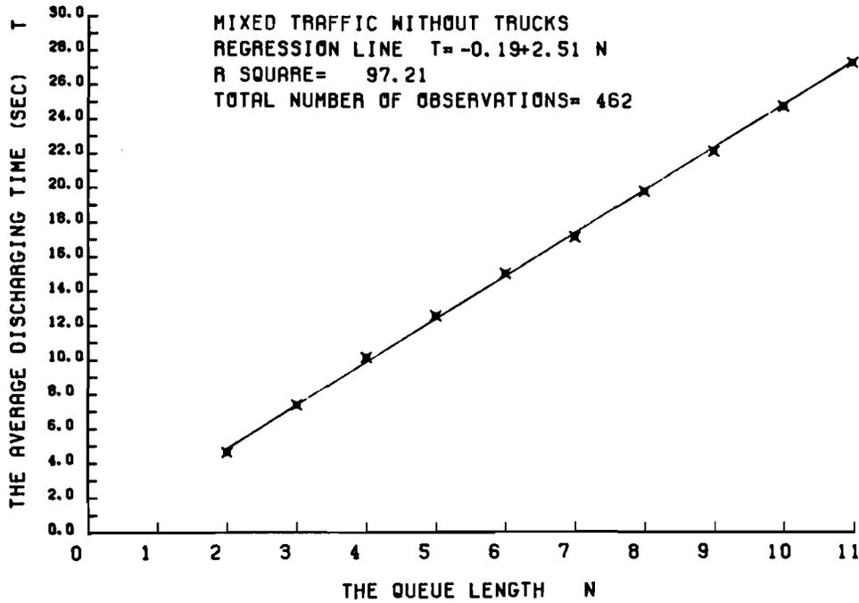
Fig 3-14. The average discharging headway at signalized intersection.
