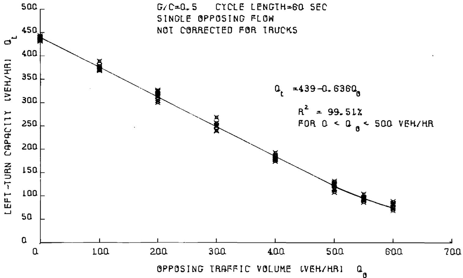
Fig 4-9. The left turn capacity under different levels of opposing volume for a simple case of left-turn movements.
