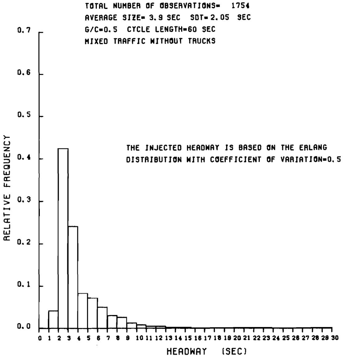
Fig 3-13. Histogram of opposing headways at the stop line after queue dissipation when the vehicles are injected at 1000 feet upstream according to an Erlang distribution with c.v. = 0.5, and mean = 7.2 sec.
