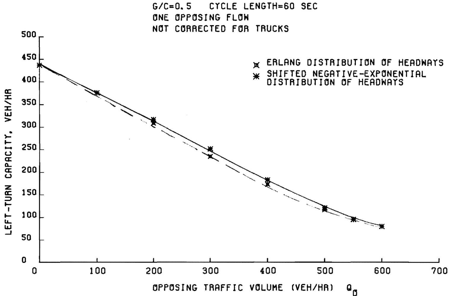
Fig 4-13. The effect of the type of headway distribution on left-turn capacity.
