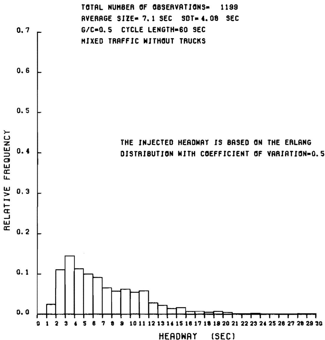
Fig 3-11. Histogram of opposing headways at the stop line after queue dissipation when the vehicles are injected at 1000 feet upstream according to an Erlang distribution with c.v. = 0.5, and mean = 12 sec.
