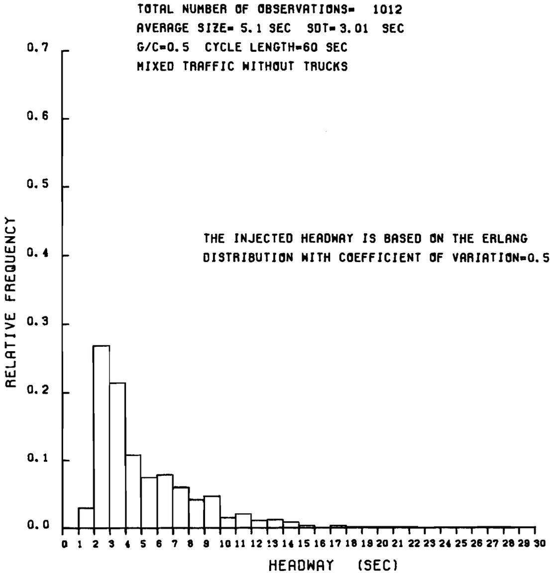
Fig 3-12. Histogram of opposing headways at the stop line after queue dissipation when the vehicles are injected at 1000 feet upstream according to an Erlang distribution with c.v. = 0.5, and mean = 7.2 sec.
