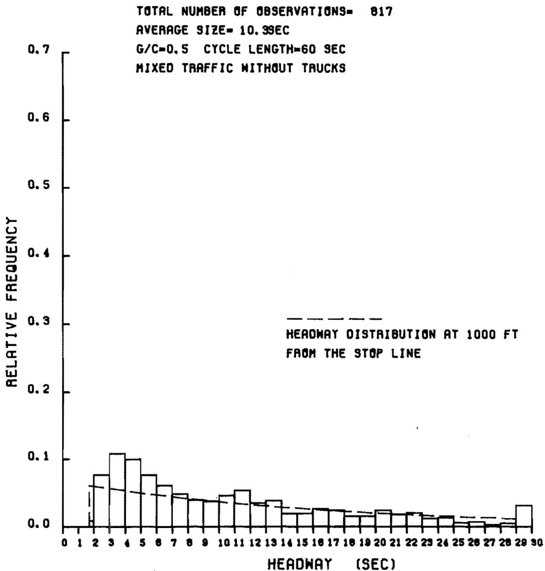
Fig 3-5. Histogram of the opposing headways at the stop line after queue dissipation when the opposing volume is 200 vph.
