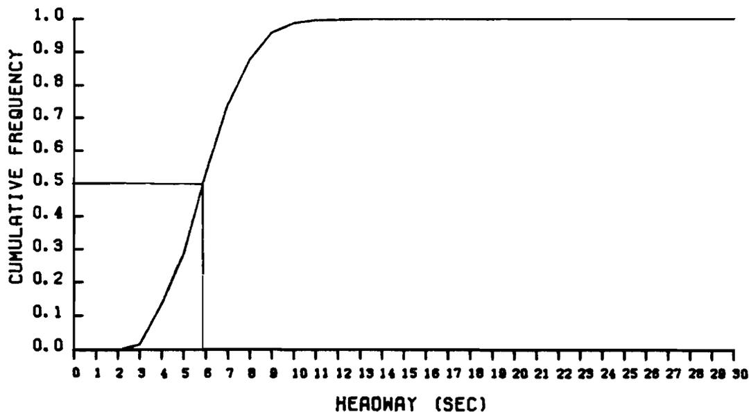
Fig 3-18. Histogram and cumulative frequency of headways which allowed no left turns.
