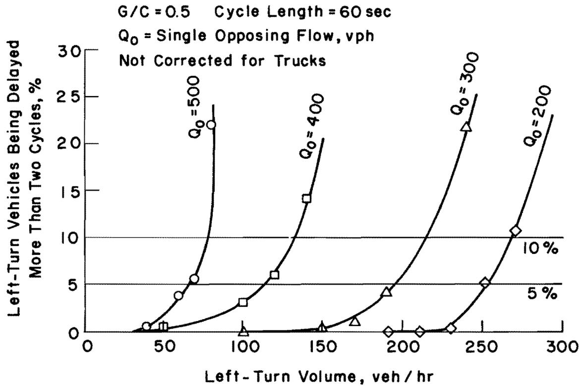
Fig 5-12. The percentage of left turners being delayed more than two cycles under various traffic conditions at two-by-two signalized intersections with adequate length of bay.
