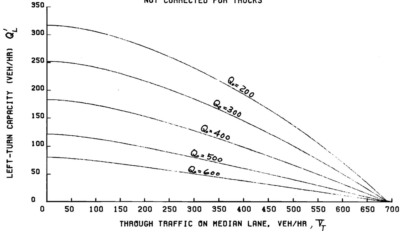
Fig 4-12. The left-turn capacity under different levels of opposing volume at two-by-two signalized intersection without a bay.
