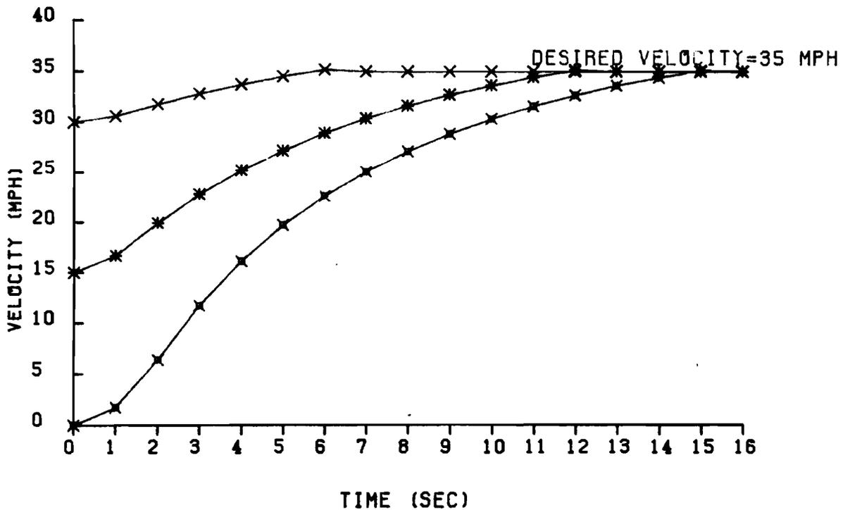
Fig 3-3. Accelerating behavior under different levels of initial velocity in reaching a desired velocity of 35 mph.
