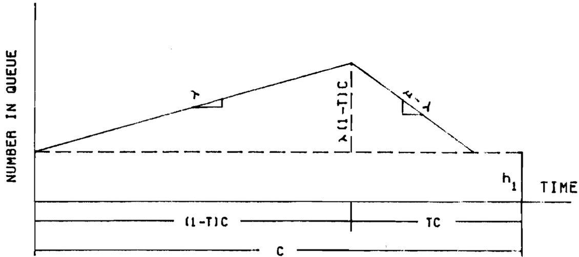
Fig 5-7. The queue diagram of left-turn operations.
