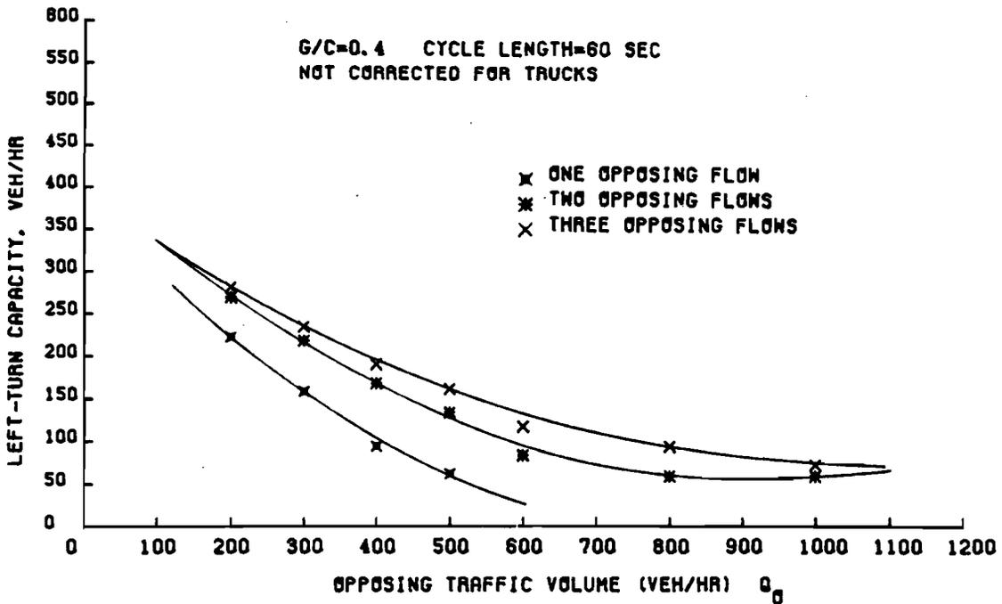
Fig 4-17. Left-turn capacity at signalized intersections having adequate length of bay for  $G/C = 0.4$  and  $C = 60$  sec.
