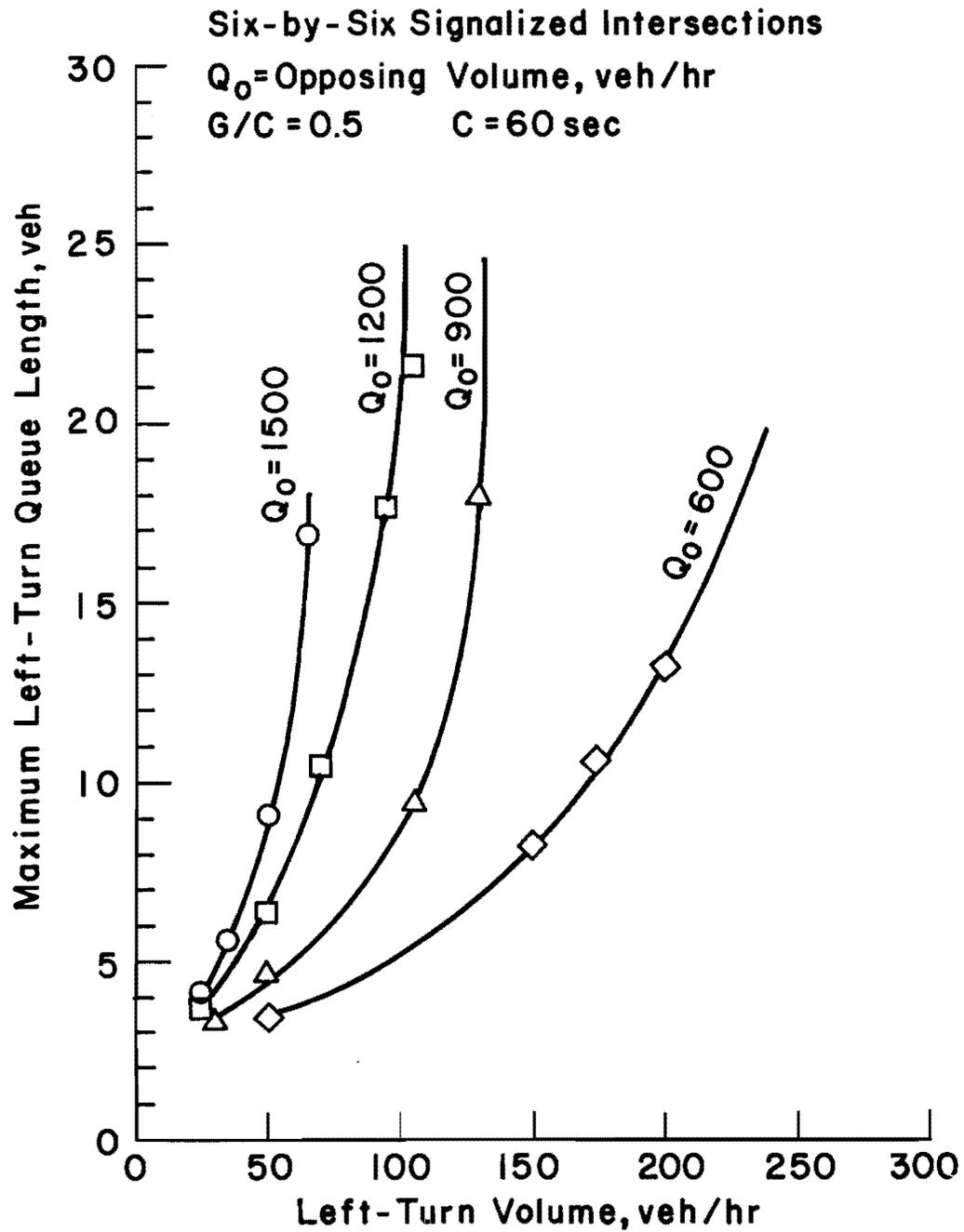
Fig 6-10. The maximum number of left-turn vehicles stored in the bay under various traffic conditions at six-by-six signalized intersections.
