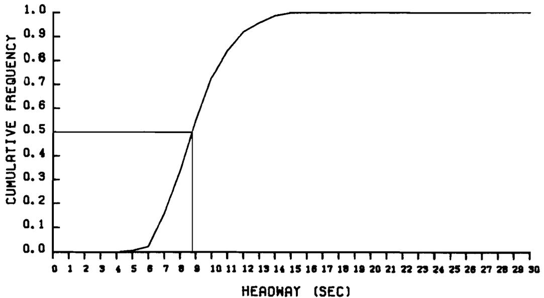
Fig 3-20. Histogram and cumulative frequency of headways in opposing traffic for accommodating two left-turns.
