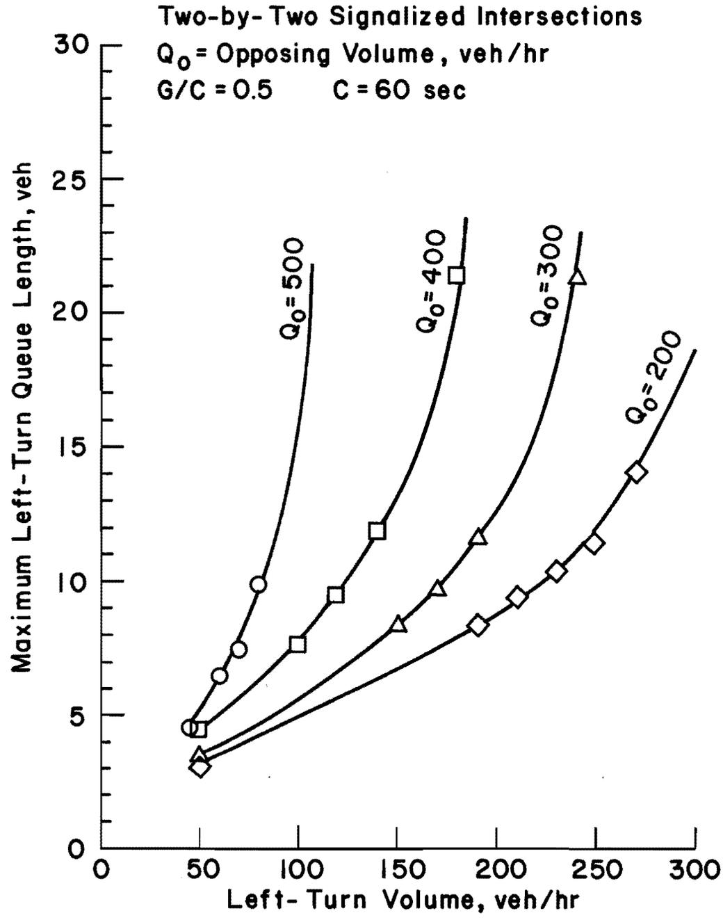
Fig 6-8. The maximum number of left-turn vehicles stored in the bay under various traffic conditions at two-by-two signalized intersections.
