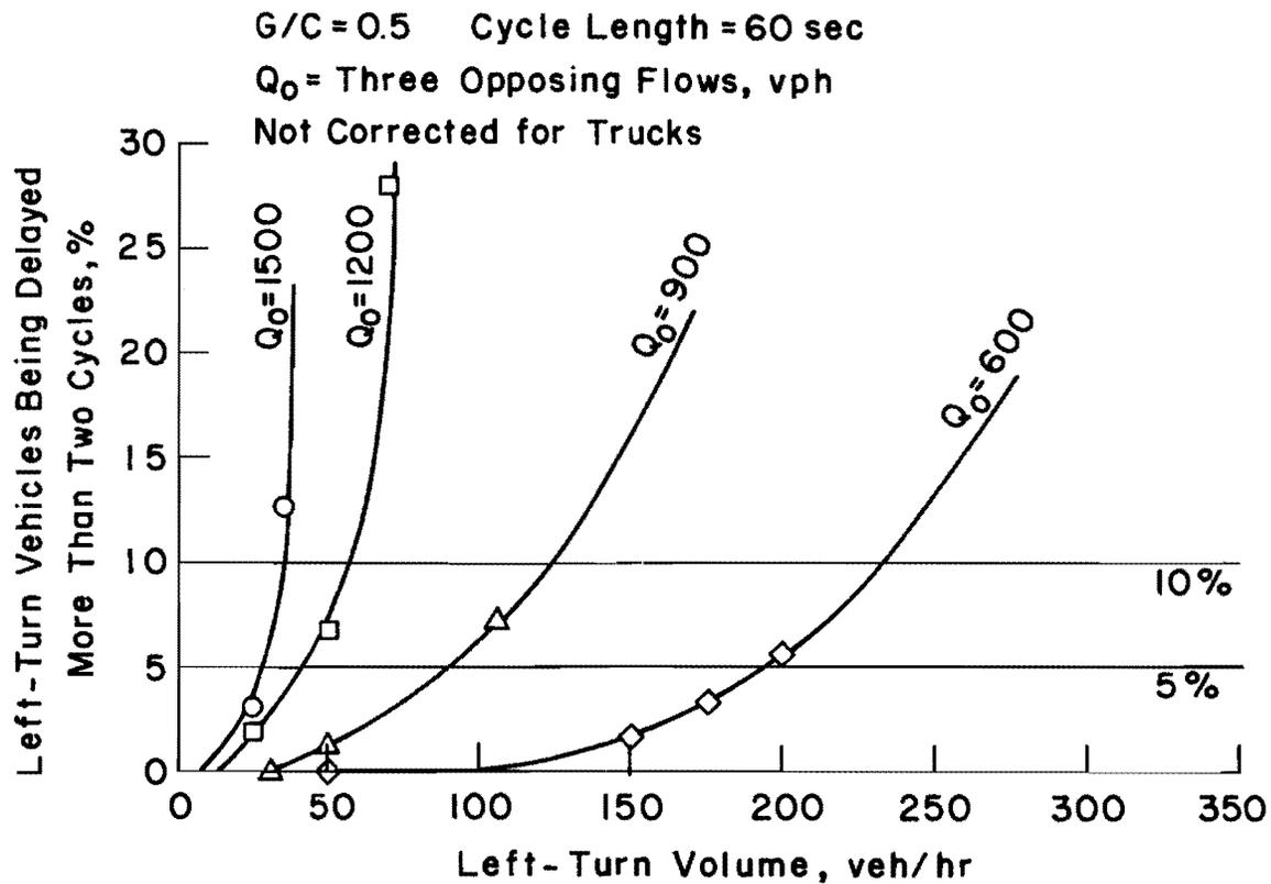
Fig 5-14. The percentage of left turners being delayed more than two cycles under various traffic conditions at six-by-six signalized intersections with adequate length of bay.
