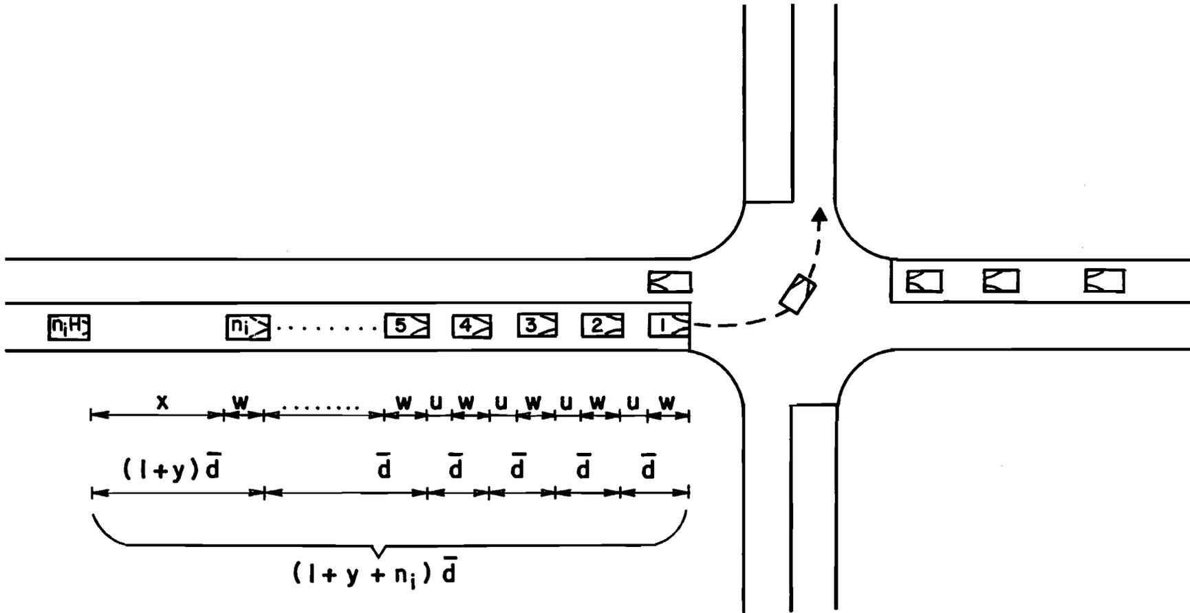
Fig 5-16. The queuing delay for the left-turner joining a queue.
