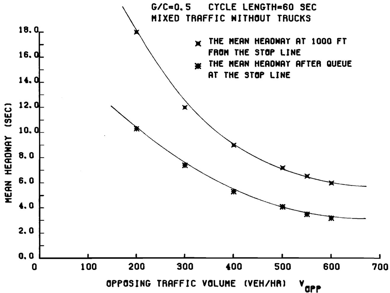
Fig 3-9. Comparison between the average opposing headway at the stop line and at 1000 feet upstream.
