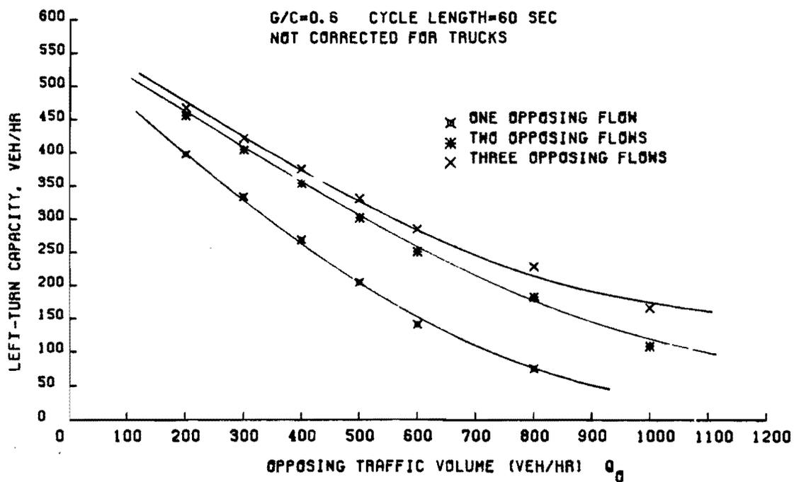
Fig 4-19. Left-turn capacity at signalized intersections having adequate length of bay for  $G/C = 0.6$  and  $C = 60$  sec.
