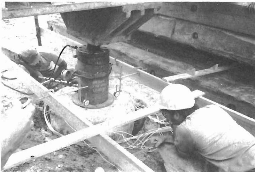
Fig. 3.2 Photographs of Instrumentation at Top of Shaft
