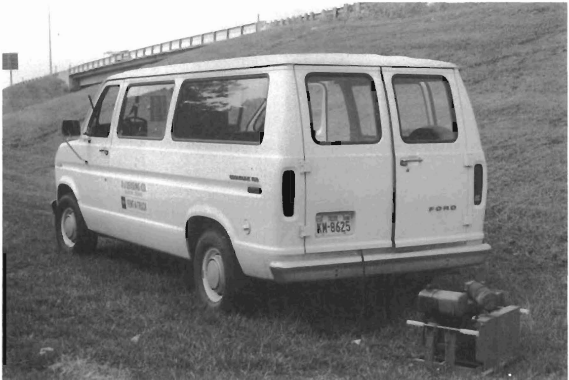
Fig. 1.10 Instrumentation van and gasoline generator
