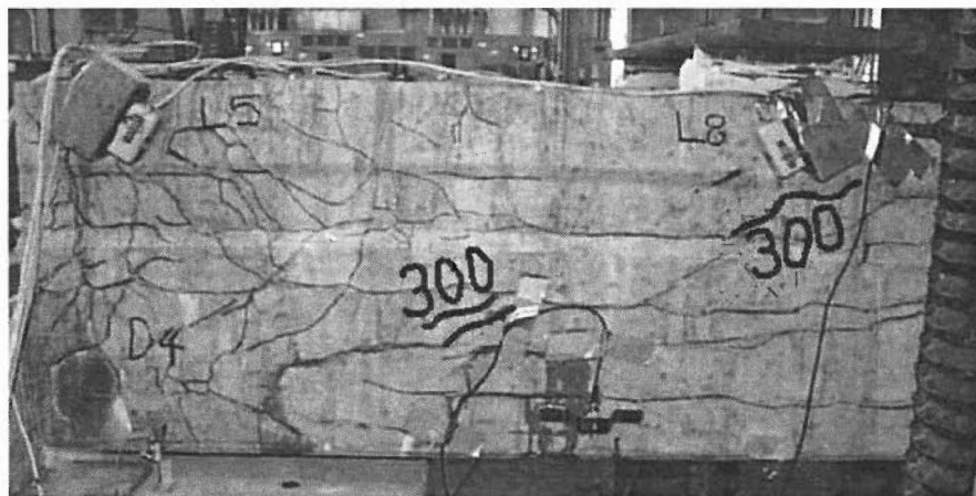
Figure 4.41 Shear-induced cracks on the east face of BG4S under a load of 300 kips (1330 kN)
