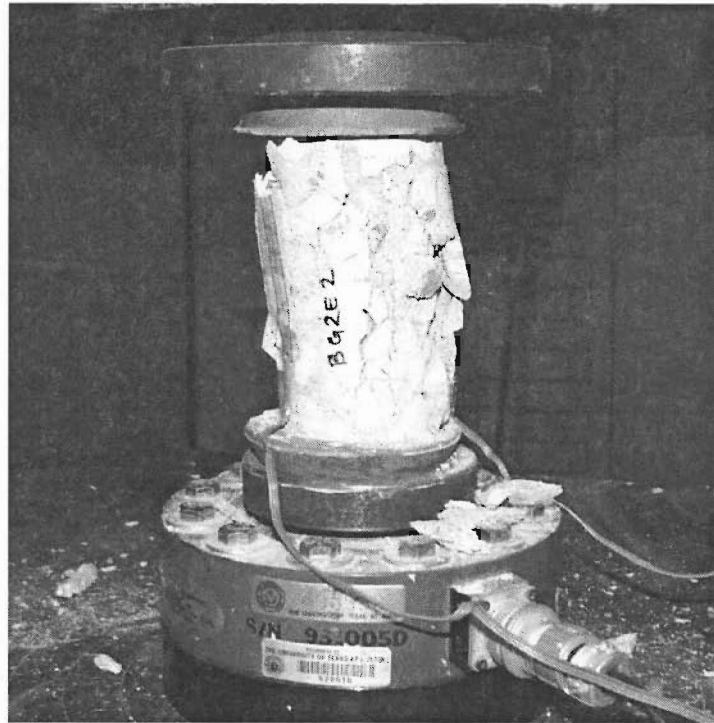
Figure 4.51 Failure of BG2E-2, typical of more-damaged cores
