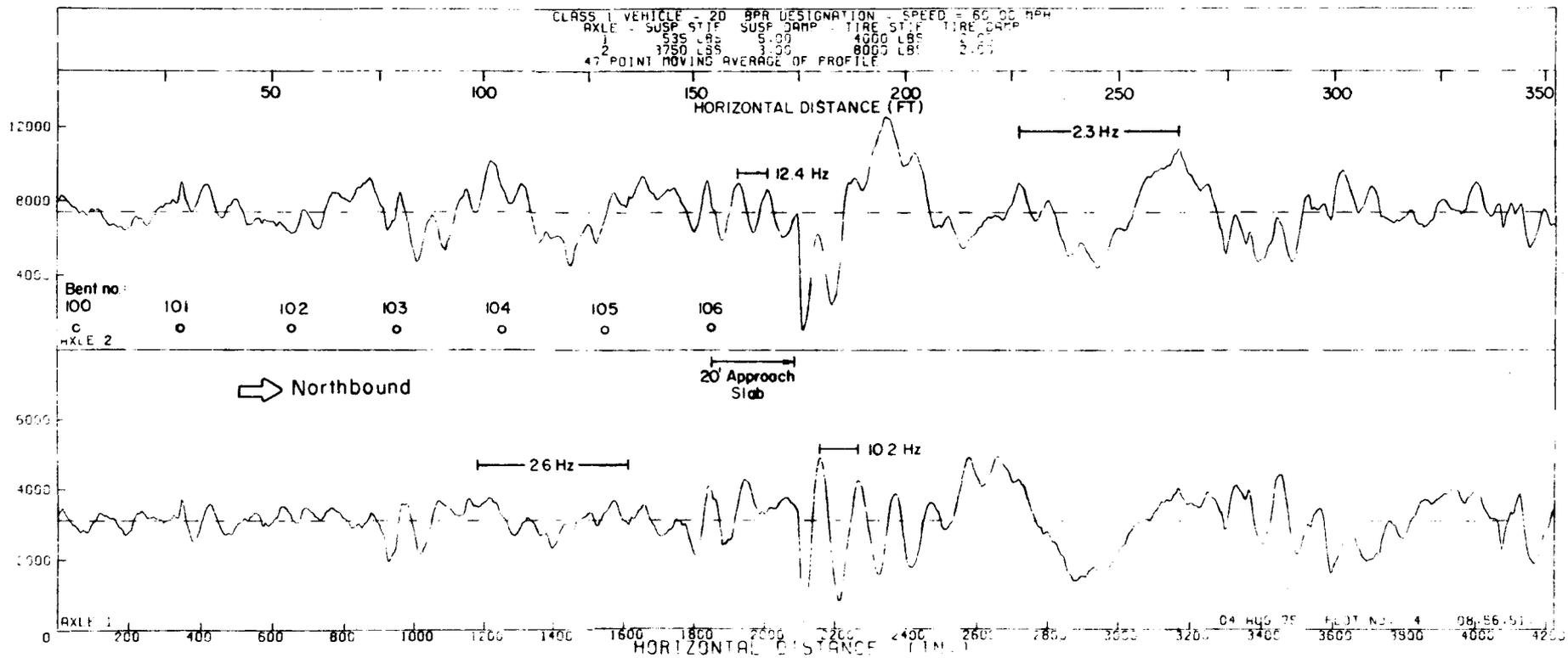
Fig 14. Left wheel forces on outside lane, northbound bridge, bent no.'s 100 to 106, 60 mph.
