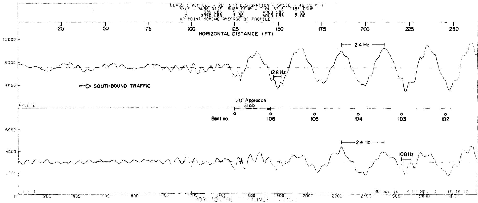
Fig 2. Left wheel forces on outside lane, southbound bridge, bent no.'s 106 to 102, 2-D truck at 40 mph.
