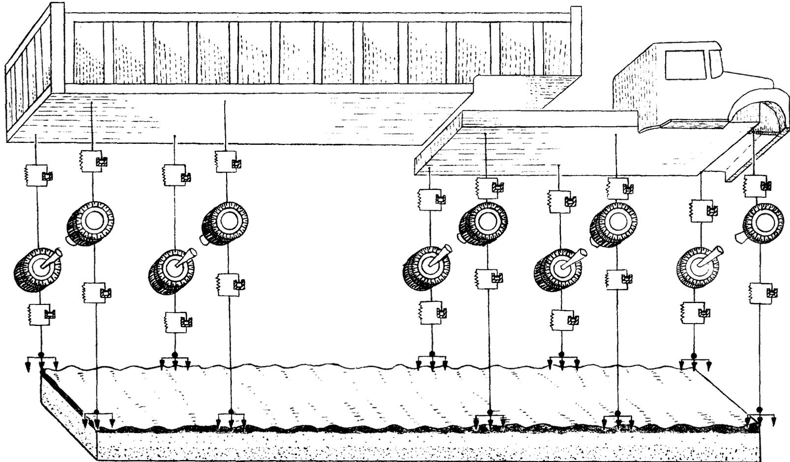
Plate B. Schematic diagram of five-axle tractor-semi-trailer articulated (Type 3S-2) vehicle model.
