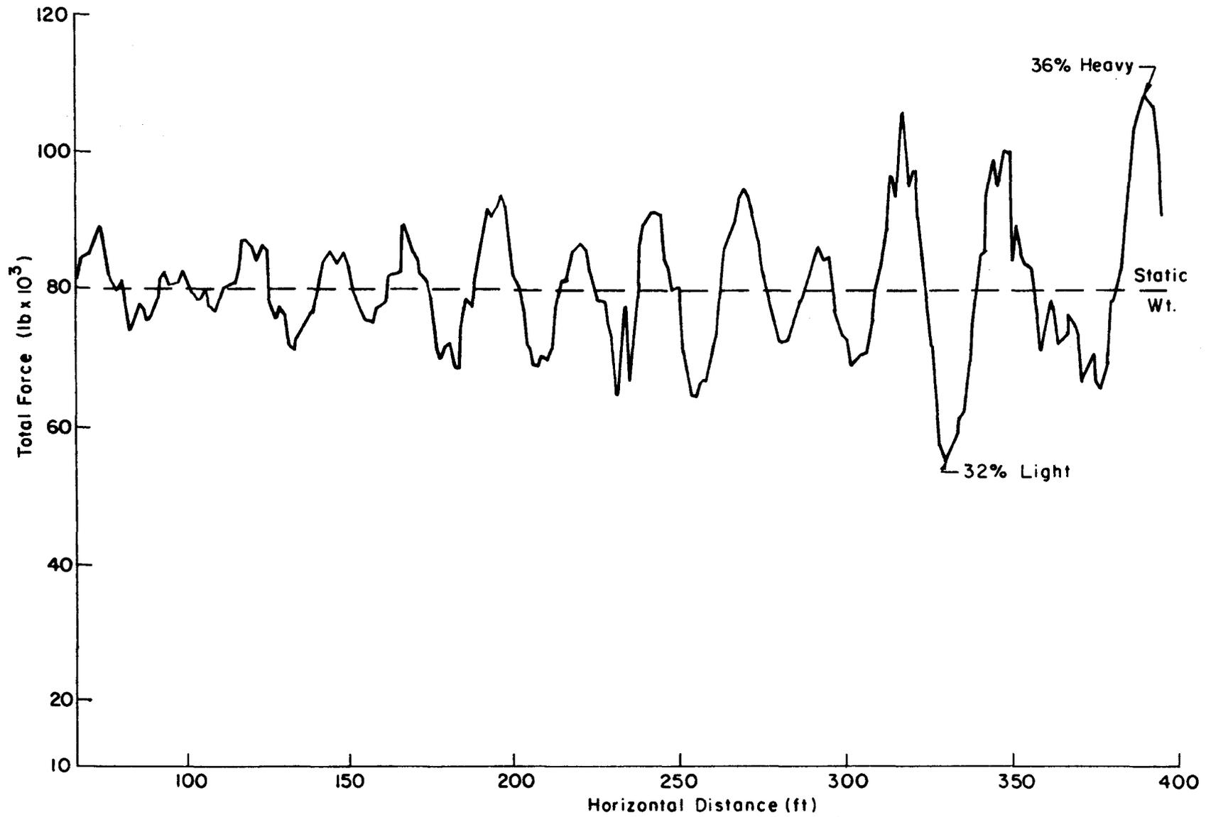
Fig 15. Total force exerted on bridge deck by 3S-2 vehicle traveling 50 mph over profile of Fig 6.
