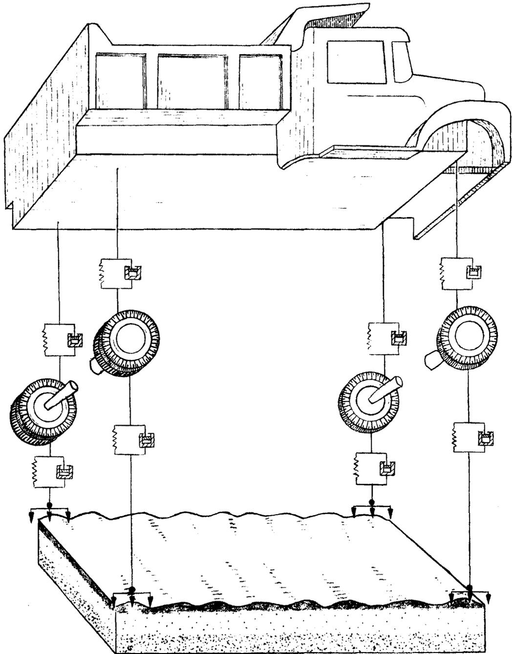
Plate A. Schematic diagram of single-unit two-axle dual tire (Type 2D) vehicle model.
