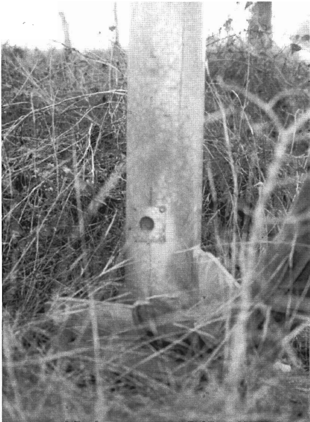
Figure D.6 ROS water-level sensor at Turtle Creek site in Kerr County
