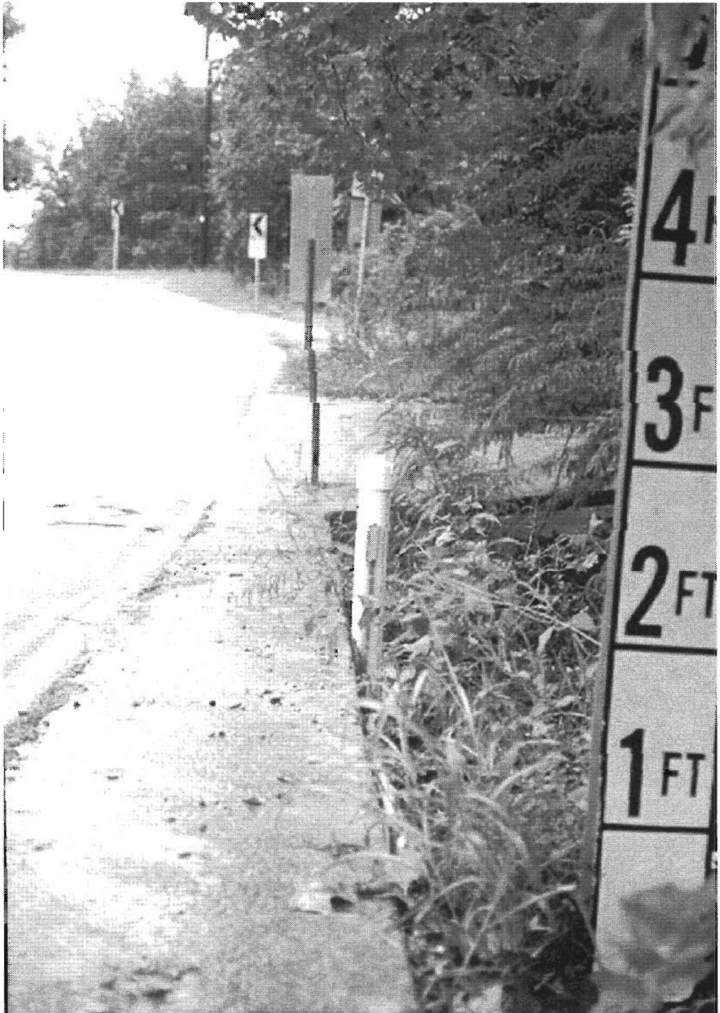
Figure D.3 A-TEK water-level sensor on Spicewood Springs Road in Austin
