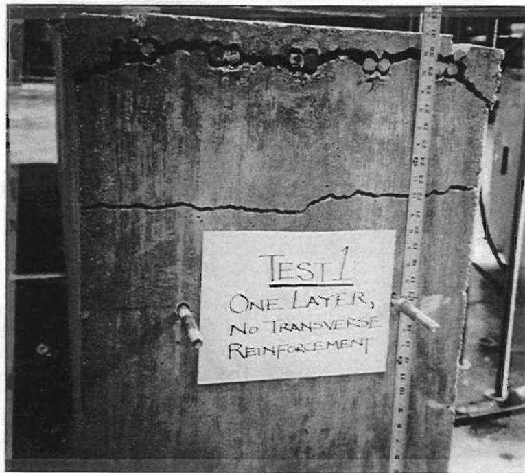
Figure A-5      *Second failure plane due to the release of energy at bond failure*
