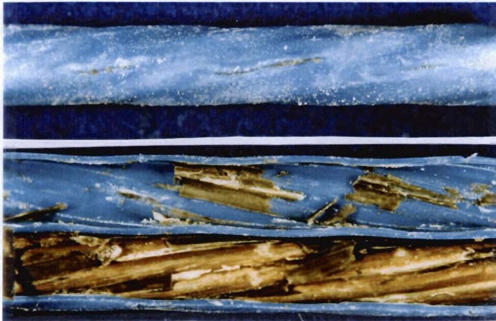
Figure 8- 38 Intrusion of grout into sheathing
