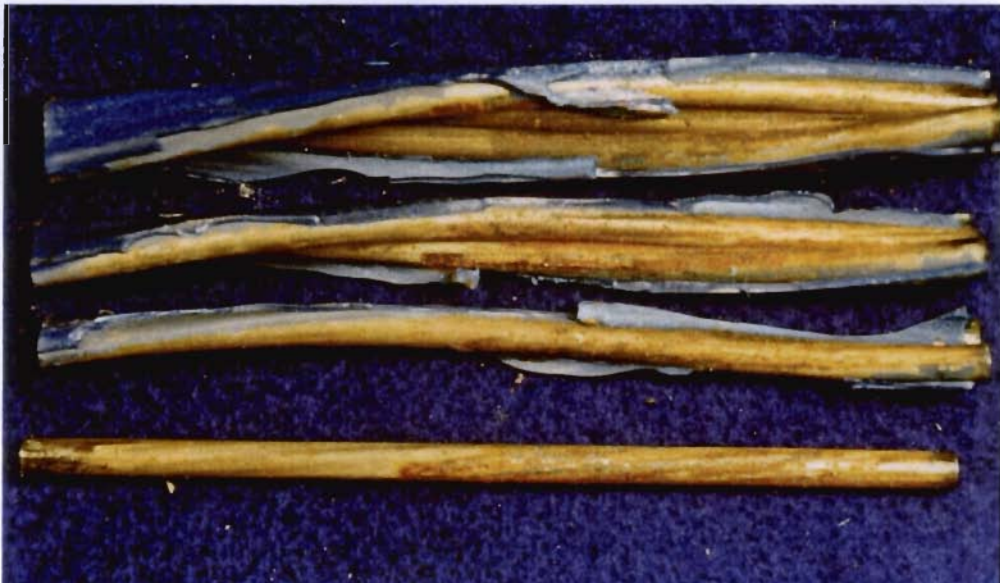
Figure 8- 29 Interstitial corrosion of epoxy-coated strand (not filled)
