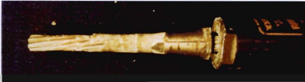
Figure 8-23 Example of removed wedge/strand section
