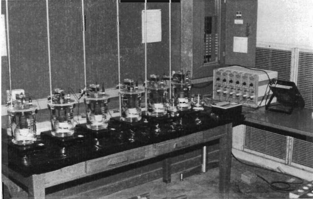
Figure 6-1 Modified accelerated corrosion test method setup
