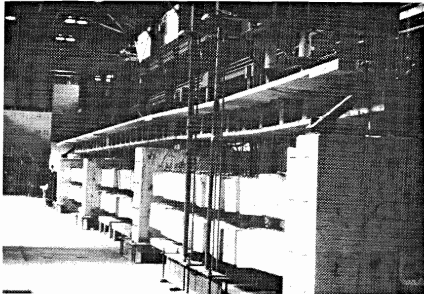
Figure 1. Model of externally post-tensioned bridge.
