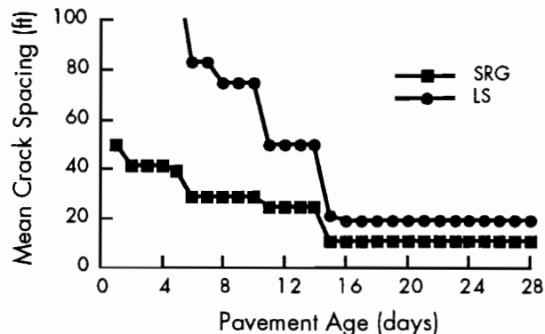
Figure 8.7. Changes in mean crack spacings with ages as affected by aggregate types
