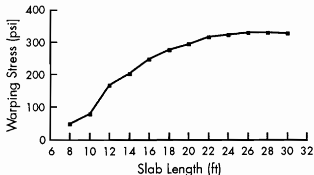
Figure 6.1. Warping stresses for 8-inch-thick slab for 20°F temperature differentials between top and bottom
