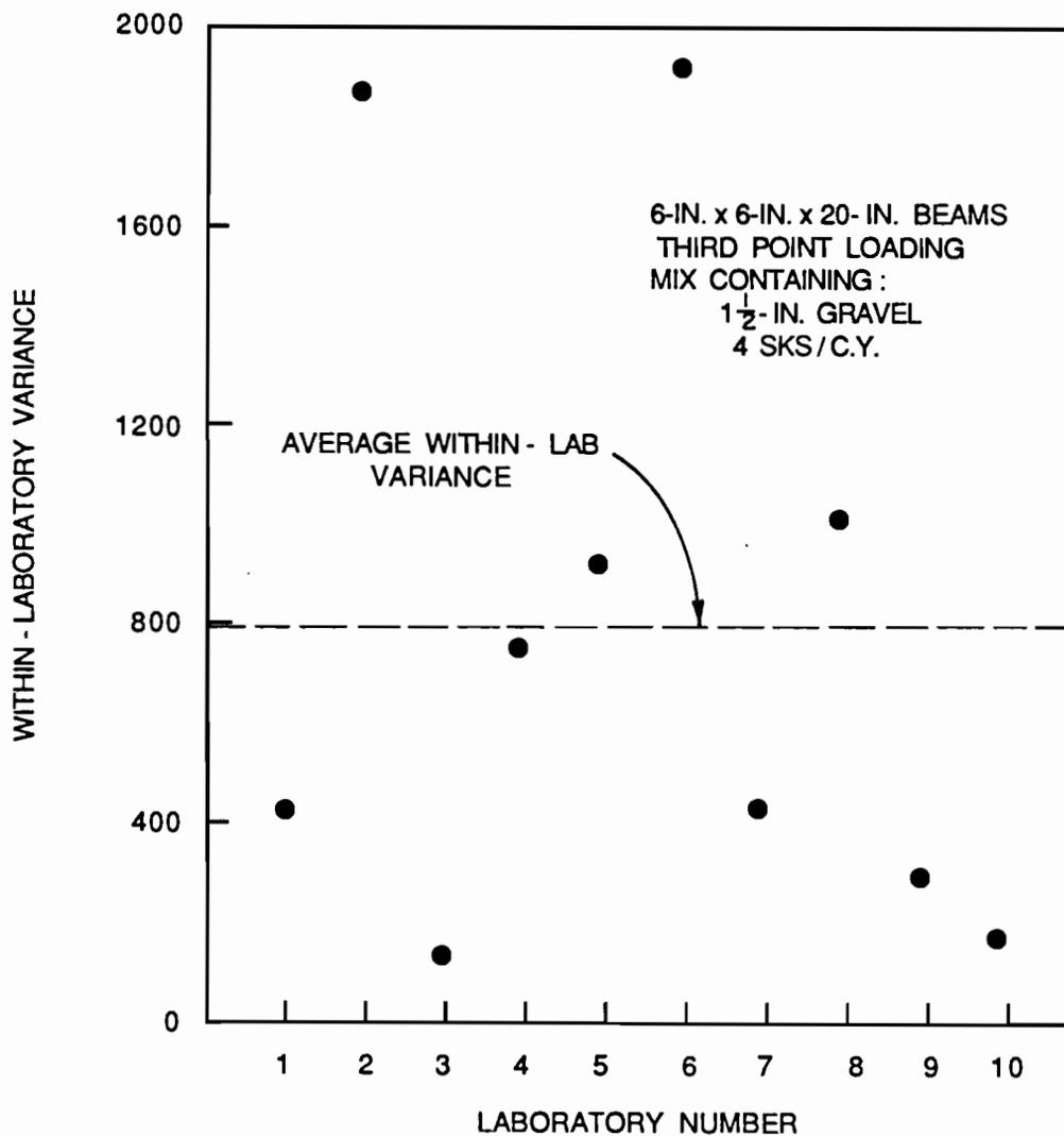
Fig. 5.6 Investigation for agreement of variances for each laboratory for test results obtained from 6-in. x 6-in. x 20-in. beams cast from the mix containing 1-1/2-in. gravel and four sacks of cement per cubic yard and tested in third point loading.
