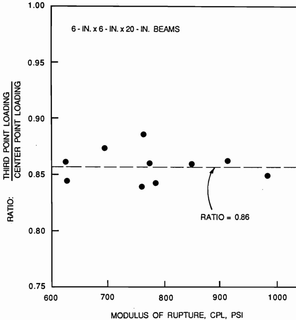
Fig. 4.18 Ratio of modulus of rupture test results obtained from third point loading to those obtained from center point loading, for 6-in. x 6-in. x 20-in. beams, potted versus results from the TSDHPT standard test method.
