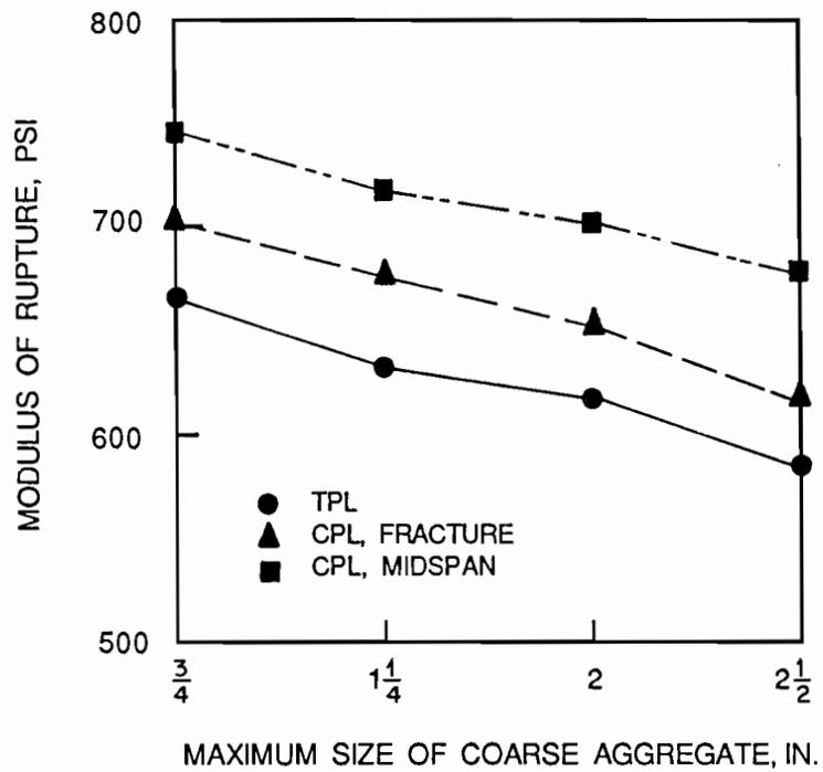
Fig. 2.1 Effect of method of loading and maximum size of coarse aggregate on average value of modulus of rupture of 6-in. x 6-in. x 21-in. beams (after Kellerman [5]).
