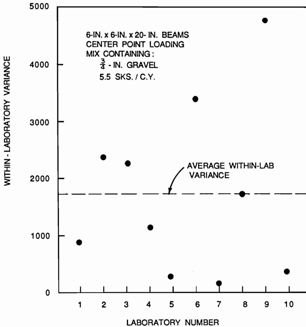
Fig. 5.2 Investigation for agreement of variances for each laboratory for test results obtained from 6-in. x 6-in. x 20-in. beams cast from the mix containing  $\frac{3}{4}$ -in. gravel and 5.5 sacks of cement per cubic yard and tested in center point loading.
