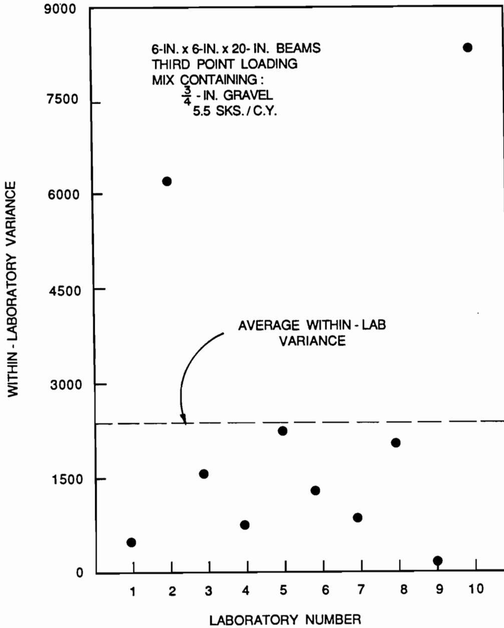
Fig. 5.7 Investigation for agreement of variances for each laboratory for test results obtained from 6-in. x 6-in. x 20-in. beams cast from the mix containing  $\frac{3}{4}$ -in. gravel and 5.5 sacks of cement per cubic yard and tested in third point loading.
