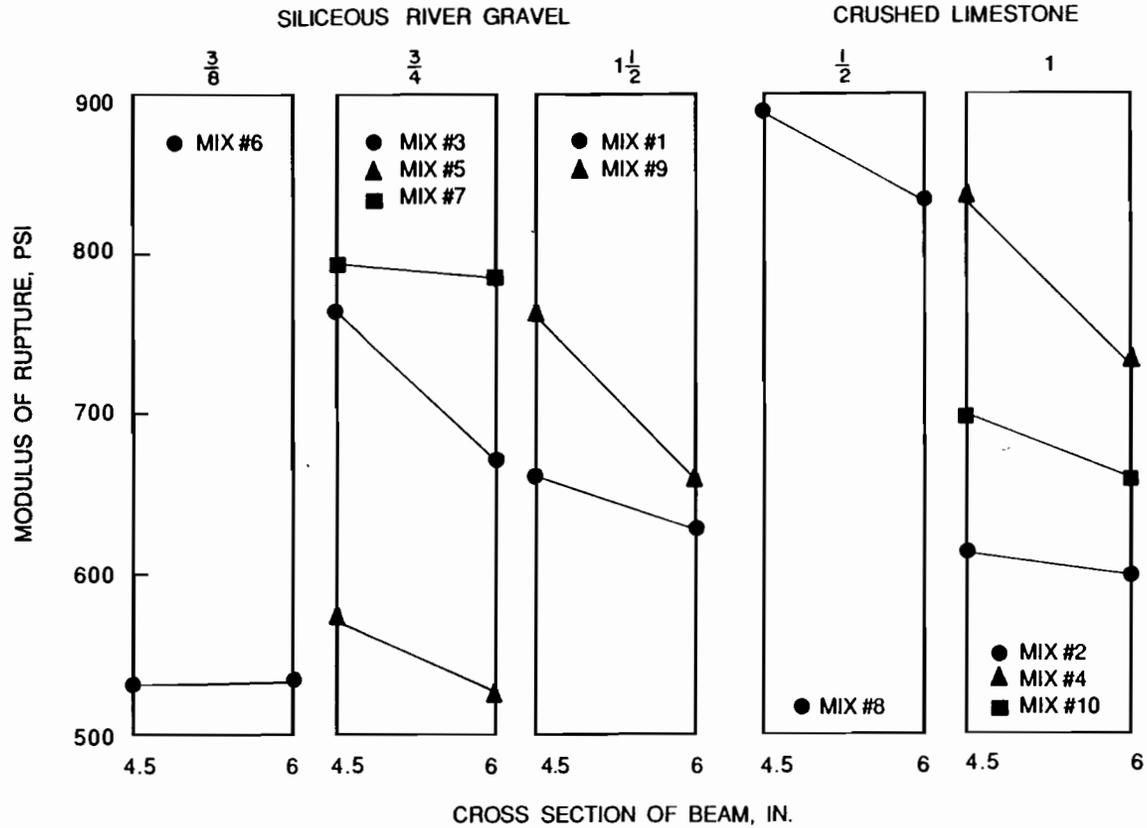
Fig. 4.7 Effect of specimen dimensions on the modulus of rupture of beams loaded at their third points for each coarse aggregate size.
