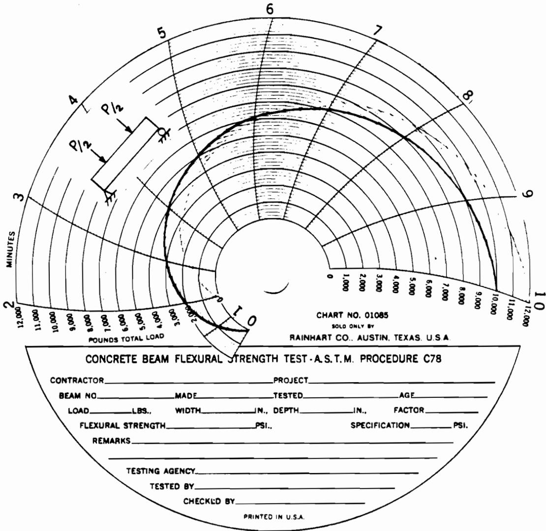
Fig. 3.5 Recording chart used for testing 4.5-in. x 4.5-in. x 15.5-in. beams in third point loading.
