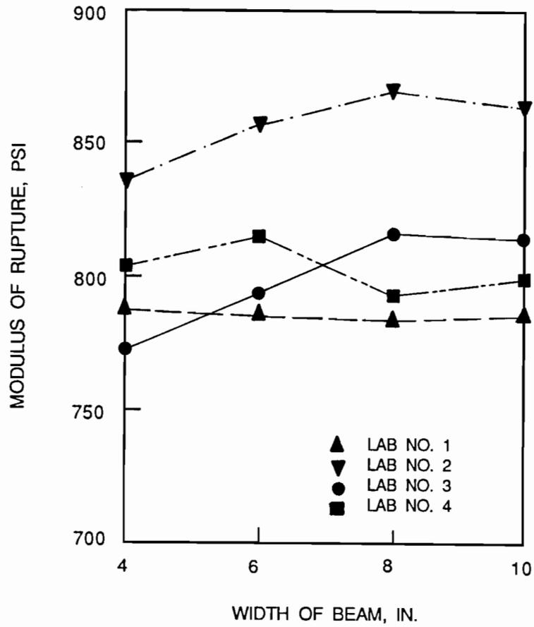
Fig. 2.4 Effect of width of beam on the average modulus of rupture of concrete test specimens tested in four different laboratories using third point loading (after Reagel and Willis [6]).
