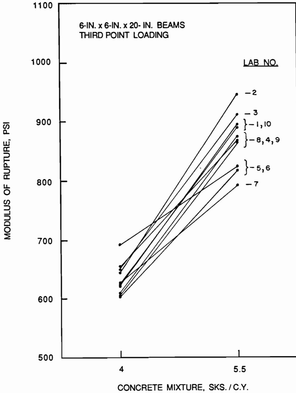
Fig. 5.8 Investigation for interactions in third point loading test results obtained from 6-in. x 6-in. x 20-in. beams.
