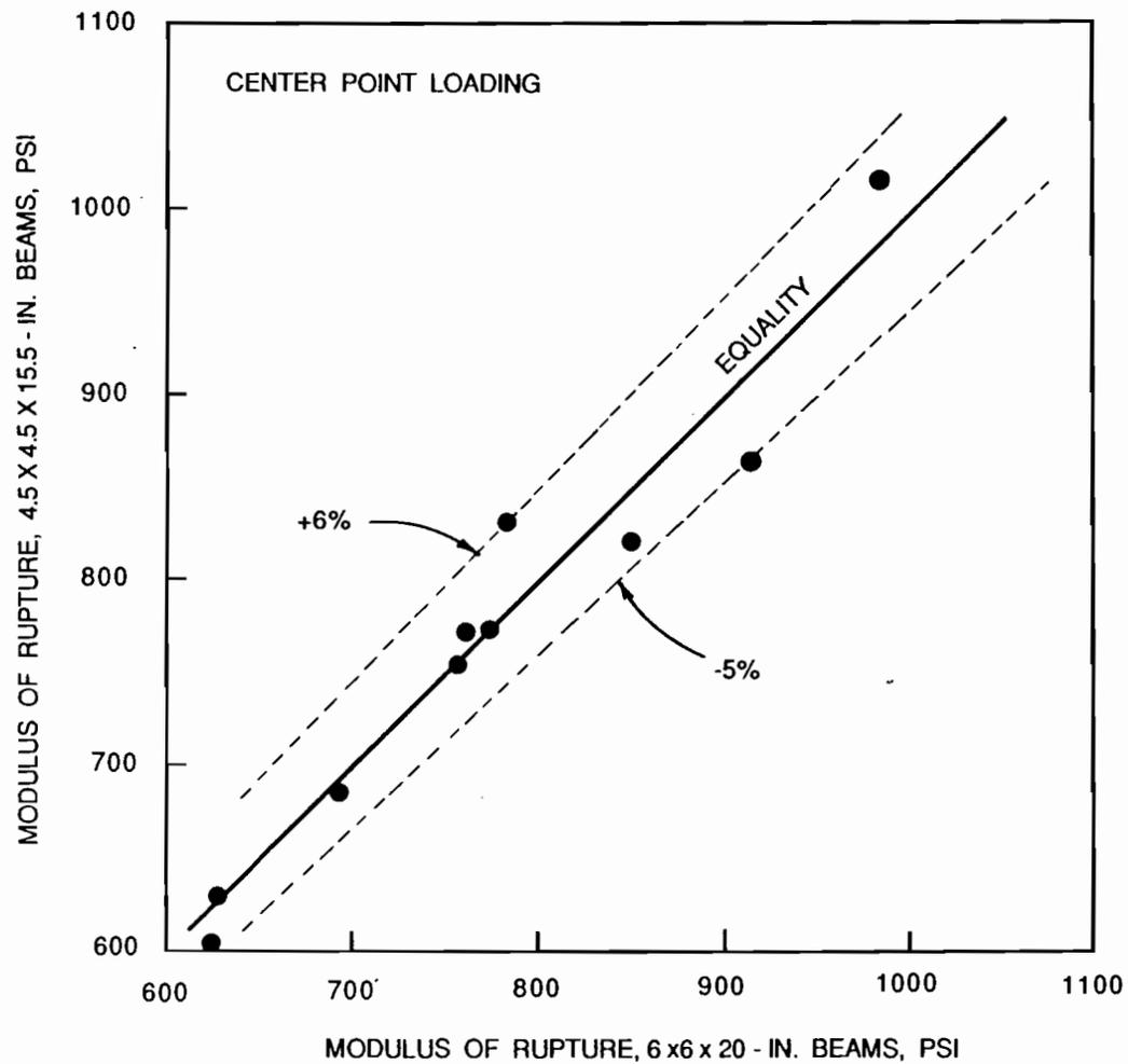
Fig. 4.4 Modulus of rupture of 4.5-in. x 4.5-in. x 15.5-in. beams versus that of 6-in. x 6-in. x 12-in. beams, both tested in center point loading.
