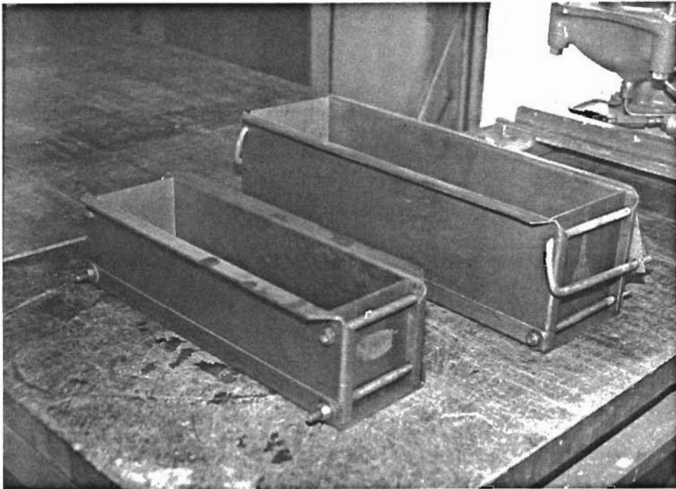
Fig. 3.1 Beam mold construction for both 4.5-in. x 4.5-in. x 15.5-in. beams and 6-in. x 6-in. x 20-in. beams.
