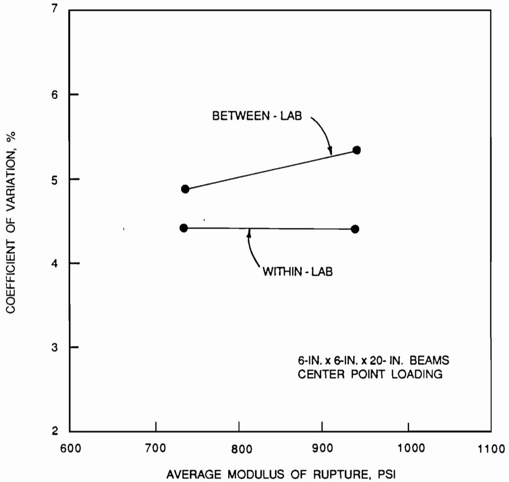
Fig. 5.5 Coefficient of variation versus average modulus of rupture for 6-in. x 6-in. x 20-in. beams tested in center point loading.
