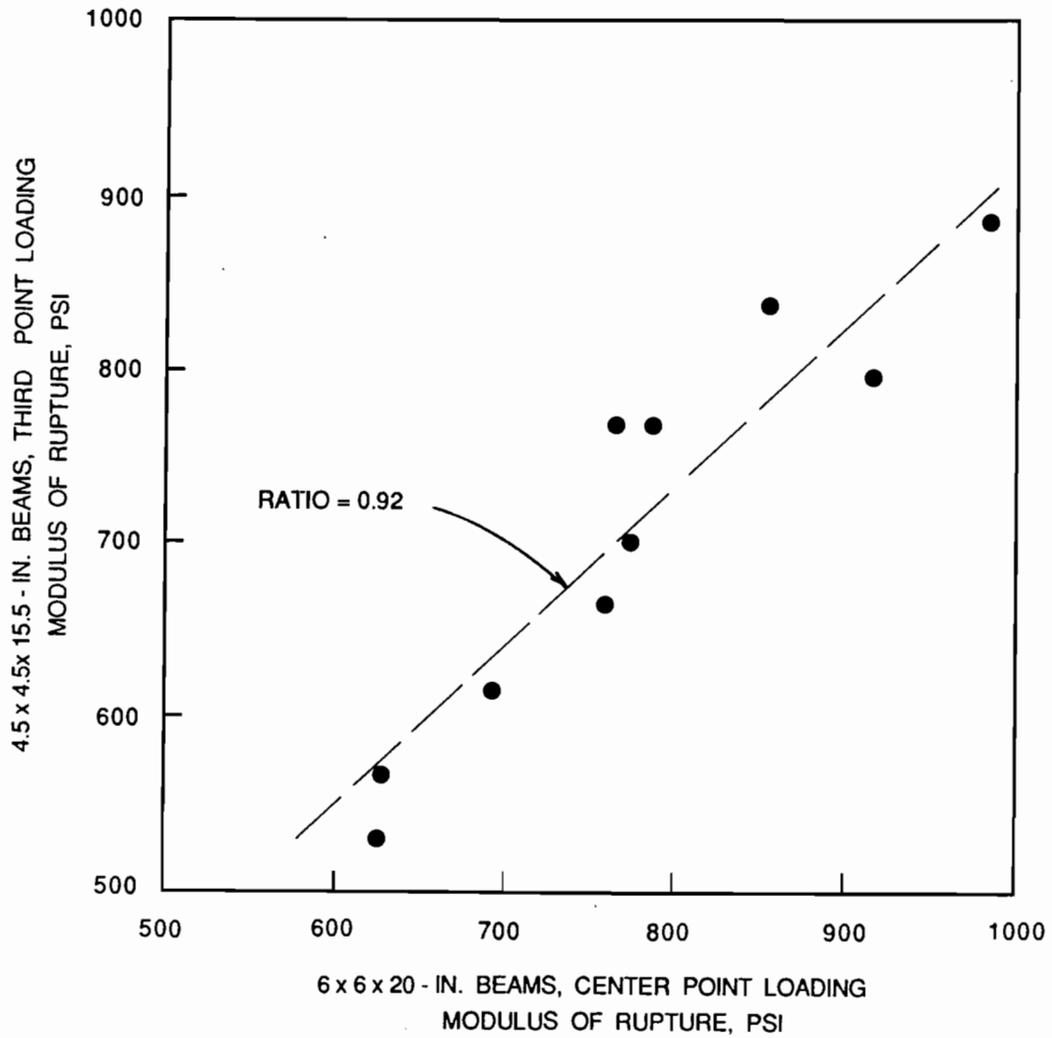
Fig. 4.22 Modulus of rupture of 4.5-in. x 4.5-in. x 15.5-in. beams tested in third point loading plotted versus 6-in. x 6-in. x 20-in. beams tested in center point loading.
