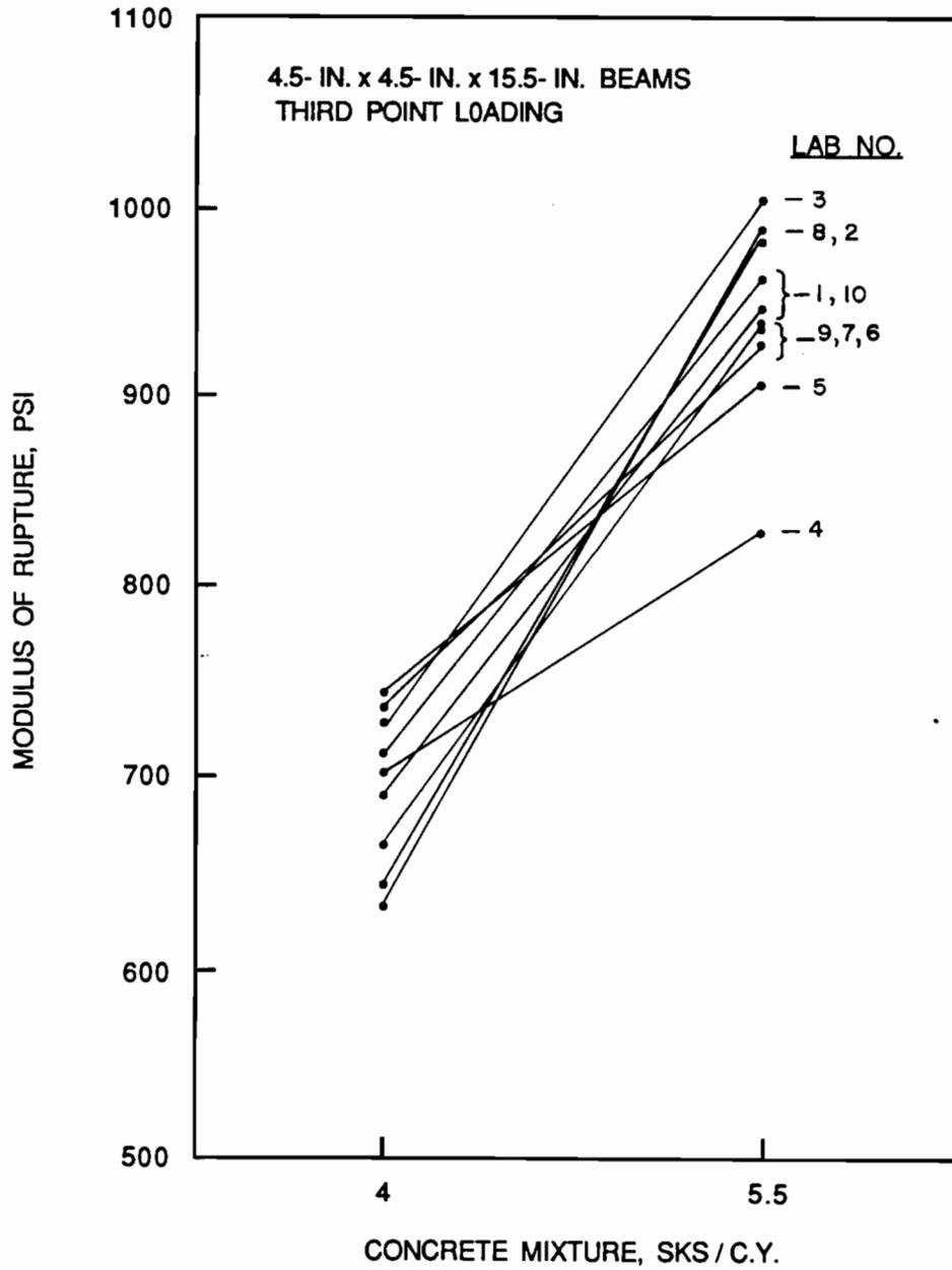
Fig. 5.18 Investigation for interactions in third point loading test results obtained from 4.5-in. x 4.5-in. x 15.5-in. beams.
