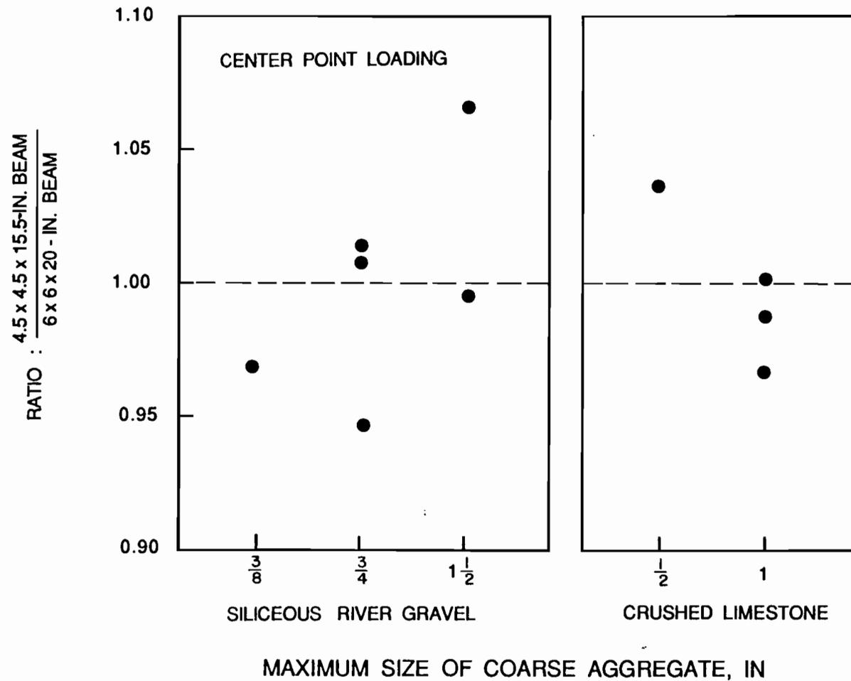
Fig. 4.6 Ratio of modulus of rupture of 4.5-in. x 4.5-in. x 15.5-in. beams to 6-in. x 6-in. x 20-in. beams, for center point loading, plotted versus coarse aggregate size.
