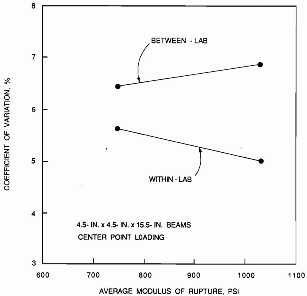
Fig. 5.15 Coefficient of variation versus average modulus of rupture for 4.5-in. x 4.5-in. x 15.5-in. beams tested in center point loading.
