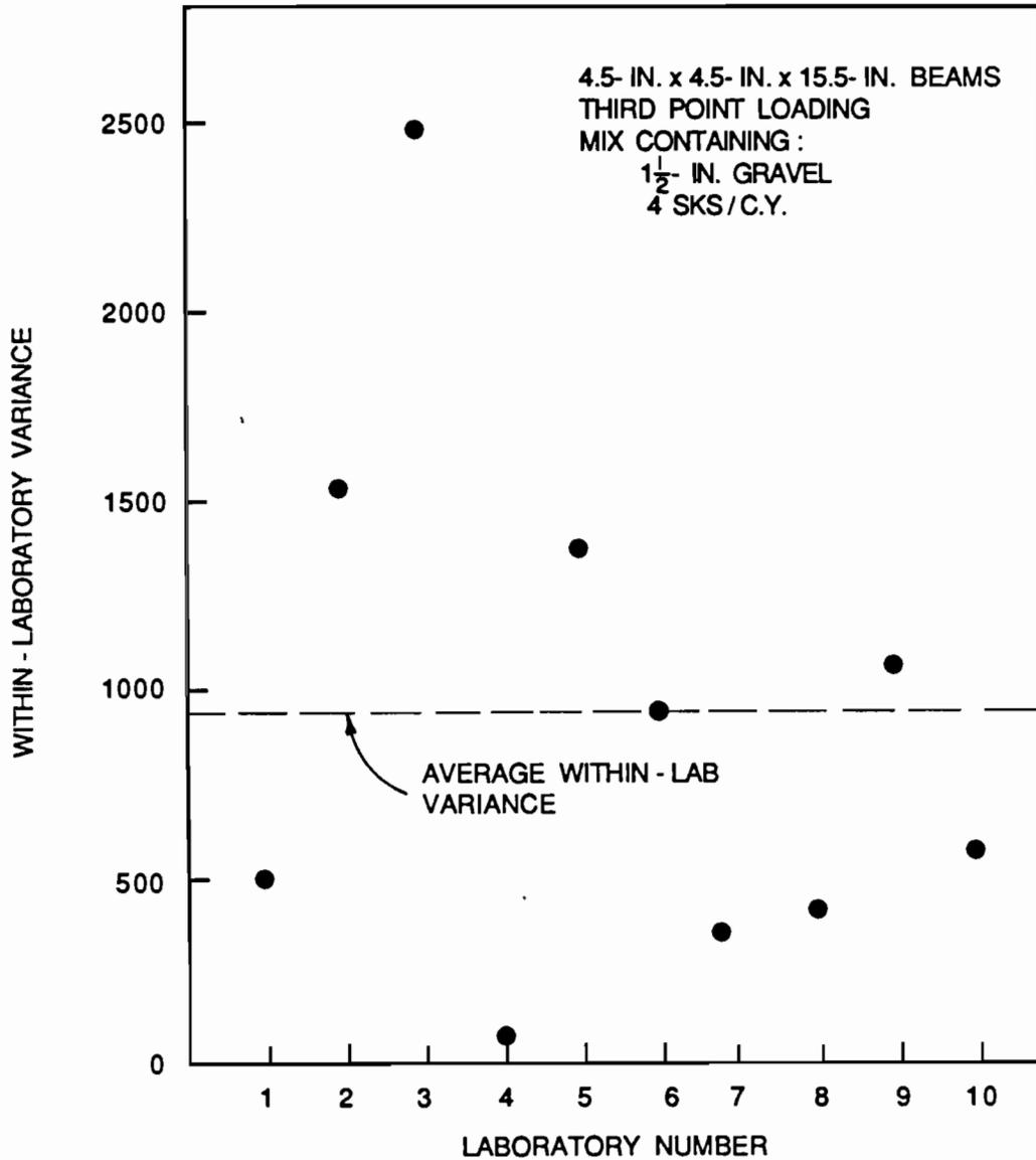
Fig. 5.16 Investigation for agreement of variances for each laboratory for test results obtained from 4.5-in. x 4.5-in. x 15.5-in. beams cast from the mix containing 1-1/2-in. gravel and four sacks of cement per cubic yard and tested in third point loading.
