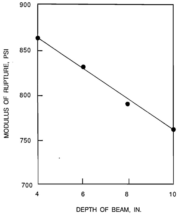
Fig. 2.6 Effect of depth of beam on the average modulus of rupture of concrete test specimens tested in third point loading, all laboratories combined (after Reagel and Willis [6]).
