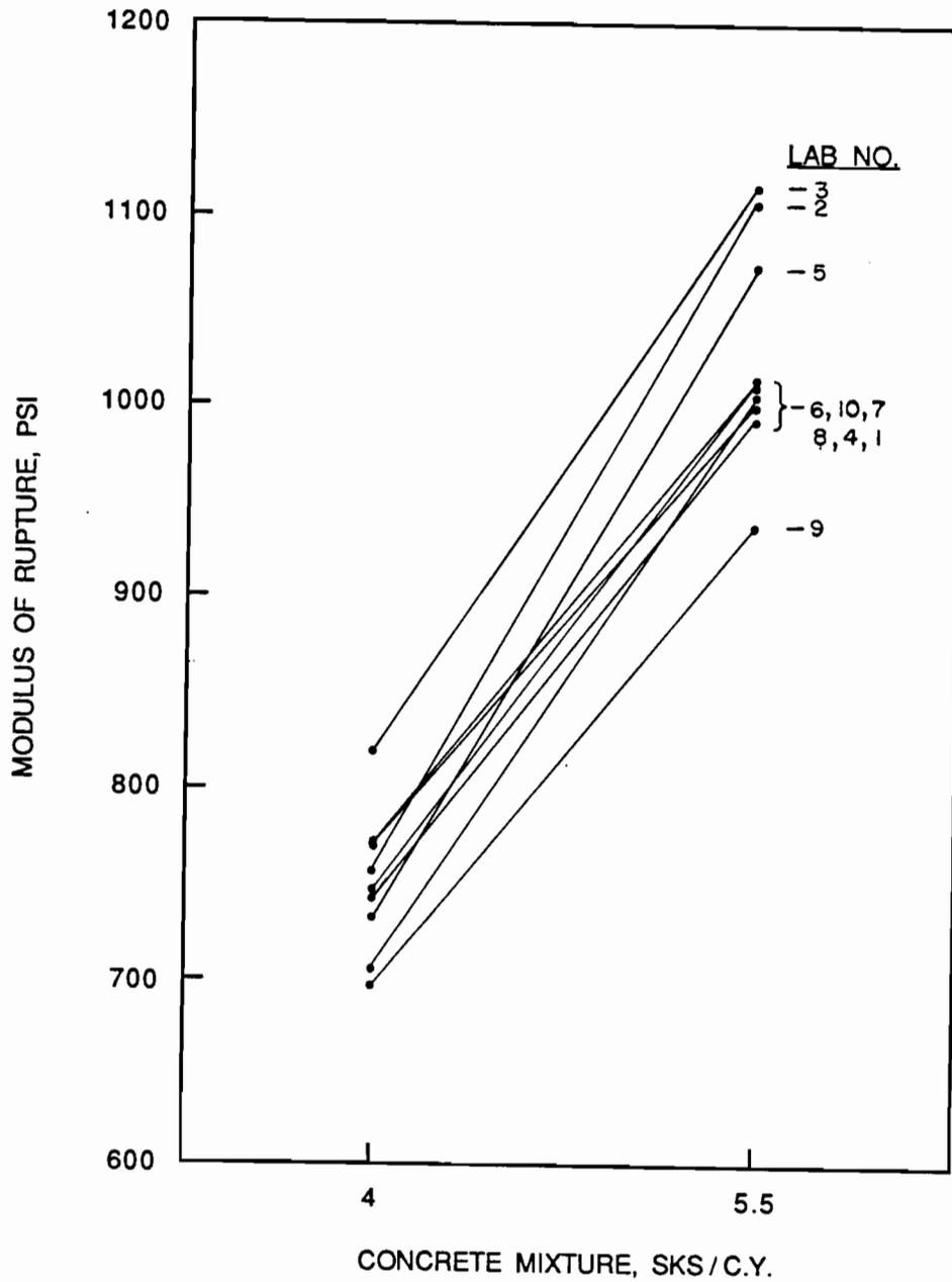
Fig. 5.13 Investigation for interactions in center point loading test results obtained from 4.5-in. x 4.5-in. x 15.5-in. beams.
