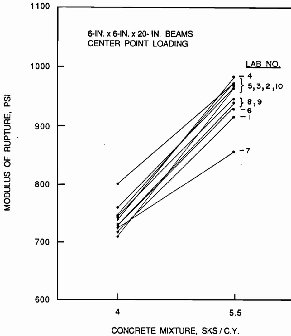
Fig. 5.3 Investigation for interactions in center point loading test results obtained from 6-in. x 6-in. x 20-in. beams.
