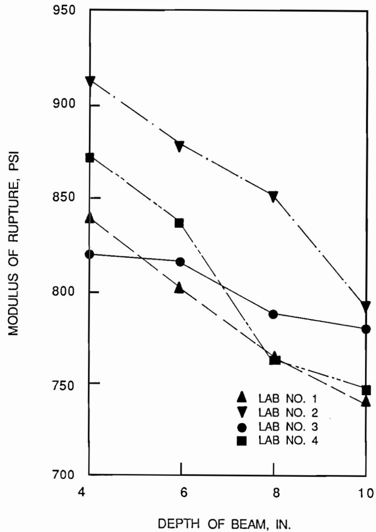
Fig. 2.5 Effect of depth of beam on the average modulus of rupture of concrete test specimens tested in four different laboratories using third point loading (after Reagel and Willis [6]).
