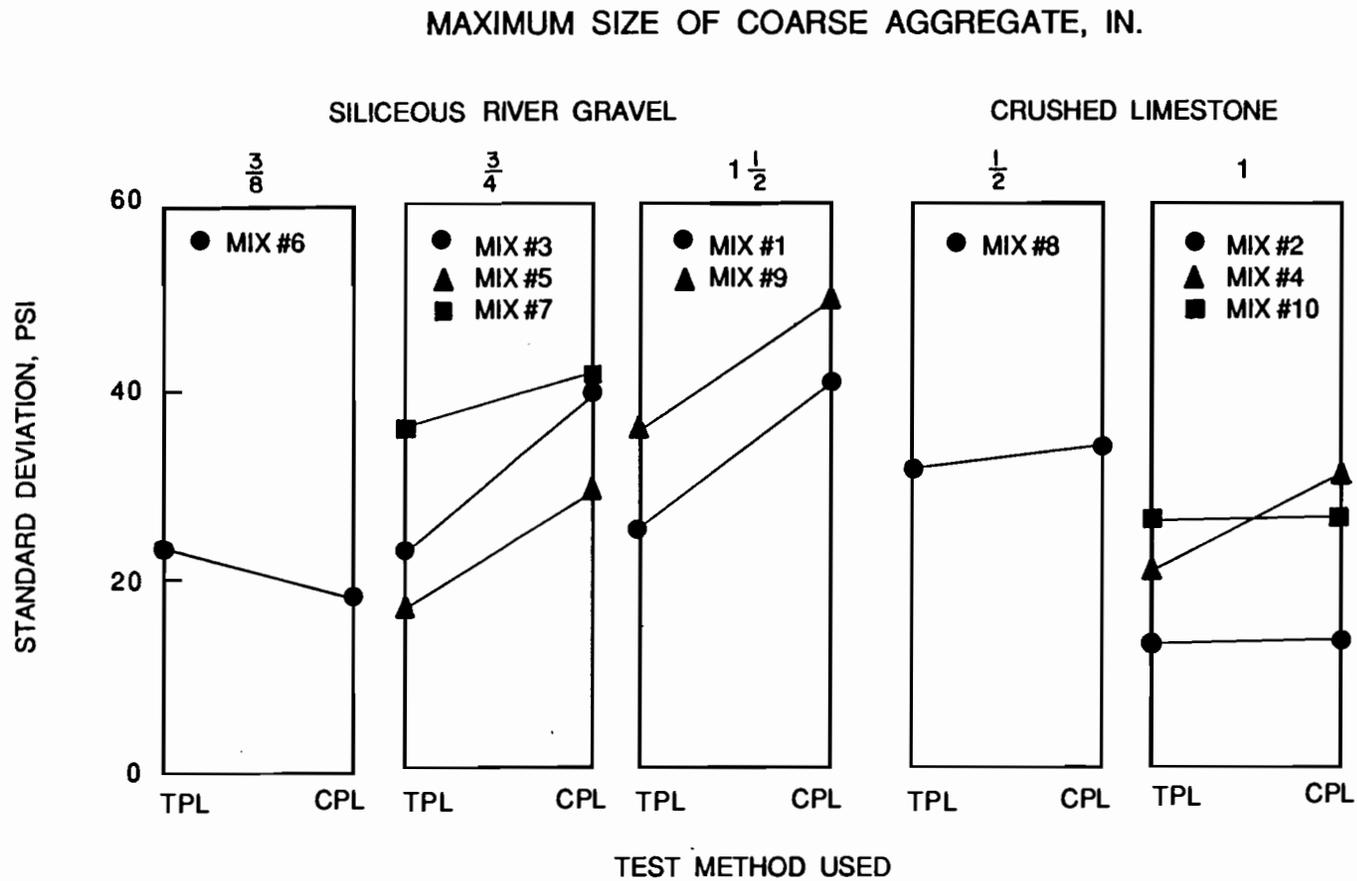
Fig. 4.20 Standard deviation of 6-in. x 6-in. x 20-in. beams tested in third point loading versus center point loading for each aggregate size.
