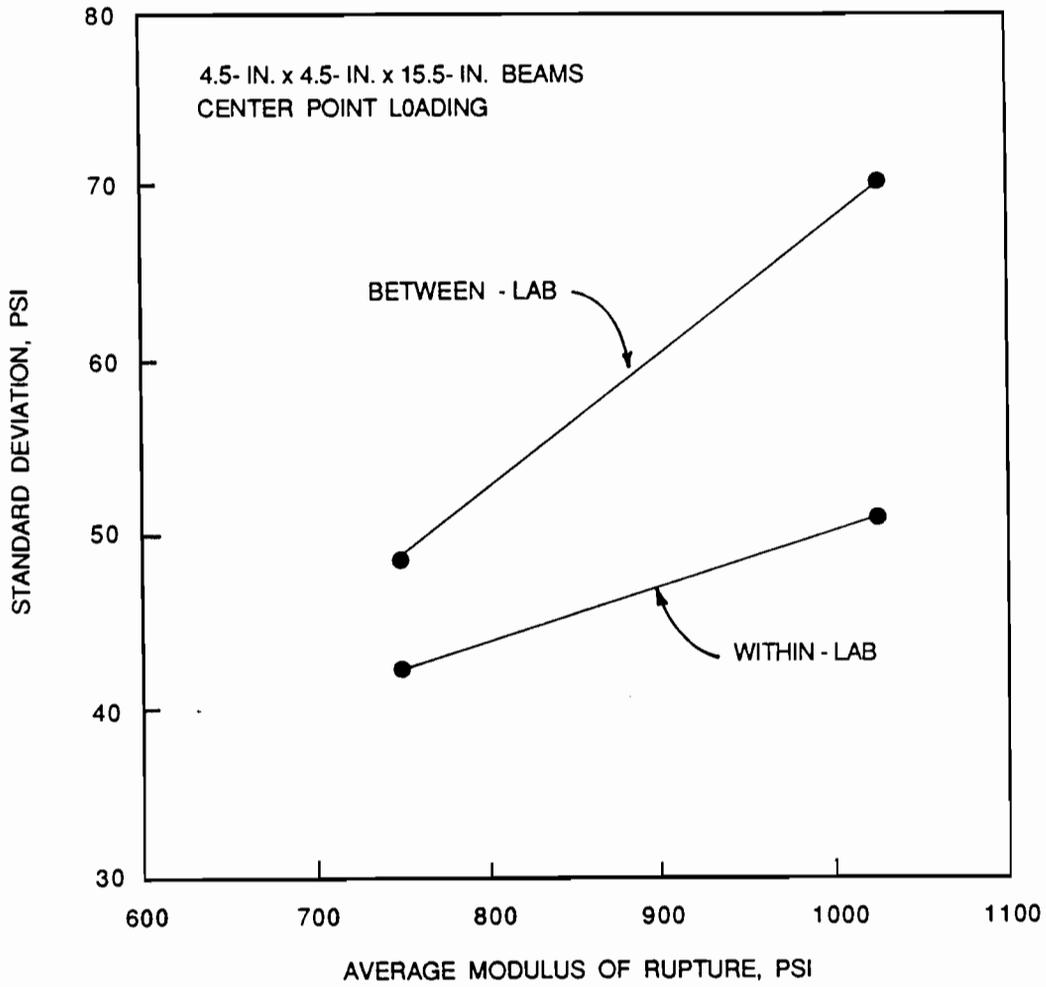
Fig. 5.14 Standard deviation versus average modulus of rupture for 4.5-in. x 4.5-in. x 15.5-in. beams tested in center point loading.
