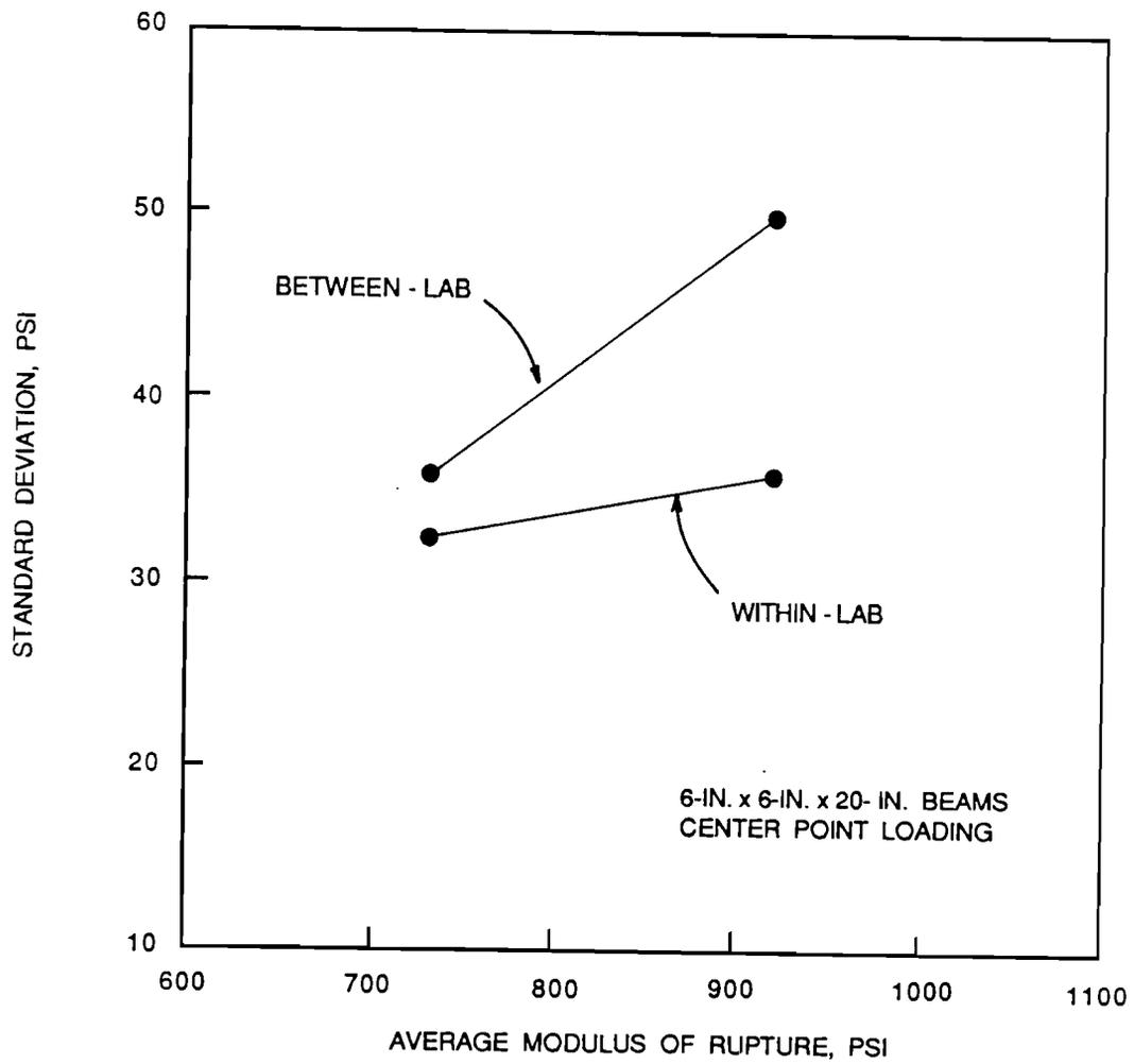
Fig. 5.4 Standard deviation versus average modulus of rupture for 6-in. x 6-in. x 20-in. beams tested in center point loading.
