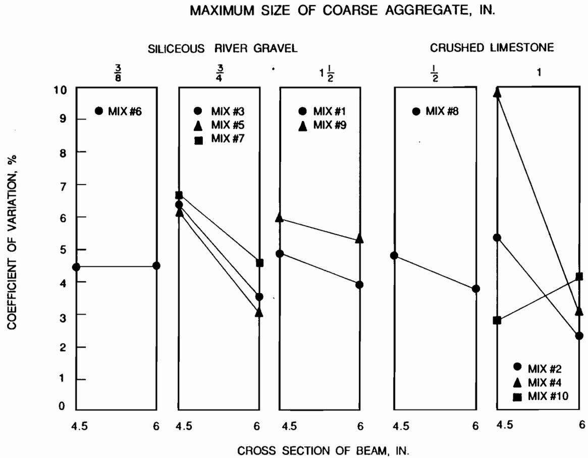
Fig. 4.9 Effect of specimen dimensions on the coefficient of variation of test results from beams loaded at their third points for each coarse aggregate size
