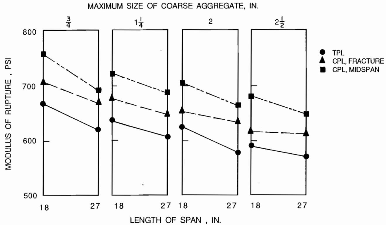
Fig. 2.8 Effect of length of span on the average modulus of rupture of concrete test specimens having a cross section of 6-in. x 6-in. (after Kellemann [5]).
