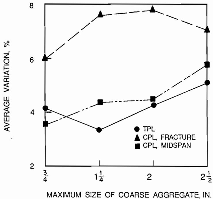
Fig. 2.2 Effect of method of loading and maximum size of coarse aggregate on average percentage variation of test results from 6-in. x 6-in. x 21-in. beams (after Kellerman [5]).
