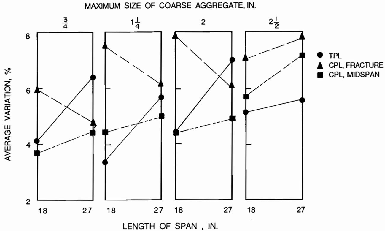
Fig. 2.9 Effect of length of span on average percentage variation of test results from 6-in. x 6-in. concrete beams (after Kellermann [5]).
