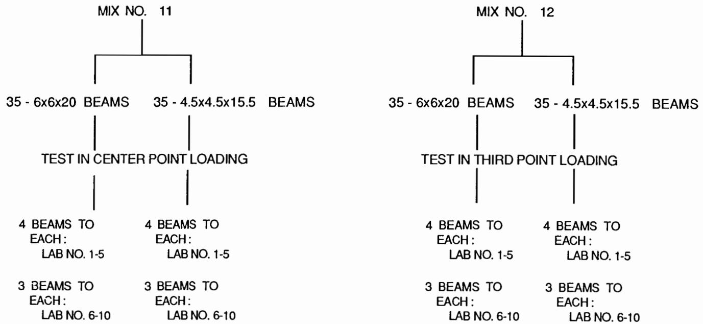
Fig. 3.6 Distribution of beams for testing in the interlaboratory study.
