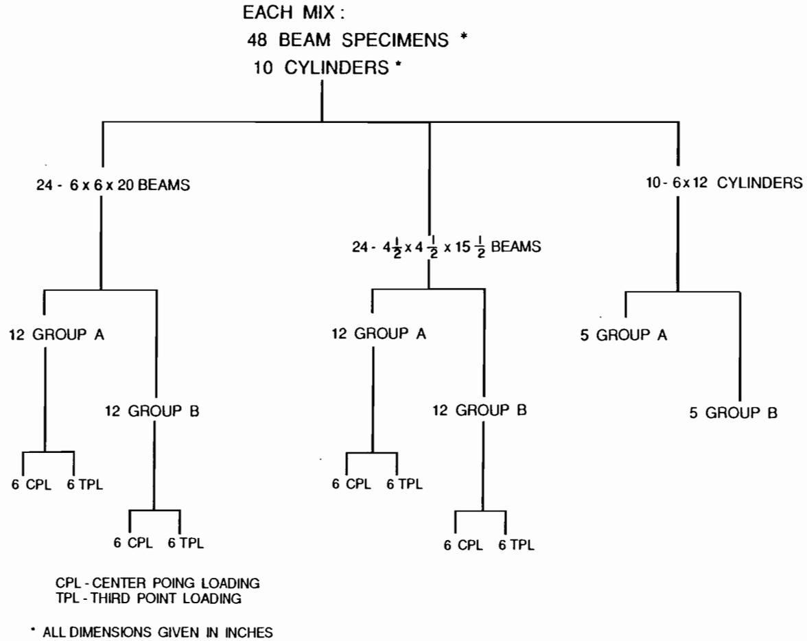
Fig. 3.2 Preparation and testing diagram of specimens for each mix from the first stage of testing.
