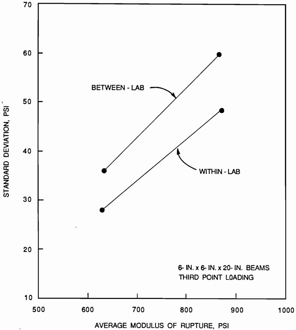
Fig. 5.9 Standard deviation versus average modulus of rupture for 6-in. x 6-in. x 20-in. beams tested in third point loading.
