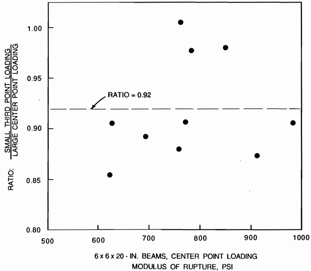
Fig. 4.23 Ratio of modulus of rupture from 4.5-in. x 4.5-in. x 15.5-in. beams tested in third point loading to 6-in. x 6-in. x 20-in. beams tested in center point loading, plotted versus the modulus of rupture of 6-in. x 6-in. x 20-in. beams tested in center point loading.
