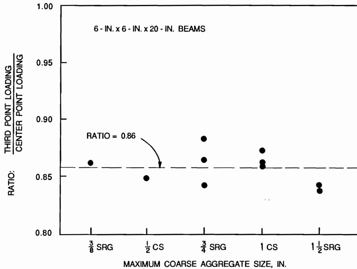
Fig. 4.19 Ratio of modulus of rupture test results obtained from third point loading to those obtained from center point loading, for 6-in. x 6-in. x 20-in. beams, plotted versus coarse aggregate size.
