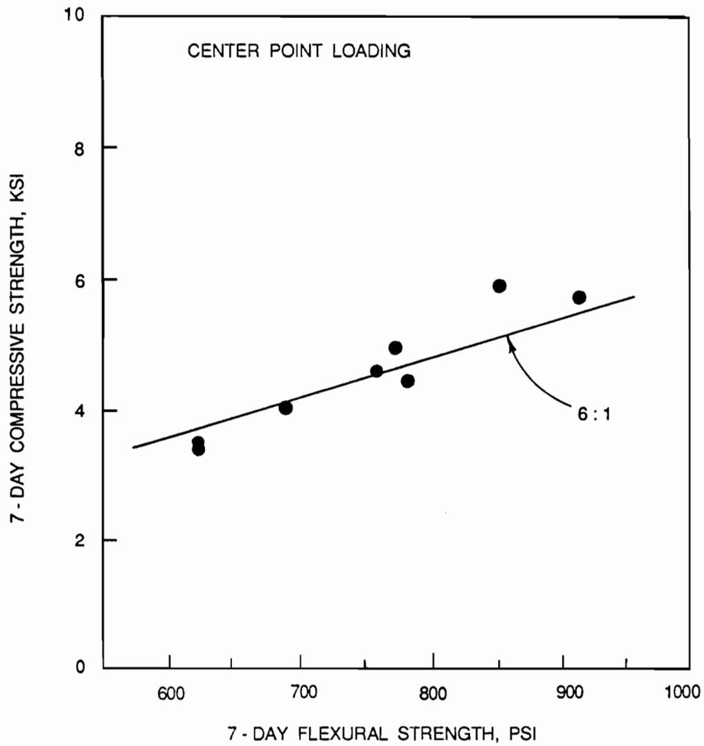
Fig. 4.29 Seven-day compressive strength versus 7-day flexural strength (center point loading).
