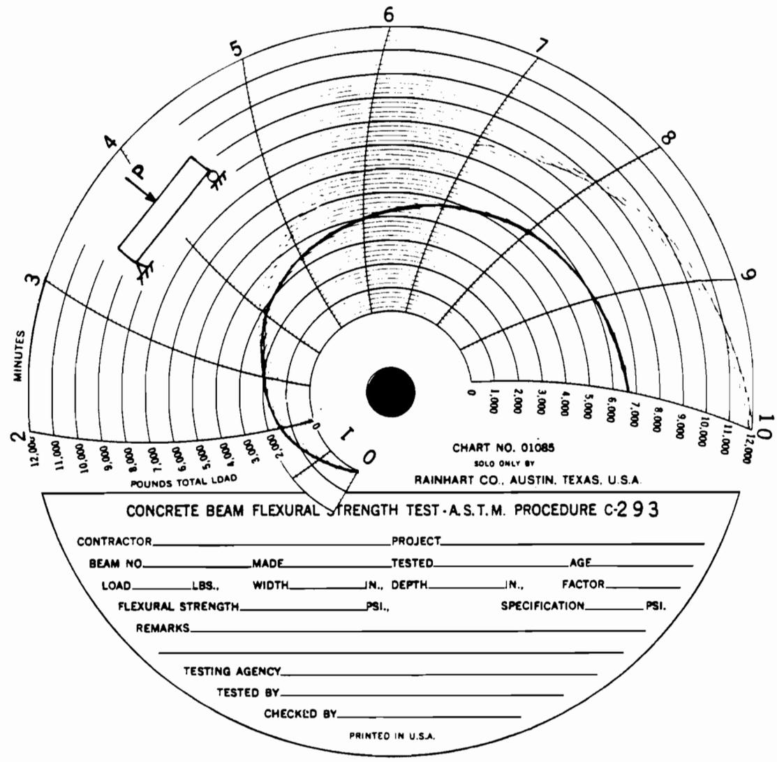
Fig. 3.4 Recording chart used for testing 4.5-in. x 4.5-in. x 15.5-in. beams in center point loading.
