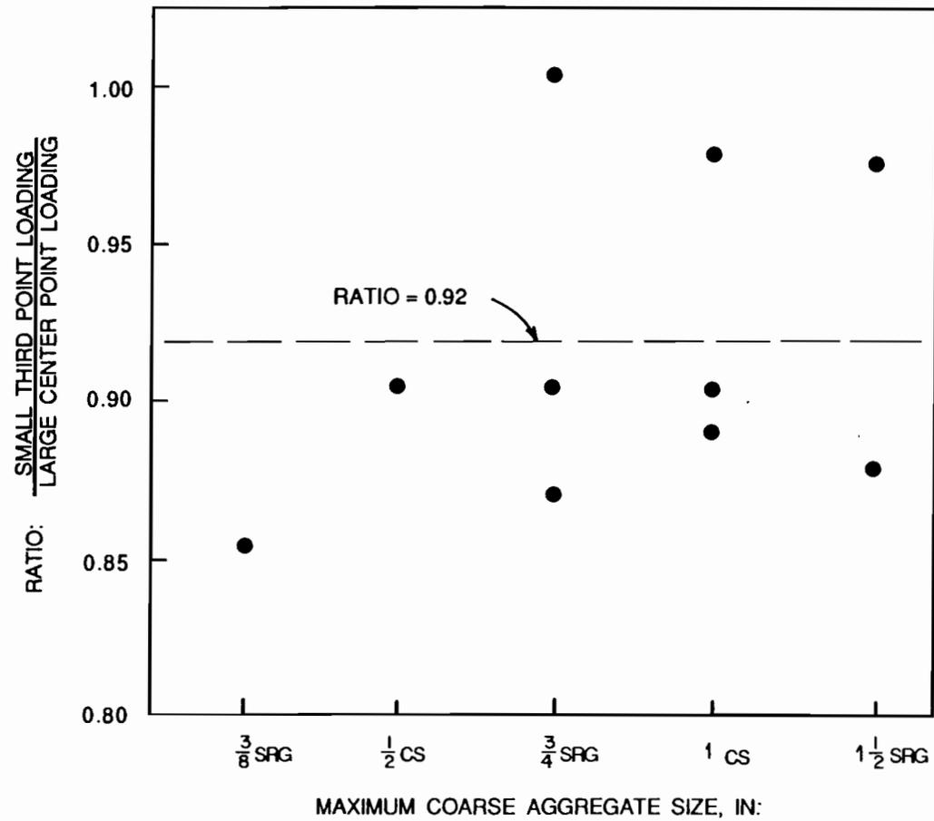
Fig. 4.24 Ratio of modulus of rupture from 4.5-in. x 4.5-in. x 15.5-in. beams tested in third point loading to 6-in. x 6-in. x 20-in. beams tested in center point loading, plotted versus coarse aggregate size.
