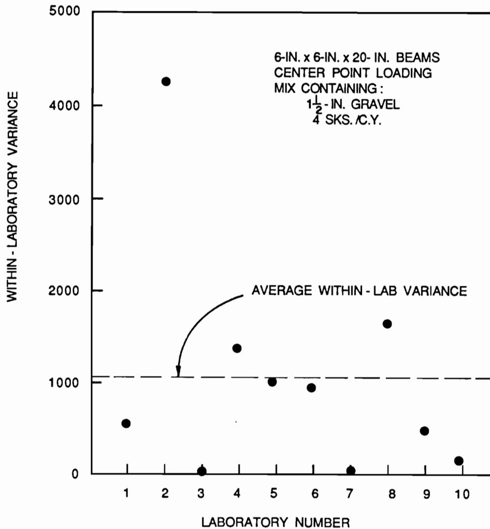
Fig. 5.1 Investigation for agreement of variances for each laboratory for test results obtained from 6-in. x 6-in. x 20-in. beams cast from the mix containing 1-1/2-in. gravel and four sacks of cement per cubic yard and tested in center point loading.
