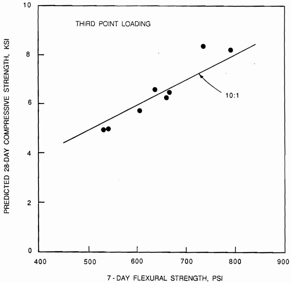
Fig. 4.31 Twenty-eight-day compressive strength versus 7-day flexural strength (third point loading).
