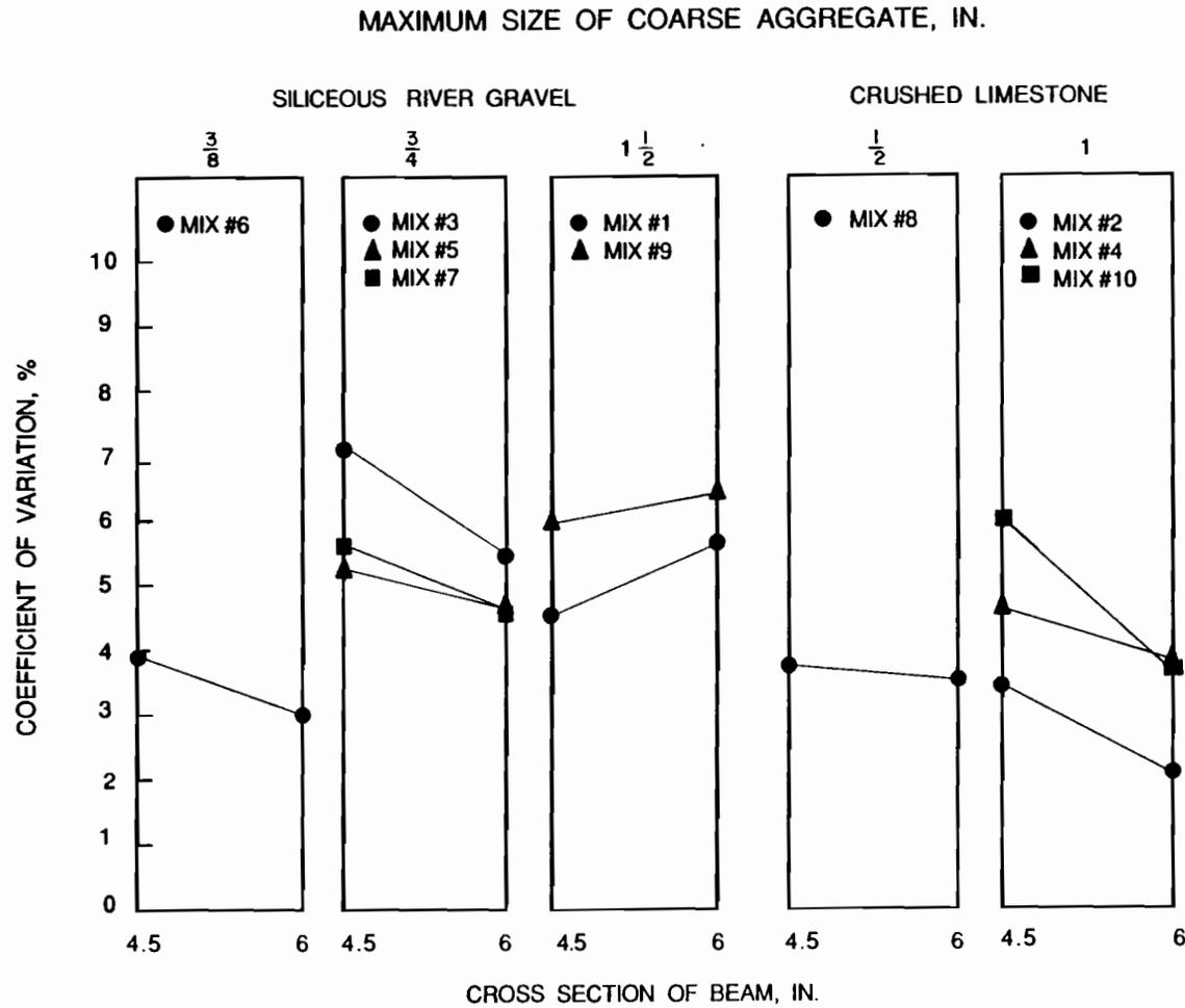
Fig. 4.3 Effect of specimen dimensions on the coefficient of variation of test results from beams loaded at their center point.
