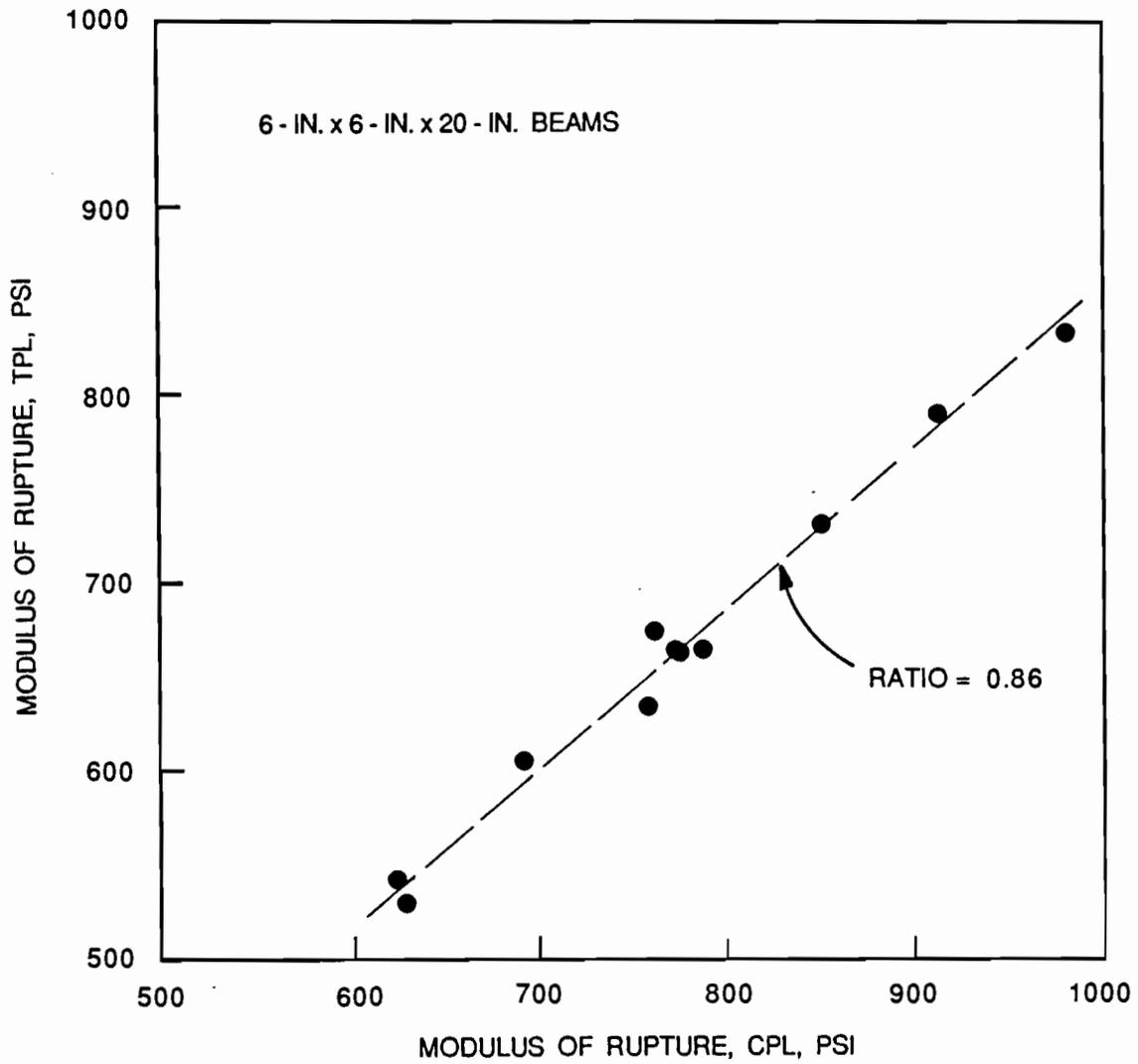
Fig. 4.17 Modulus of rupture of beams tested in center point loading versus third point loading, for 6-in. x 6-in. x 20-in. beams.
