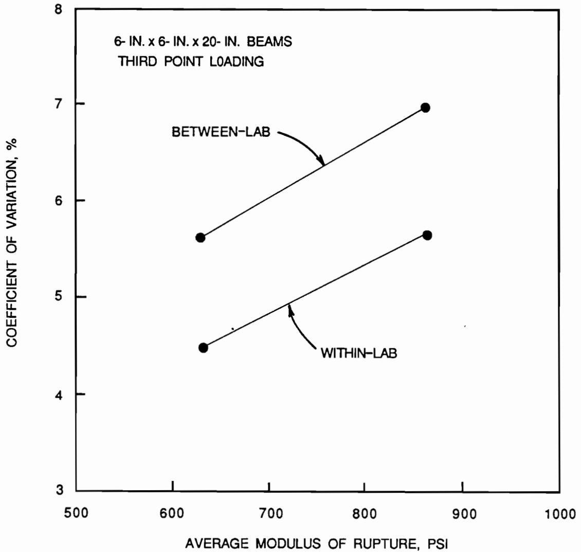
Fig. 5.10 Coefficient of variation versus average modulus of rupture for 6-in. x 6-in. x 20-in. beams tested in third point loading.
