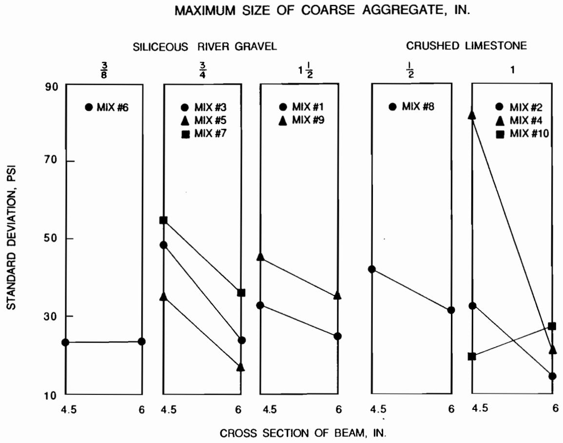
Fig. 4.8 Effect of specimen dimensions on the standard deviation of test results from beams loaded at their third points for each coarse aggregate size
