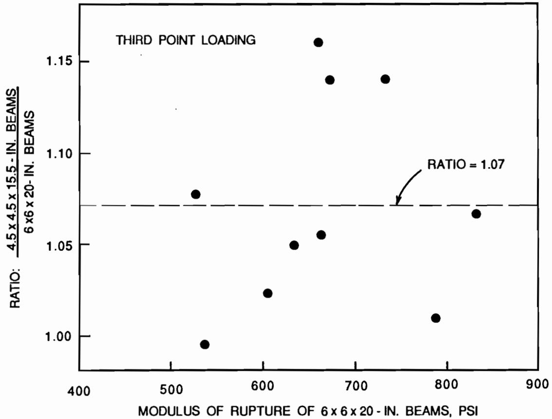
Fig. 4.11 Ratio of modulus of rupture in third point loading of 4.5-in. x 4.5-in. x 15.5-in. beams to 6-in. x 6-in. x 20-in. beams, plotted versus the modulus of rupture of 6-in. x 6-in. x 20-in. beams.
