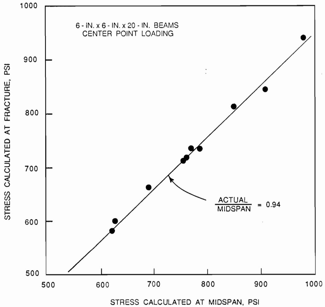
Fig. 4.28 Average modulus of rupture obtained from 6-in. x 6-in. x 20-in. beams tested in center point loading with the moment calculated at the plane of fracture versus the moment calculated at midspan.
