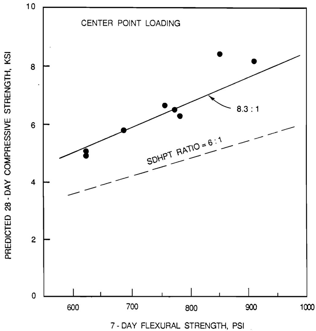
Fig. 4.30 Twenty-eight-day compressive strength versus 7-day flexural strength (center point loading).
