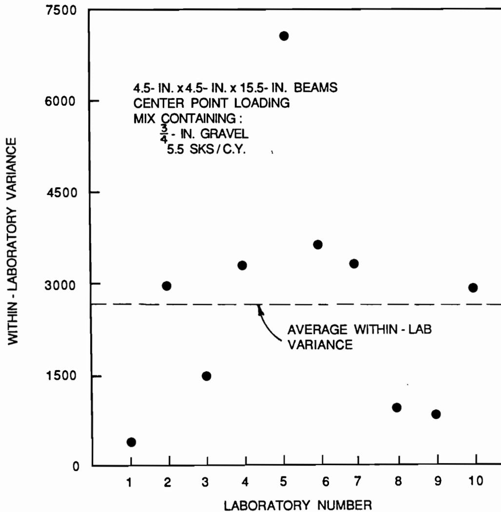
Fig. 5.12 Investigation for agreement of variances for each laboratory for test results obtained from 4.5-in. x 4.5-in. x 15.5-in. beams cast from the mix containing 3/4-in. gravel and 5.5 sacks of cement per cubic yard and tested in center point loading.
