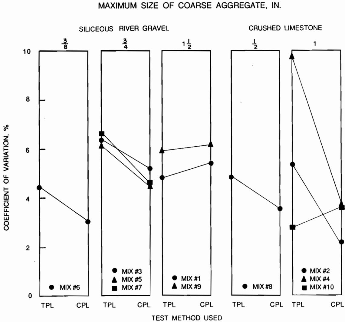
Fig. 4.26 Coefficient of variation of test results obtained from third point loading of 4.5-in. x 4.5-in. x 15.5-in. beams and center point loading of 6-in. x 6-in. x 20-in. beams for each coarse aggregate size.
