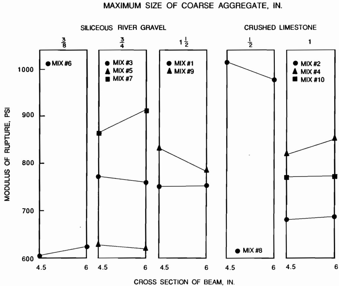
Figure 4.1 Effect of specimen dimensions on the modulus of rupture of beams loaded at their center point.
