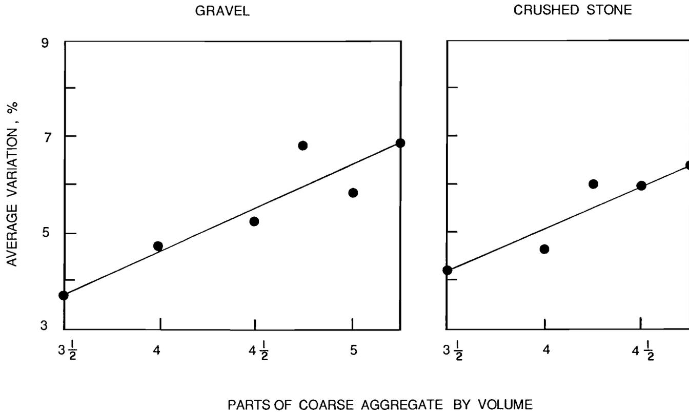
Fig. 2.10 Effect of volume of coarse aggregate on average percentage variation of test results from concrete beams loaded at their third points (after Jackson and Kellermann [4]).
