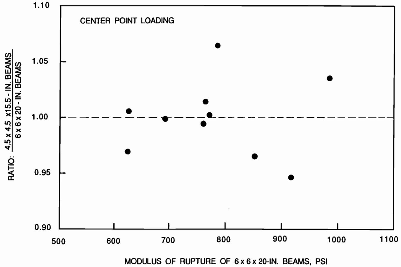
Fig. 4.5 Ratio of modulus of rupture of 4.5-in. x 4.5-in. x 15.5-in. beams to 6-in. x 6-in. x 20-in. beams, tested in center point loading, plotted versus the modulus of rupture of 6-in. x 6-in. x 20-in. beams.
