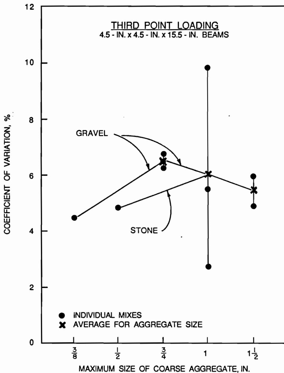
Fig. 4.16 Coefficient of variation of test results from 4.5-in. x 4.5-in. x 15.5-in. beams loaded at their third points, plotted versus coarse aggregate size.
