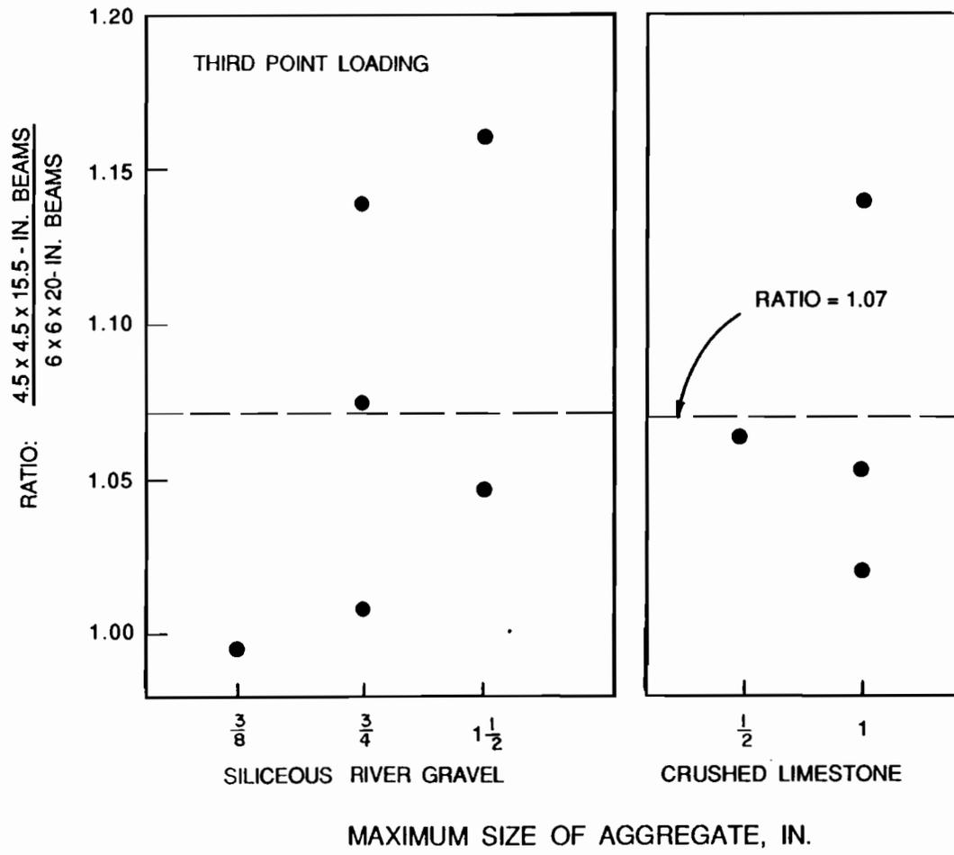
Fig. 4.12 Ratio of modulus of rupture in third point loading of 4.5-in. x 4.5-in. x 15.5-in. beams to 6-in. x 6-in. x 20-in. beams plotted versus coarse aggregate size.
