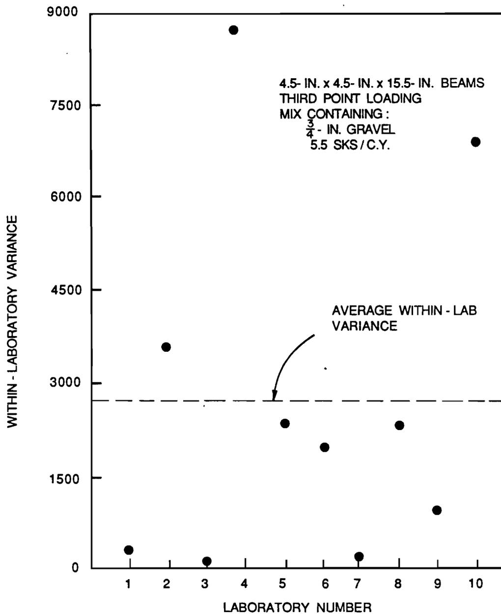
Fig. 5.17 Investigation for agreement of variances for each laboratory for test results obtained from 4.5-in. x 4.5-in. x 15.5-in. beams cast from the mix containing  $\frac{3}{4}$ -in. gravel and 5.5 sacks of cement per cubic yard and tested in third point loading.
