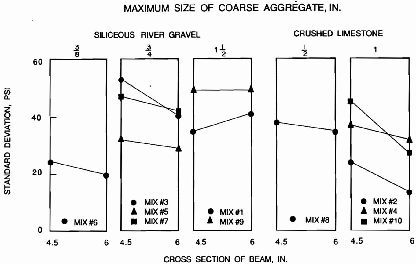
Fig. 4.2 Effect of specimen dimensions on the standard deviation of test results from beams loaded at their center point.
