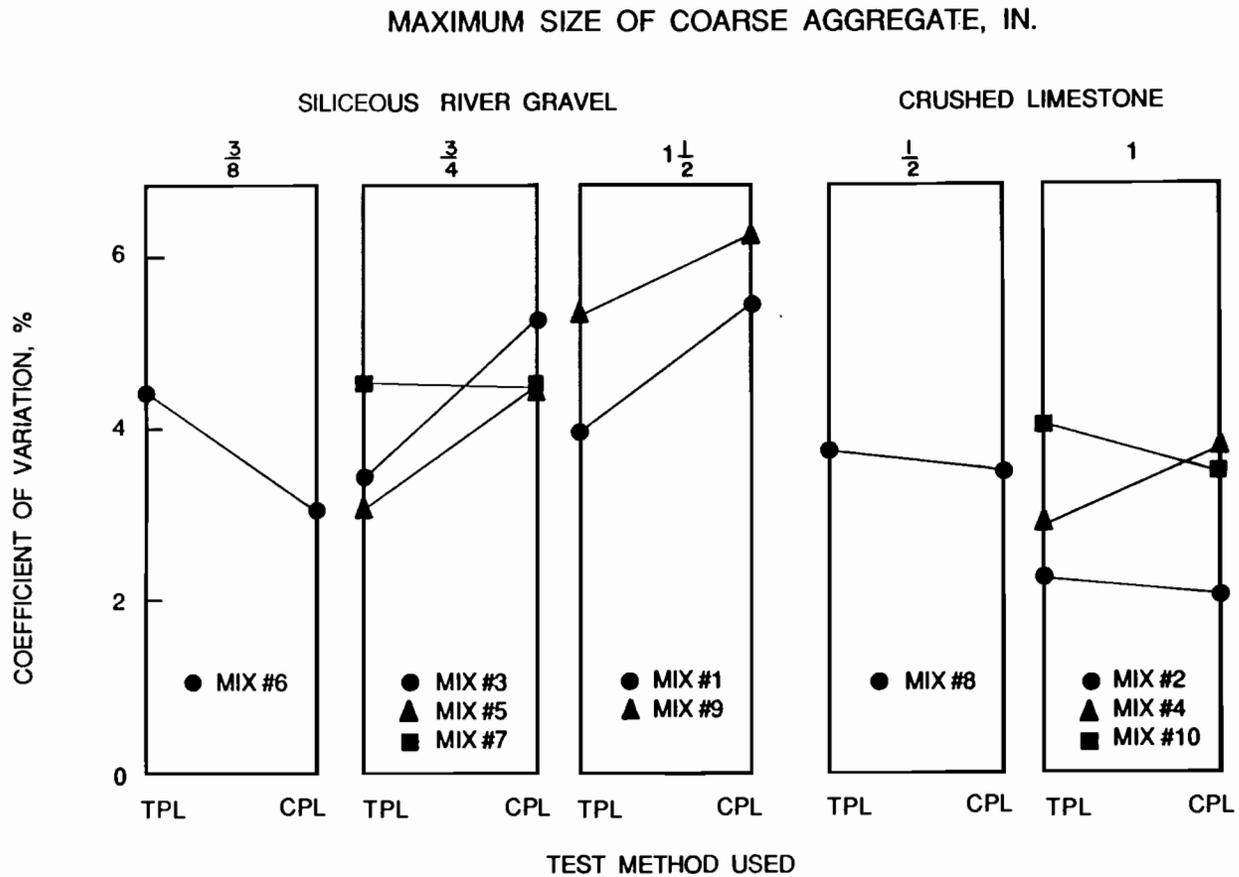
Fig. 4.21 Coefficient of variation of 6-in. x 6-in. x 20-in. beams tested in third point loading versus center point loading for each aggregate size.
