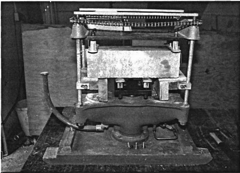
Fig. 3.3 Modification of Rainhart Beam Tester to accommodate 4.5-in. x 4.5-in. x 15.5-in. beams; third point loading head shown.
