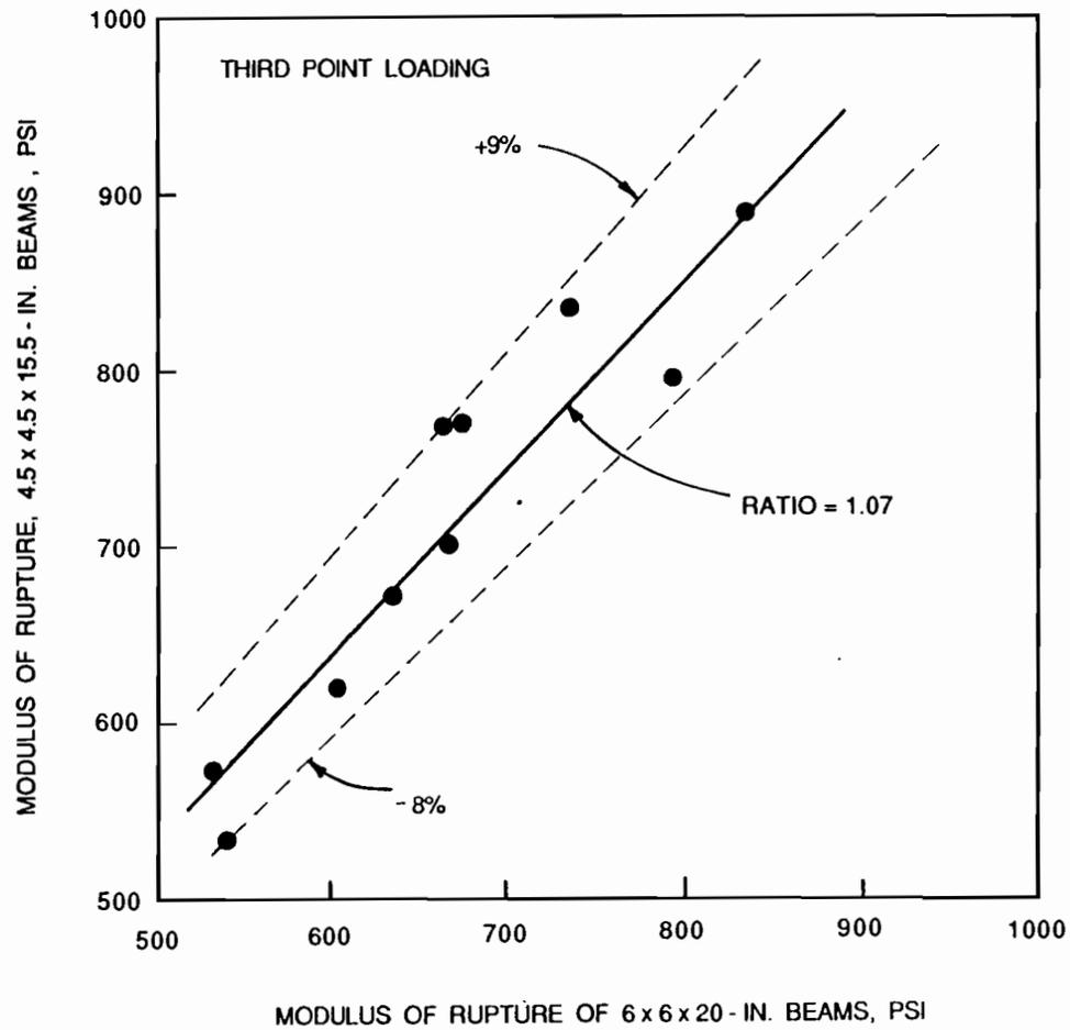
Fig. 4.10 Modulus of rupture in third point loading of 4.5-in. x 4.5-in. x 15.5-in. beams versus that of 6-in. x 6-in. x 20-in. beams.
