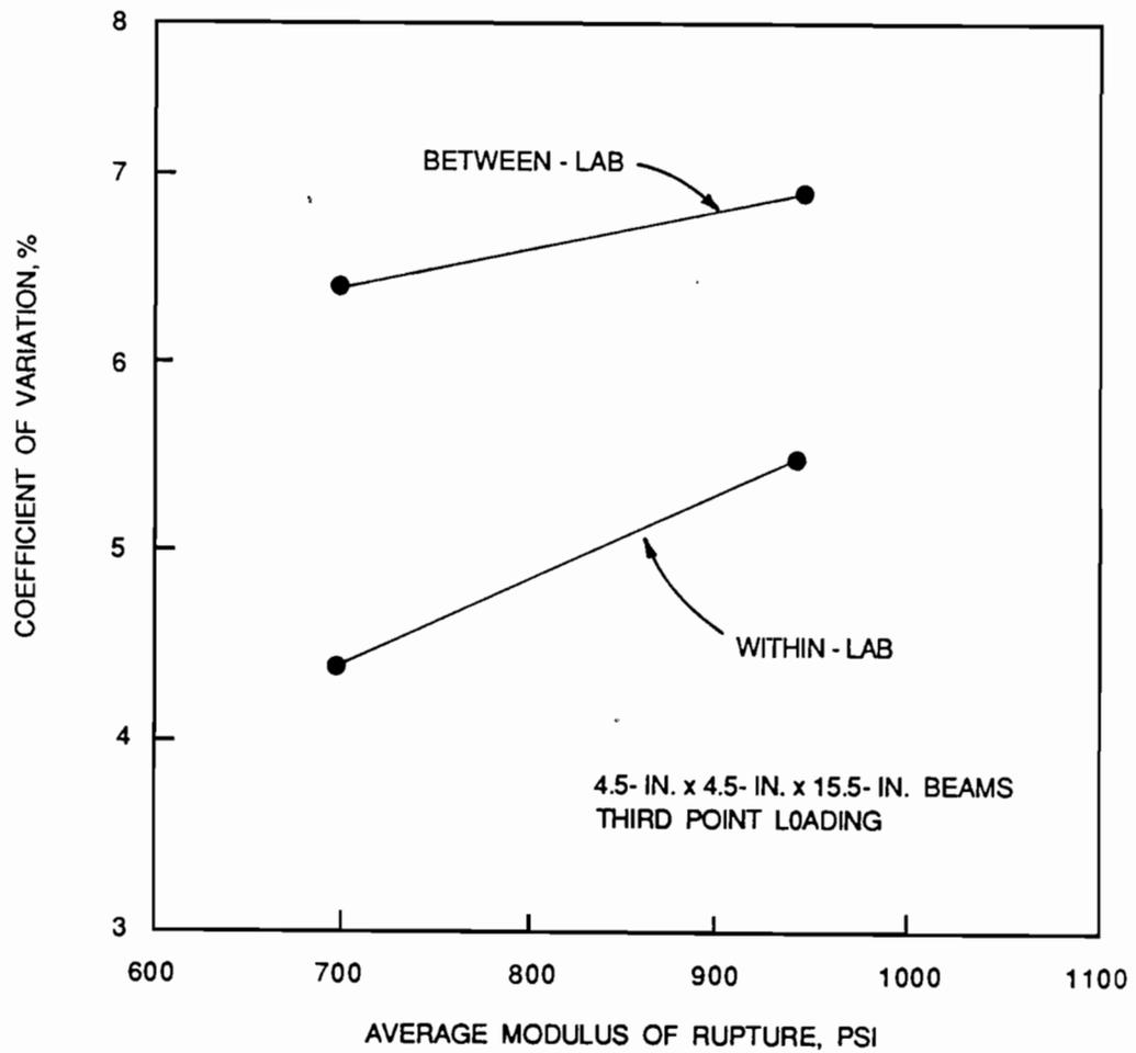
Fig. 5.20 Coefficient of variation versus average modulus of rupture for 4.5-in. x 4.5-in. x 15.5-in. beams tested in third point loading.
