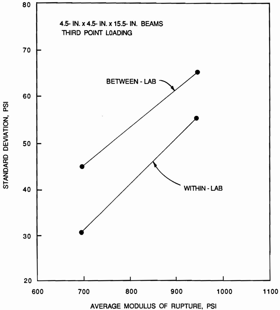
Fig. 5.19 Standard deviation versus average modulus of rupture for 4.5-in. x 4.5-in x 15.5-in. beams tested in third point loading.
