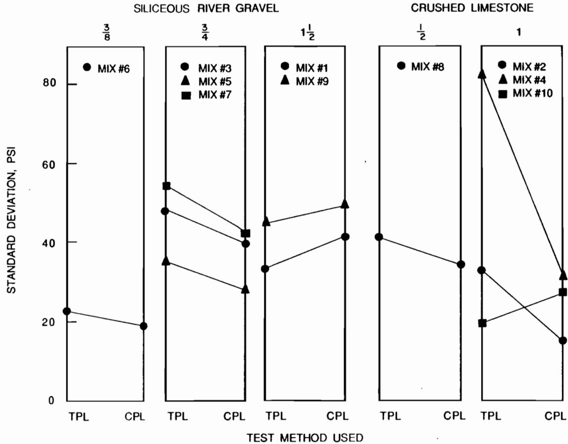
Fig. 4.25 Standard deviation of test results obtained from third point loading of 4.5-in. x 4.5-in. x 15.5-in. beams and center point loading of 6-in. x 6-in. x 20-in. beams for each coarse aggregate size.
