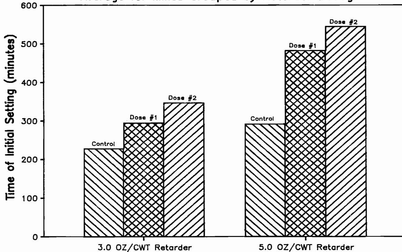
Fig. 5.23 Summary of average initial setting times for control and both superplasticizer dosage specimens for the nine laboratory mixes grouped by retarder dosage
