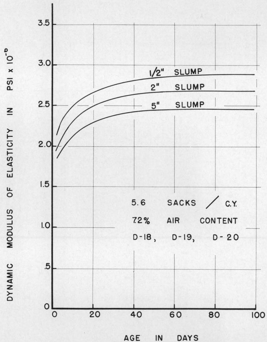
Figure 30. Effect of water content on modulus of elasticity.
