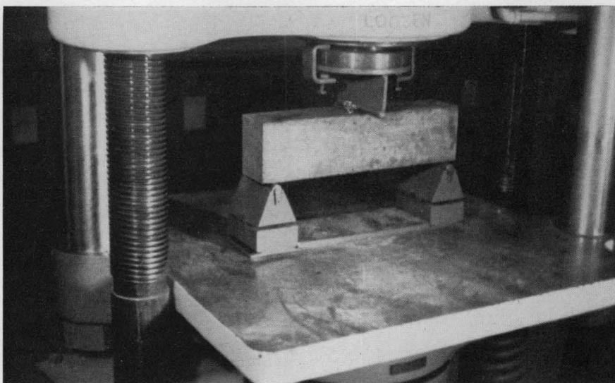
Figure 5. Modulus of rupture test with center point load.
