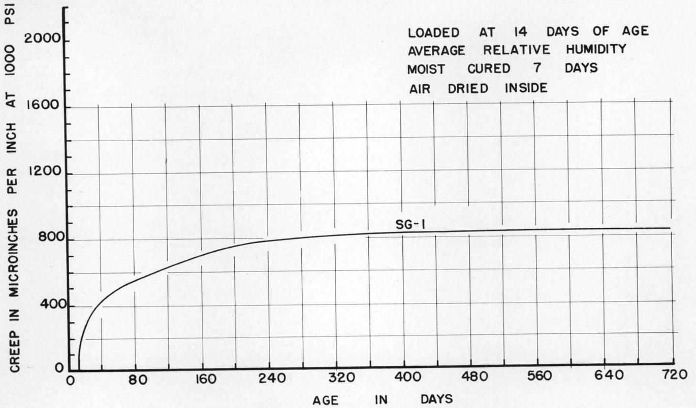
Figure 35. Creep of Hearne sand and gravel concrete at 1000 psi.
