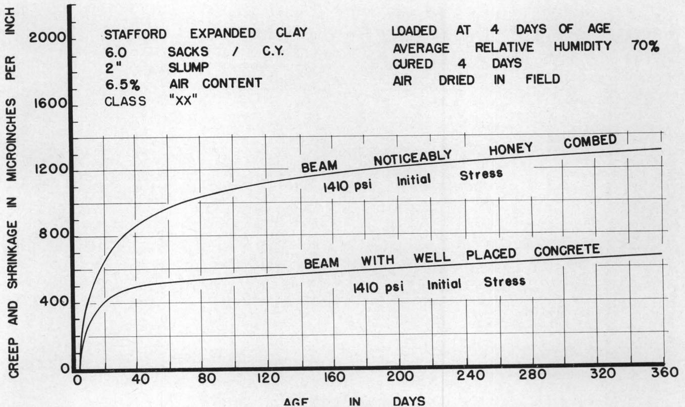
Figure 48. Effect of honey combing on creep and shrinkage of bridge beams.
