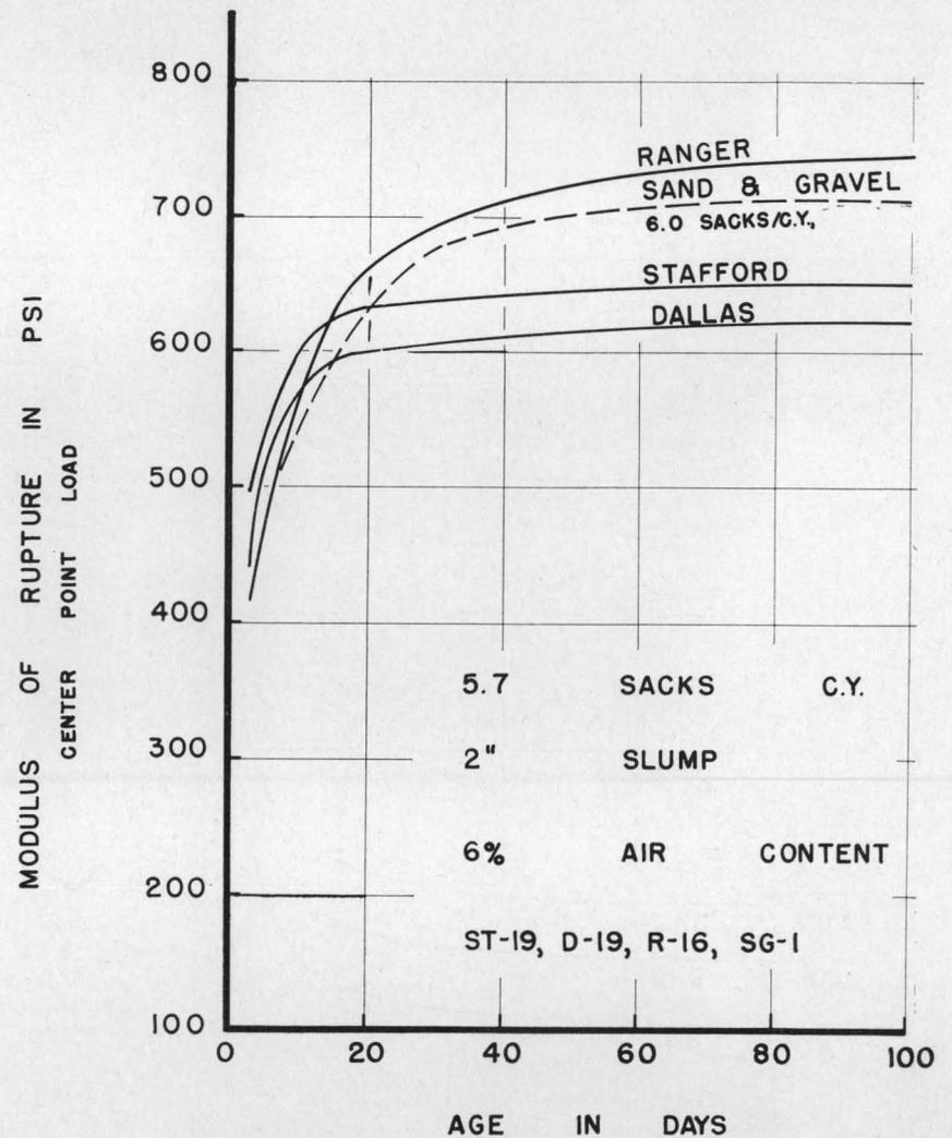
Figure 22. Effect of aggregate type on modulus of rupture.
