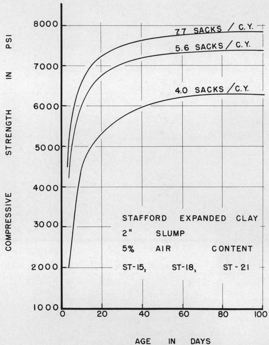
Figure 18. Effect of cement content on compressive strength.
