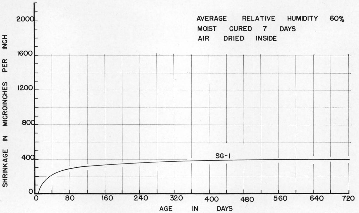
Figure 39. Shrinkage of Hearne sand and gravel concrete.
