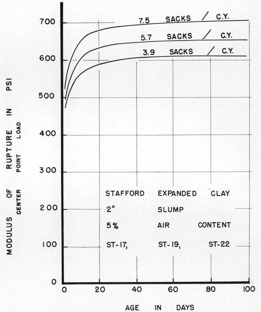
Figure 24. Effect of cement content on modulus of rupture.
