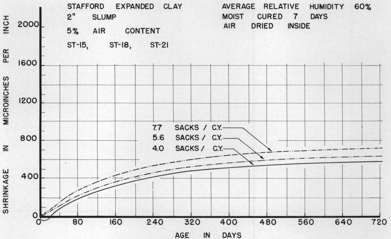
Figure 42. Effect of cement on shrinkage of concrete.
