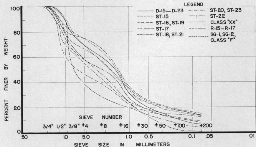
Figure 15. Gradation curves for aggregate in concrete batches.
