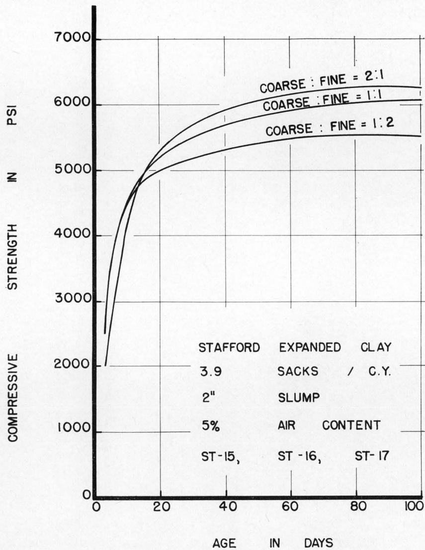
Figure 17. Effect of aggregate gradation on compressive strength.
