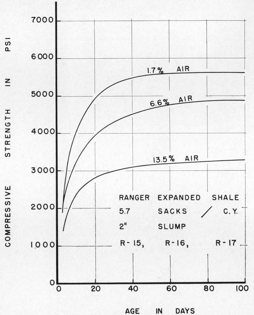
Figure 20. Effect of air content on compressive strength.
