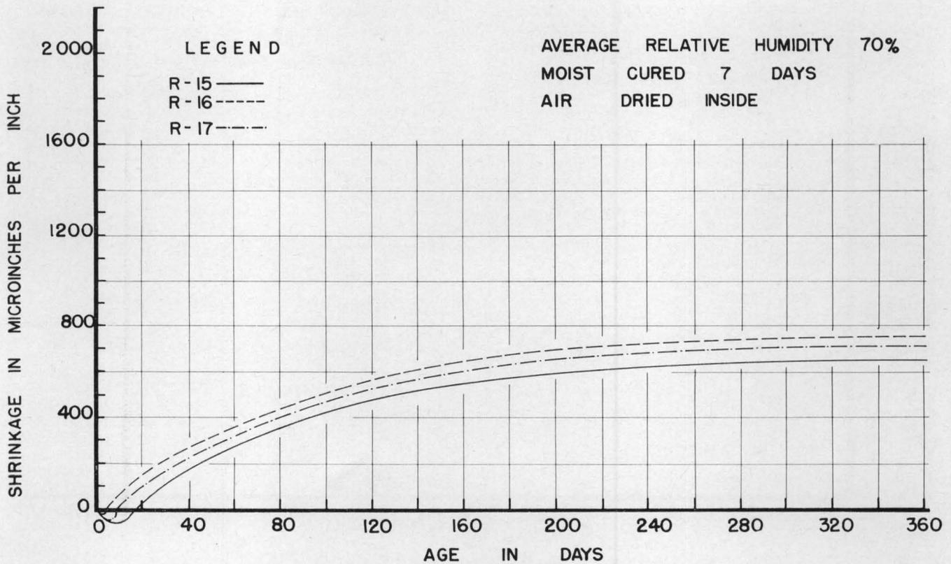
Figure 38. Shrinkage of Ranger expanded shale aggregate concrete.
