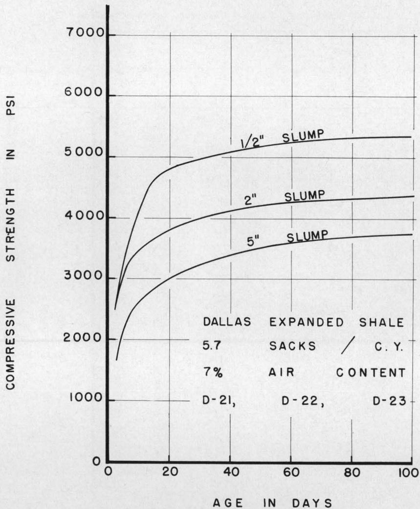
Figure 19. Effect of water content on compressive strength.
