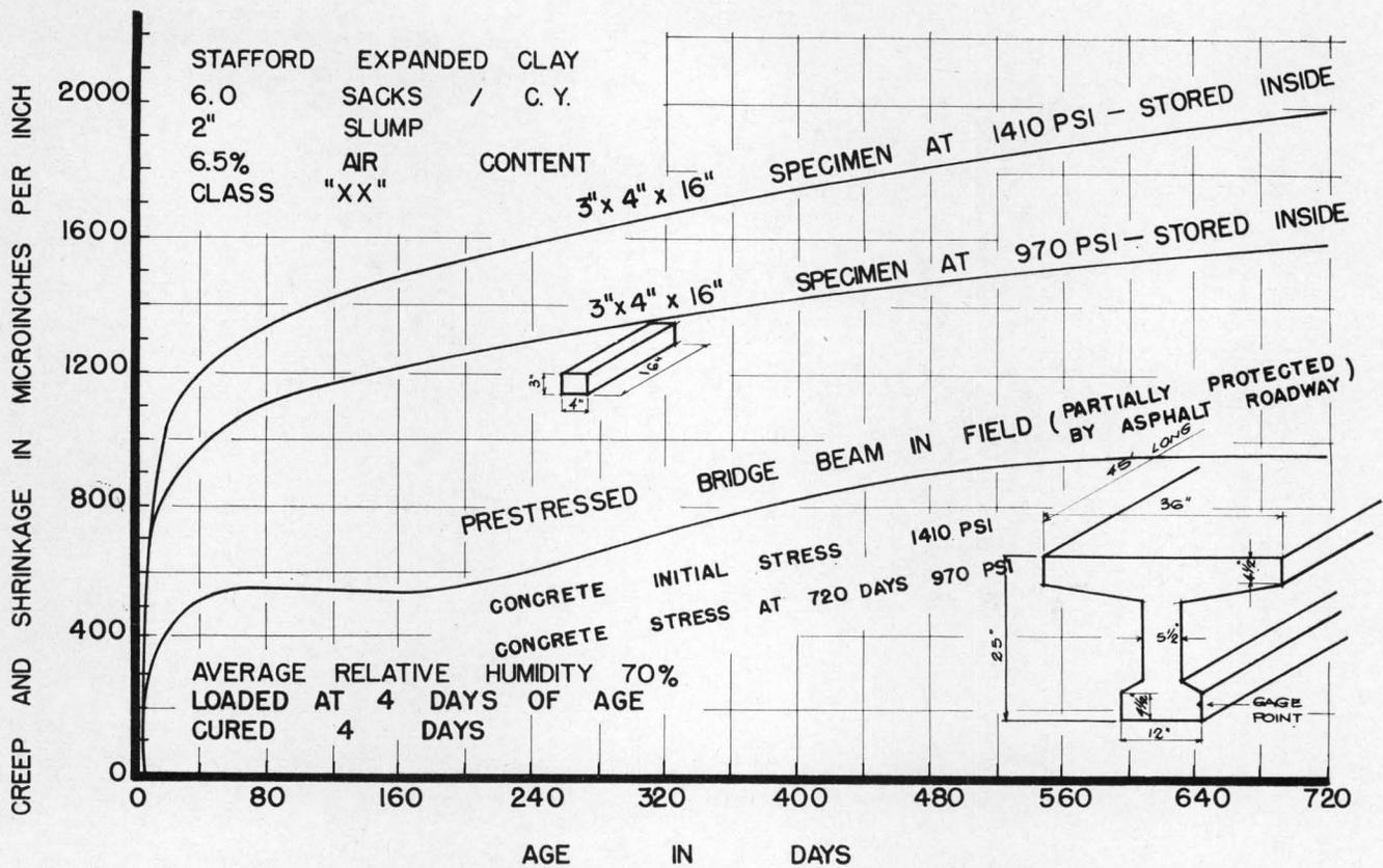
Figure 55. Comparison of creep plus shrinkage of laboratory specimen to that of prototype prestressed bridge beam.
