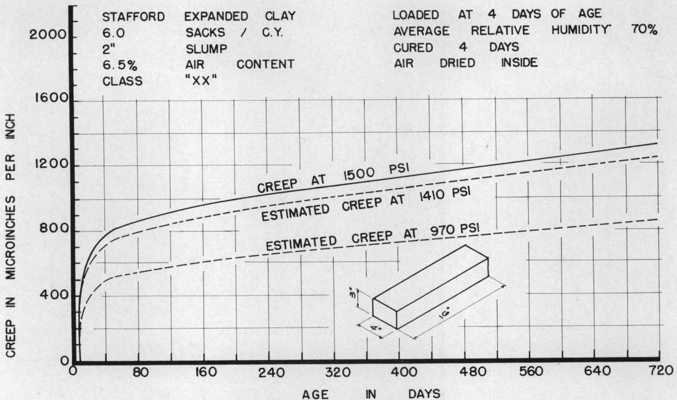
Figure 57. Creep laboratory specimens of concrete used in prototype prestressed bridge beams.
