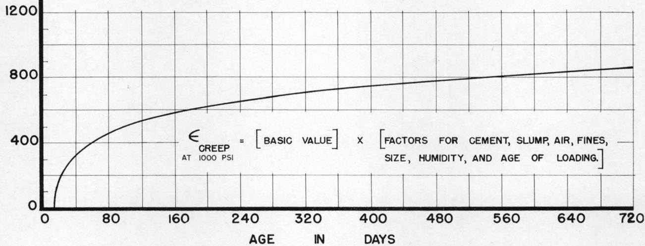
Figure 65. Basic curve for estimating creep of concrete made with expanded clay and shale aggregate.
