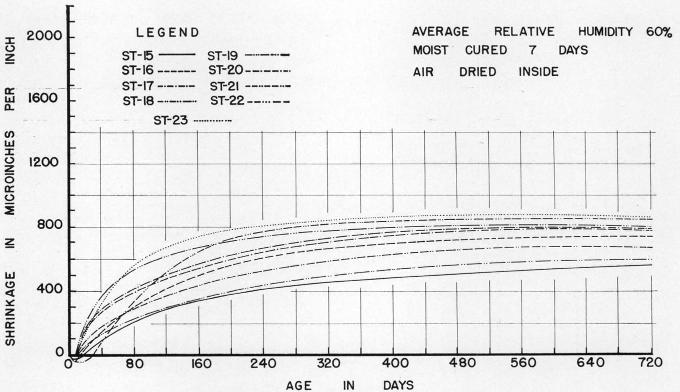
Figure 36. Shrinkage of Stafford expanded clay aggregate concrete.
