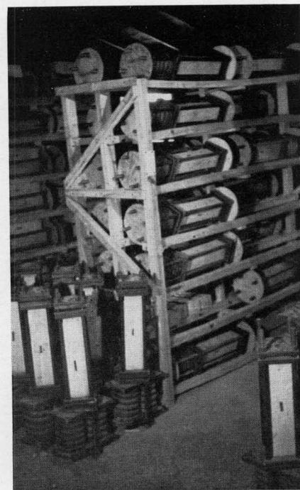
Figure 11. Creep and shrinkage specimens air dried inside. Specimens with double springs are loaded to 3000 psi.
