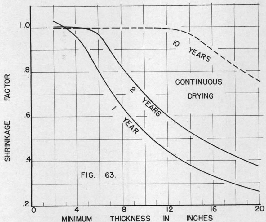
Figure 63. Shrinkage factor for minimum thickness in inches.
