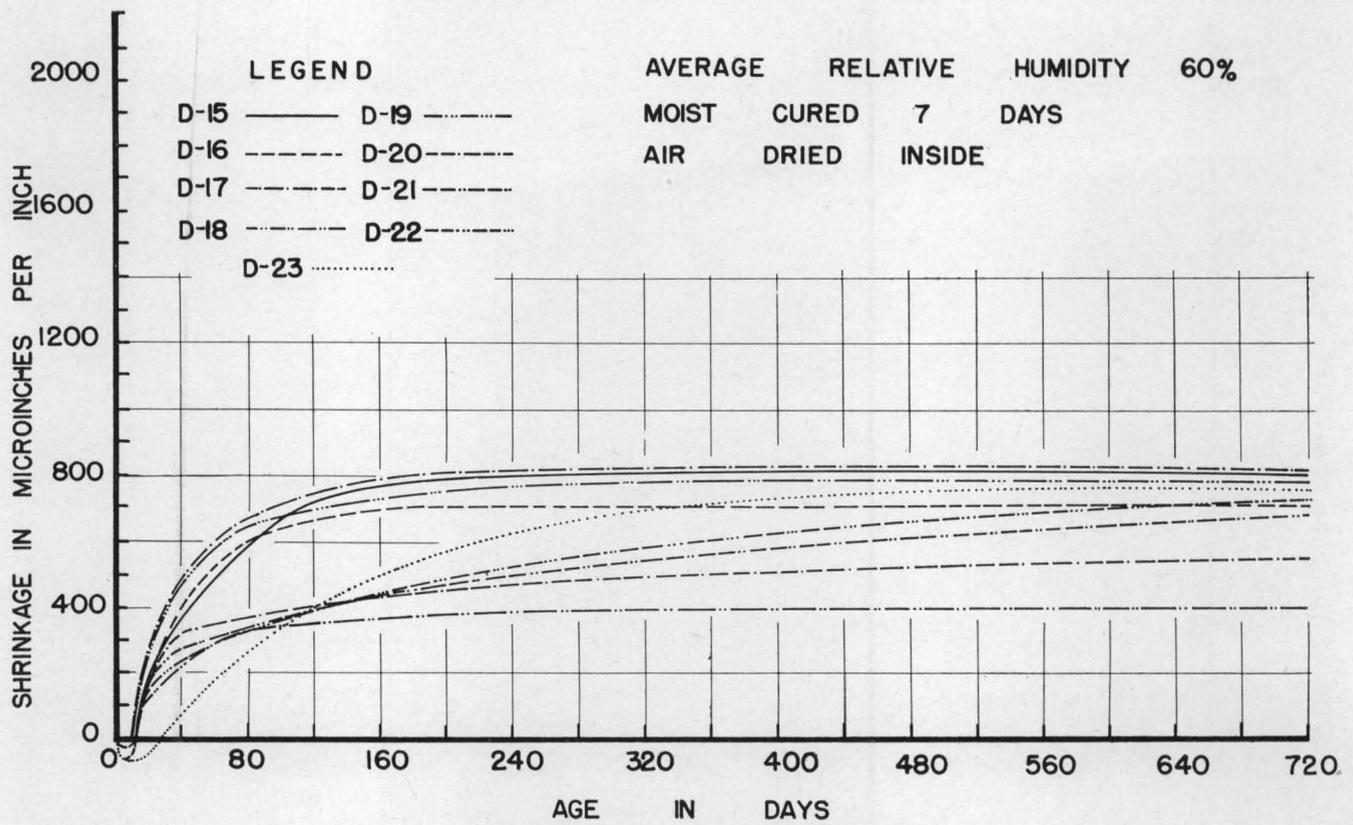
Figure 37. Shrinkage of Dallas expanded shale aggregate concrete.
