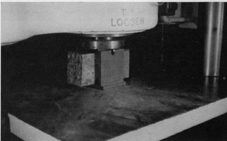
Figure 6. Steel loading device used in modified cube compressive test.
