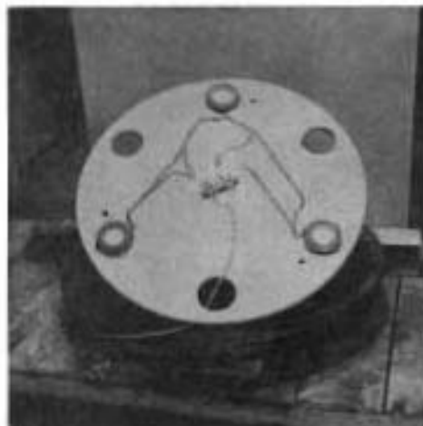
b. Wiring of Bridge
