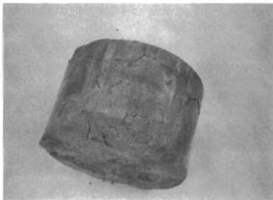
b. Partially Dried Section Showing Fissure Planes
