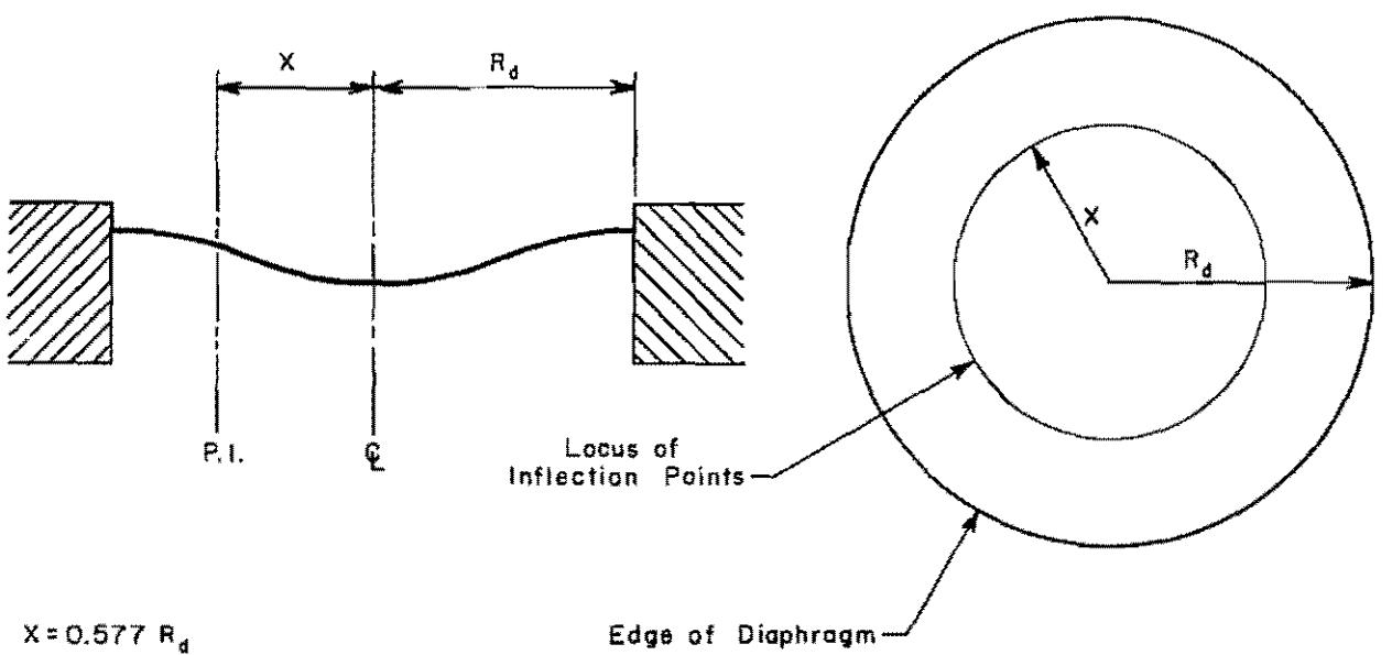
Fig 7. Clamped-edge-diaphragm behavior under uniform load.
