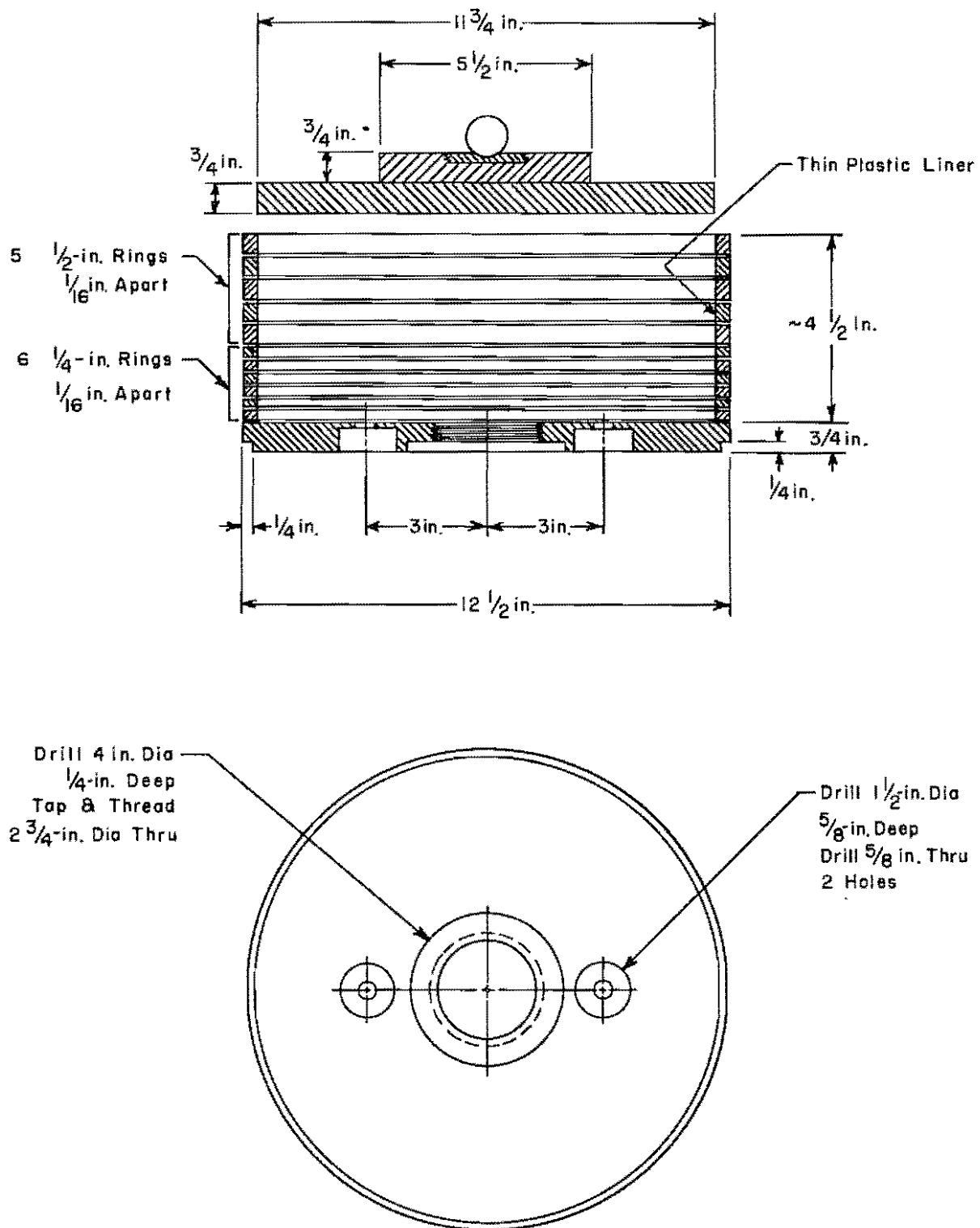
Fig 29. Rings and baseplate assembly for soil-column test.
