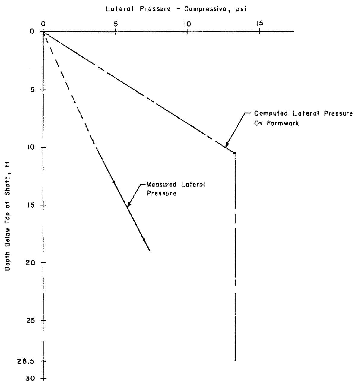
Fig 41. Lateral pressure distribution immediately after pouring, January 18, 1967.
