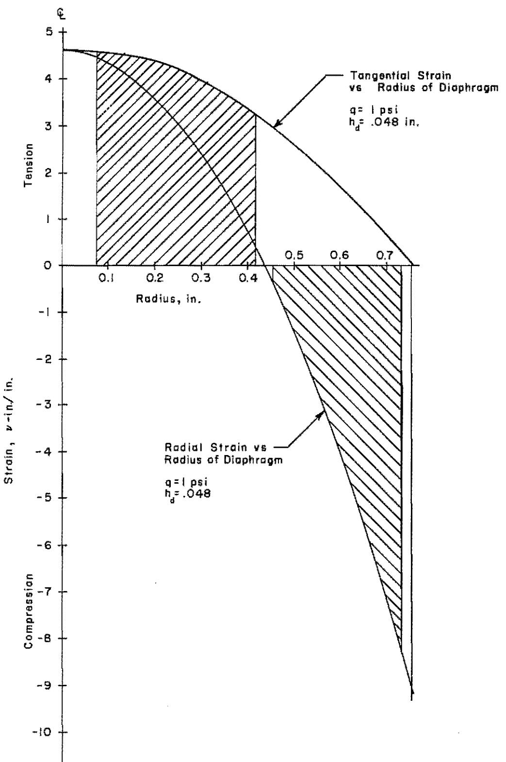
Fig 9. Graphical representation of strains measured by diaphragm strain gage.
