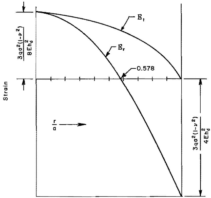
Distribution of Radial and Tangential Strain on Uniformly Loaded Circular Diaphragm with Clamped Edges
