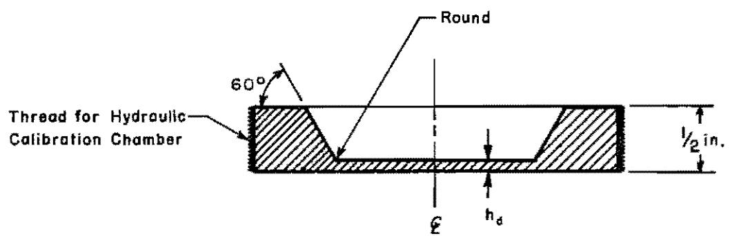
Fig 6. The WT lateral earth-pressure cell.
