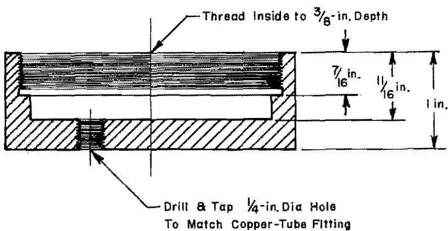
Fig 17. Hydraulic calibration chamber.
