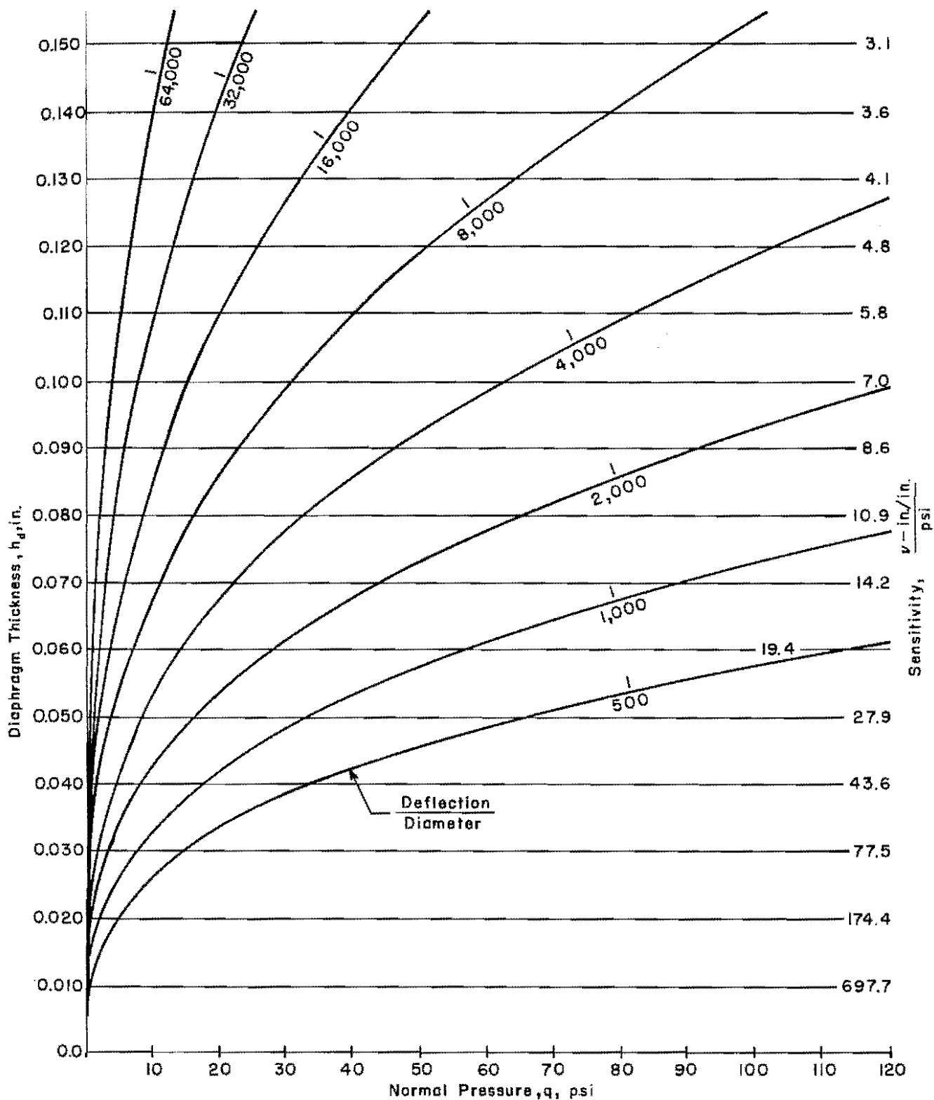
Circular Diaphragm, Clamped Edges
