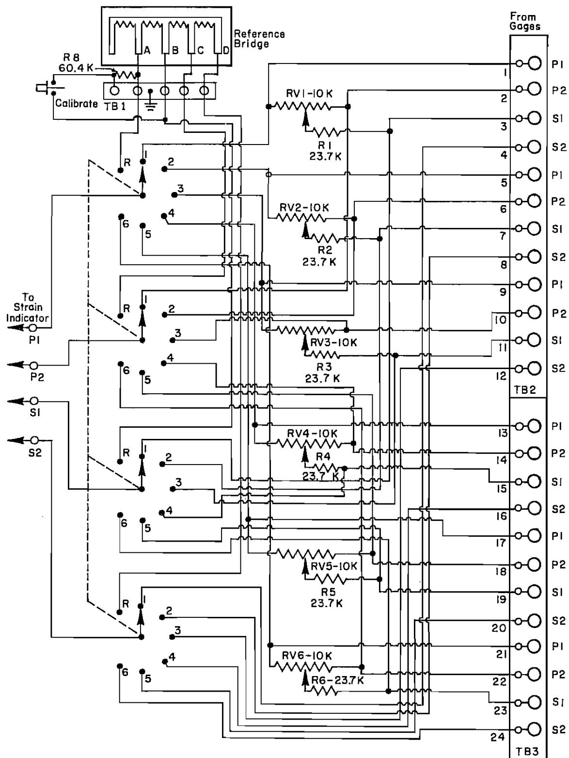
Fig C.1. Six-channel switch and balance unit.
