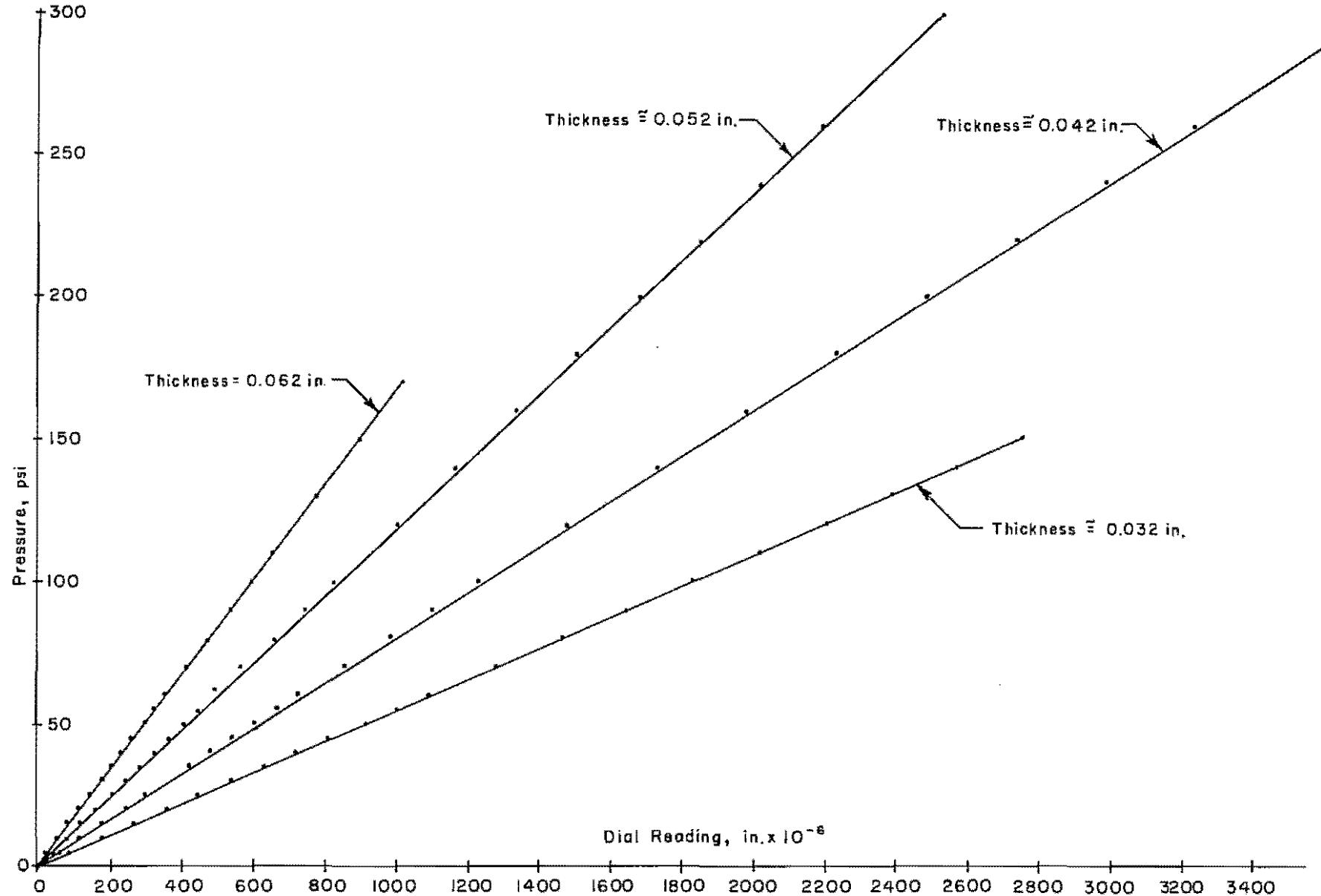
Fig 14. Calibration curves for steel test cell.
