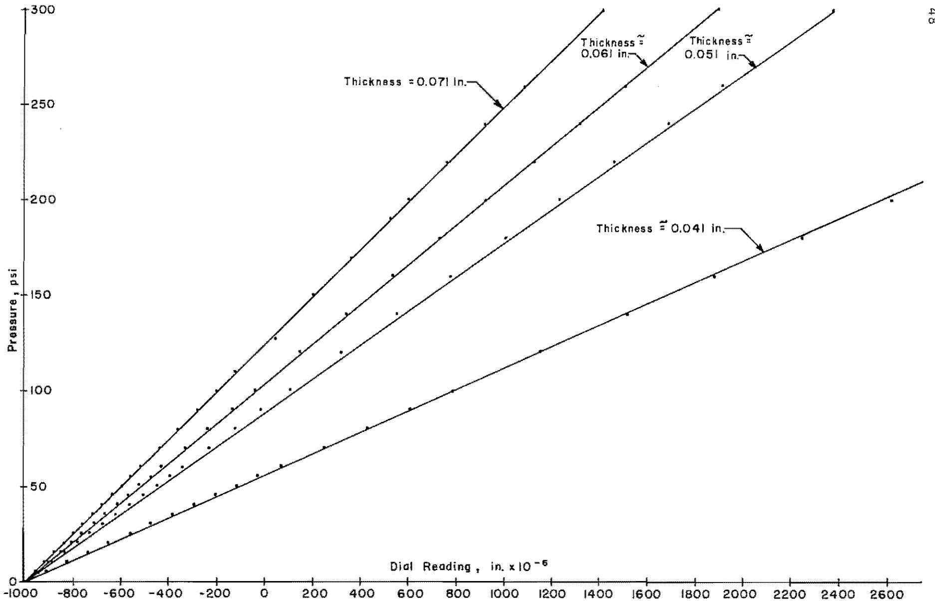
Fig 13. Calibration curves for beryllium-copper test Cell No. 1.
