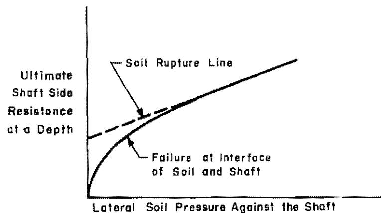
Fig 2b. Ultimate shaft side resistance at a depth as affected by the lateral soil pressure against the shaft.
