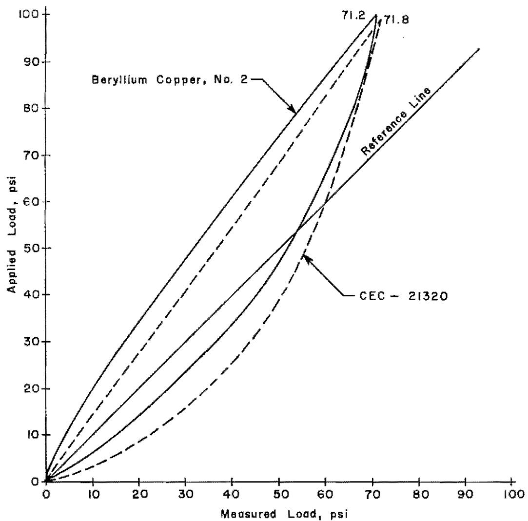
Fig 30. Plot of applied pressure versus measured pressure at base of sand column.
