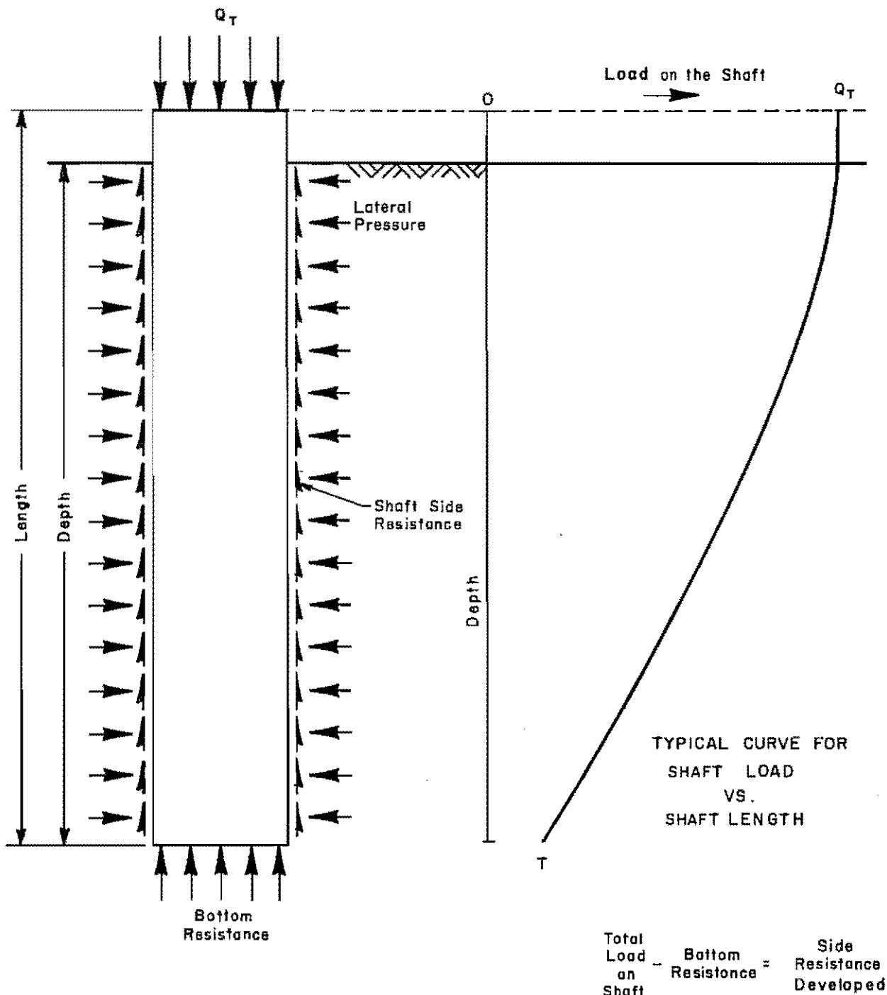
Fig 1. Typical load transfer curve for a drilled shaft.
