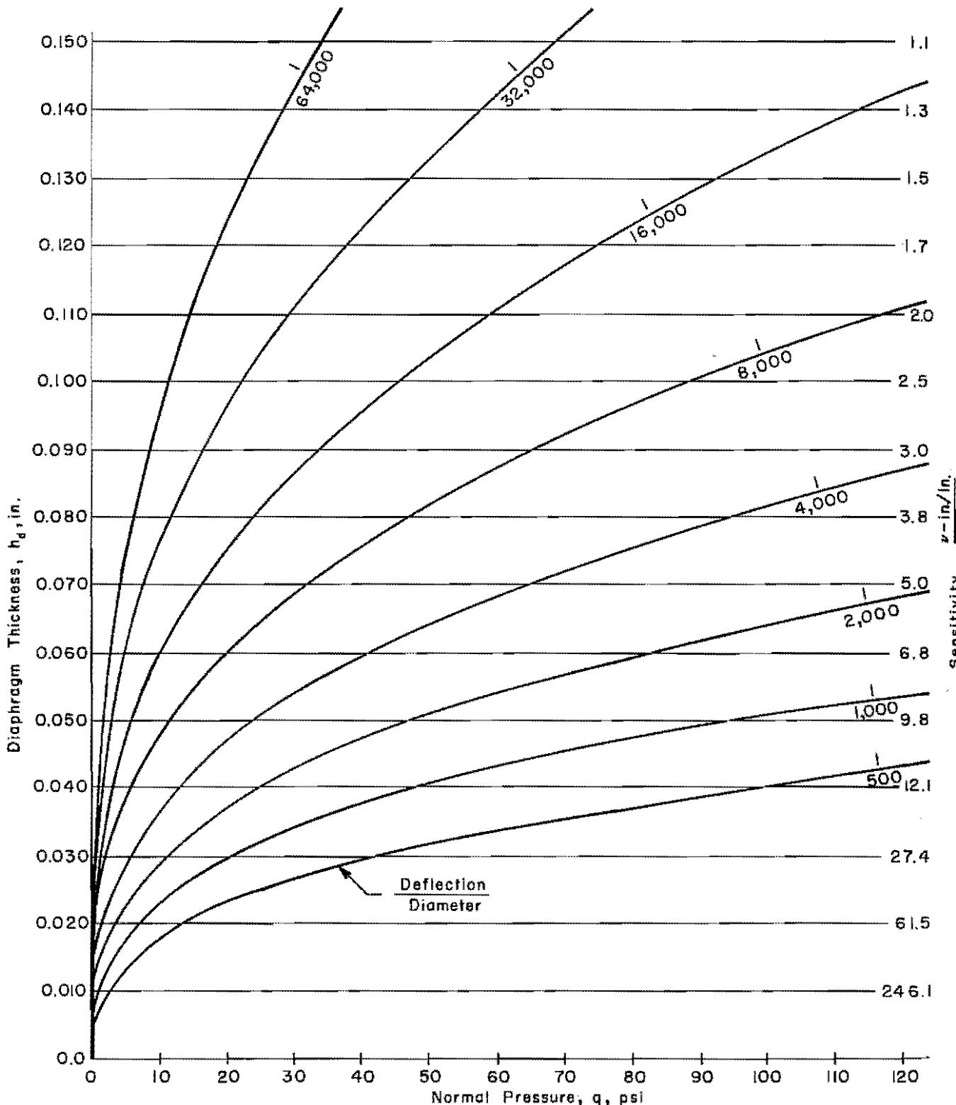
Circular Diaphragm, Clamped Edges
