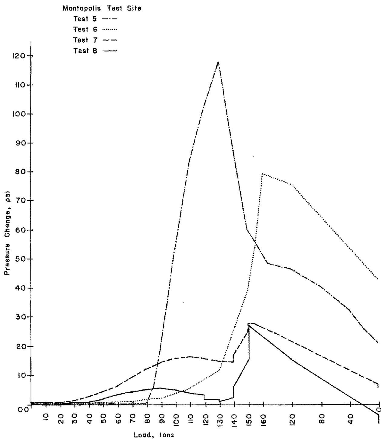
Fig D. 1. Behavior of Cell No. 5 during load tests at 10-foot depth in Austin shaft.
