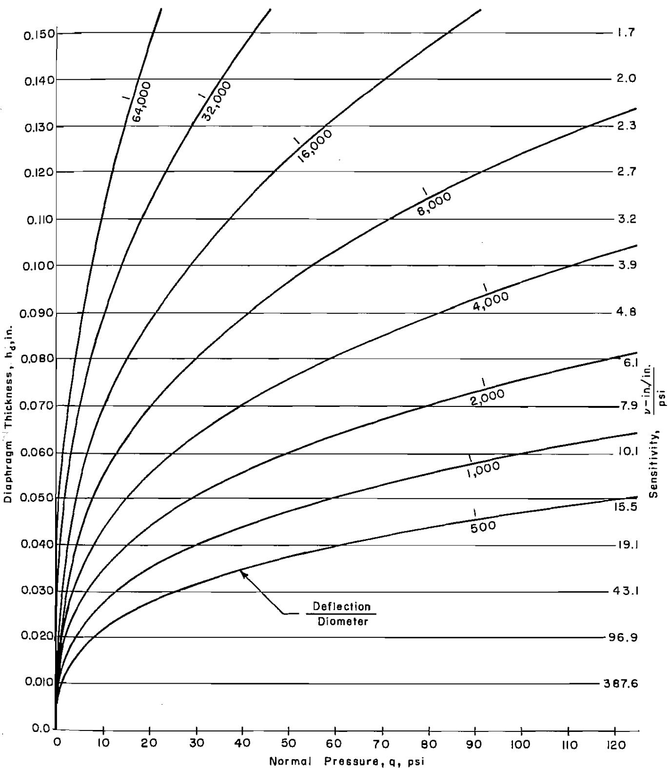
Circular Diaphragm, Clamped Edges
