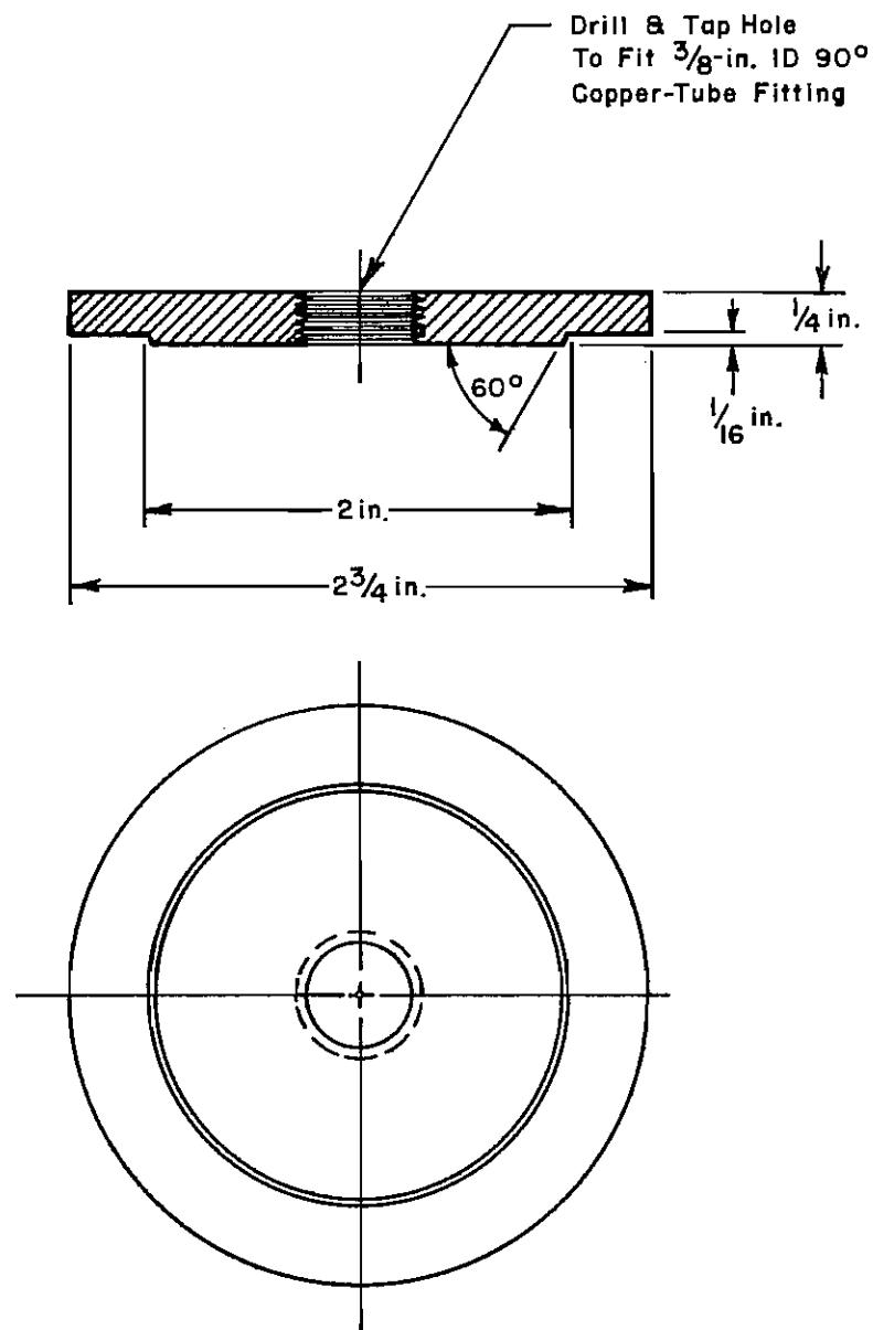
Fig 34. Back coverplate for UT cell.
