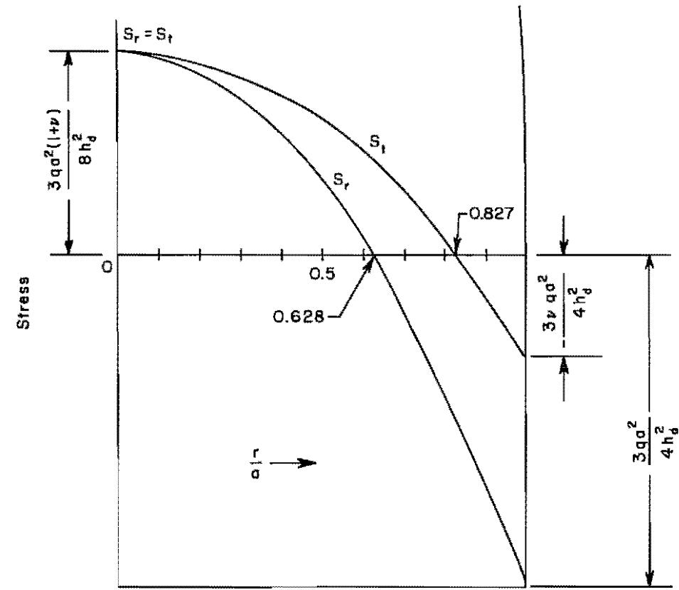
Variation of Radial and Tangential Stresses Along Radius of Uniformly Loaded Circular Diaphragm with Clamped Edges
