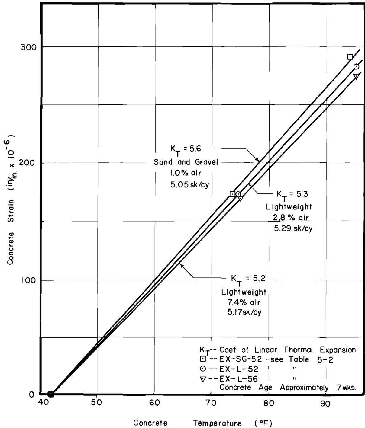
Figure 3-1. Concrete Strain — Temperature Properties of Normal Weight and Lightweight Concretes
