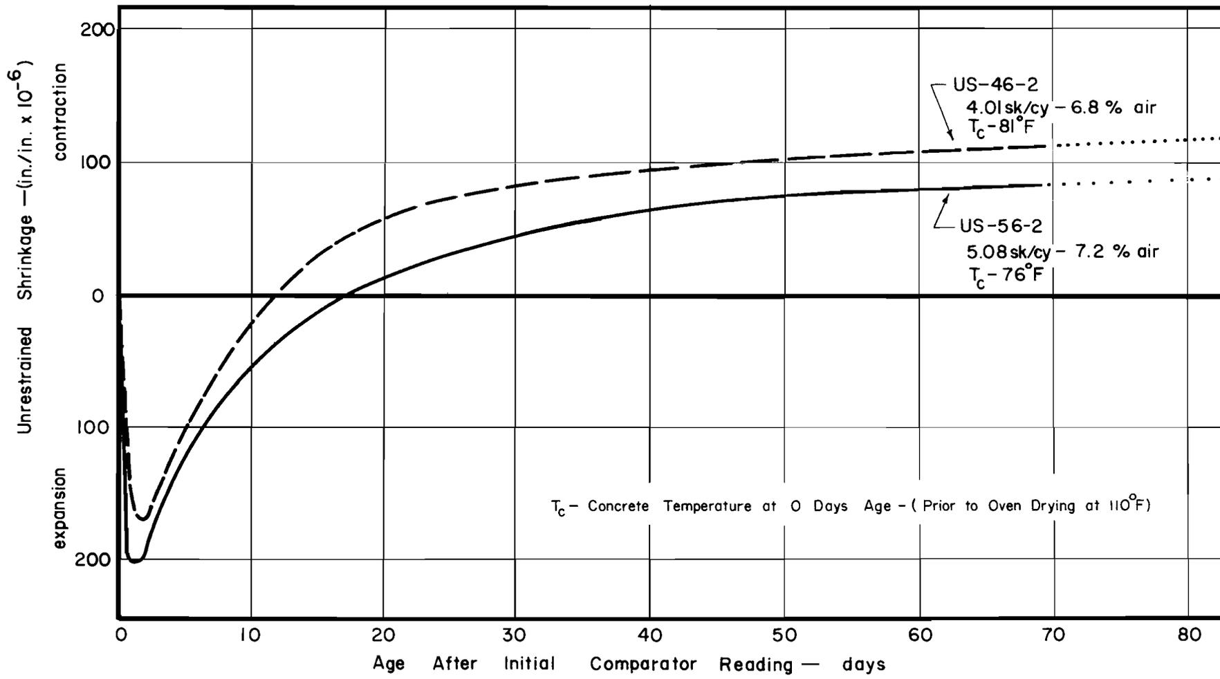
Figure 3-2. Unrestrained Shrinkage — Age After Approximately One Day for Oven Cured Lightweight Concrete
