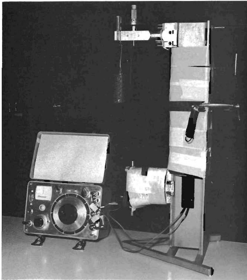
Fig. 2-2. Over-All View of Comparator and Strain Indicator
