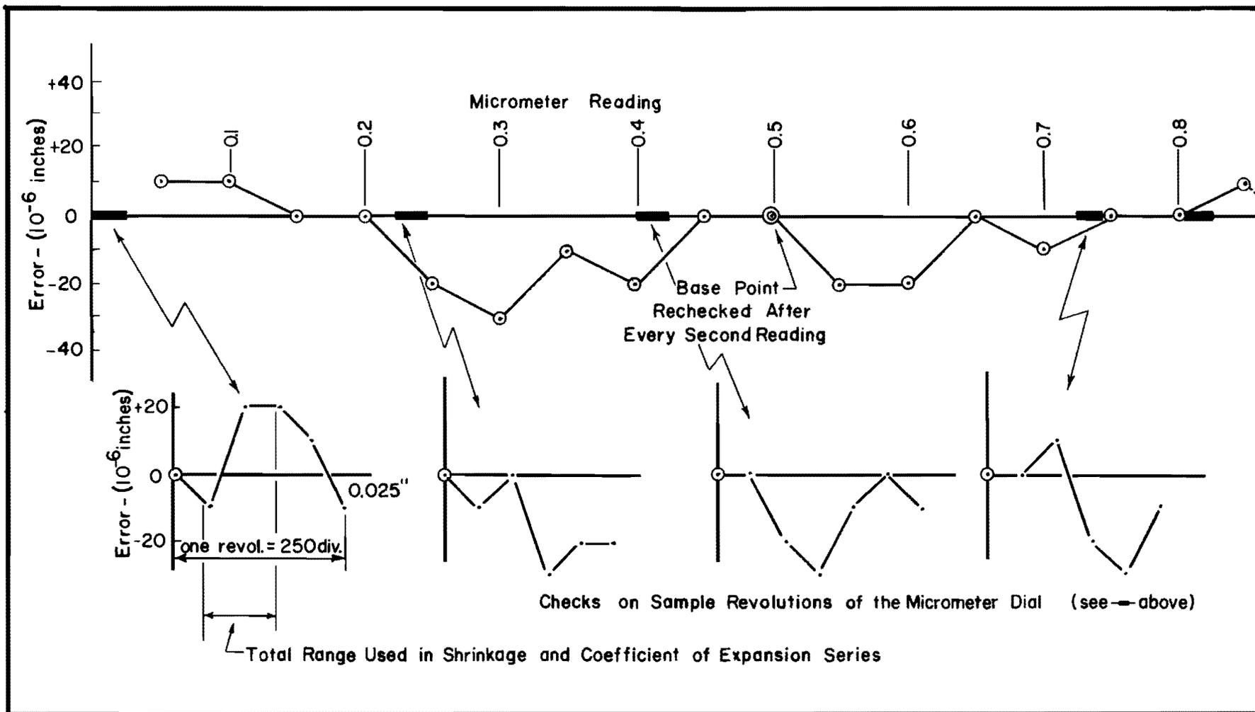
Figure 2-13. Micrometer Calibration Curves by Matlock
