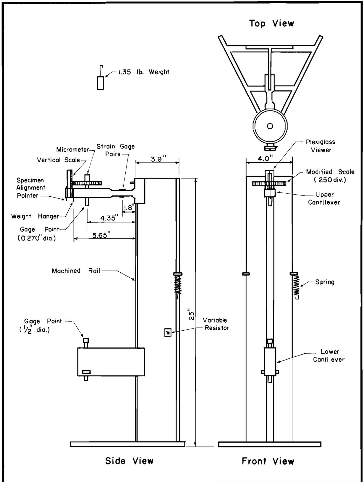
Figure 2-1. Comparator Measuring System
