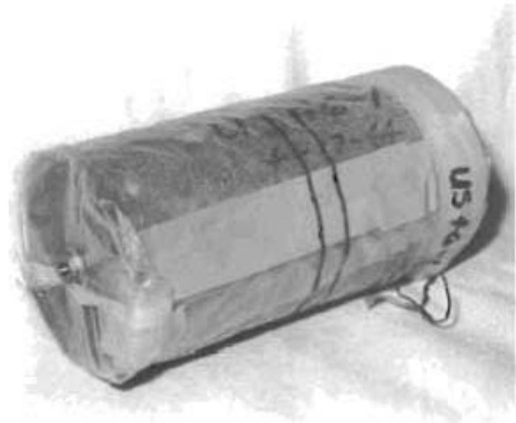
Fig. 5-6. Bag-Cured Unrestrained Shrinkage Specimen
