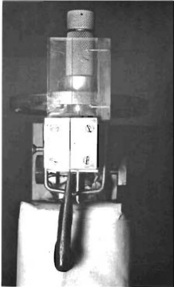
Fig. 2-9. Alignment of Standard Bar
