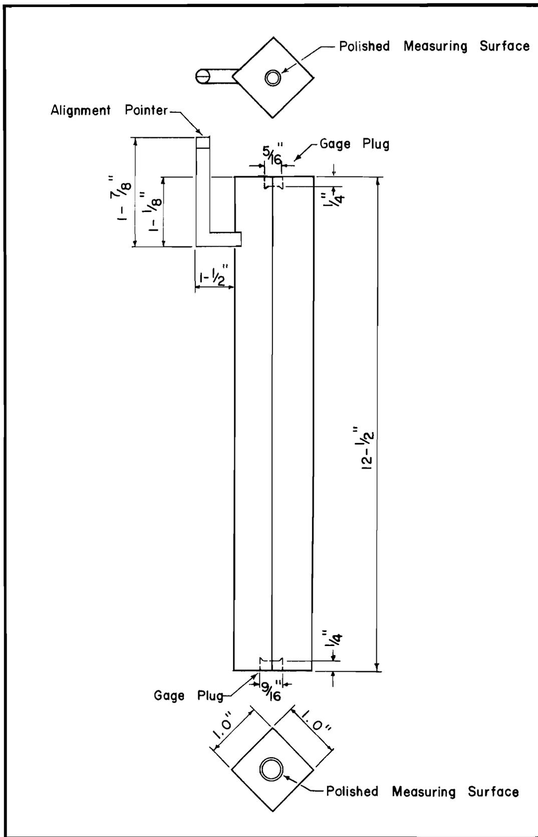
Figure 2-6. Standard Bar with Alignment Device
