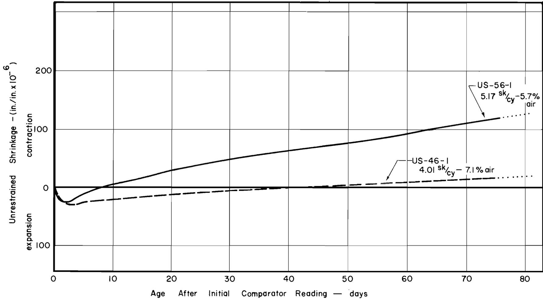
Figure 3-3. Unrestrained Shrinkage - Age After Approximately One Day for Bag Cured Lightweight Concrete
