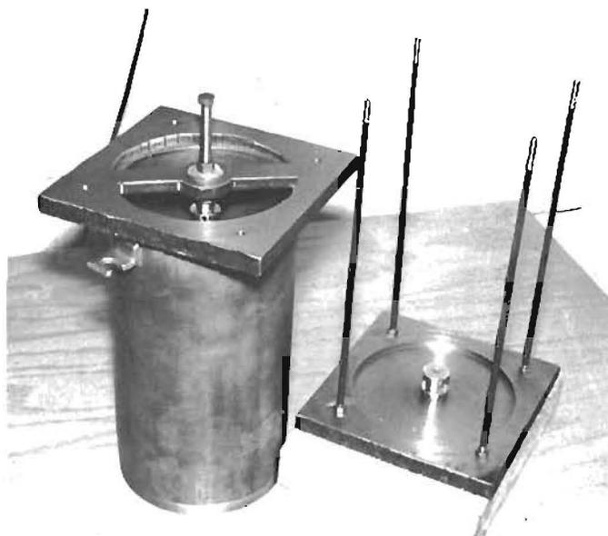
Fig. 5-2. Special Mold Used to Form Shrinkage and Coefficient-of-Expansion Specimen
