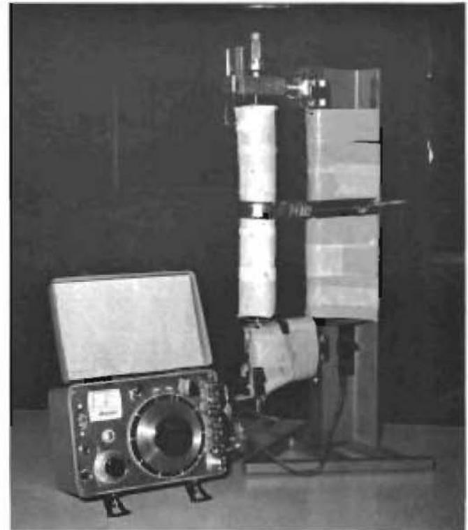
Fig. 2-10. Band-Spring Method of Applying Constant Horizontal Pressure to Standard Bar
