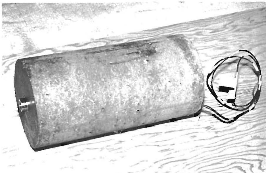
Fig. 5-1. Typical Shrinkage or Coefficient-of-Expansion Specimen
