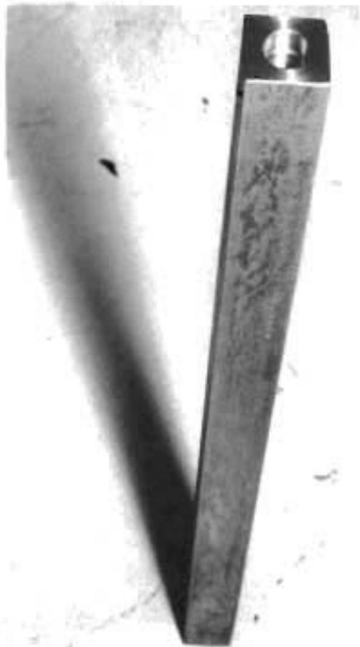
Fig. 2-7. View of Standard Bar Showing Polished Gage Plug
