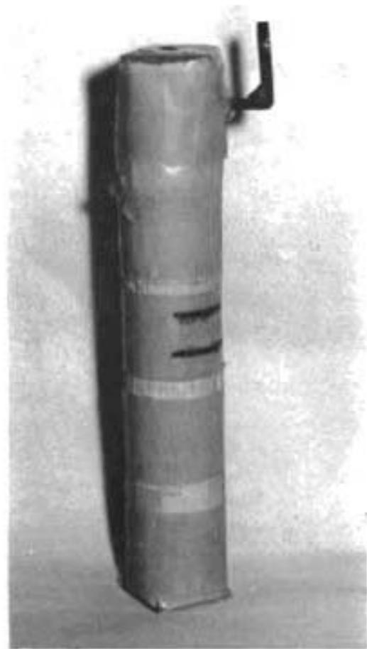
Fig. 2-8. Fiberglass Insulation of Standard Bar 15
