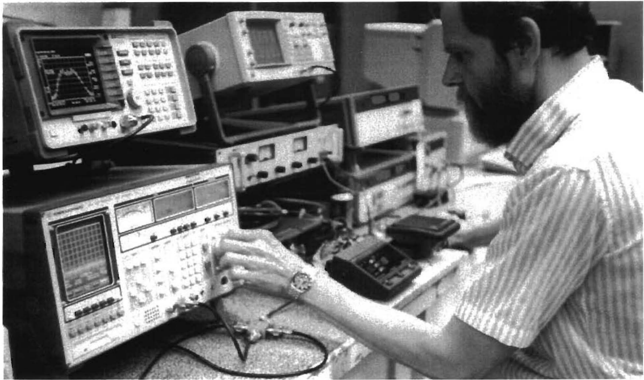
Figure 3. Laboratory evaluation of RF noise with EMI receiver and FM radio
