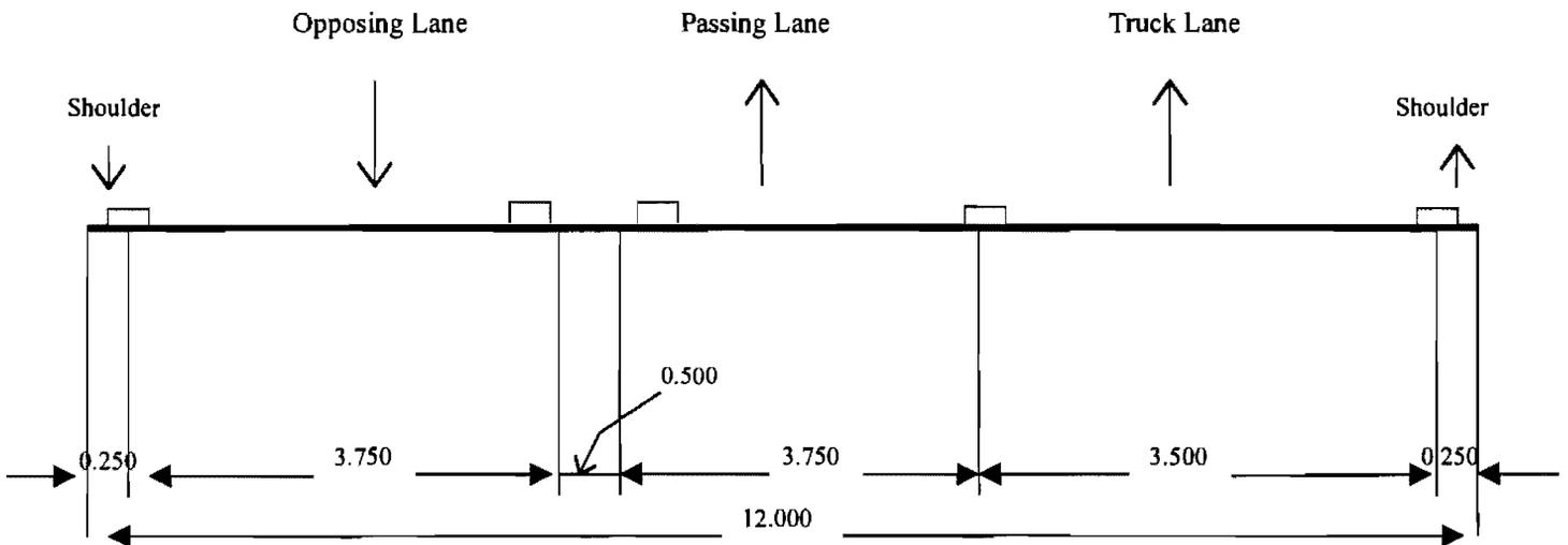
**Figure 2-3:** Three Lane Highway Cross Section in Germany
