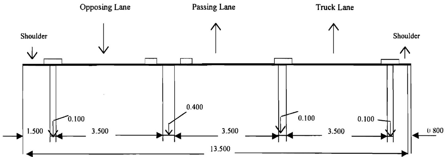
**Figure 2-4: Three Lane Highway Cross Section in Mexico**
