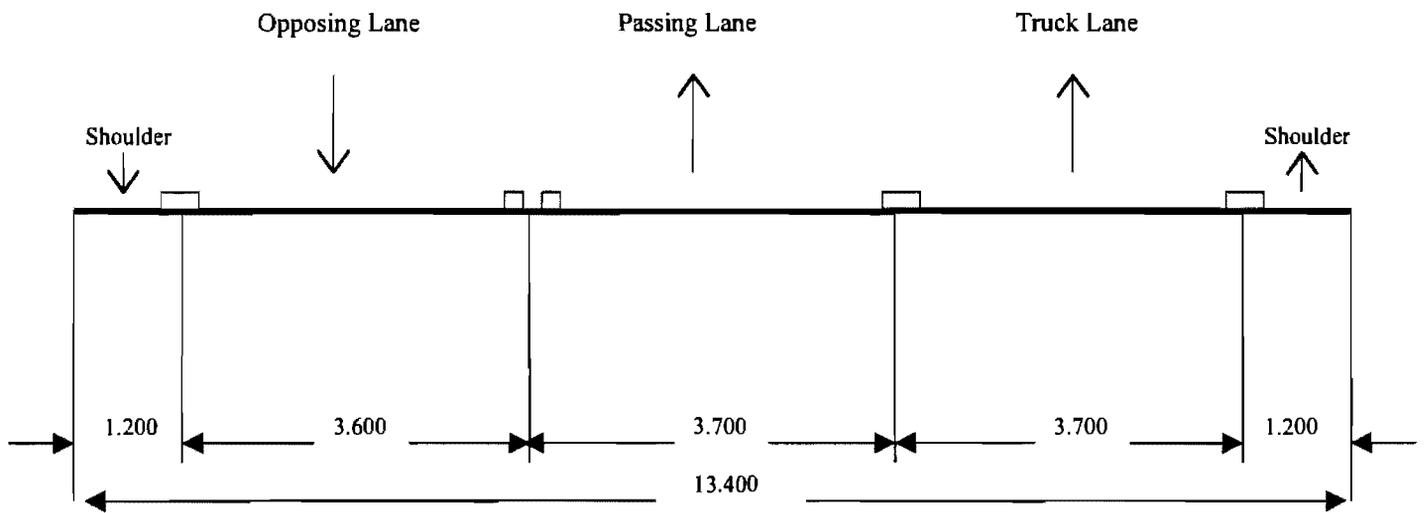
**Figure 2-2:** Three Lane Highway Cross Section in Canada
