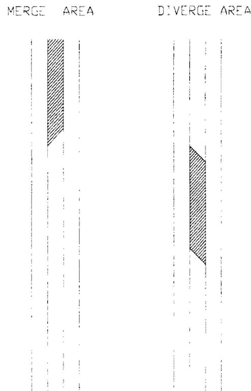
**Figure B- 1:** Type A Design with Continuous Interior Alternating Passing Lane
