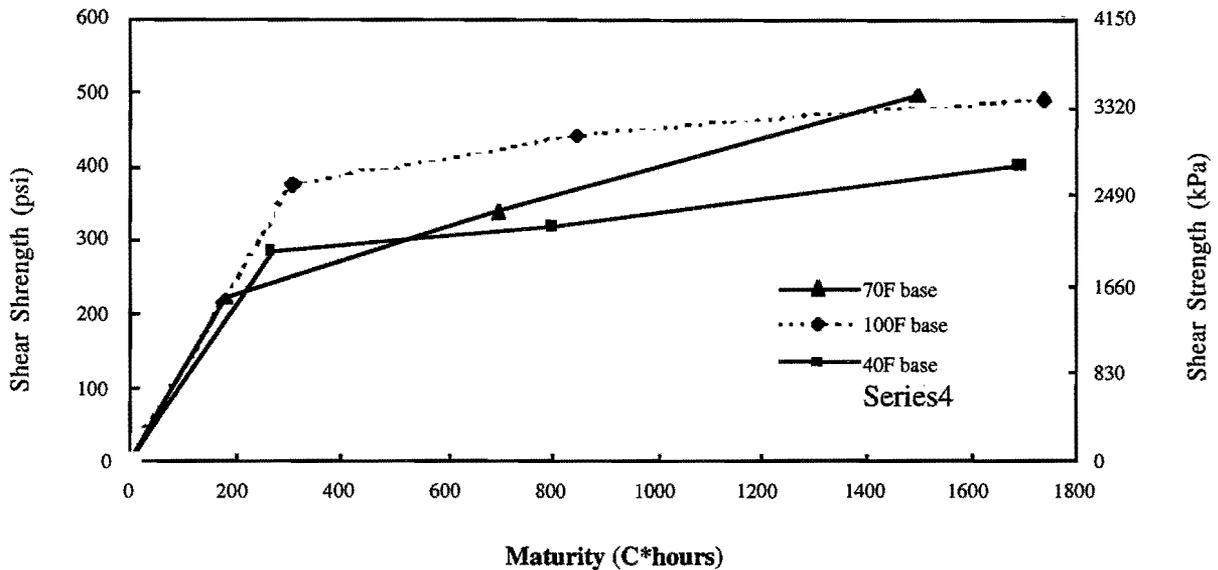
Figure 7.5. Maturity Values as a Function of Guillotine Test Bond Results (Low Evaporation Rate).
