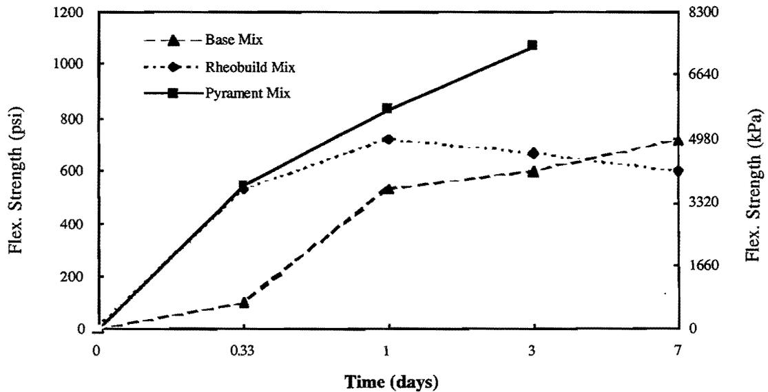
Figure 3.2. Flexural Strength Development for the Three Mixes Tested.
