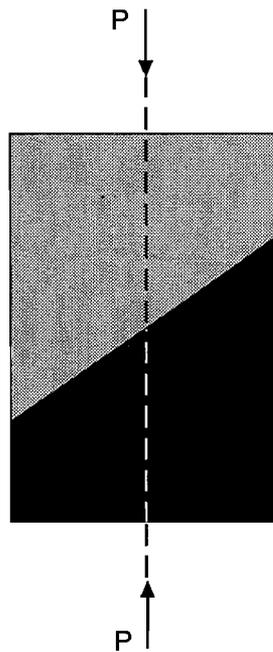
*Figure 2.5. Shear-Compression Test Specimen.*
