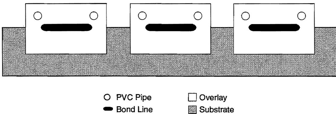
*Figure 6.2. Shear Block Test Set-Up (Elevation).*
