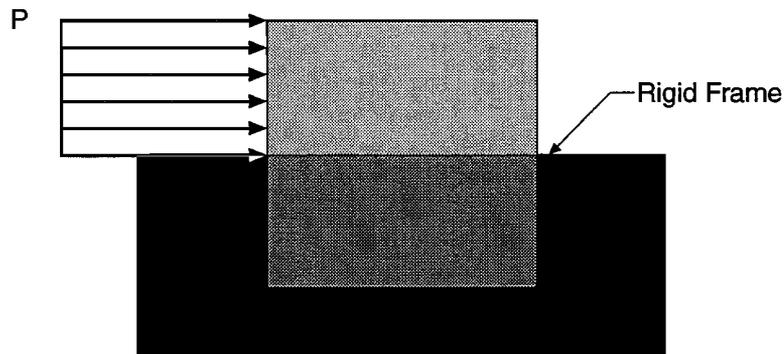
*Figure 2.4. Shear Test Specimen.*
