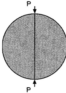
*Figure 2.3. Indirect Tension Test Specimen.*
