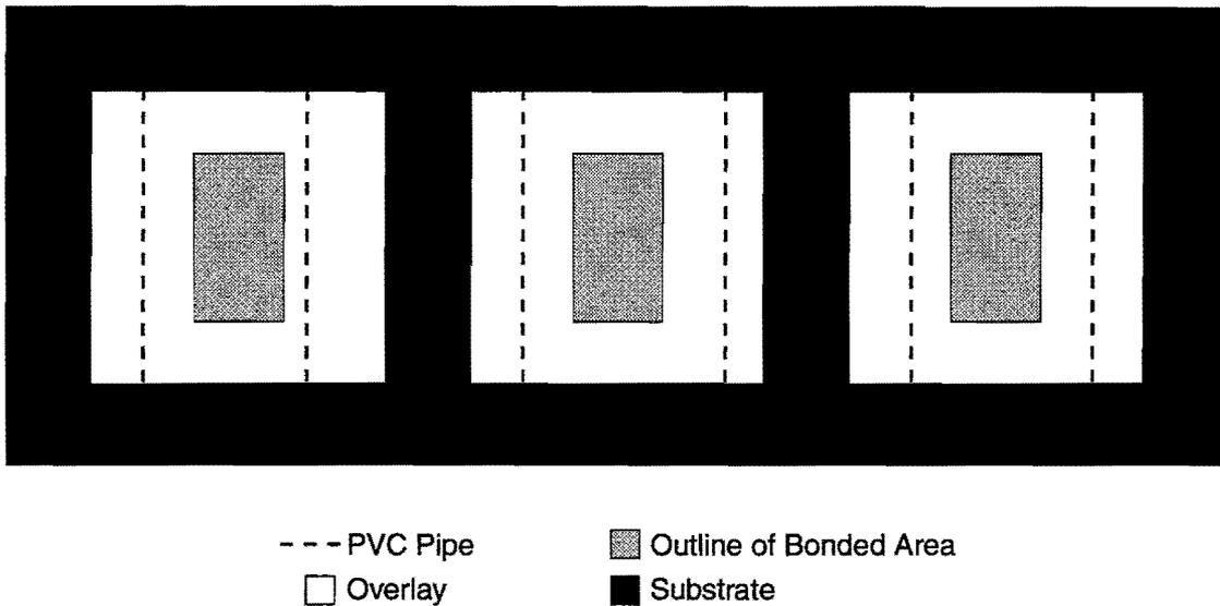
*Figure 6.1. Shear Block Test Set-Up (Plan).*
