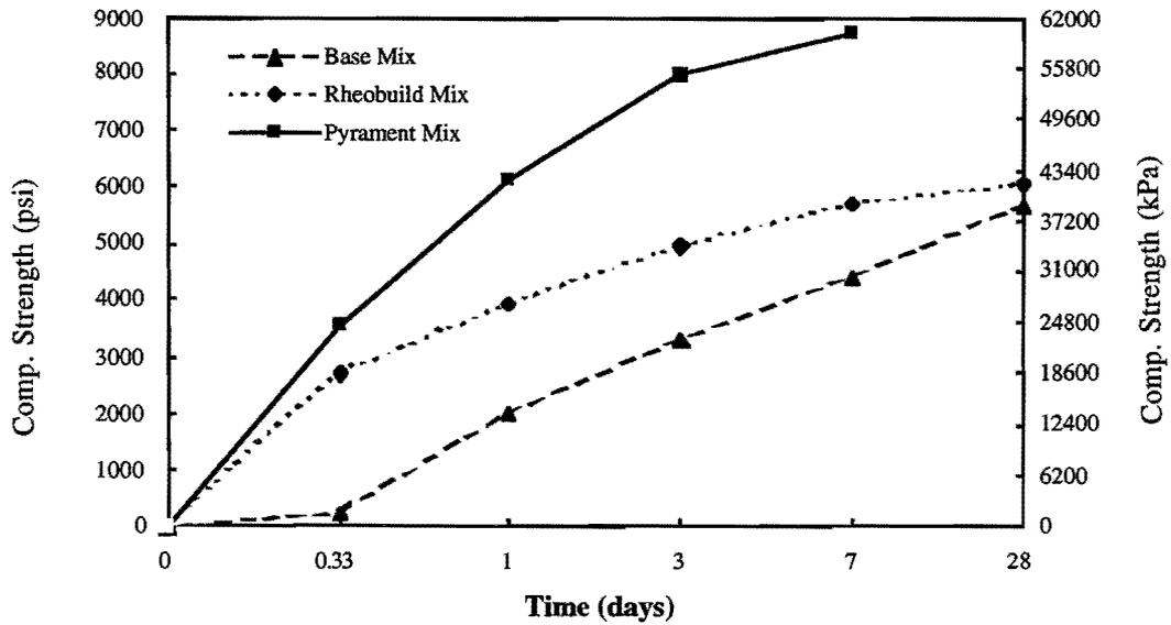
Figure 3.1. Compressive Strength Development for the Three Mixes Tested.
