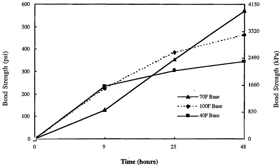
*Figure 6.5. Bond Development of Guillotine Specimens (High Evaporation Rate).*
