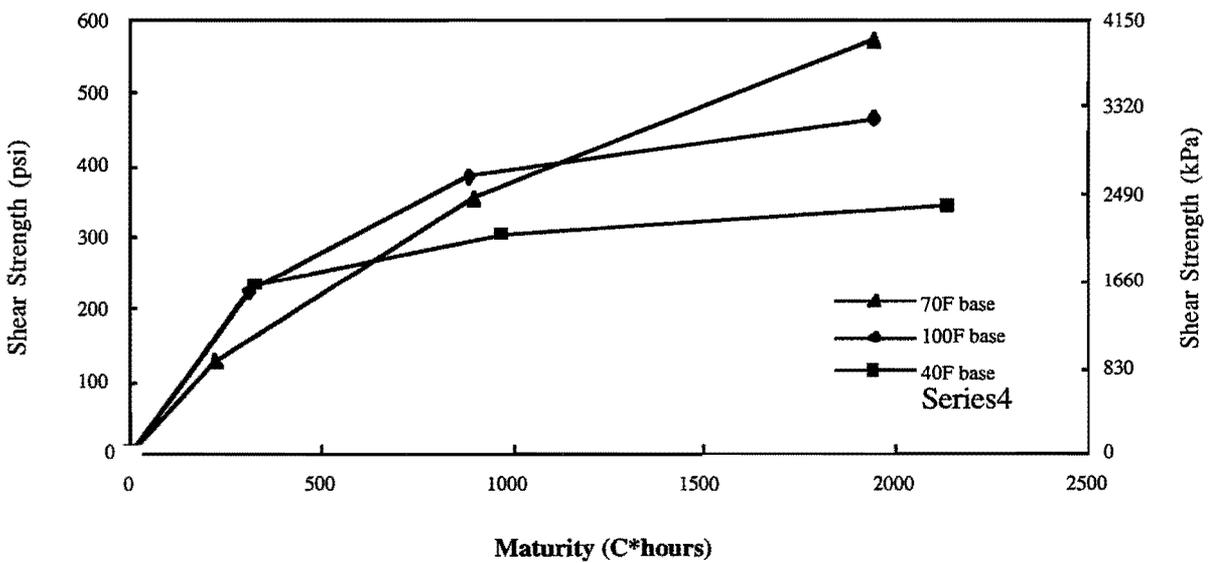
Figure 7.4. Maturity Values as a Function of Guillotine Bond Test Results (High Evaporation Rate).
