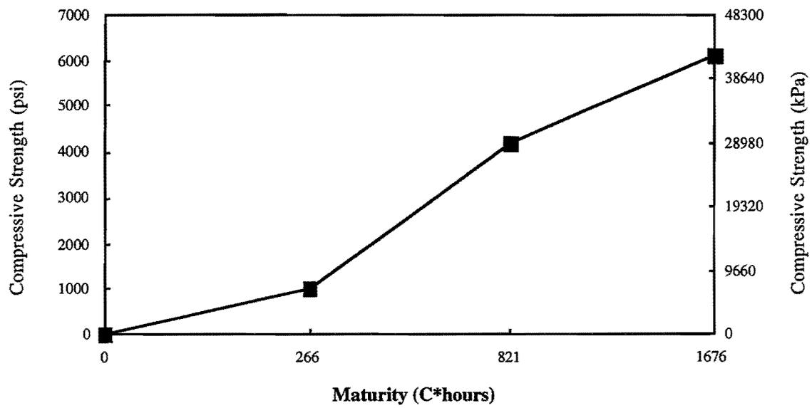
*Figure 7.6. Compressive Strength as a Function of Maturity.*
