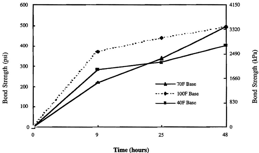
Figure 6.4. Bond Development of Guillotine Specimens (Low Evaporation Rate).
