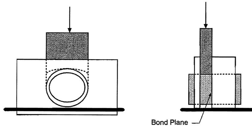
Figure 6.3. Guillotine Test Set-Up.
