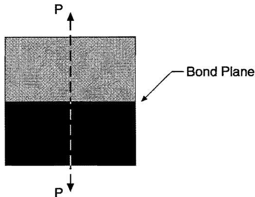
Figure 2.2. Direct Tension Test Specimen.
