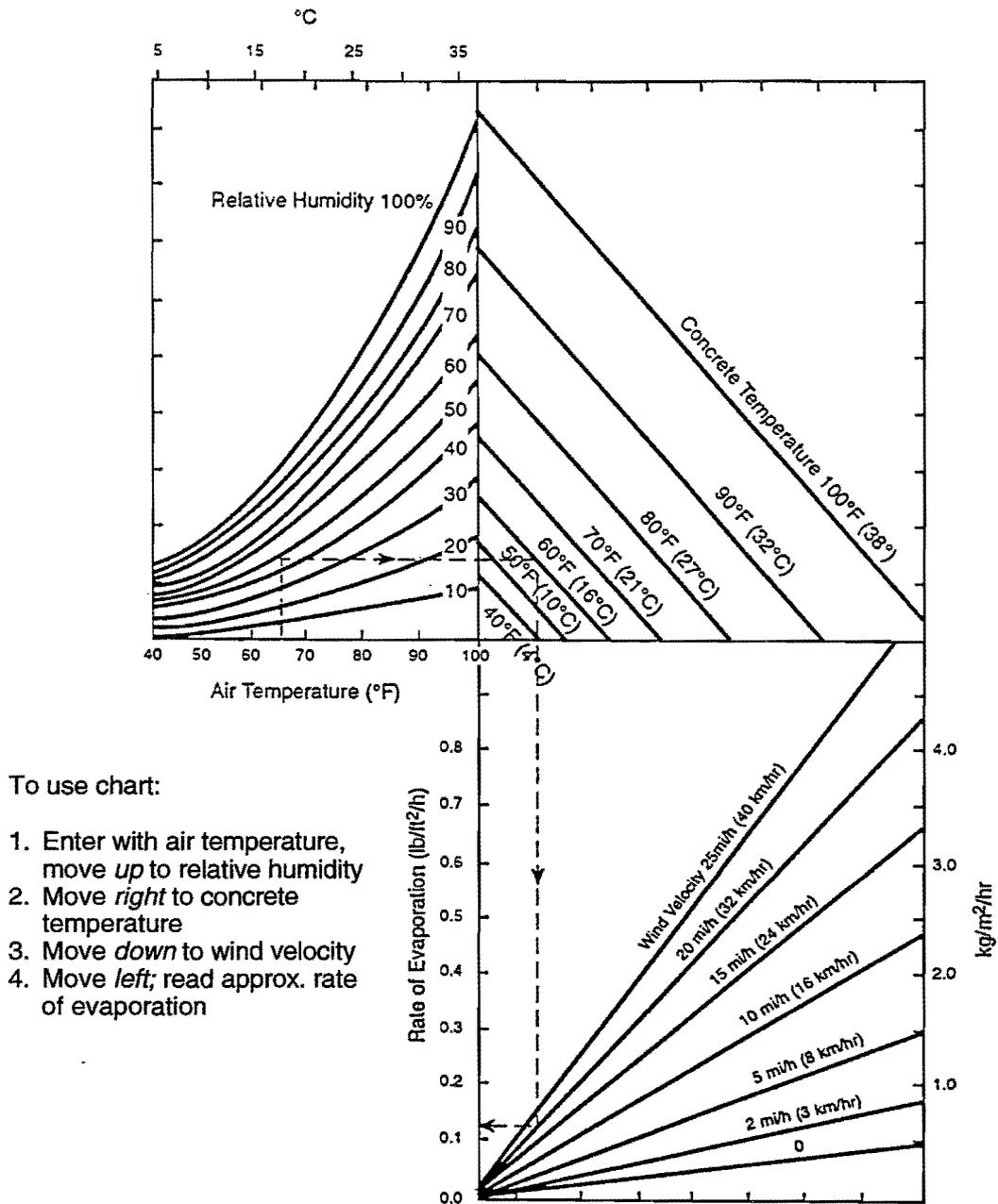
Figure 2.1. Nomograph for Calculating Evaporation Rate of Water from Freshly Placed Concrete (Ref 12).
