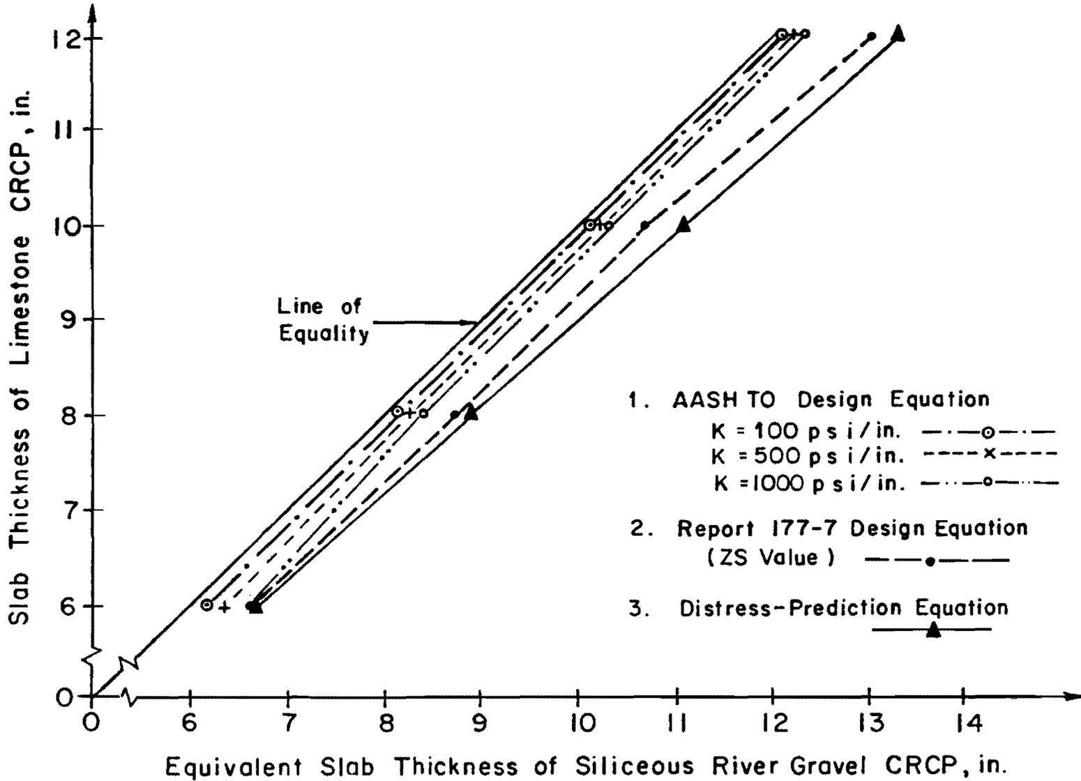
Fig 3.3. Comparison of the thickness equivalencies between a limestone and a siliceous river gravel CRCP obtained from the three different approaches.
