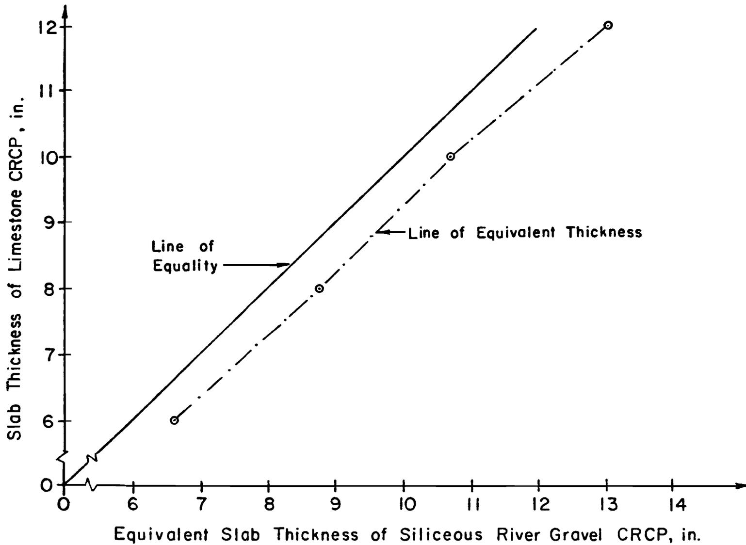
Fig 3.2. Thickness equivalencies between a limestone and a siliceous river gravel CRCP as determined from second approach.
