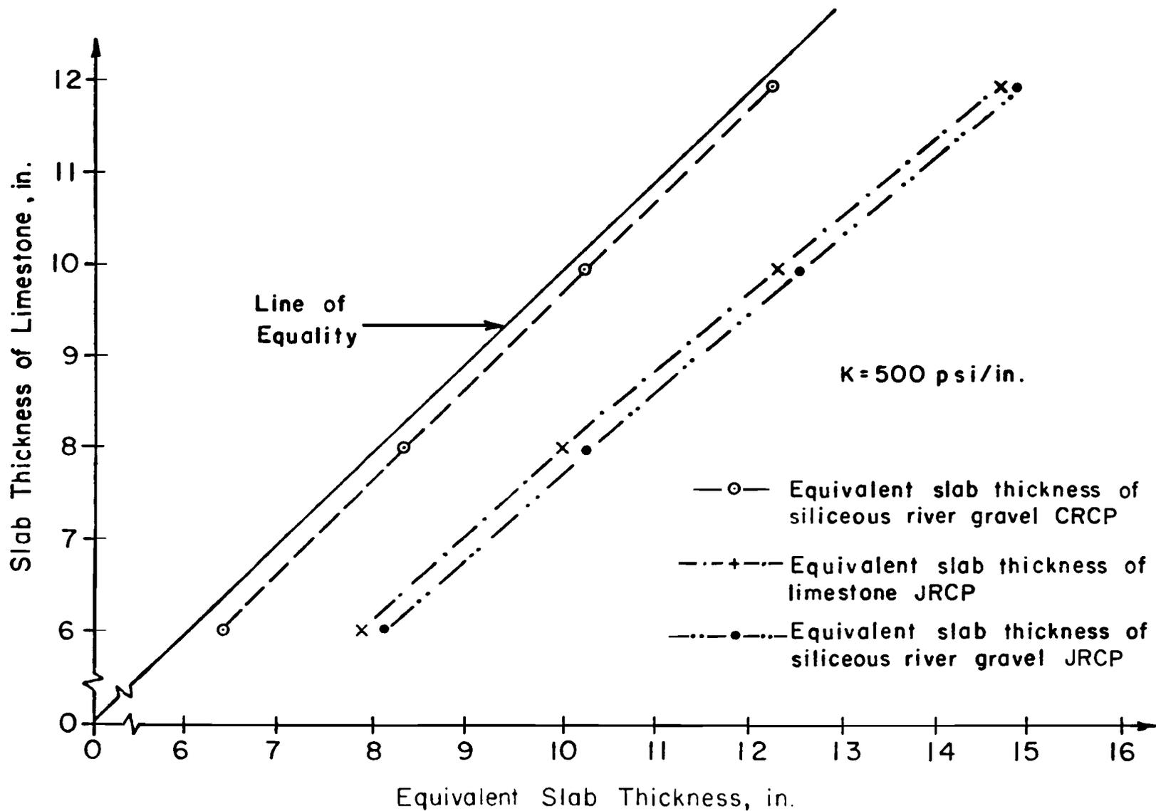
Fig A.1. Thickness equivalencies between a limestone CRCP and three different types of rigid pavements for a K-value of 500 p s i /inch, as determined from first approach.
