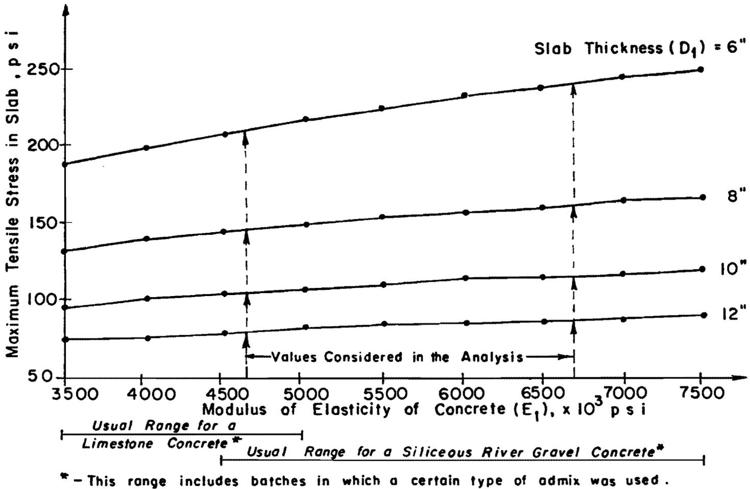
Fig A.3. Maximum tensile stress in the CRCP slab as a function of modulus of elasticity of concrete ( $E_1$ ) and slab thickness ( $D_1$ ) for the pavement structure shown in Fig A.2.
