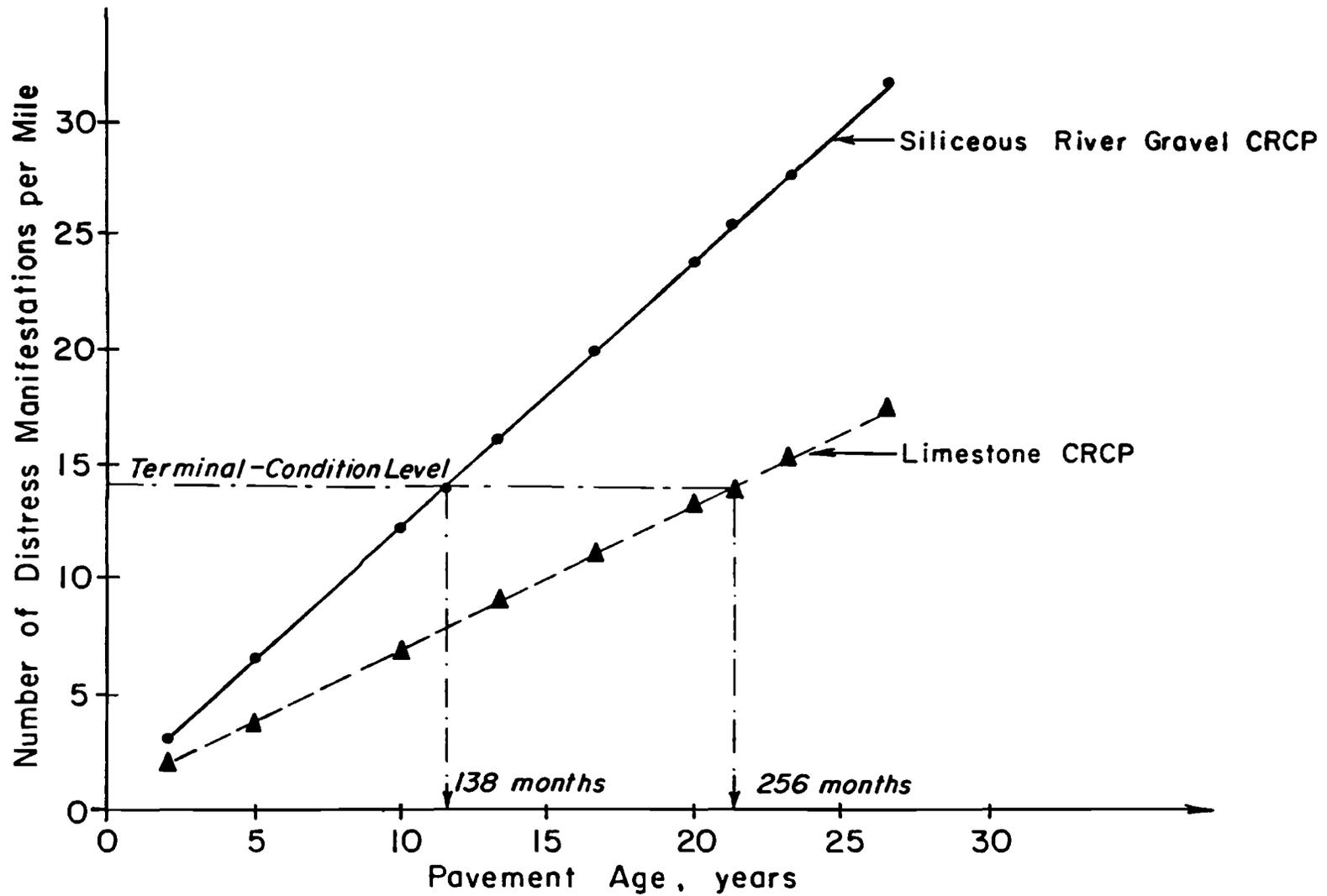
Fig A.5. Graphical determination of the pavement age to reach terminal-condition level for the data given in Table A.15.
