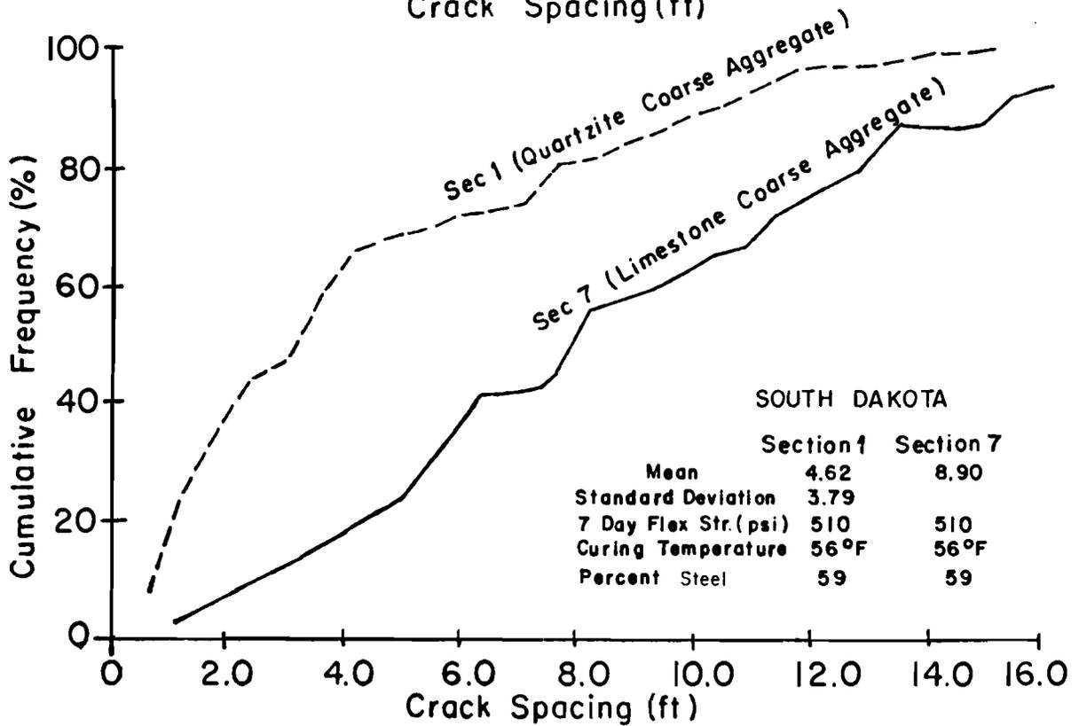
Fig 2.1. Effect of coarse aggregate type on distribution of crack spacing for two different conditions (Ref 3).
