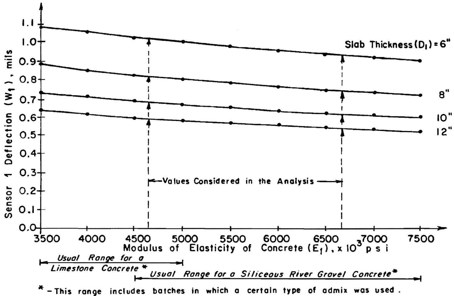
Fig A.4. Simulated sensor 1 deflection ( $W_1$ ) as a function of modulus of elasticity of concrete ( $E_1$ ) and slab thickness ( $D_1$ ) for the pavement structure shown in Fig A.2.
