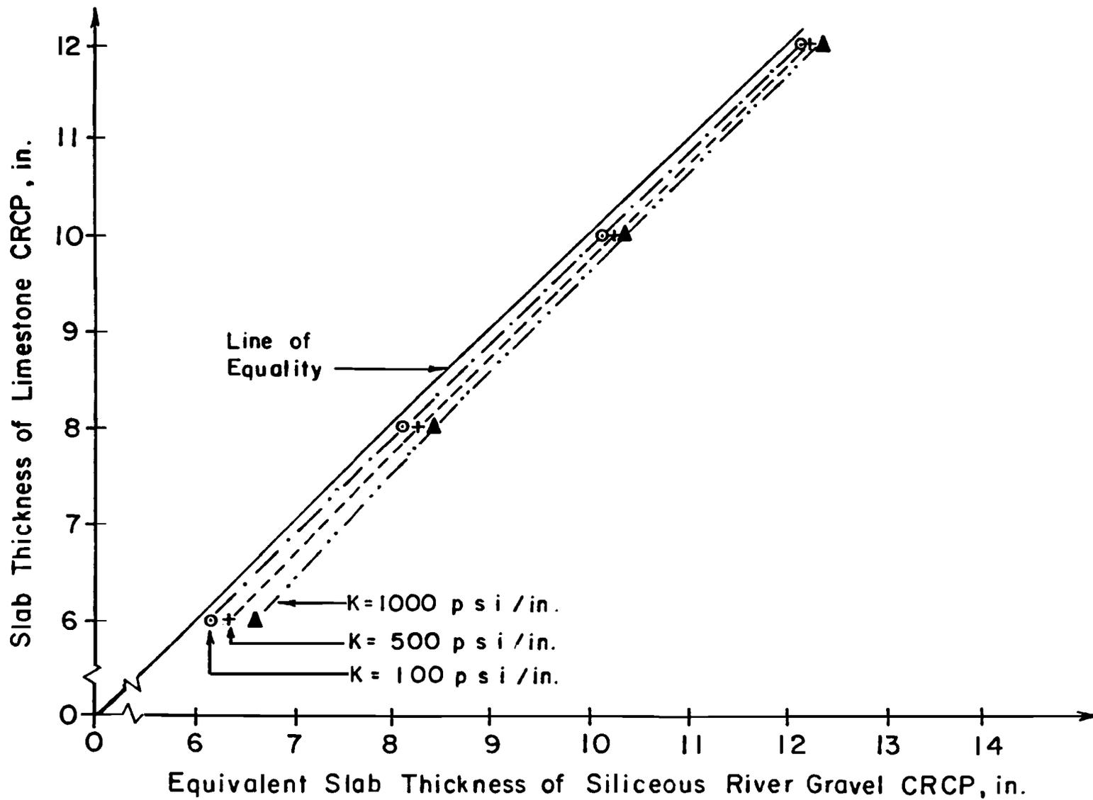
Fig 3.1. Thickness equivalencies between a limestone and a siliceous river gravel CRCP for various K-values, as determined from first approach.
