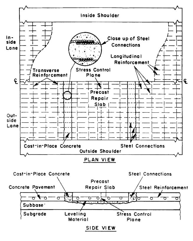
Fig 1. Precast repair methodology applied to CRCP. (After Ref 1).
