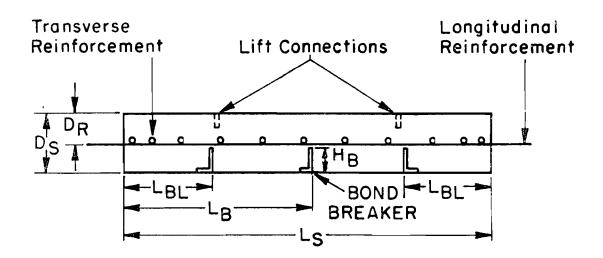
Fig 3. Guidelines for dimensions of precast repair slabs for Texas. (After Ref 1).
