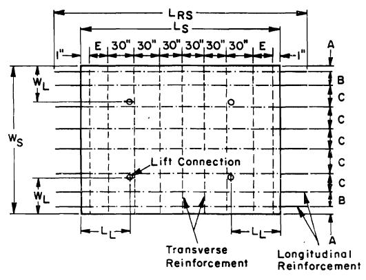
E = variable spacing to accommodate the transverse steel spacing
