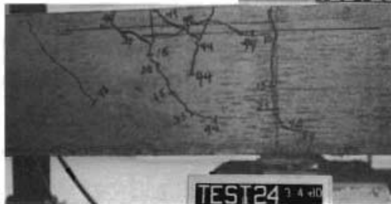
Fig. 4.7 Crack patterns, 53 in. shear span, #9 bars, f'_c \approx 6 ksi
