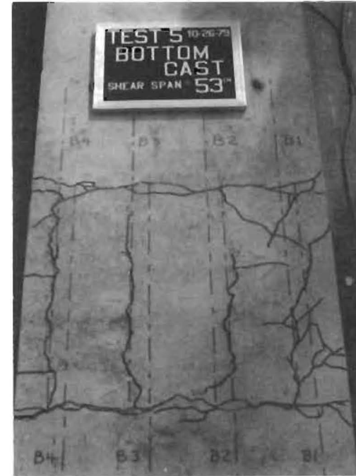
(c) Crack pattern on tension face, P_u = 56.9k
