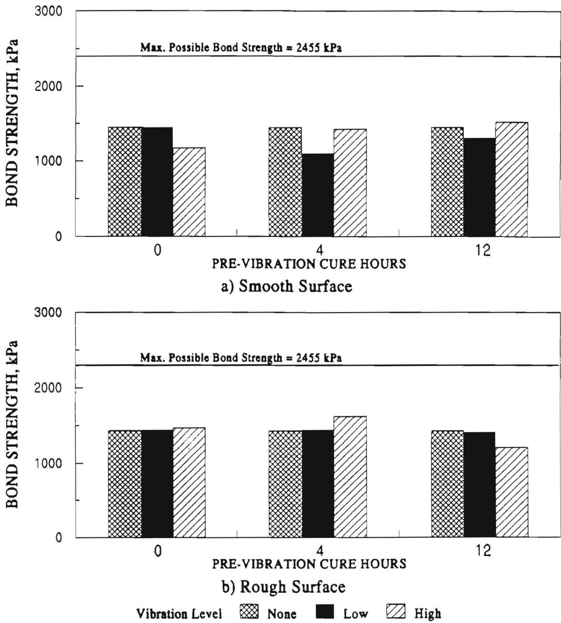
Figure 4.10 Impact of Pre-Vibration Cure Time on Bond Strength for 5-cm-Thick Overlays (Wet Interface)
