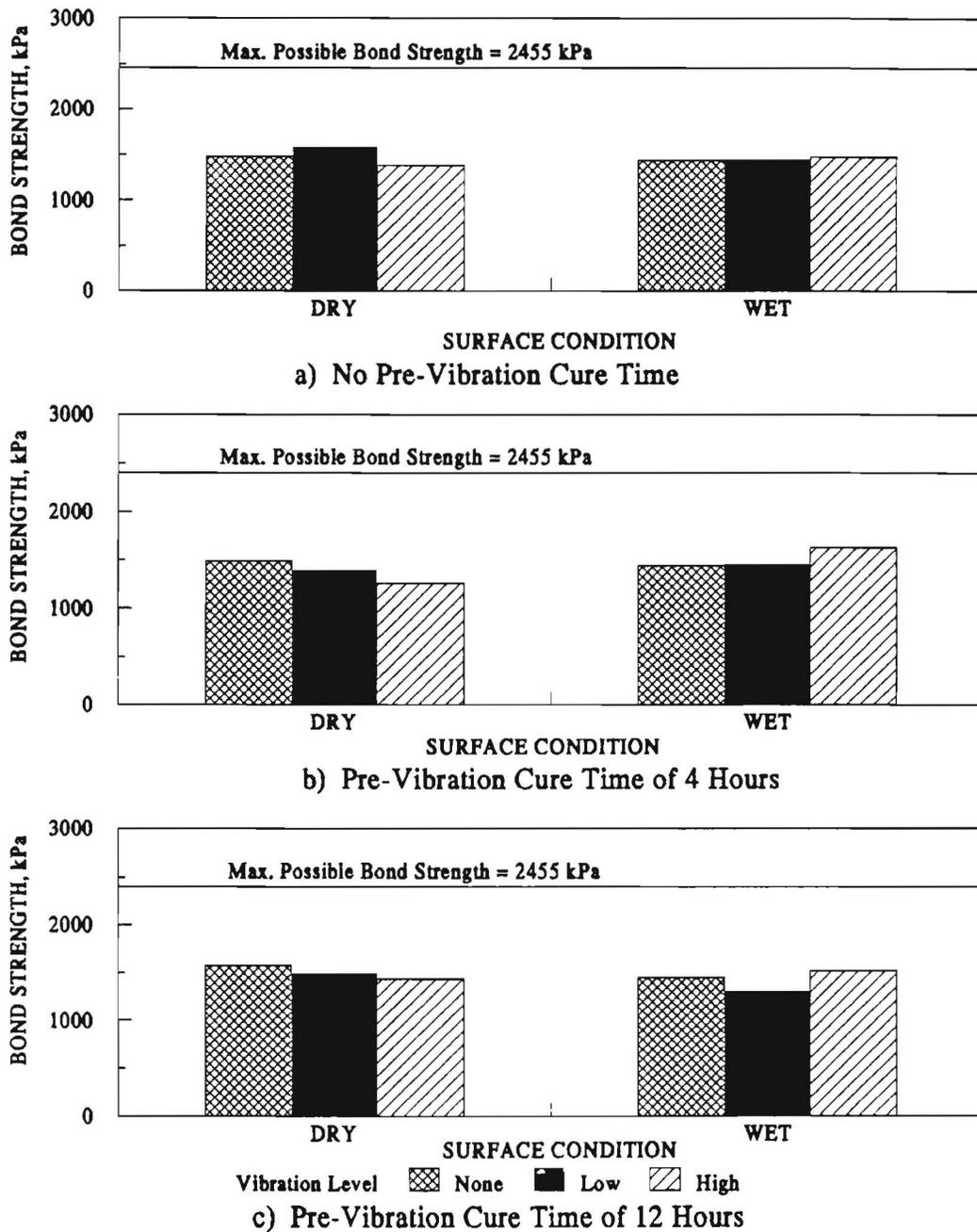
Figure 4.2 Impact of Surface Condition on Bond Strength for 5-cm-Thick Overlays (Rough Surface)
