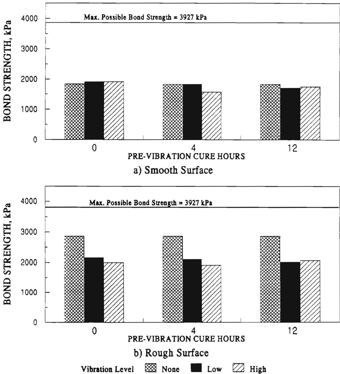
Figure 4.12 Impact of Pre-Vibration Cure Time on Bond Strength for 10-cm-Thick Overlays (Wet Interface)
