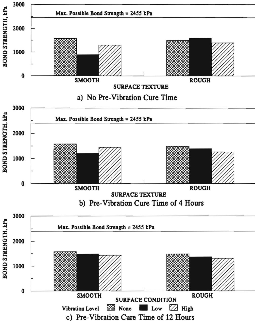
Figure 4.5 Impact of Surface Texture on Bond Strength for 5-cm-Thick Overlays (Dry Interface)
