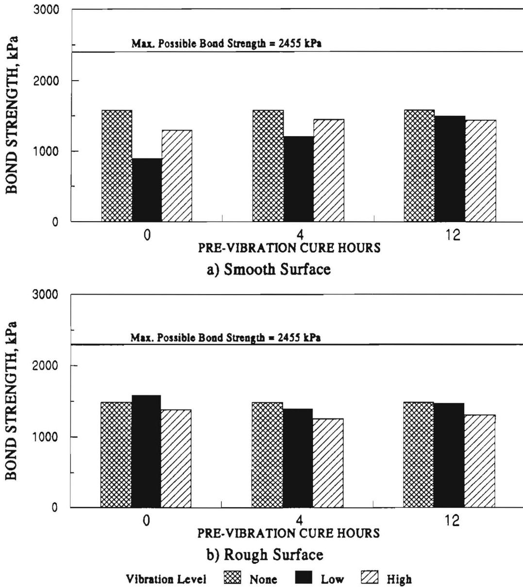
Figure 4.9 Impact of Pre-Vibration Cure Time on Bond Strength for 5-cm-Thick Overlays (Dry Interface)
