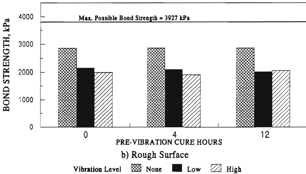
Figure 4.11 Impact of Pre-Vibration Cure Time on Bond Strength for 10-cm-Thick Overlays (Dry Interface)
