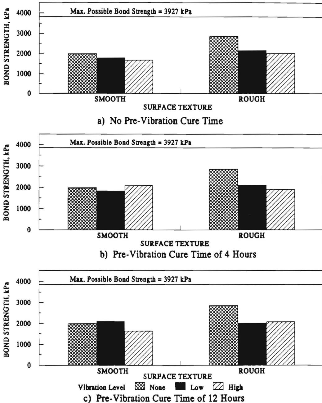
Figure 4.7 Impact of Surface Texture on Bond Strength for 10-cm-Thick Overlays (Dry Interface)
