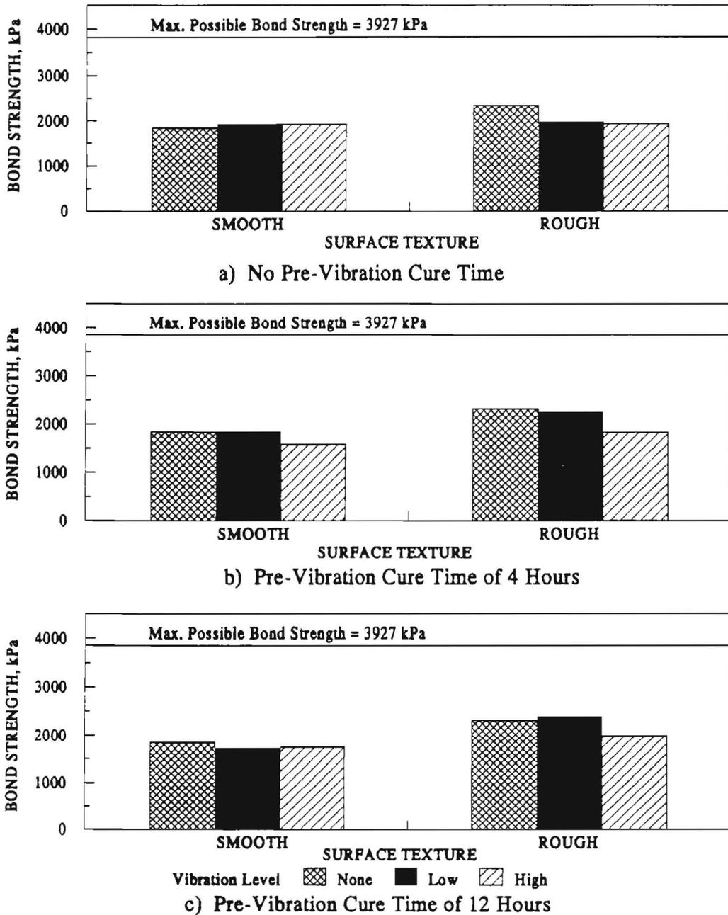
Figure 4.8 Impact of Surface Texture on Bond Strength for 10-cm-Thick Overlays (Wet Interface)
