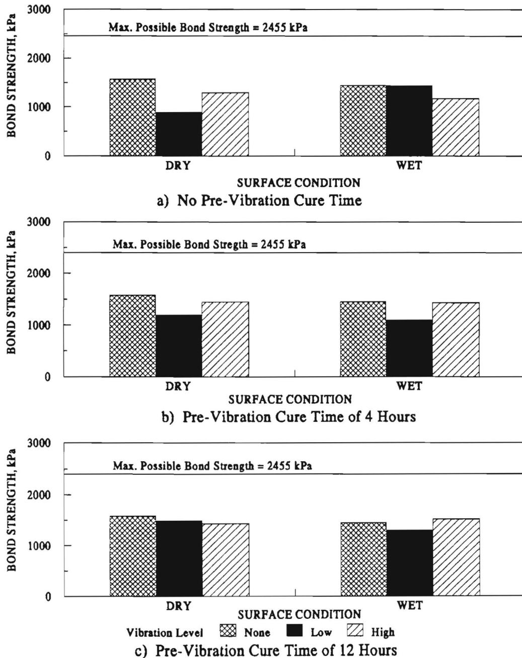
Figure 4.1 Impact of Surface Condition on Bond Strength for 5-cm-Thick Overlays (Smooth Surface)
