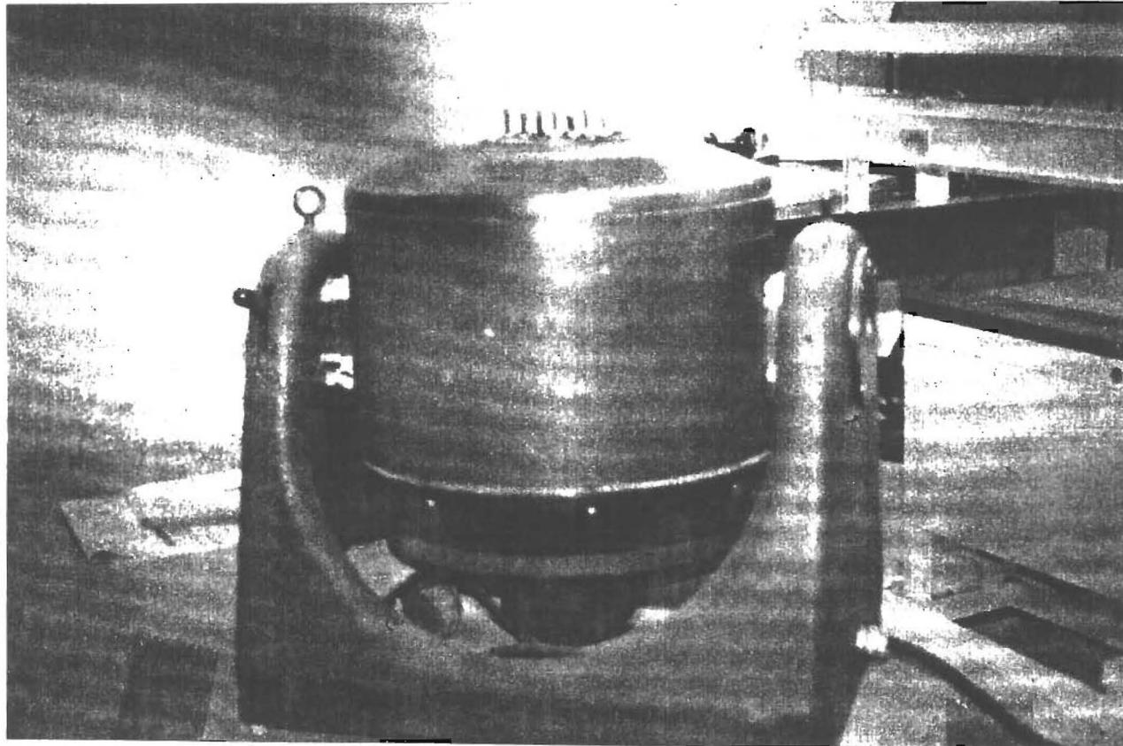
Figure 2.5 9-kN Shaker Used in This Study
