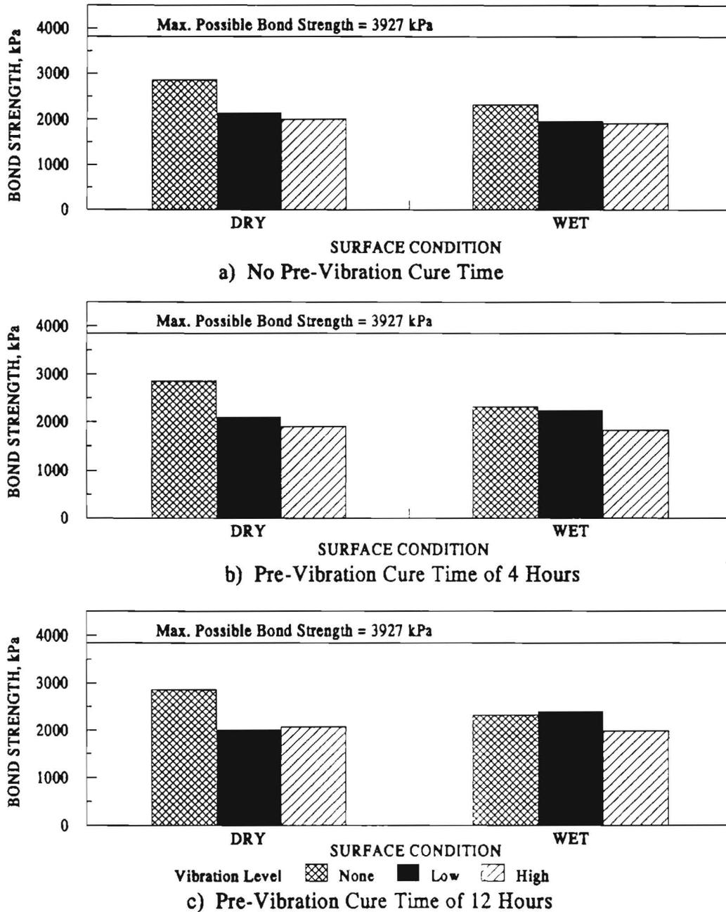
Figure 4.4 Impact of Surface Condition on Bond Strength for 10-cm-Thick Overlays (Rough Surface)
