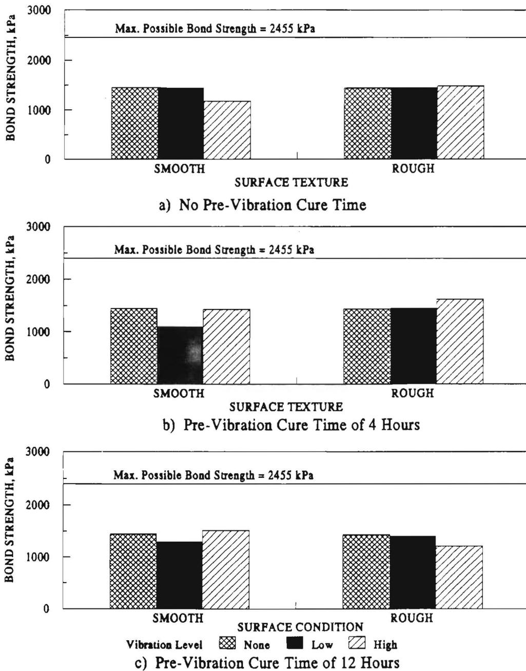
Figure 4.6 Impact of Surface Texture on Bond Strength for 5-cm-Thick Overlays (Wet Interface)
