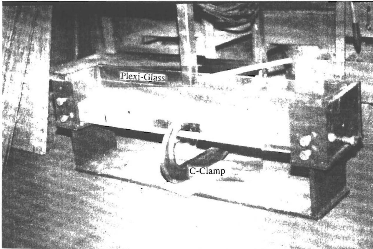
Figure 2.3 Platform Used to Place Large Specimens on 9-kN Shaker
