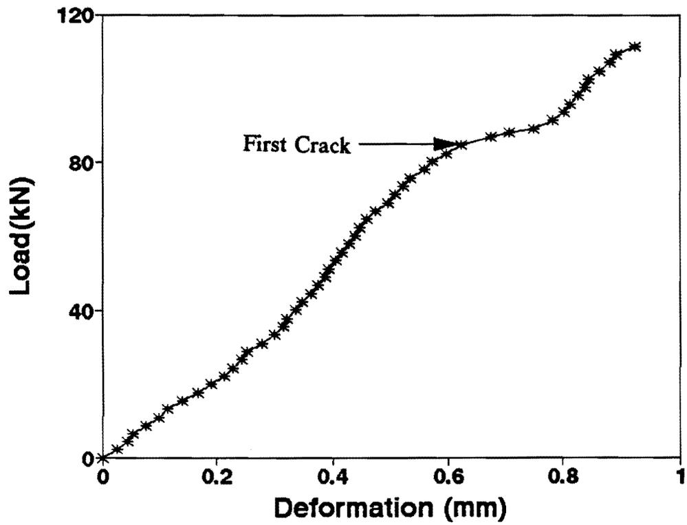
Figure 3.3 Typical Load Deformation Curve from Bending Tests
