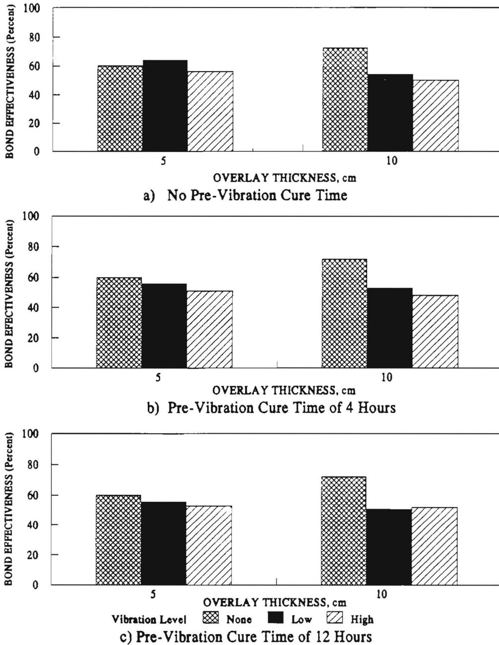
Figure 4.15 Impact of Overlay Thickness on Bond Effectiveness for Specimens with Rough, Dry Interface
