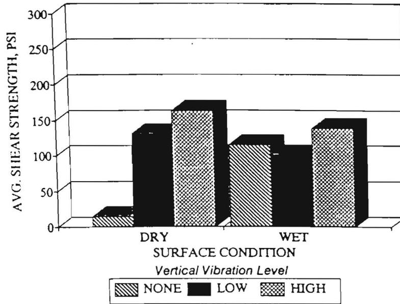
Figure 4.5 Comparison of Average Shear Strengths for a 4-in Overlay After 4 Hrs. of Pre-Vibration Cure (Smooth Interface) Under Vertical Vibration Mode
