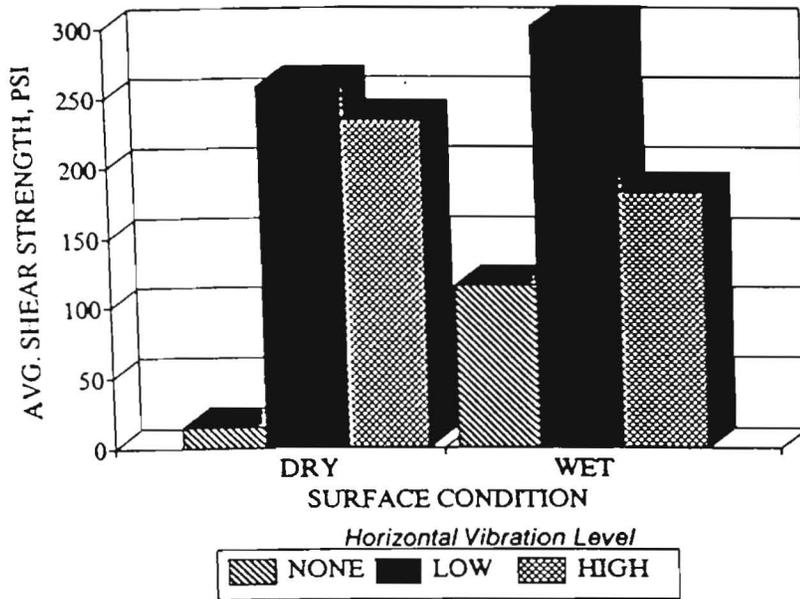
Figure 4.17 Comparison of Average Shear Strengths for a 4-in Overlay After 12 hrs. of Pre-Vibration Cure (Smooth Interface) Under Horizontal Vibration Mode
