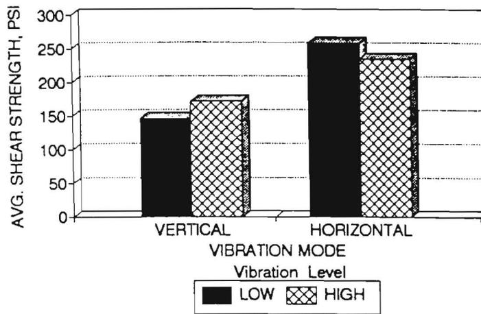
Figure 4.29 Comparison of Average Shear Strengths for a 4-in Overlay After 12 hrs. of Pre-Vibration Cure (Smooth-Dry Interface) Under Vertical and Horizontal Vibration Modes
