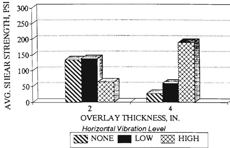
Figure 4.21 Comparison of Average Shear Strengths After 0 hrs. of Pre-Vibration Cure (Rough-Wet Interface) Under Horizontal Vibration Mode
