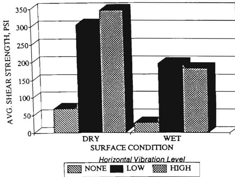
Figure 4.18 Comparison of Average Shear Strengths for a 4-in Overlay After 12 hrs. of Pre-Vibration Cure (Rough Interface) Under Horizontal Vibration Mode
