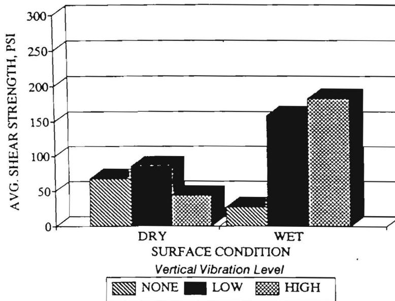
Figure 4.4 Comparison of Average Shear Strengths for a 4-in Overlay After 0 Hrs. of Pre-Vibration Cure (Rough Interface) Under Vertical Vibration Mode
