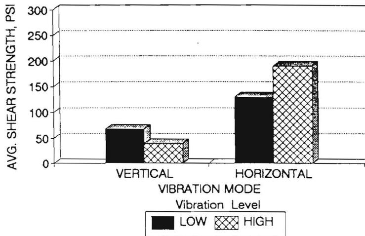
Figure 4.24 Comparison of Average Shear Strengths for a 2-in Overlay after 0 hrs. of Pre-Vibration Cure (Rough-Dry Interface) Under Vertical and Horizontal Vibration Modes
