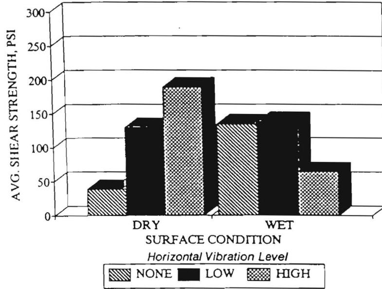
Figure 4.13 Comparison of Average Shear Strengths for a 2-in Overlay After 0 hrs. of Pre-Vibration Cure (Rough Interface) Under Horizontal Vibration Mode
