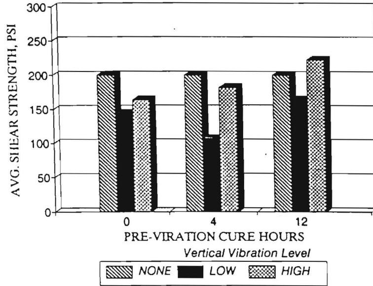
Figure 4.9 Comparison of Average Shear Strengths for a 6-in. Overlay (Rough-Dry Interface) Under Vertical Vibration Mode
