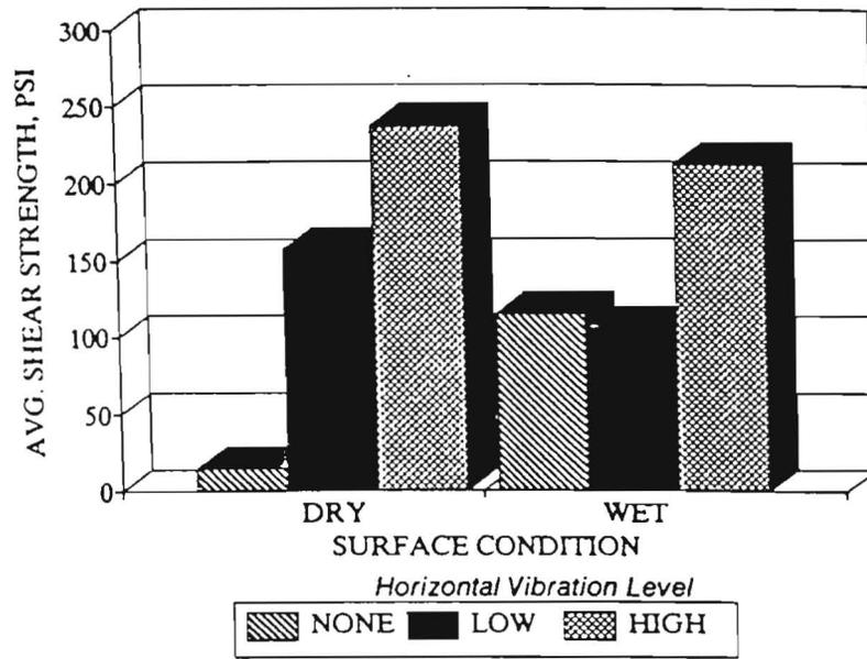
Figure 4.15 Comparison of Average Shear Strengths for a 4-in Overlay After 4 hrs. of Pre-Vibration Cure (Smooth Interface) Under Horizontal Vibration Mode
