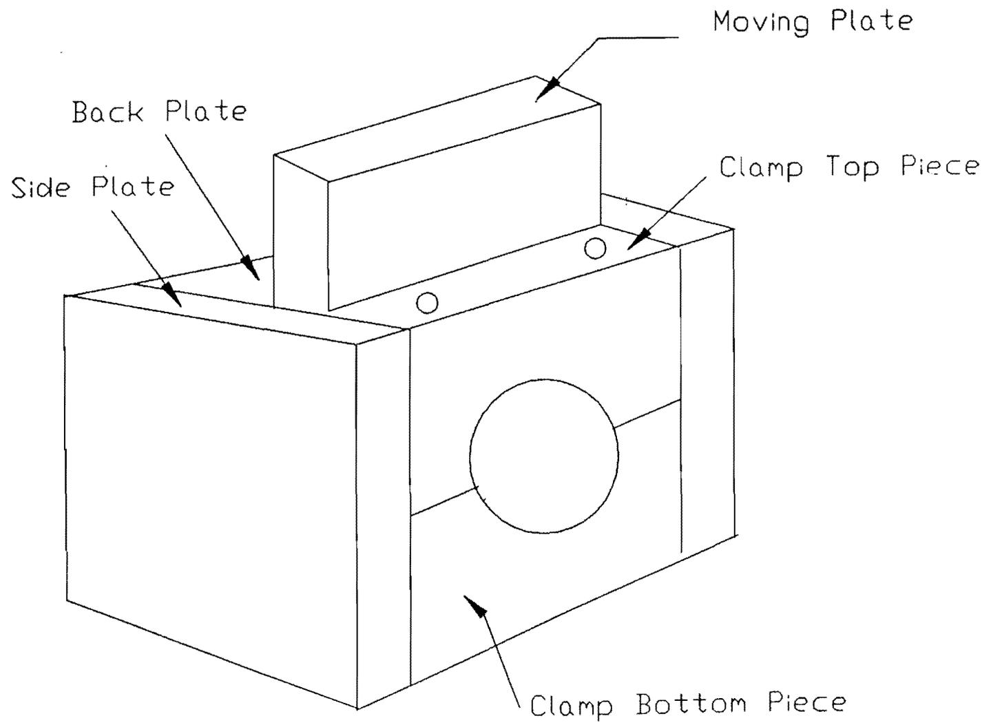
Figure 3.11 Guillotine Direct Shear Test Apparatus
