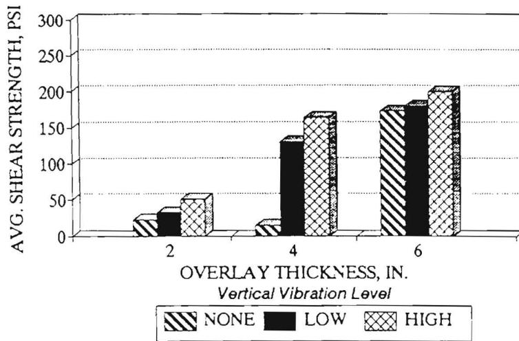
Figure 4.11 Comparison of Average Shear Strengths After 4 Hrs. of Pre-Vibration Cure (Smooth-Dry Interface) Under Vertical Vibration Mode
