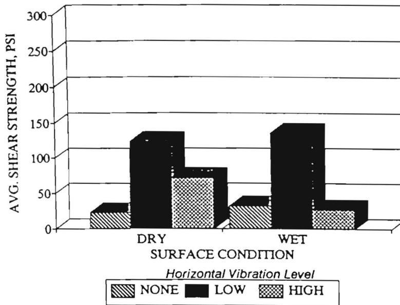
Figure 4.14 Comparison of Average Shear Strengths for a 2-in Overlay After 4 hrs. of Pre-Vibration Cure (Smooth Interface) Under Horizontal Vibration Mode
