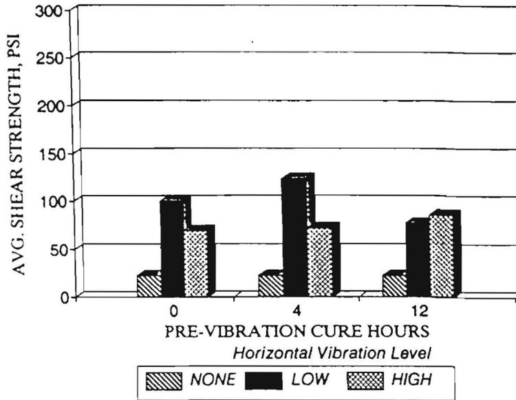
Figure 4.19 Comparison of Average Shear Strengths for a 2-in Overlay (Smooth-Dry Interface) Under Horizontal Vibration Mode
