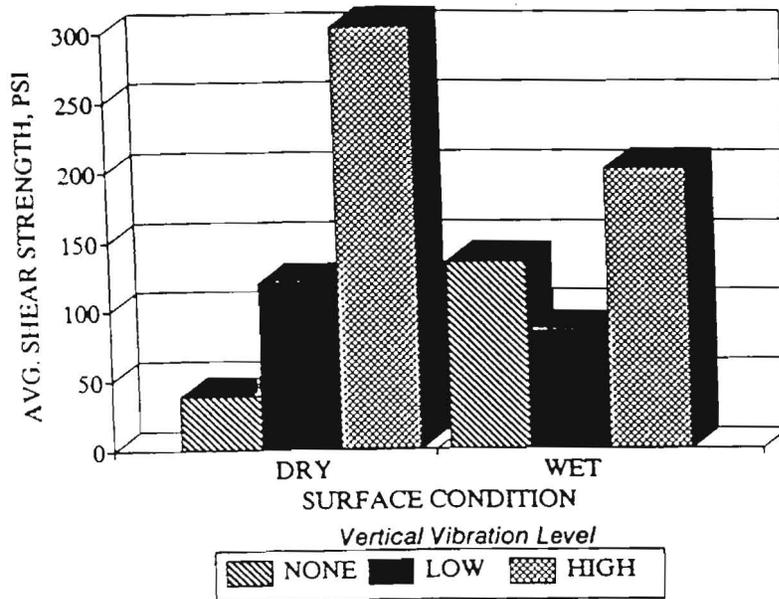
Figure 4.3 Comparison of Average Shear Strengths for a 2-in Overlay After 12 Hrs. of Pre-Vibration Cure (Rough Interface) Under Vertical Vibration Mode
