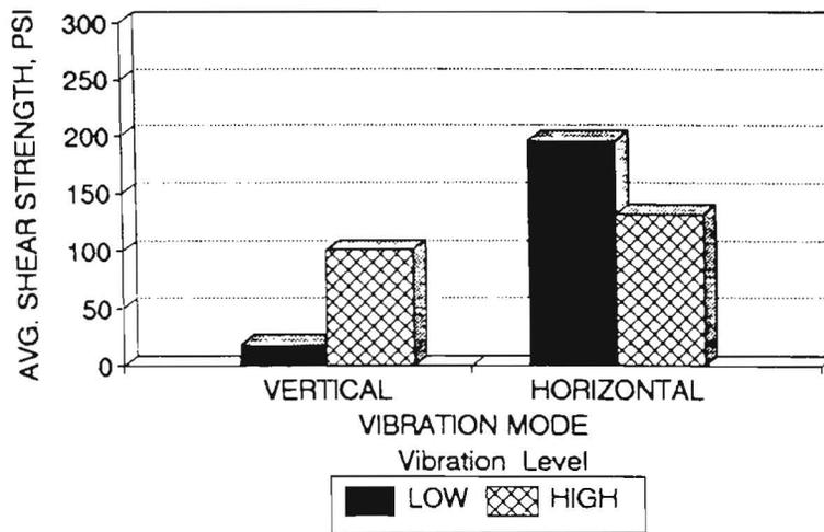
Figure 4.25 Comparison of Average Shear Strengths for a 2-in Overlay After 4 hrs. of Pre-Vibration Cure (Rough-Dry Interface) Under Vertical and Horizontal Vibration Modes
