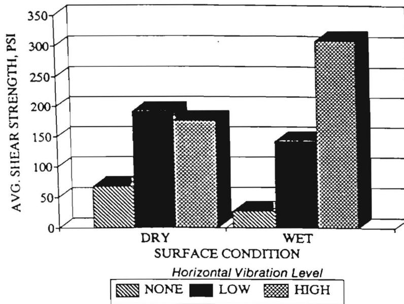
Figure 4.16 Comparison of Average Shear Strengths for a 4-in Overlay After 4 hrs. of Pre-Vibration Cure (Rough Interface) Under Horizontal Vibration Mode
