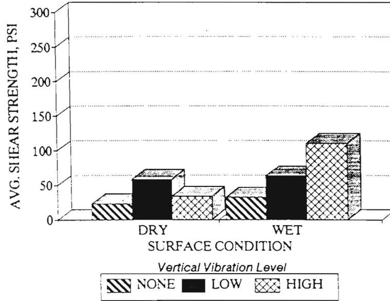
Figure 4.1 Comparison of Average Shear Strengths for a 2-in Overlay After 0 Hrs. of Pre-vibration Cure (Smooth Interface) Under Vertical Vibration Mode
