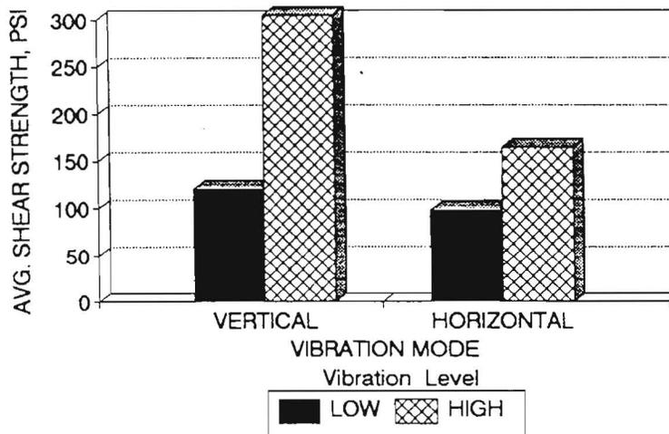
Figure 4.26 Comparison of Average Shear Strengths for a 2-in Overlay After 12 hrs. of Pre-Vibration Cure (Rough-Dry Interface) Under Vertical and Horizontal Vibration Modes
