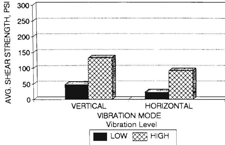
Figure 4.27 Comparison of Average Shear Strengths for a 4-in Overlay after 0 hrs. of Pre-Vibration Cure (Smooth-Dry Interface) Under Vertical and Horizontal Vibration Modes
