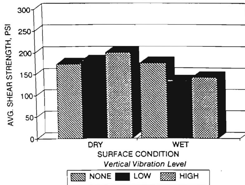
Figure 4.6 Comparison of Average Shear Strengths for a 6-in Overlay After 4 Hrs. of Pre-Vibration Cure (Smooth Interface) Under Vertical Vibration Mode
