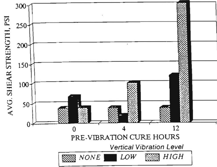
Figure 4.7 Comparison of Average Shear Strengths for a 2-in. Overlay (Rough-Dry Interface) Under Vertical Vibration Mode
