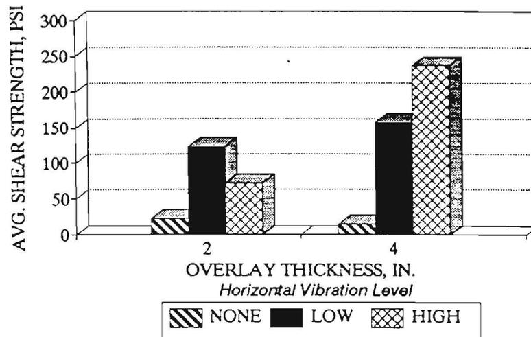
Figure 4.22 Comparison of Average Shear Strengths After 4 hrs. of Pre-Vibration Cure (Smooth-Dry Interface) Under Horizontal Vibration Mode
