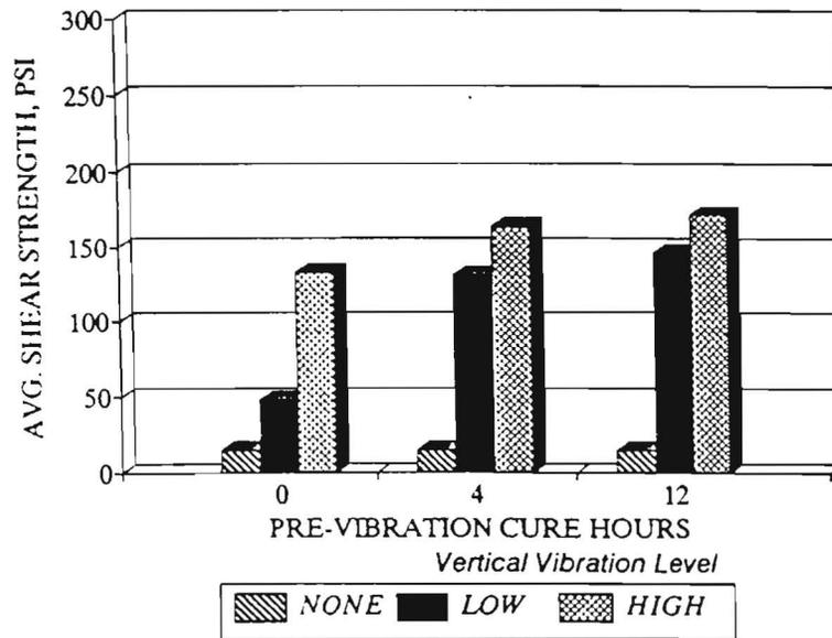
Figure 4.8 Comparison of Average Shear Strengths for a 4-in. Overlay (Smooth-Dry Interface) Under Vertical Vibration Mode
