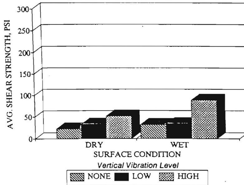
Figure 4.2 Comparison of Average Shear Strengths for a 2-in Overlay After 4 Hrs. of Pre-vibration Cure (Smooth Interface) Under Vertical Vibration Mode
