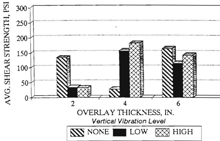
Figure 4.10 Comparison of Average Shear Strengths After 0 Hrs. of Pre-Vibration Cure (Rough-Wet Interface) Under Vertical Vibration Mode
