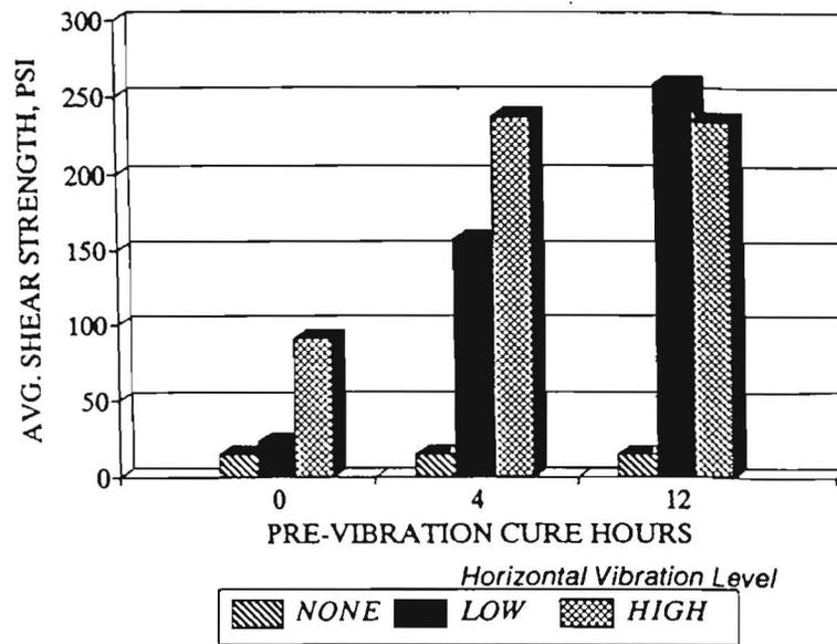
Figure 4.20 Comparison of Average Shear Strengths for a 4-in Overlay (Smooth-Dry Interface) Inerface) Under Horizontal Vibration Mode
