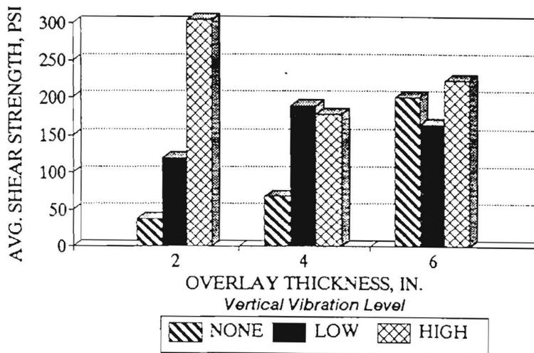
Figure 4.12 Comparison of Average Shear Strengths After 12 Hrs. of Pre-Vibration Cure (Rough-Dry Interface) Under Vertical Vibration Mode
