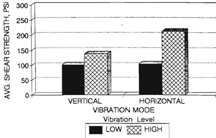
Figure 4.28 Comparison of Average Shear Strengths for a 4-in Overlay After 4 hrs. of Pre-Vibration Cure (Smooth-Wet Interface) Under Vertical and Horizontal Vibration Modes
