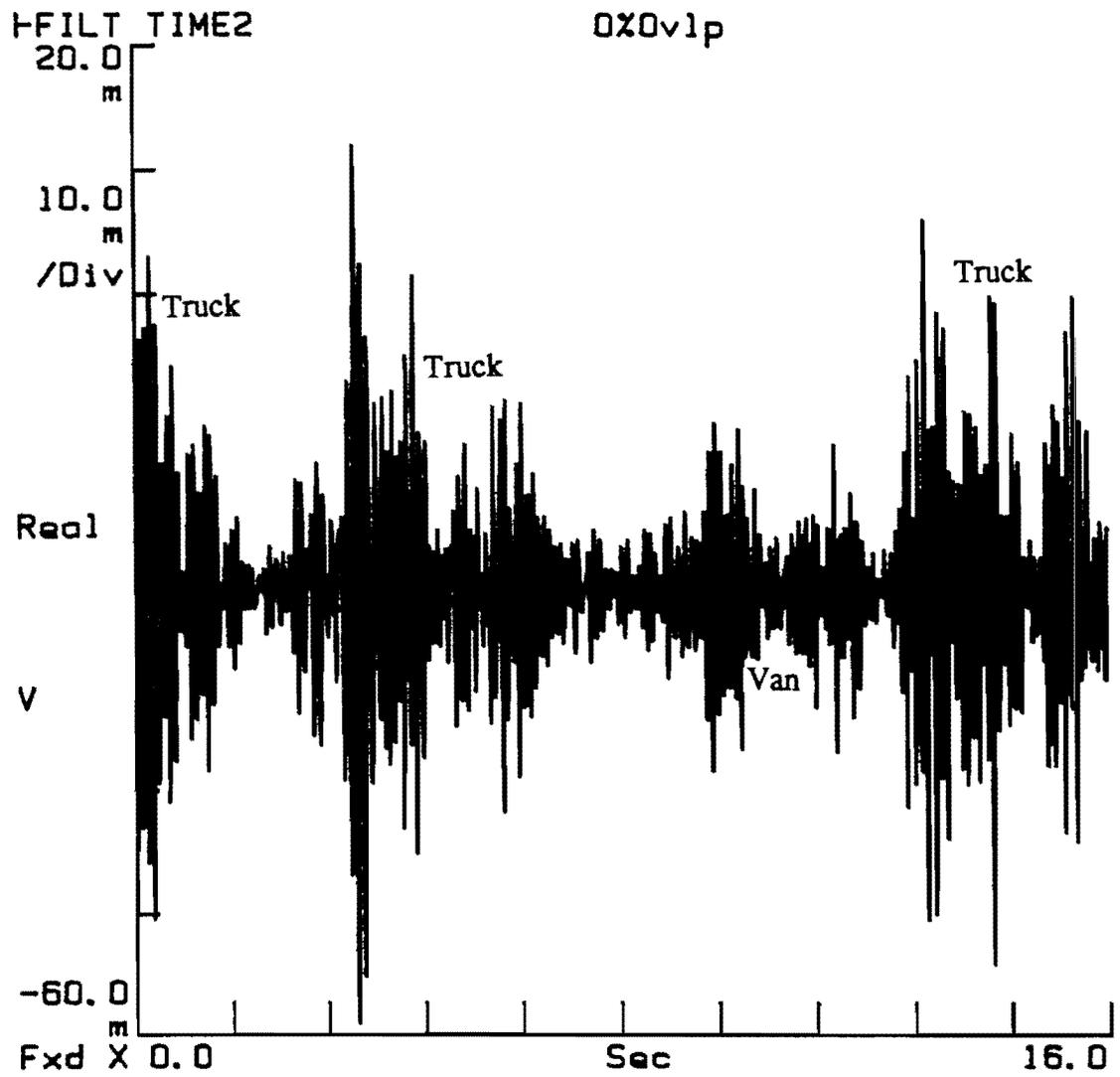
Figure 3.5 Vibration Amplitude Time History of Bridge Deck
