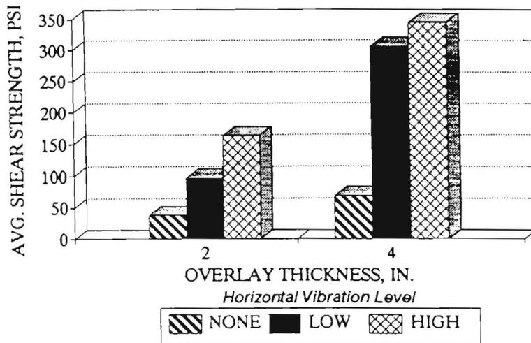
Figure 4.23 Comparison of Average Shear Strengths After 12 hrs. of Pre-Vibration Cure (Rough-Dry Interface) Under Horizontal Vibration Mode
