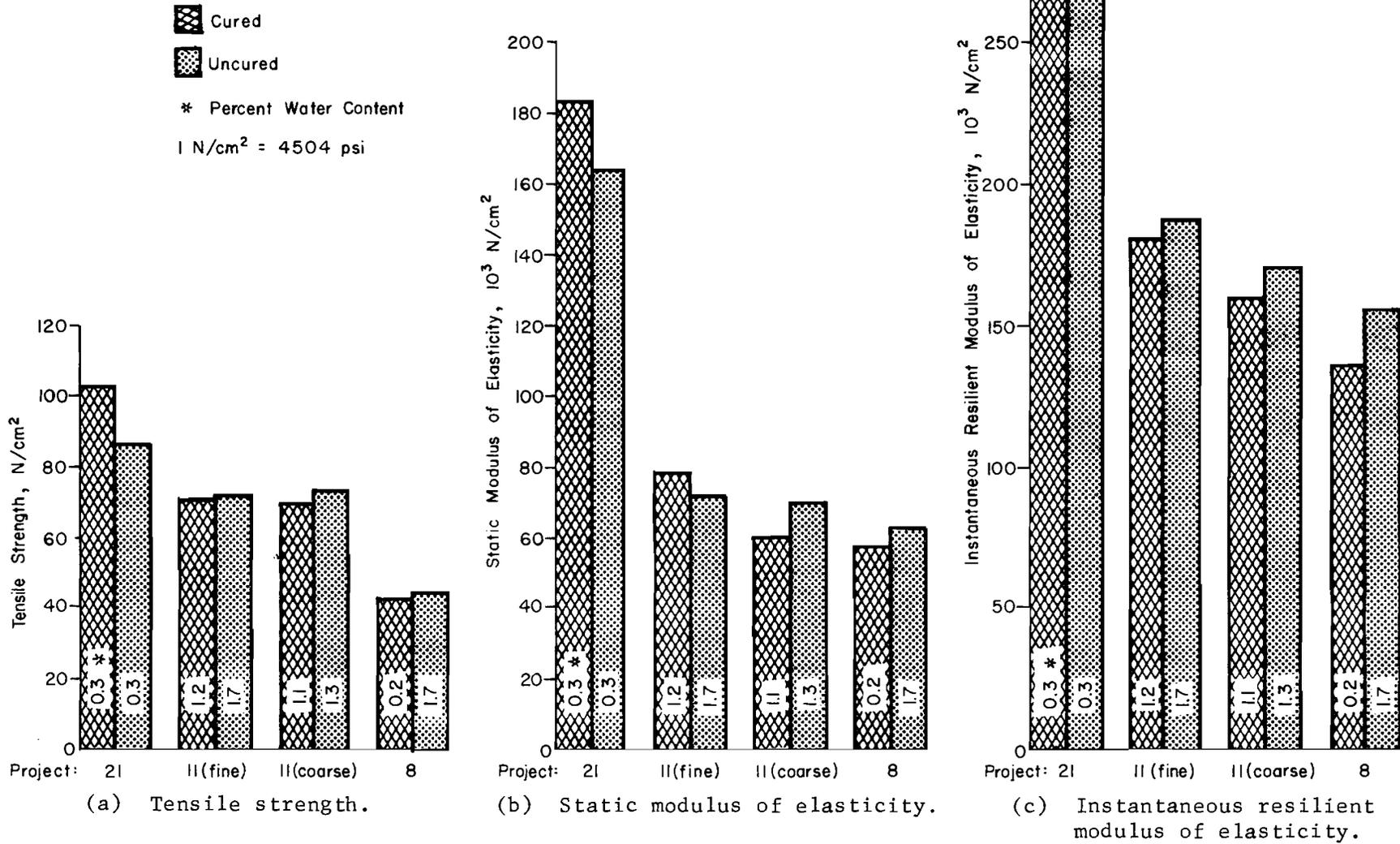
Fig 22. Effect of curing treatment on engineering properties.
