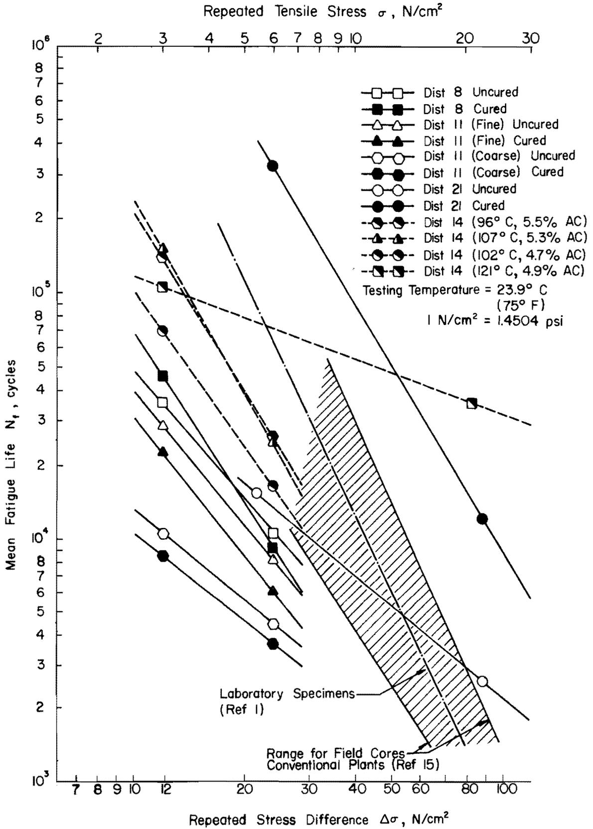
Fig 16. Logarithmic relationships between fatigue life and stress.
