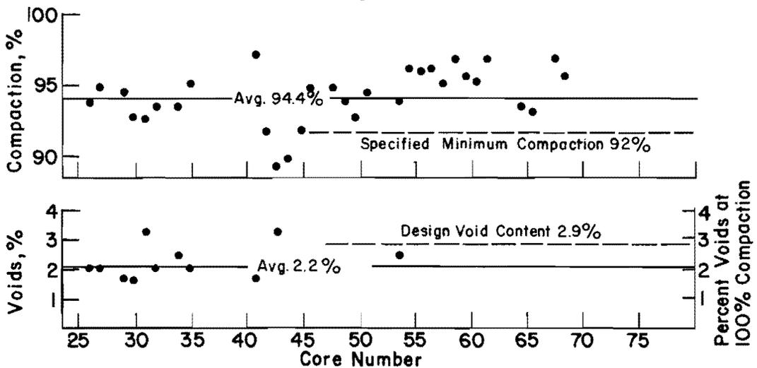
Fig 10. Uniformity of density and voids (Refs 19 and 21).
