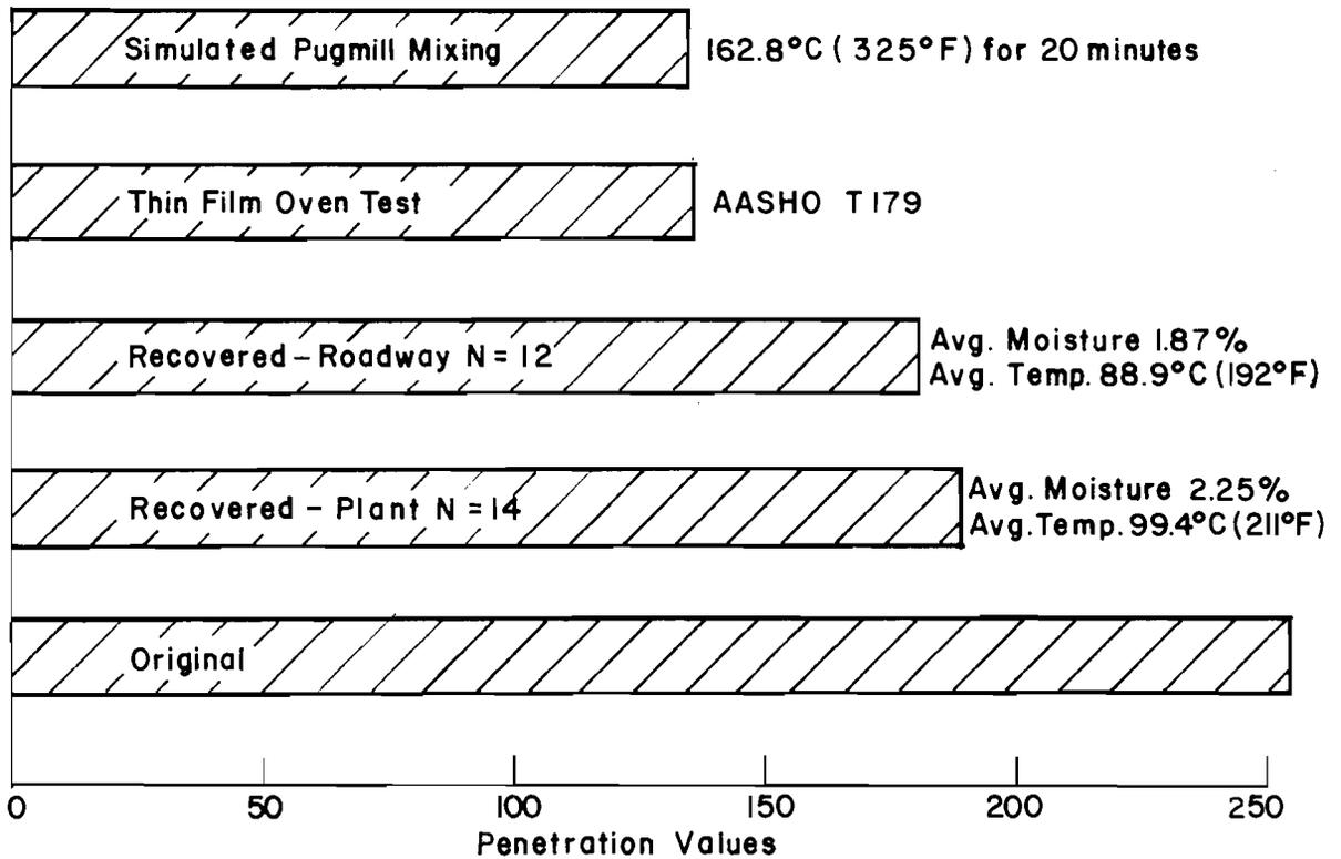
Fig 3. Hardening of 200/300 penetration asphalt for project in North Dakota (Refs 6 and 19).
