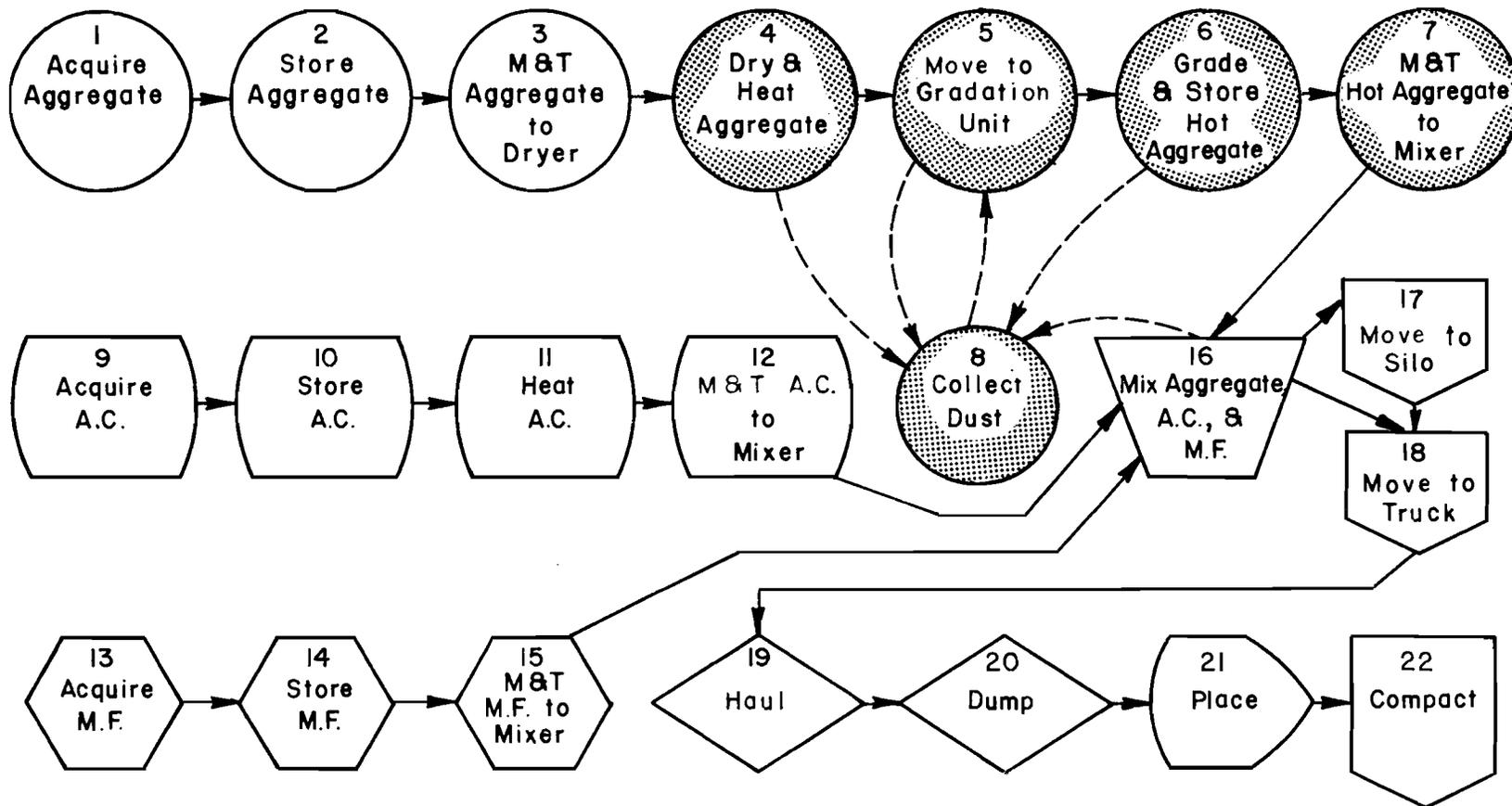
M & T - Measure and Transport, A.C. - Asphalt Cement, M.F. - Mineral Filler
