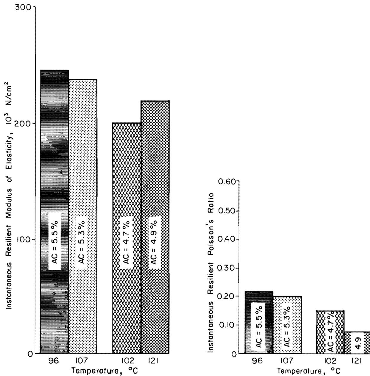
Fig 25. Effect of mixing and compaction temperature on resilient properties of Project 14.
