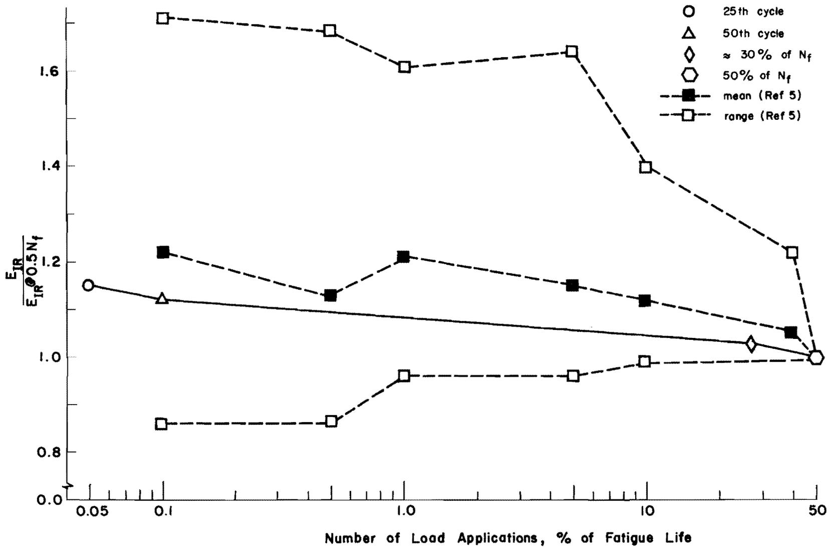
Fig 21. Relationship between instantaneous resilient modulus and number of load applications for Project 14.
