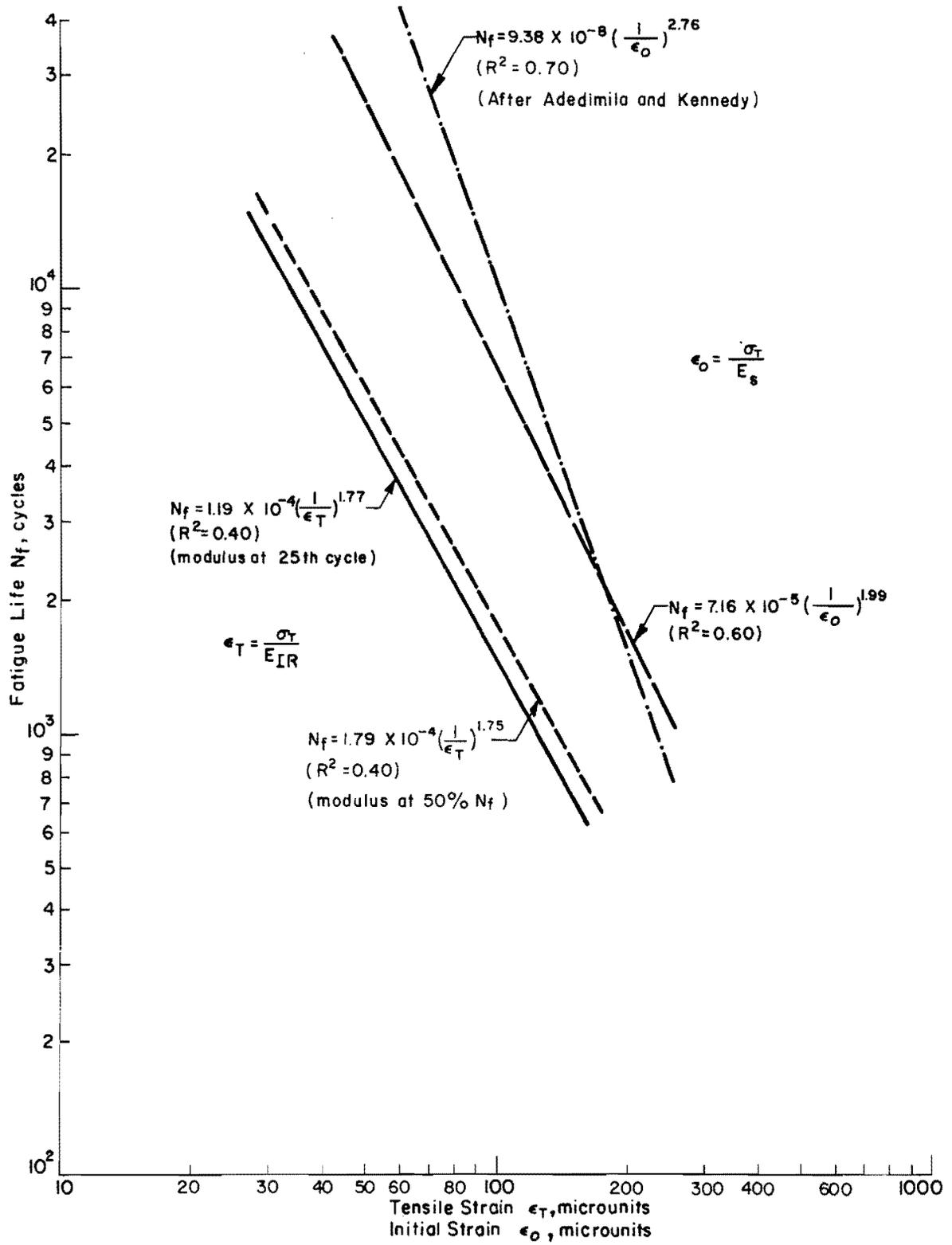
Fig 26. Relationships between fatigue life and strain for Project 14.
