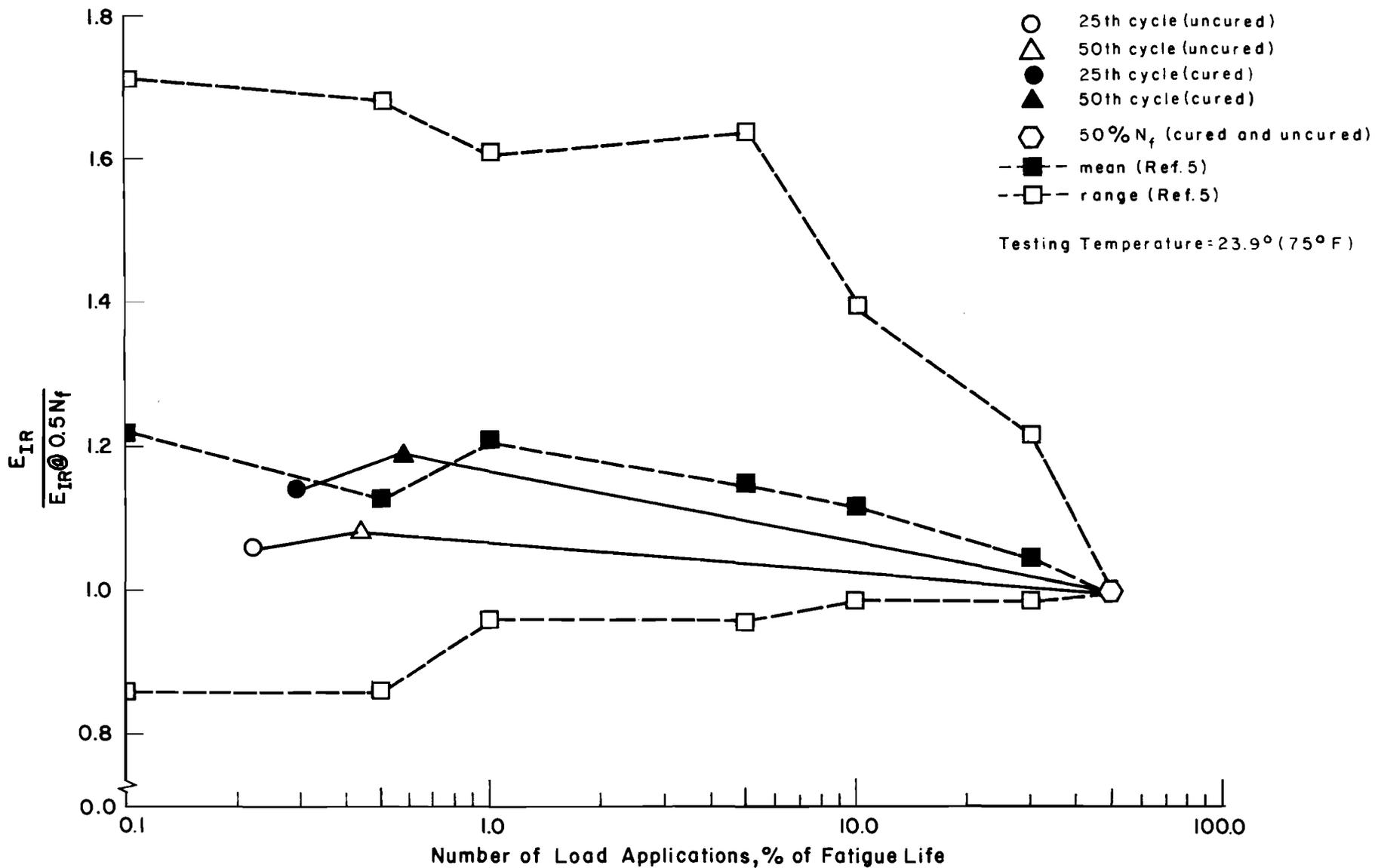
Fig 18. Relationship between resilient modulus and number of load applications for Project 11 (fine).
