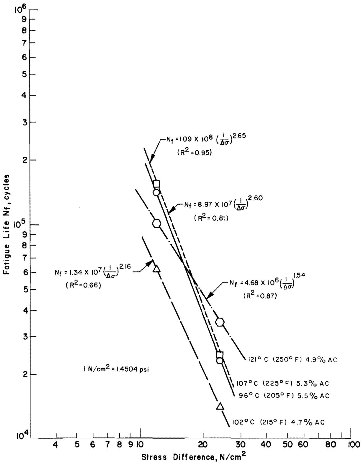
Fig 24. Relationship between the logarithms of fatigue life and stress differences for different mixing temperatures for Project 14.
