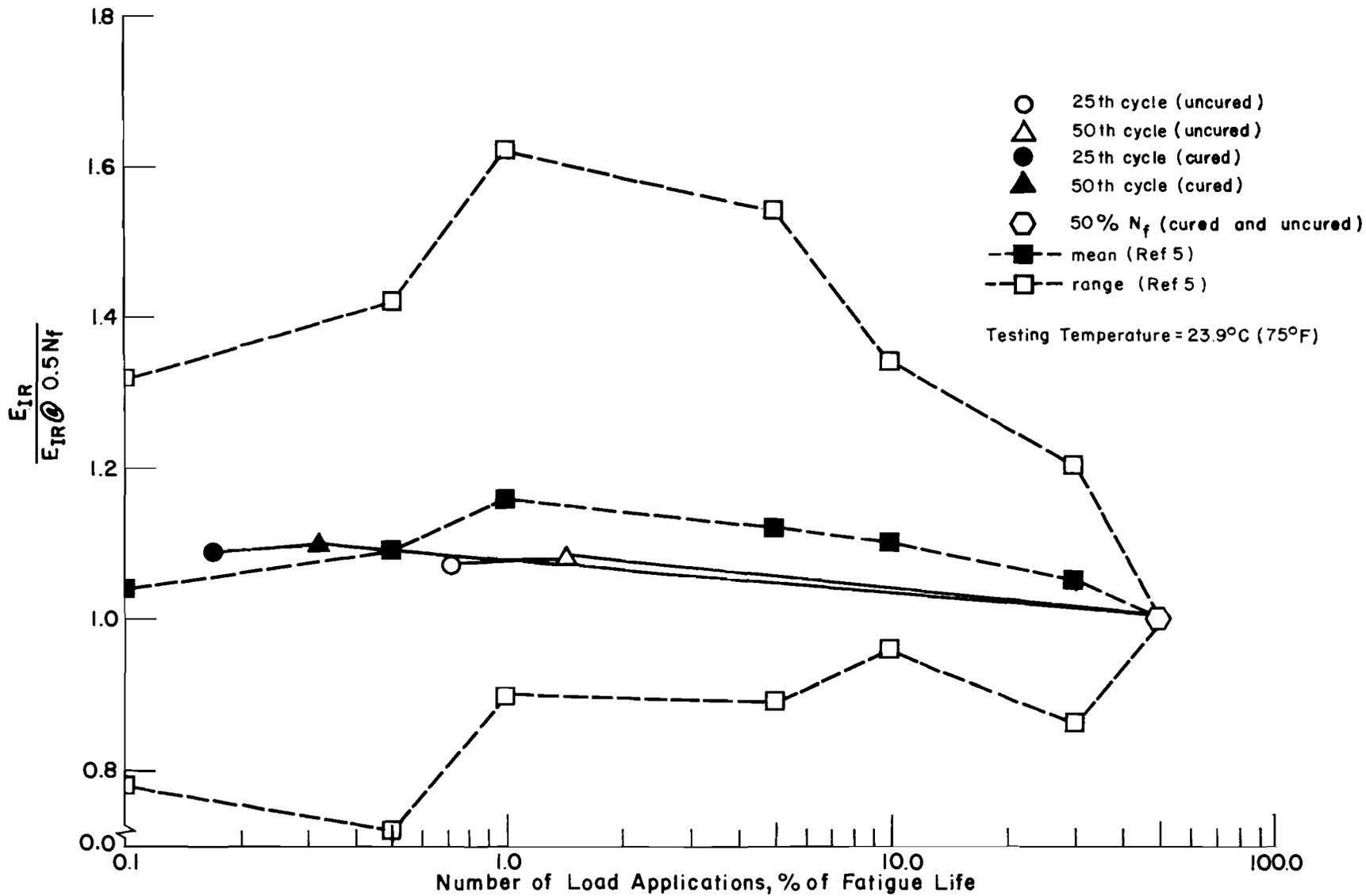
Fig 17. Relationship between instantaneous resilient modulus and number of load applications for Project 21.
