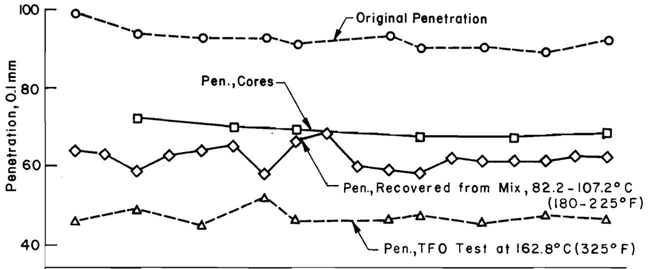
Fig 2. Hardening of 85/100 penetration asphalt for project in Washington (Ref 19).
