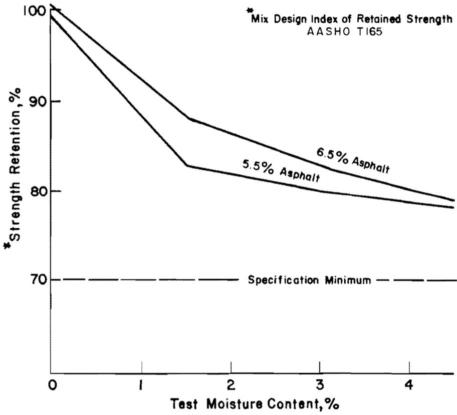
Fig 5. Strength retention after soaking (Ref 19).
