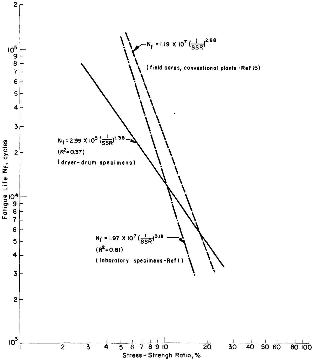
Fig 27. Logarithmic relationships between fatigue life and stress-strength ratio.
