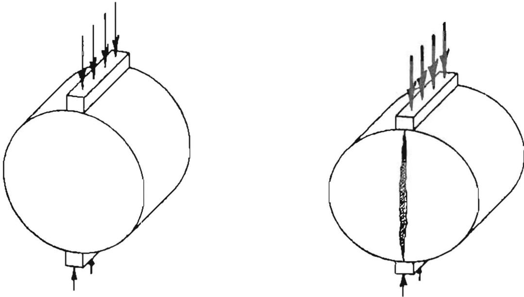
(a) Compressive load being applied.
