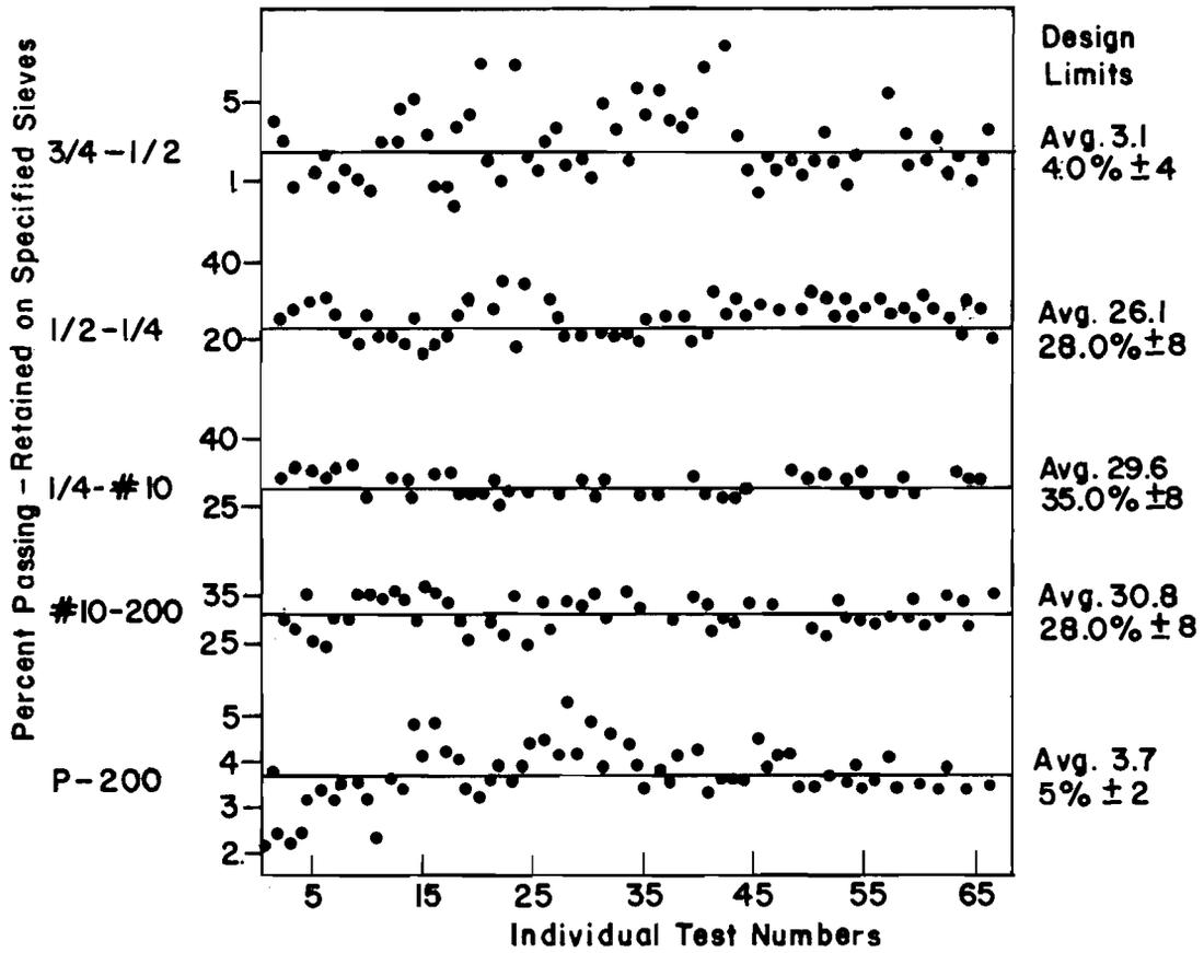
Fig 8. Uniformity of aggregate gradation (Ref 19).
