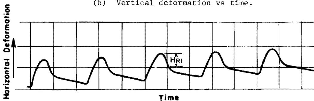
Fig 15. Typical load and deformation versus time relationships for repeated-load indirect tensile test.
