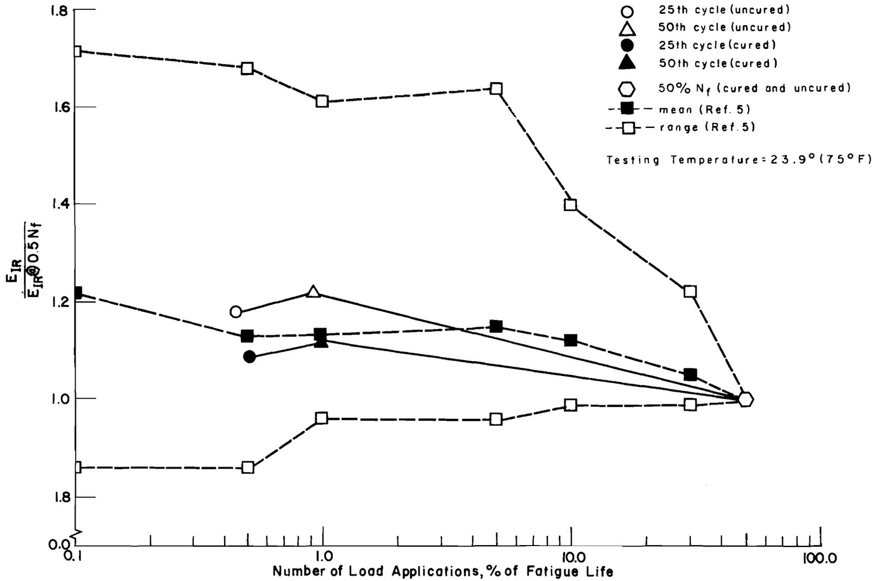
Fig 19. Relationship between resilient modulus and number of load applications for Project 11 (coarse).
