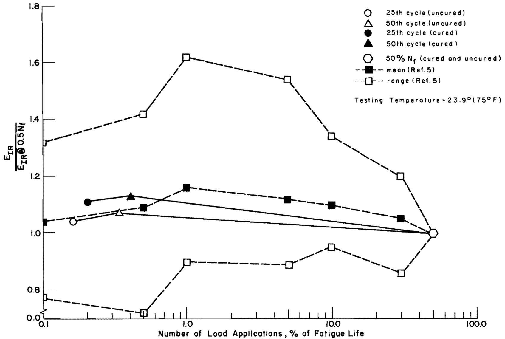
Fig 20. Relationship between resilient modulus and number of load applications for Project 8.
