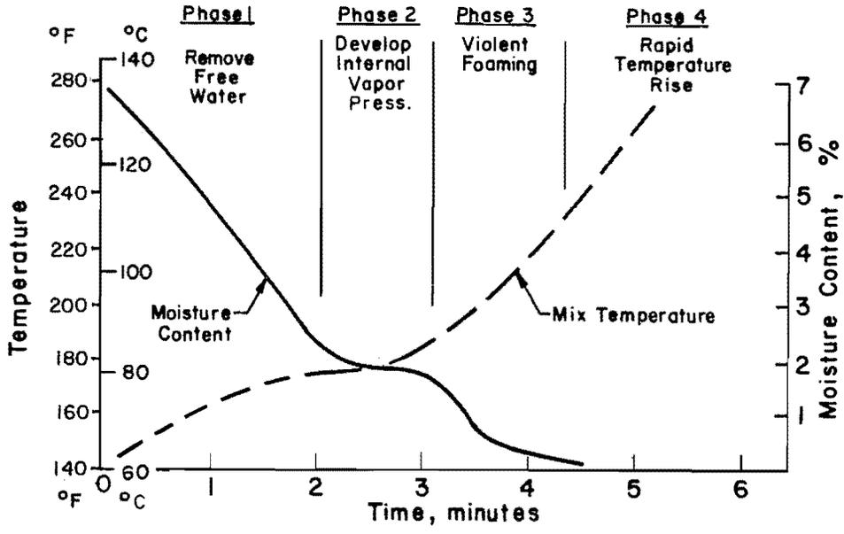
Fig 4. Relationship of moisture and temperature inside the drum (Ref 19).
