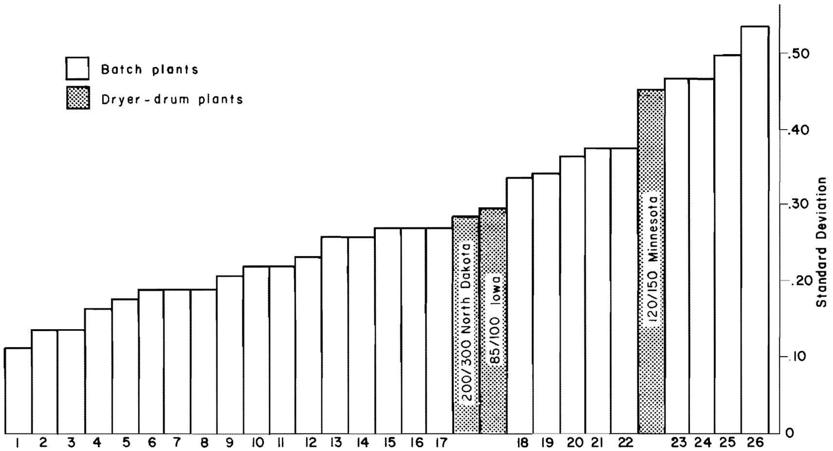
Fig 7. Uniformity of asphalt content (Refs 6 and 7).
