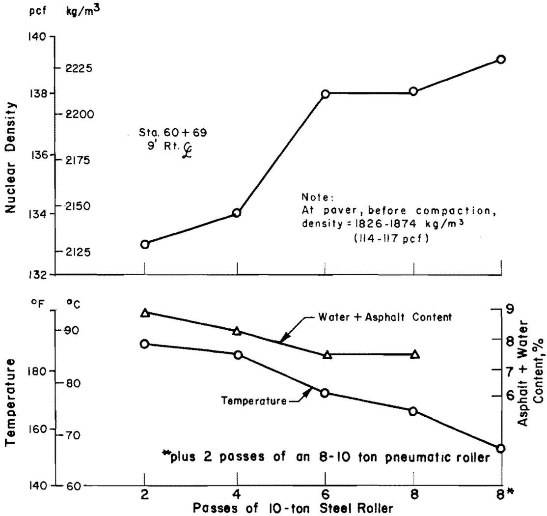
Fig 9. Effect of increased compactive effort during temperature drop and moisture evaporation (Ref 19).
