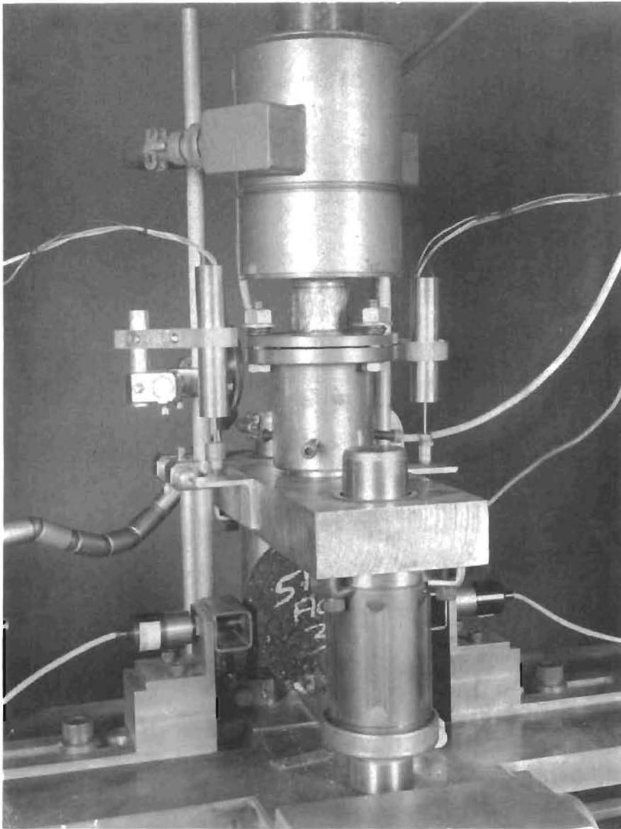
Fig 14. Repeated-load indirect tensile test.
